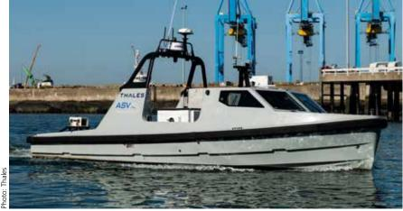
Thales' C-SWEEP ASV features a robust glass-reinforced plastic hull, twin diesel engines and is operated using the ASView Control System.
