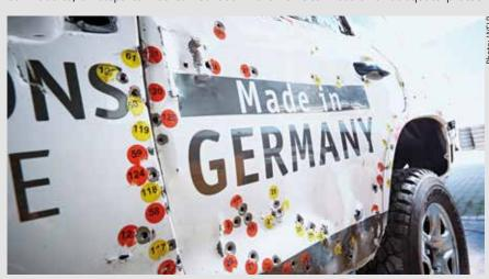
by the company. In addition to this range of automotive services, the Group has extensive expertise in the development and manufacture of highly protected vehicles and modules as well as special vehicles. tion against firearms and explosions. One method that meets these requirements is hot forming, also known as press hardening. With this new technology, we are able to offer unparalleled protective
