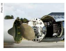
and ELTA. The radar can be installed on a variety of airborne fighters. As one of the leading radars of its type, it is operational in many countries worldwide.
