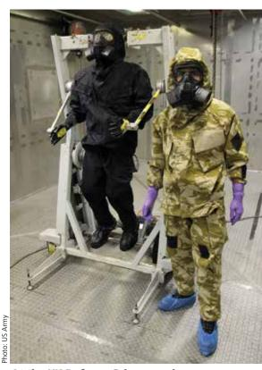
At the UK Defence Science and Technology Laboratory, known as DSTL, a US Army chemist works with the Porton Man, a contaminated mannequin dressed in full protective gear. At DSTL, chemical-protection experts can enter a laboratory to get a first-hand look at chemical-protective ensembles, which enables system-level research and testing.
