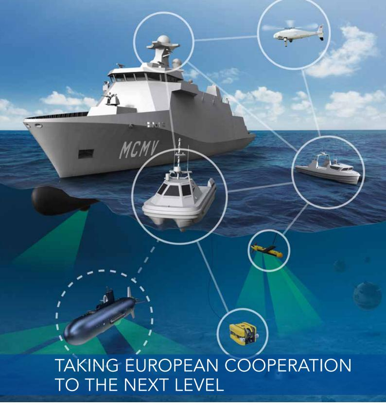
WHEN BELGIUM AND THE NETHERLANDS JOIN FORCES IN REALISING THEIR NAVAL PROGRAMMES, IMTECH BELGIUM AND DAMEN ARE READY TO DELIVER THE FUTURE MINE COUNTER MEASURE VESSELS (MCMV). FITTED WITH A MODULAR TOOLBOX CONSISTING OF UNMANNED AERIAL, SURFACE AND UNDERWATER VEHICLES, THE MCMV WILL BE ABLE TO STAY OUT OF THE MINEFIELD.
