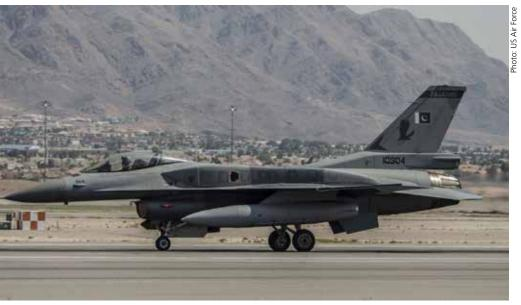
The most modern combat aircraft in the Pakistan Air Force inventory are 12 Lockheed Martin F-16C Block 52 (shown here) and six F-16D Block 52 aircraft delivered under the Peace Drive programme in 2010. Worsening relations with the US could cause problems, especially if spares deliveries are blocked.
