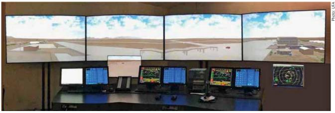
An airport tower simulator at Libby Airfield, Arizona, with four visual control channels and a Fixed Based Precision Approach Radar (FBPAR) system for instrument approaches
