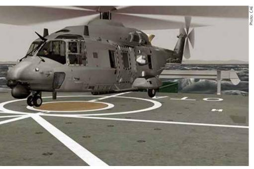
A 700MR Series fixed-base flight training device (FTD) for the NH90 helicopter developed by the Canadian company CAE
