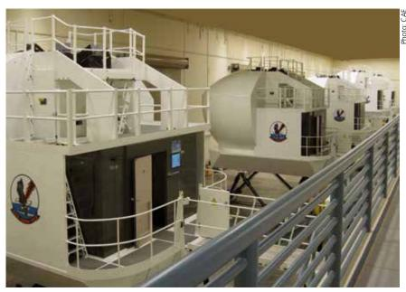
Full flight simulators for the P-8A POSEIDON maritime surveillance aircraft built by CAE
