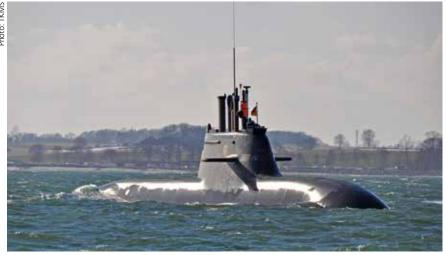
The Type 212A class platforms (six in the German Navy and four in the Italian Navy) with Fuel Cell AIP are equipped with FCM 34 modules, which were developed from 1984 onwards for the German MoD.
