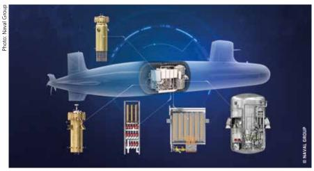
Naval Group has developed a second-generation Fuel Cell AIP (FC-2G) system.
