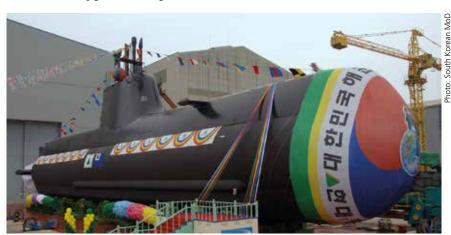
Based on experience gained with the KSS-IIIType 214 depicted here, South Korea's DSME has recently launched a larger next-generation KSS-III boat equipped with an AIP system and domestically produced lithium-ion batteries.
