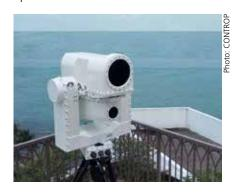
image is updated continuously - every 3 seconds - with automatic and simultaneous detection of any moving targets in the water. A small boat of 3x1 metres can be detected at a distance of 5 nm and more. The TORNADO-ER includes two Thermal Imaging InfraRed (IR) cameras that provide
