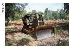
system's performance, including comprehensive testing of the maturity of the technology and its safe integration with combat systems. The new autonomous system incorporates IAI's robot technology based on the customer's operational requirements. The new autonomous bulldozer offers different degrees of autonomy including motion and earthworks for a variety of ap-
