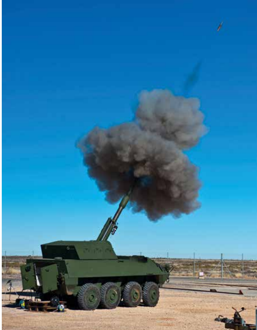
The turreted variant of Denel's long-range 105mm gun during firing trials from a US Army LAV platform
