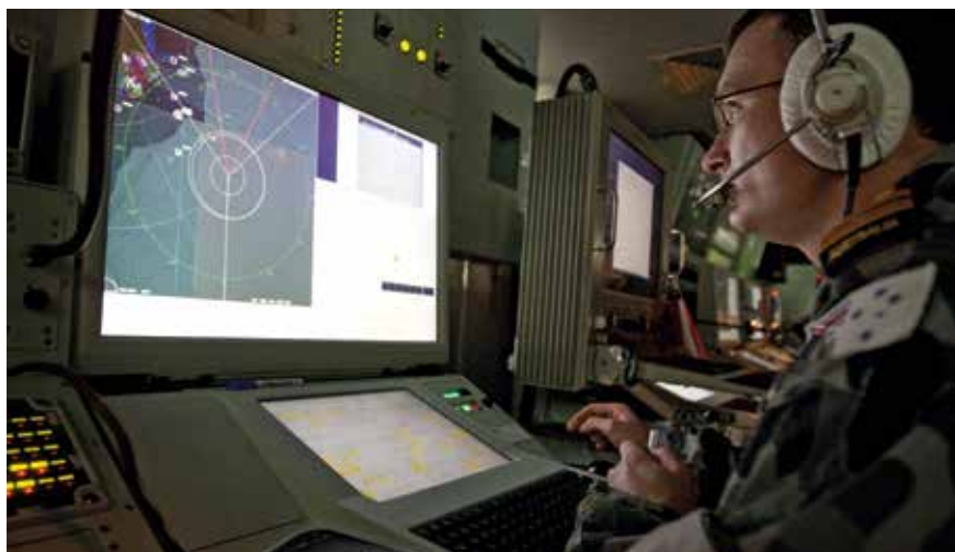
Saab's latest 9LV CMS displays all relevant information on a single large screen console, featuring a 30-inch HD display and a 15-inch table-mounted touch screen.
