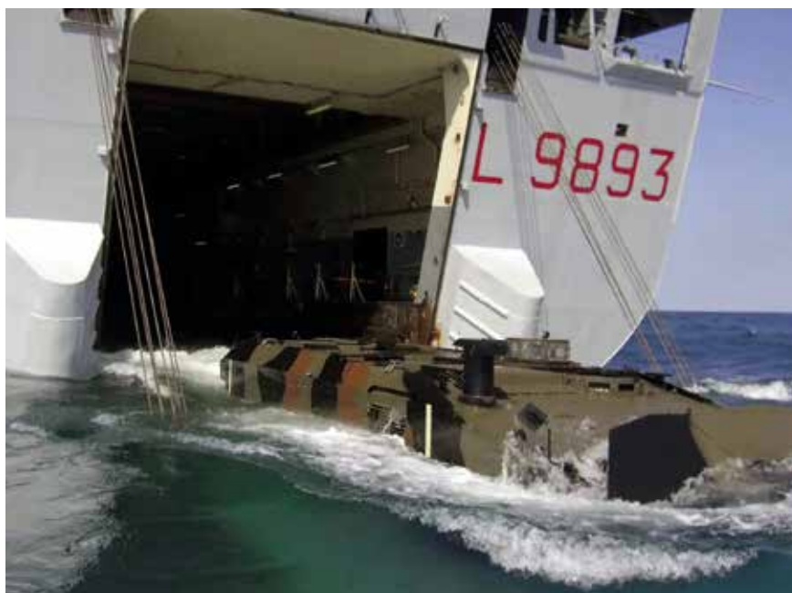
An Iveco 8x8 SUPERAV launched from an LHD-1. The SUPERAV is capable of supporting littoral operations in open ocean beyond sea state 3. The vehicle can carry a 10 t mission load, including an overhead weapon station mounting up to a 40mm cannon. The SUPERAV platform is equipped with a new 700 hp powerpack and driven in water by two propellers.
