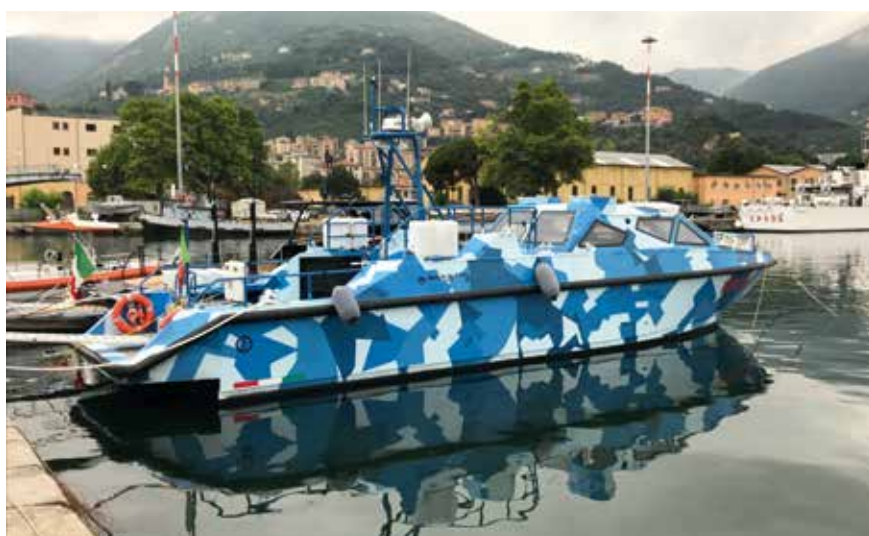
The 15-metre FFC-15 fast multipurpose transport landing vessel designed by Baglietto
