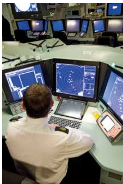
BAE Systems produces the Royal Navy's CMS systems – the OUTFIT DNA(2) fitted to Type 23 frigates and amphibious platforms, and the CMS-1 system for the Type 45 destroyers and the QUEEN ELIZABETH Class aircraft carriers.
