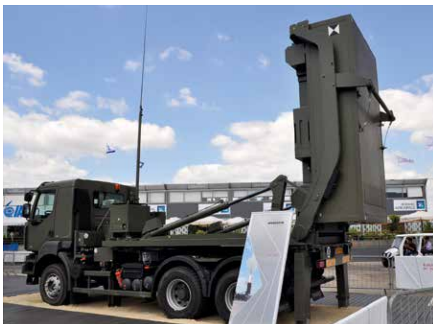
The use of a vertical-launch technique has given MBDA's MICA air-to-air missile an additional SHORAD role. Fighter aircraft and surface-to-air launchers can draw on a common stock of RF – or IR-guided missiles.
