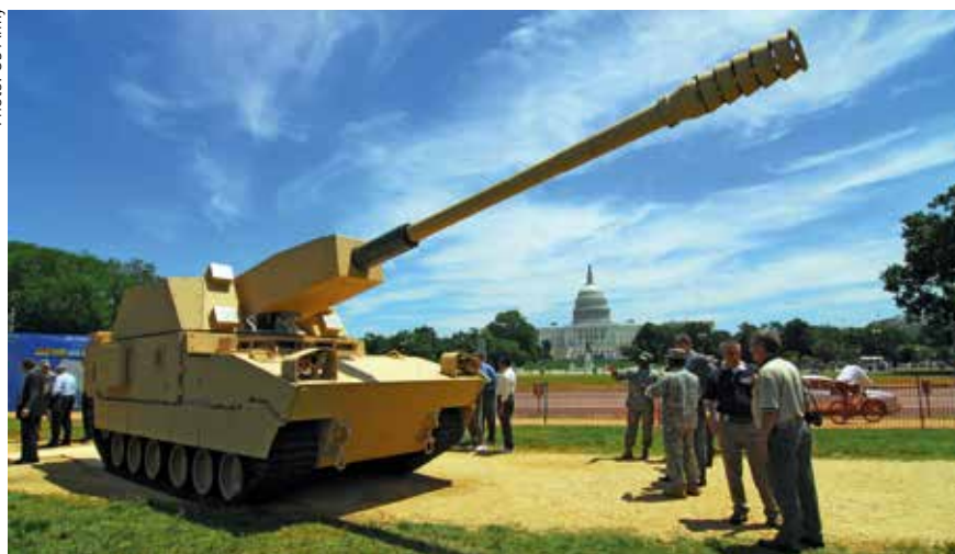
All manned vehicles of the proposed Future Combat System were to be equipped with hybrid drive. The programme was terminated in 2009 over cost issues and technical difficulties, not specifically related to the drive concepts.
