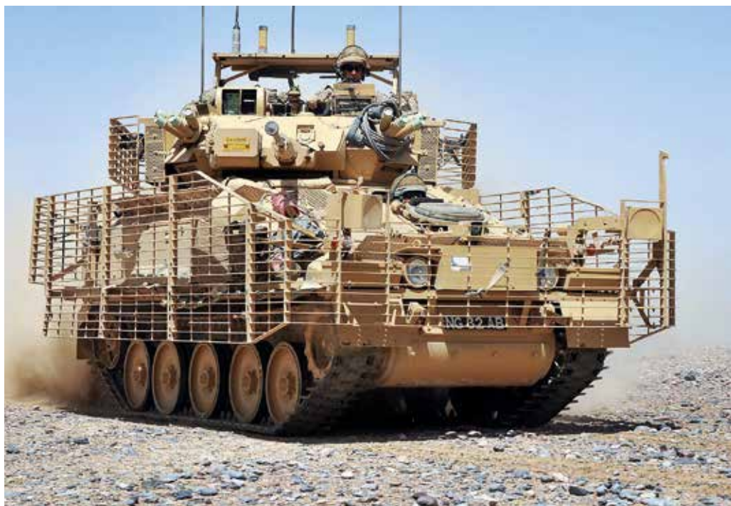
In 2010/2011, BAE Systems were awarded a contract to modernise CVR(T) armoured vehicles to the CVR(T) Mk 2 configuration, as illustrated by this SCIMITAR Mk 2 vehicle on operations in Afghanistan.
