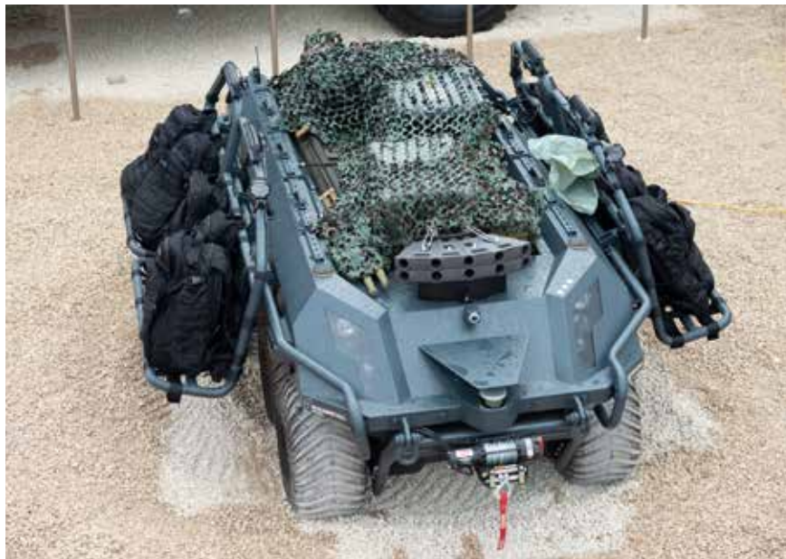
The Rheinmetall Canada MISSION MASTER Unmanned Ground Vehicle (UGV) already has its first export customer. The system is capable of semi-autonomous or autonomous operation, and the cargo variant can carry a 600 kg payload. Systems of this nature are an effective means of reducing infantry combat loads.
