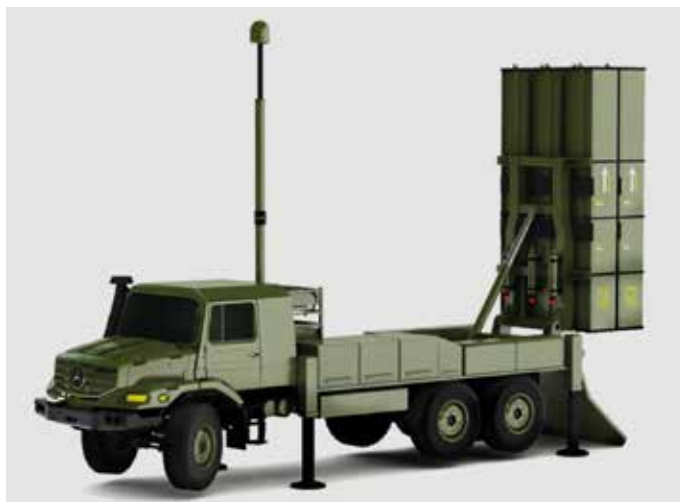
Turkey's HISAR-A will be deployed in the truck-mounted configuration shown here, or on a tracked chassis equipped with vertical launchers.
