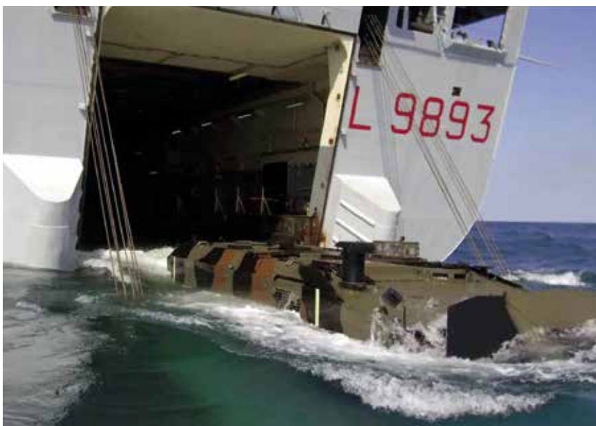
An Iveco 8x8 SUPERAV launched from an LHD-1. The SUPERAV is capable of supporting littoral operations in open ocean beyond sea state 3. The vehicle can carry a 10 t mission load, including an overhead weapon station mounting up to a 40mm cannon. The SUPERAV platform is equipped with a new 700 hp powerpack and driven in water by two propellers.
