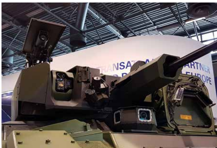
Turret of an ASCOD 2 AJAX showing add-on armour and optronics protection
