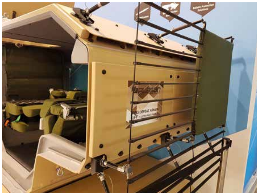
Different types of add-on armour and anti-RPG protection developed by Plasan
