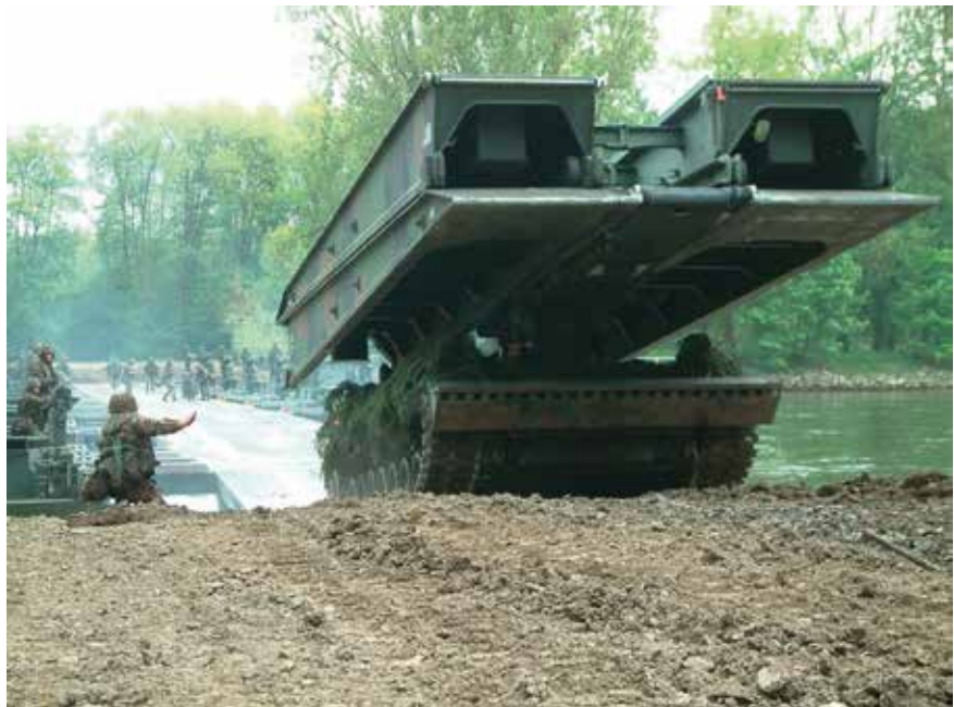
The BIBER Armoured Vehicle Launched Bridge (AVLB) is in service with the armies of Australia, Canada, Chile, Denmark, Germany, Italy, The Netherlands and Poland.
