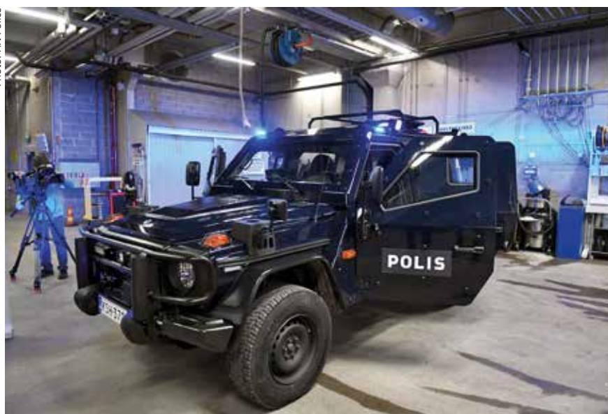
A Mercedes-Benz G280 CDI LAPV 5.4 ENOK armoured vehicle of the Helsinki Police Department. The vehicle was designed and built by ACS; Mercedes-Benz is the prime contractor in Finland for this project.
