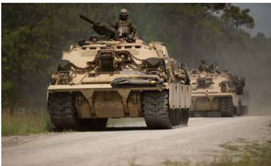
A pair of M88A2 HERCULES ARV systems of the US Marine Corps on exercise at Camp Lejeune. The M88A2 is the third generation of this ARV family to enter US service and was developed to recover the M1 ABRAMS, which was beyond the capabilities of the earlier M88A1. Now an M88A3 variant is being proposed to cope with even heavier M1 tank variants.
