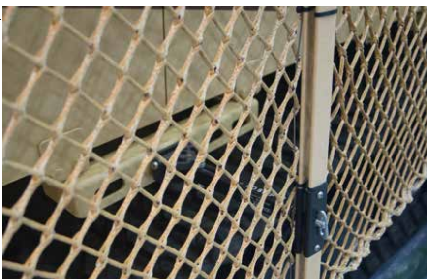
The TARIAN RPG net is designed to reduce vulnerability to RPGs.
