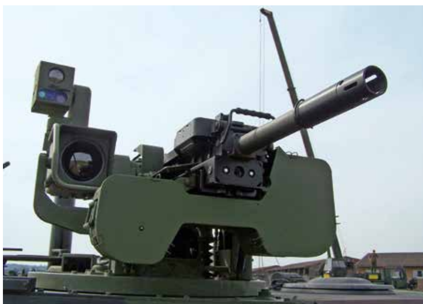
A Heckler & Koch GMG automatic grenade launcher mounted on a German Army FENNEK light armoured reconnaissance vehicle
