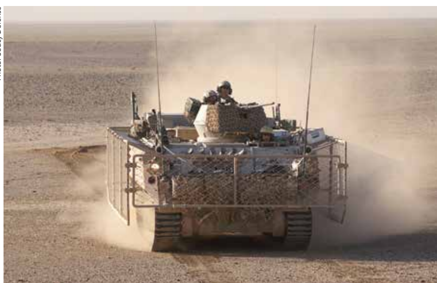
An M113 in Afghanistan fitted with Soucy CRT: Traditionally, the M113 runs on single-pin tracks.
