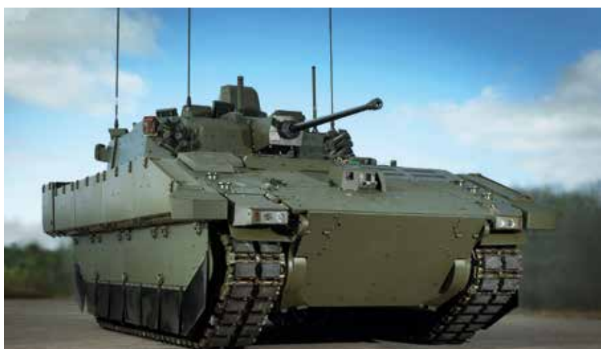
The UK's AJAX Infantry Fighting Vehicle will feature the CTAS weapon system, including a 40mm autocannon firing cased telescopic ammunition.
