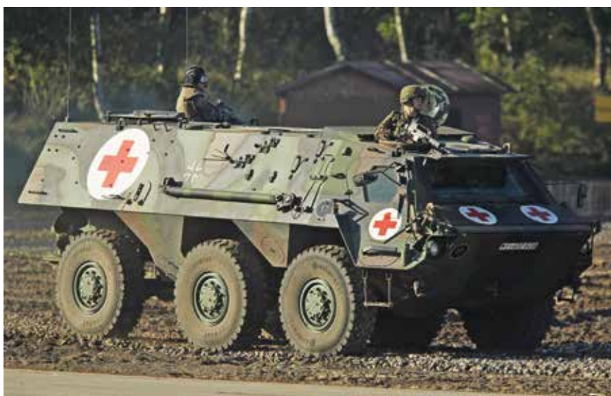
A legacy vehicle, the Tpz1 FUCHS is still in service in the German Army; such ambulances have been brought up to the A4 standard but are no longer used in high-risk scenarios.
