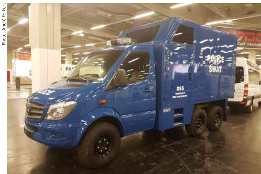
A protected Mercedes-Benz SPRINTER 6x6 designed by Carl Friedrich GmbH for Police Special Forces operations.
