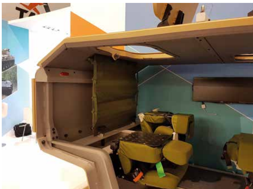
A curtain-shaped spall liner designed by Plasan
