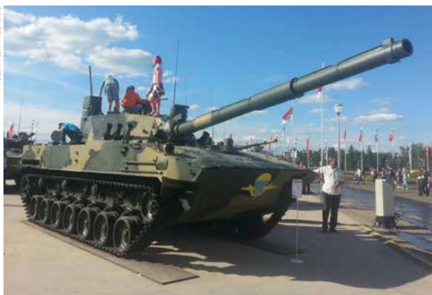
The SPRUT SDM-1 light tank/tank destroyer is capable of conducting amphibious landings and being airdropped. The 125mm cannon can fire regular tank shells and ATGMs.
