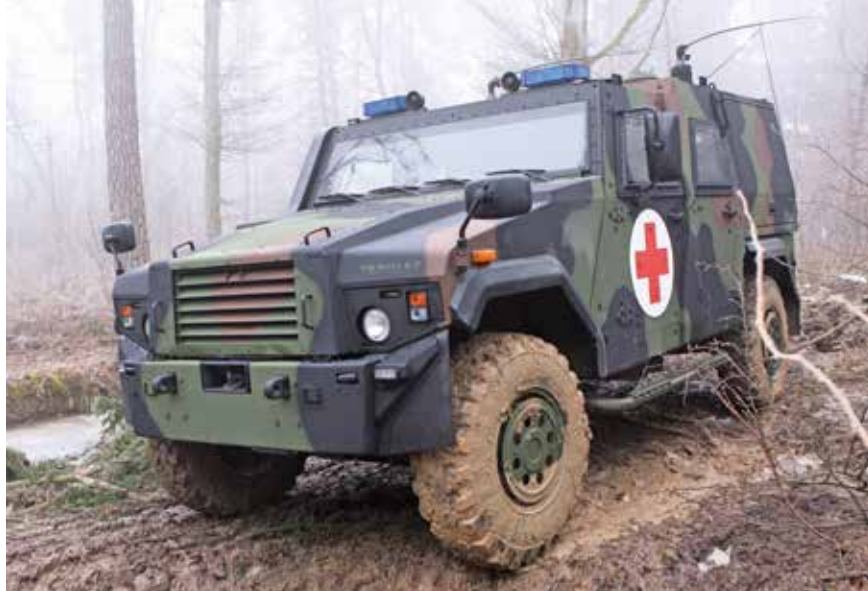
The EAGLE is the lightest armoured ambulance fielded by the German Army; it allows light infantry units to be supported when operating in constricted terrain.
