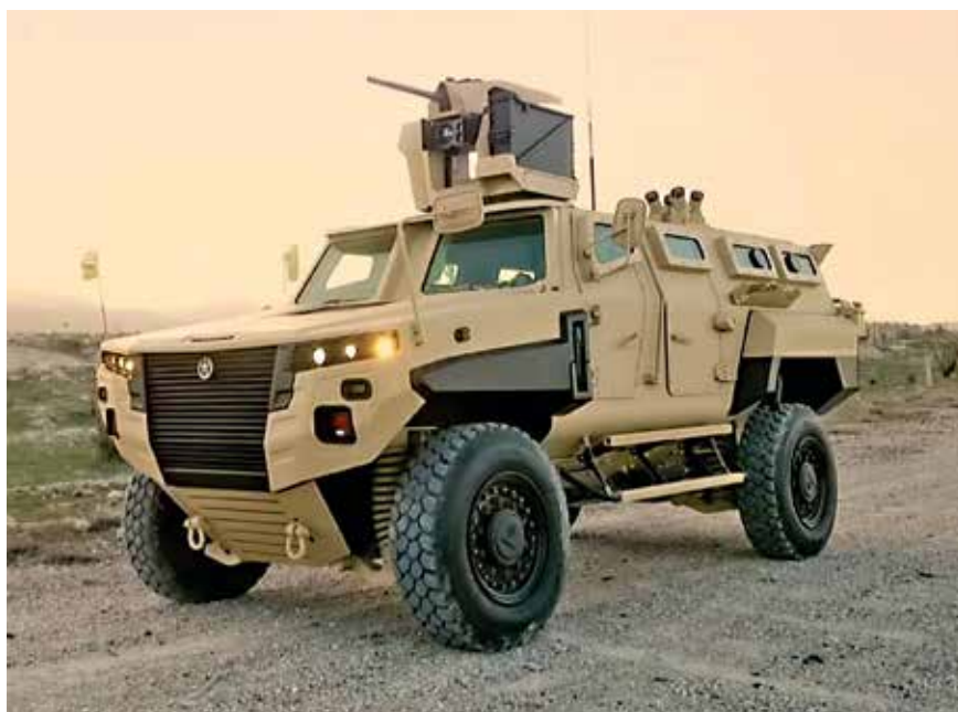
The PUSAT 4x4 developed by TUMOSAN is a 12-tonne vehicle with a 5.2-litre 250 hp diesel engine.
