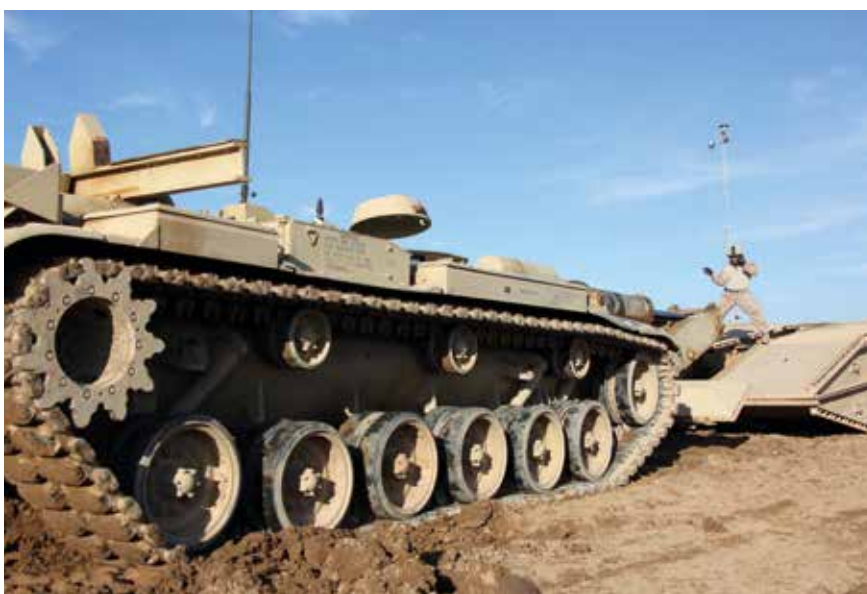
The M60 AVLB deploying its MLC 70 class bridge in Afghanistan. The AVLB is based on the M60A1 chassis, which caused a problem when the M1 ABRAMS came into service, as the AVLB could not keep up with the faster tank. The M60 AVLB remains in US service, as the planned full replacement programme in the shape of the WOLVERINE system never took place.
