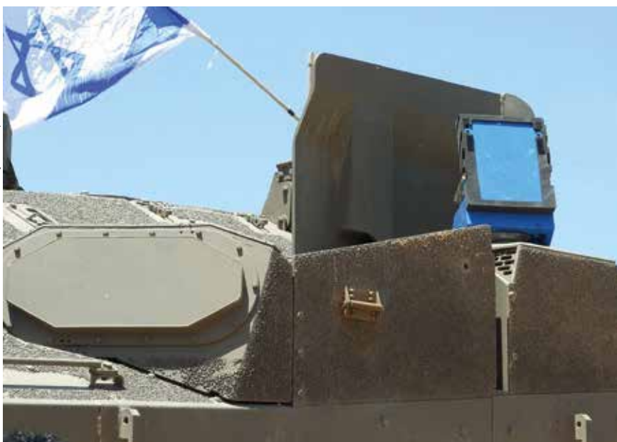
TROPHY system with AESA radar (left) and a dummy launcher on a MERKAVA MBT
