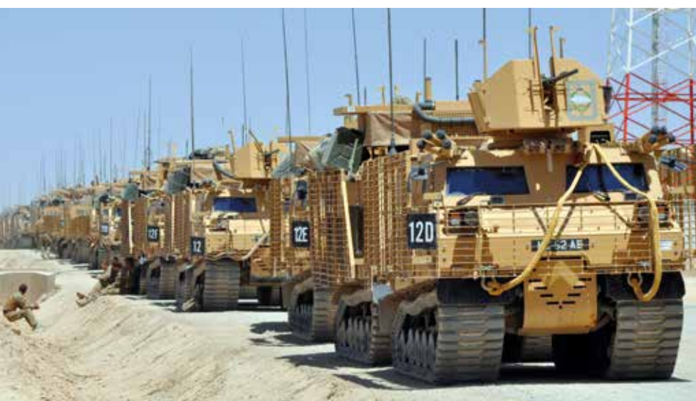
BRONCO vehicles fitted with Soucy CRT. Usually, heavier vehicles require double-pin tracks with an increased surface area for a greater load-carrying capacity.
