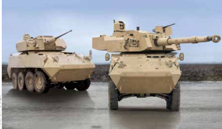
The COCKERILL 3000 family of turrets can accommodate guns between 25mm and 105mm. Displayed here are the 30mm and 105mm versions.
