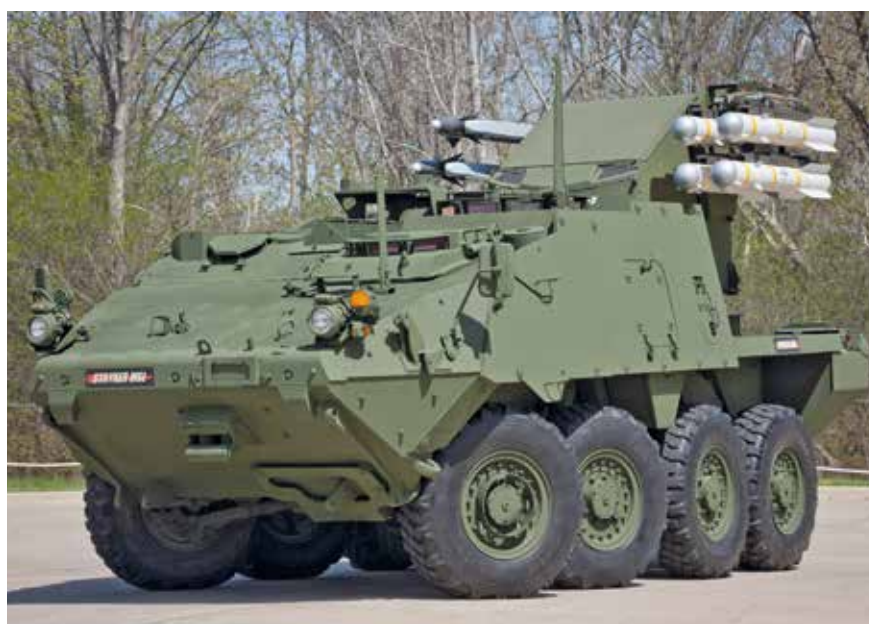
A STRYKER Mobile SHORAD Launcher – a STRYKER prototype configured for the SHORAD role with HELLFIRE missiles
