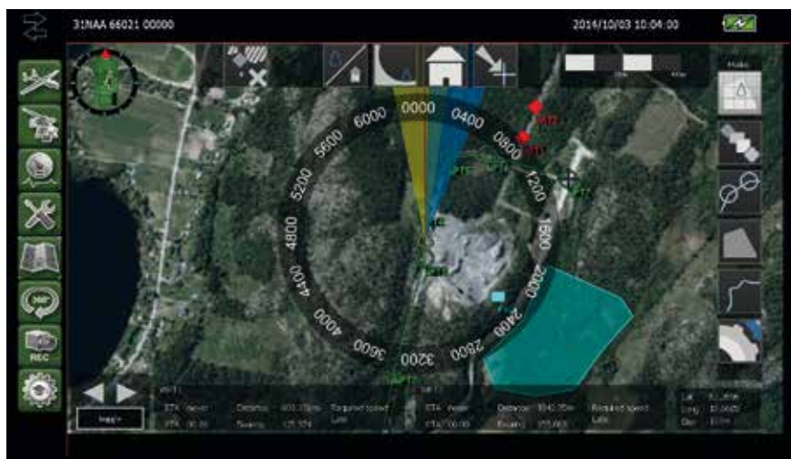
BAE Systems' Battlview 360 display displays the outside view as seen by the panoramic camera with overlaid navigational and tactical data layers.
