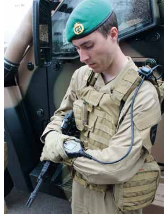
Demonstrator of the Norwegian Modular Network Soldier – the operation and display device is worn on the arm.
