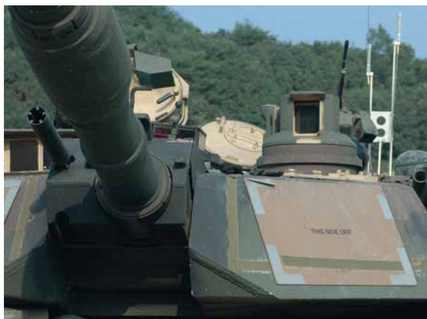
Raytheon's Commanders' Independent Thermal Viewer (CITV) on a M1A2
