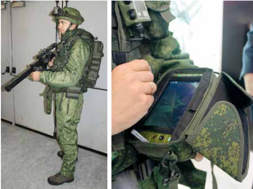
The Russian RATNIK soldier system, which includes the STRELETS command system, can also use GPS as well as the Russian counterpart GLONASS. The equipment for command personnel includes portable command computers, such as the Commanding Officer Manpack Kit, which covers the chain of command of company-platoon-squad-individual soldier.
