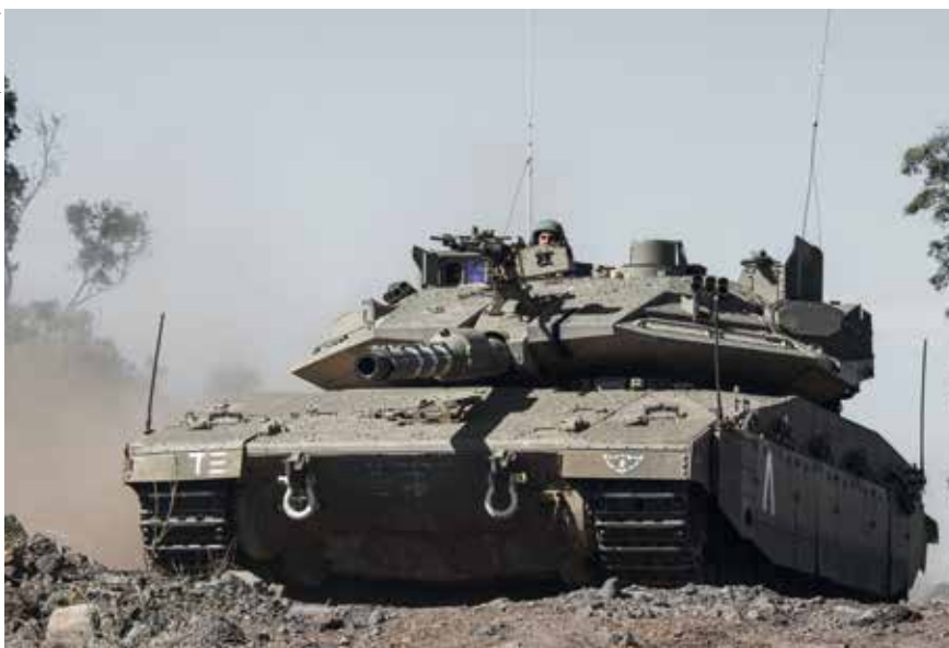
Israel's MERKAVA Mk4m is equipped with the TROPHY active protection system. The system's radar (developed by IAI Elta) also adds situational awareness to the crew.
