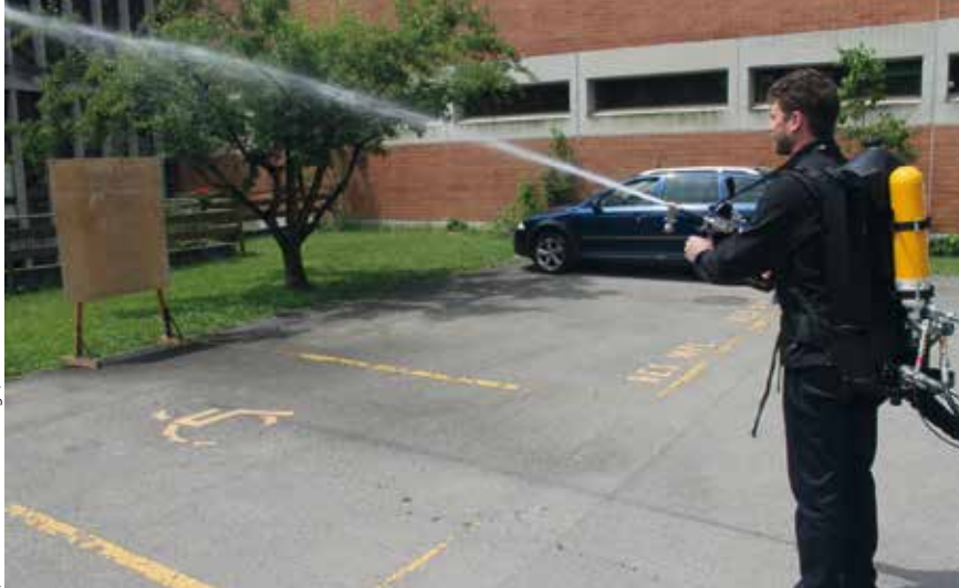
The TW1000/RWG10/2 irritant projector in jet mode
