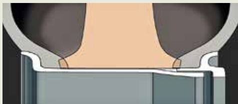
Figure 1 showing how a rubber runflat ensures beadlock.
