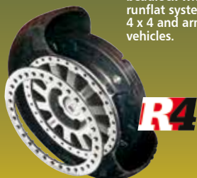
Tyron Multi Band - the low cost, short distance runflat system. Approved by NATO and used by the MOD.
