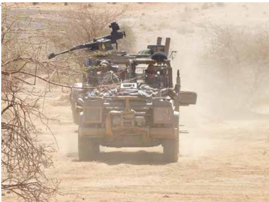
Vehicle-Mounted V-AMMS by Microflown. Sensor is above the driver.
