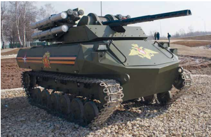
The Russian URAN-9 Unmanned Ground Combat Vehicle carries automatic cannon, coaxial MG, and antitank projectiles.
