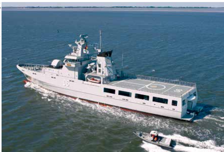
Lürssen's OPV 80 has been designed to deploy up to four RHIBs, e.g. in the context of operations against irregular forces.
