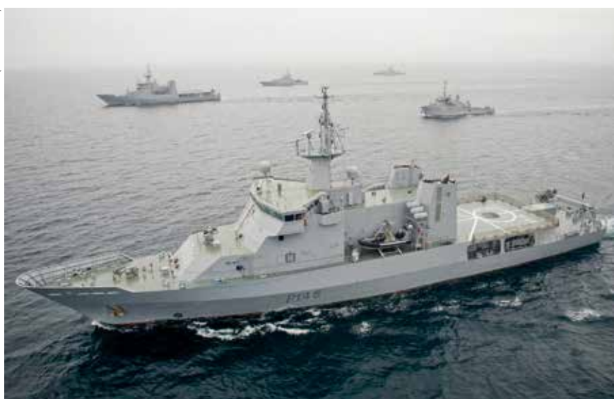
The PROTECTOR Class OPVs of the RNZN (pictured here is HMNZS OTAGO) have a range of 6,000 nautical miles and can deploy two RHIBs (or one RHIB for special forces missions). The weapons fit comprises a 25mm Bushmaster automatic cannon and two .50 cal. machine guns.
