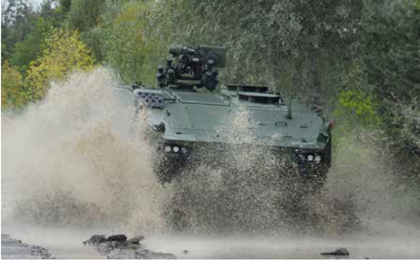
PIRANHA V in APC configuration with machine gun and smoke launchers
