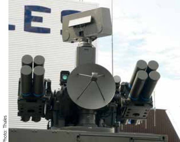
CROTALE NG – seen here at the 2007 Paris Air Show – was the final variant of this widely-exported French SHORAD. It uses the VT-1 missile developed by what was then LTV Missiles and Electronics Group.
