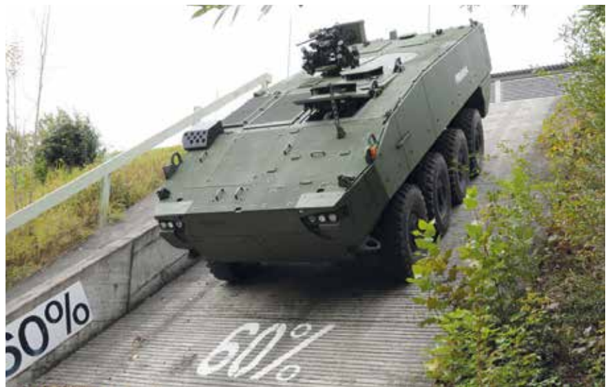
The vehicle during performance tests. The rope cutter in front of the open hatch is to support protection against IEDs.
