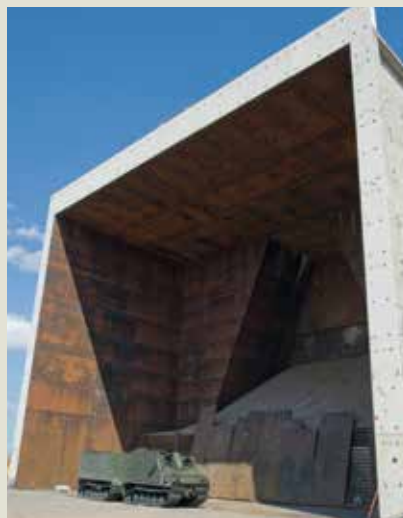
The Karlsborg Test Range offers one of the largest catch boxes in the world at (25m x 20m x 35m).
