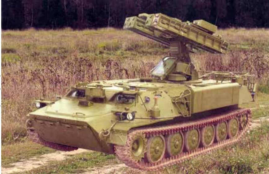
Russia offers the widely-deployed STRELA-10 (SA-13 GOPHER) VSHORAD system in the upgraded 10M4 version shown here.
