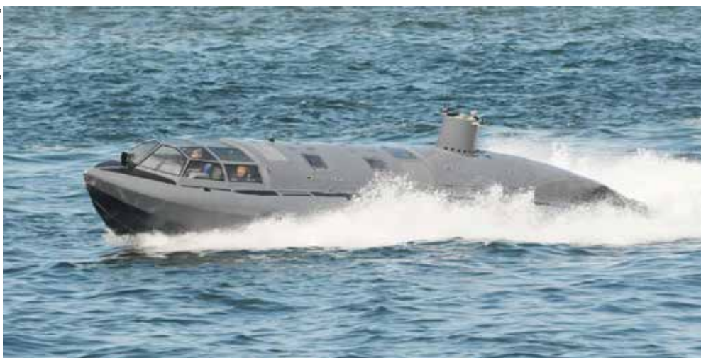
The South Korean company Vogo Engineering has been developing and manufacturing SDVs for many years. Here is the 35 knot, 10-man, 1.5 tonne SDV 1000.
