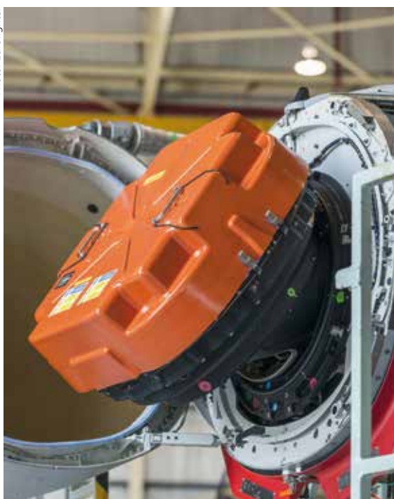
The CAPTOR-E antenna can be repositioned well off the centreline of the aircraft. While the US, France and Russia allow fighter-mounted AESA antennas to be photographed, the CAPTOR-E antenna coyly lurks behind a cover in all the photographs released to date.
