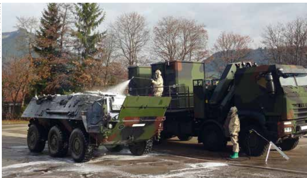
TEP 90 from Kärcher Futuretech/Veco is the modular decontamination system of the Bundeswehr.
