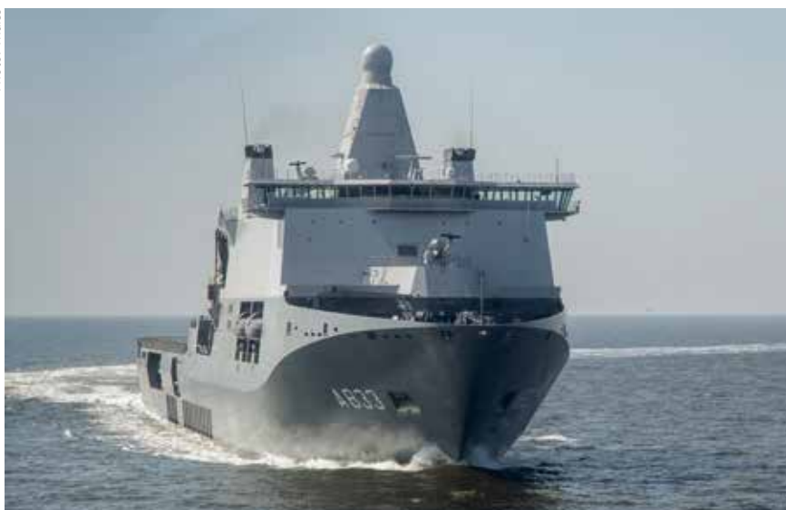
The Integrated Mast from Thales onboard the HNLMS KAREL DOORMAN. The company is working on a successor, called the Integrated Sensor Suite.
