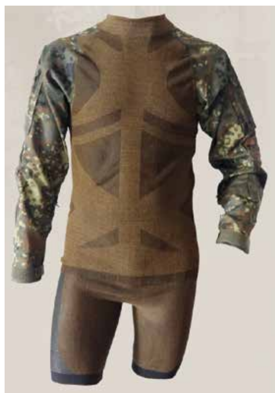
Using the latest ballistic fibers, Hexonia developed a knitted ballistic underwear that protects against fragments and blast. The strong polyethylene, knitted seamless, reduces the depth and number of penetrating fragments and the product's high burst load and tearing strength makes it withstand blast waves. By adjusting weave and thickness different ballistic requirements can be met.
