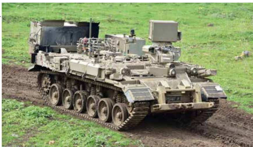
Rafael's THOR add-on system for armoured and up-armoured vehicles uses high-energy lasers to provide rapid route clearance and neutralise explosive hazards
