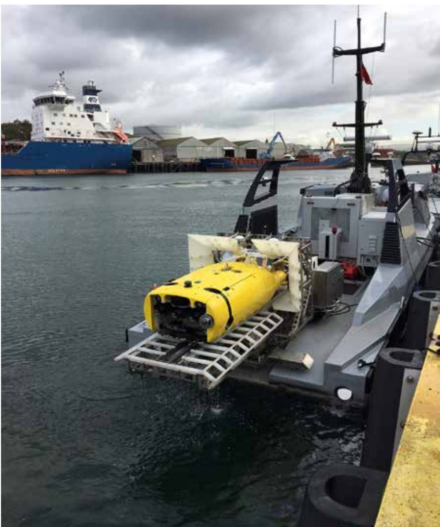
The French/UK MMCM mission package will use the Saab MuMNS (Multi-Shot Mine Neutralisation System) ROV to-relocate and neutralise the threat. The MuMNS is equipped with three reloadable munitions to accomplish multiple neutralisations in one mission.
