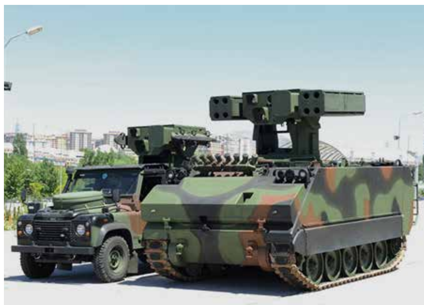
The sensor fit mounted in the central section of the turret carried by Aselsan's ATILGAN mobile short-range SAM system includes a second-generation, two-field-of-view focal plane array thermal imager.
