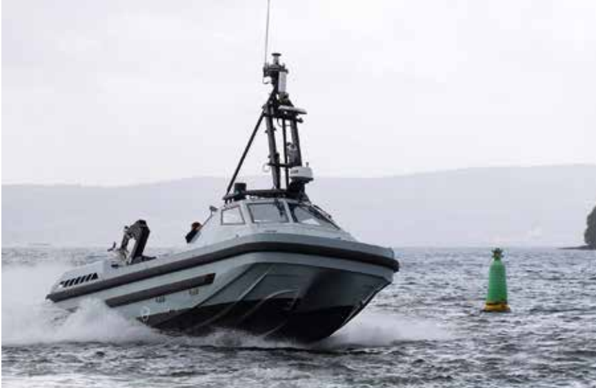
The Atlas Elektronik UK (AEUK) autonomous ARCIMS USV will be used by the Royal Navy for minehunting applications, hydrographic and mine-sweeping operations, in the latter case with a system developed by AEUK.
