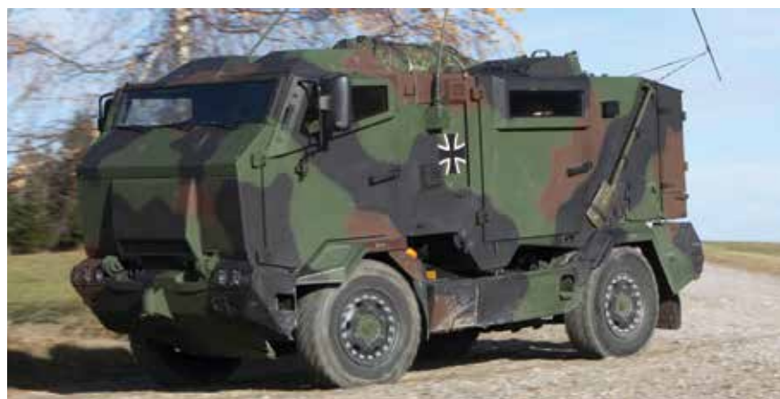
The MUNGO CBRN recce vehicle enables NIC detection and preliminary identification of NBC agents and comparable industrial hazardous substances. It can also be used to monitor contamination and document its extent.
