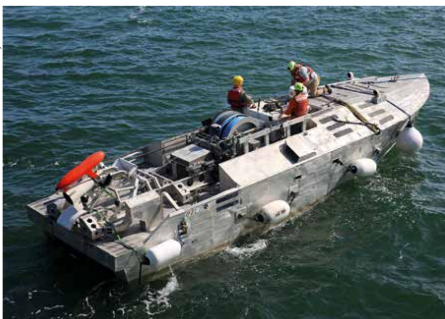
The Textron Systems 12.7-metre long Common Unmanned Surface Vessel (CUSV) will deploy from LCS and vessels of opportunity carrying alternatively the same company UISS (Unmanned Influence Sweep System) or the remote minehunting mission equipment.
