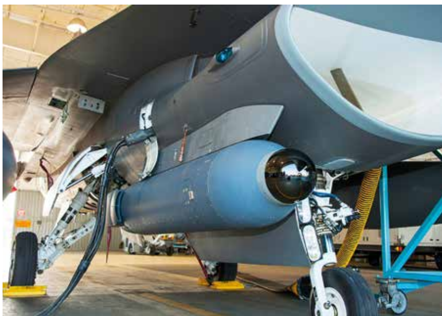
Suitable for installation on one of the external weapon stations of an F-16 fighter, the Lockheed Martin LEGION POD currently carries a nose-mounted passive long-wave infrared receiver, but could be modified to accommodate other types of sensor.
