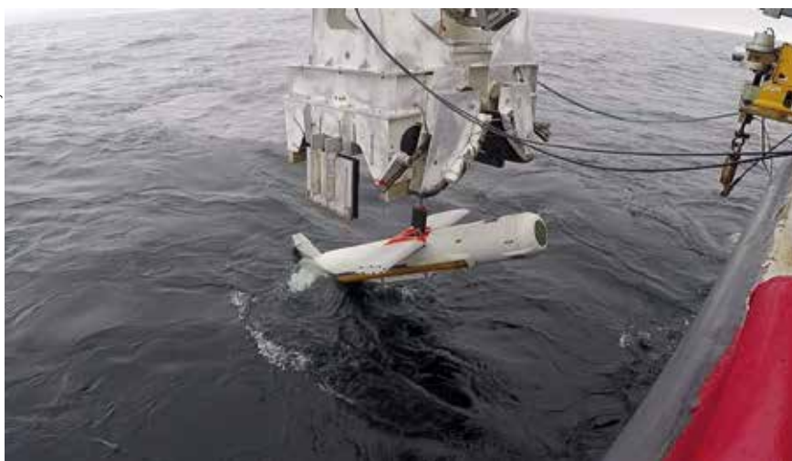
The Raytheon AN/AQS-20C towed minehunting sonar together with the future BARRACUDA mine neutralisation system will provide the US Navy a full-cycle semi-autonomous MCM capability.
