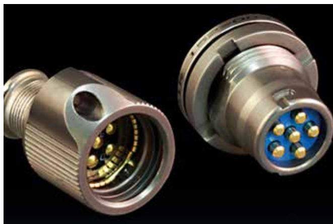
Vibration lab tests on the Series 151 MIL-DTL-55116 reproduce conditions that might be encountered in a moving armoured vehicle. In temperature cycling tests, the Glenair Series 151 MIL-DTL-55116 must be capable of five cycles of mating/unmating while meeting all electrical and air leakage requirements in conditions from -55°C to +85°C.
