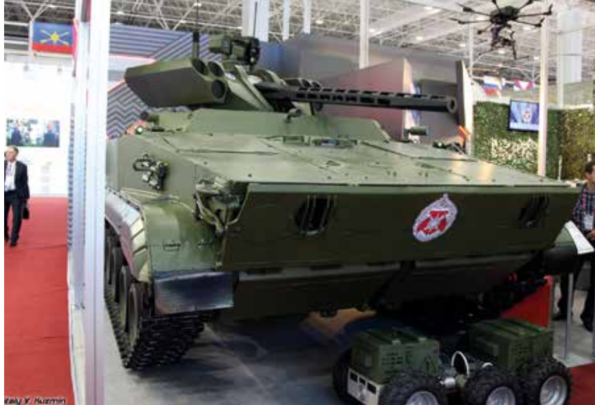
The VIKHR reconnaissance-attack ground robotic system with ABM-BSM 30 combat module based on the BMP-3 platform
