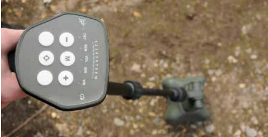
GroundHunter Multi-Head Detection System (MHDS) is the world's first IED detector to have interchangeable command wire and metal detection heads. This allows search teams to respond rapidly to changing search requirements.
