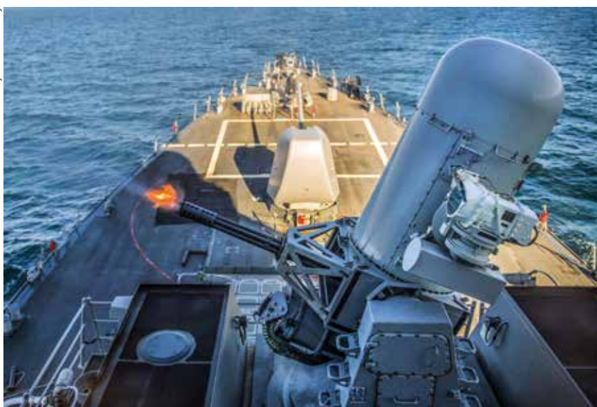
The Raytheon Mk15 CIWS in the PHALANX version with the six-barrel 20mm Gatling gun M61A1 is the subject of a development programme to replace the current pneumatic gun drive systems with an electric gun drive system.
