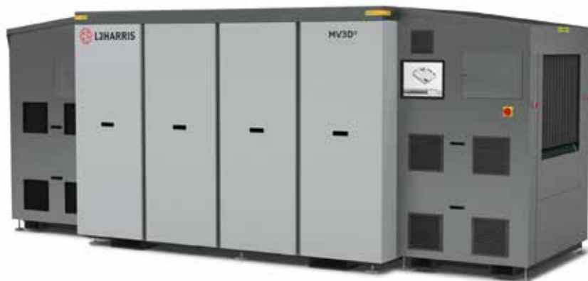
The ultra-high-speed, dual-energy MV3D can scan at a rate of 1,800 bags per hour and uses a series of fixed X-ray sources and multiple detector arrays to create high resolution 2D and 3D images of target objects.
