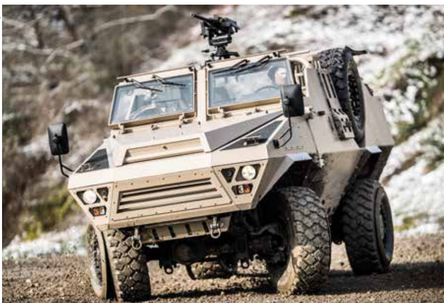
Arquus' PATSAS is based on the BASTION armoured personnel carrier.
