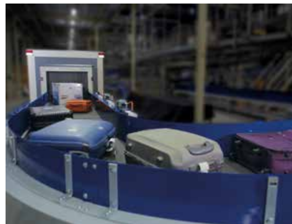
Smiths Detection's HI-SCAN 10080 XCT is a dual-energy scanner that can handle 1,800 bags per hour. The system is currently being trialled at Sydney Airport in Australia.
