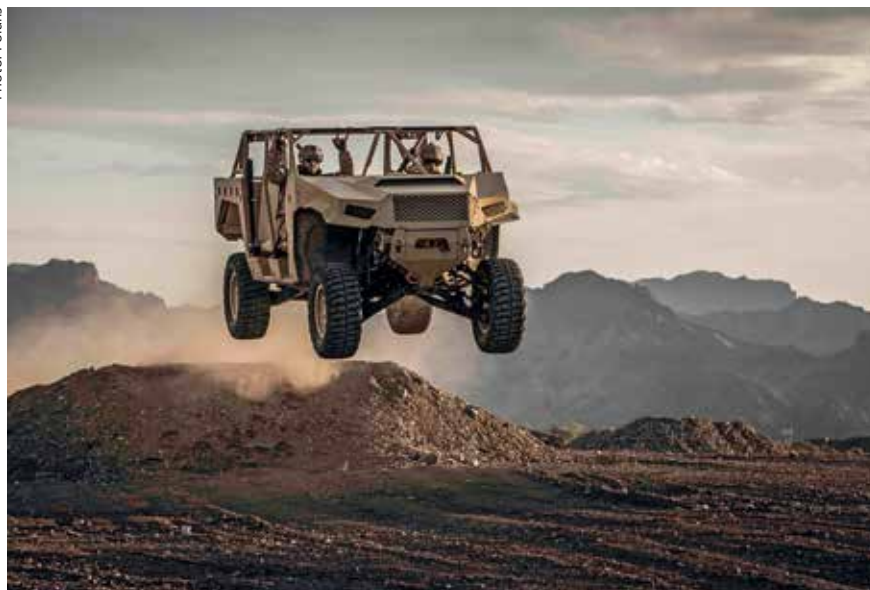
The Polaris DAGOR's suspension is based on desert racing vehicle technology.
