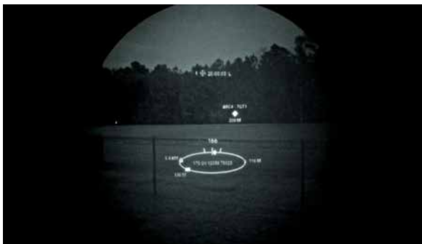
The company Thermoteknix offers the CoVid video injection unit, which enables users to view HUD data covertly for combat operations in complete darkness.
