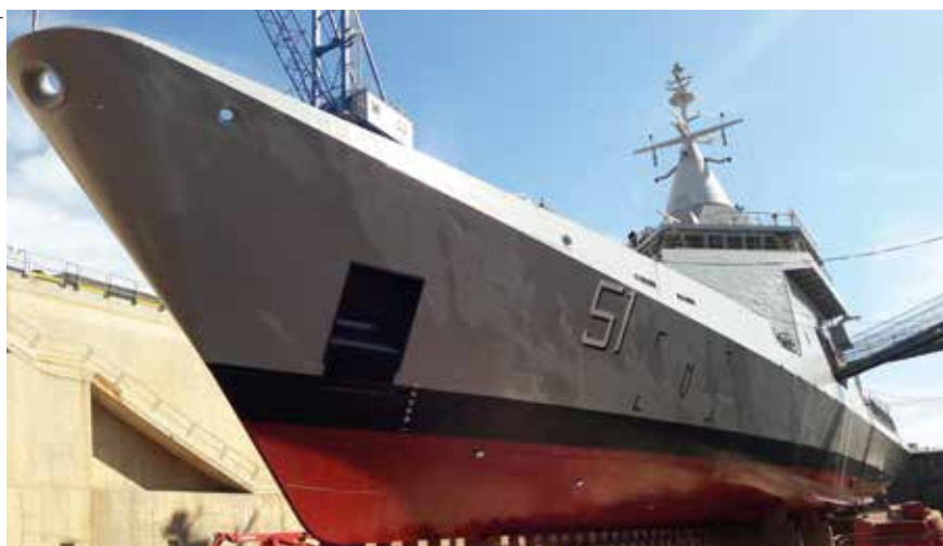
The French-built GOWIND type OPV L'ADROIT pictured under refit prior to its transfer to Argentina as BOUCHARD at the end of 2019. A variant of the design is a potential contender for future French OPV construction.
