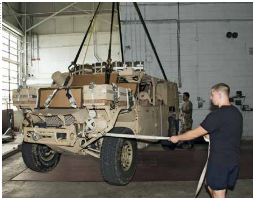
Soldiers rig the Ground Mobility Vehicle 1.1 (GMV 1.1) to assess its suitability for aerial delivery with current parachute systems, rigging materials, and rigging procedures. The GMV v1.1 supports tactical operators in both urban and non-urban environments across the full range of Special Operations Forces (SOF) military operations and terrain profiles.
