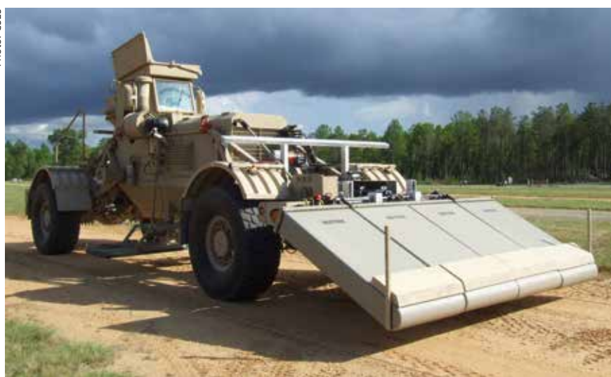
The HMDS (Husky-Mounted Detection System) Wire Detector system consists of up to six PODS sensors integrated into a single assembly routed into a Vehicle Interface Box feeding into the GPR. The sensor array is located forward of the vehicle front bumper to provide detection prior to overpass.
