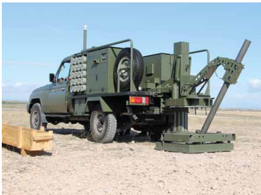
A Toyota LAND CRUISER 4x4 with the Spanish ALAKRAN 81mm mortar system lowered to the ground over the rear
