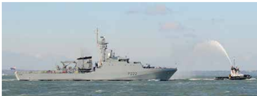
The lead Batch II RIVER class OPV FORTH seen entering Portsmouth Harbour in 2018. Although lightly armed, the design uses a frigate-type hull form and incorporates a capable combat management system.
