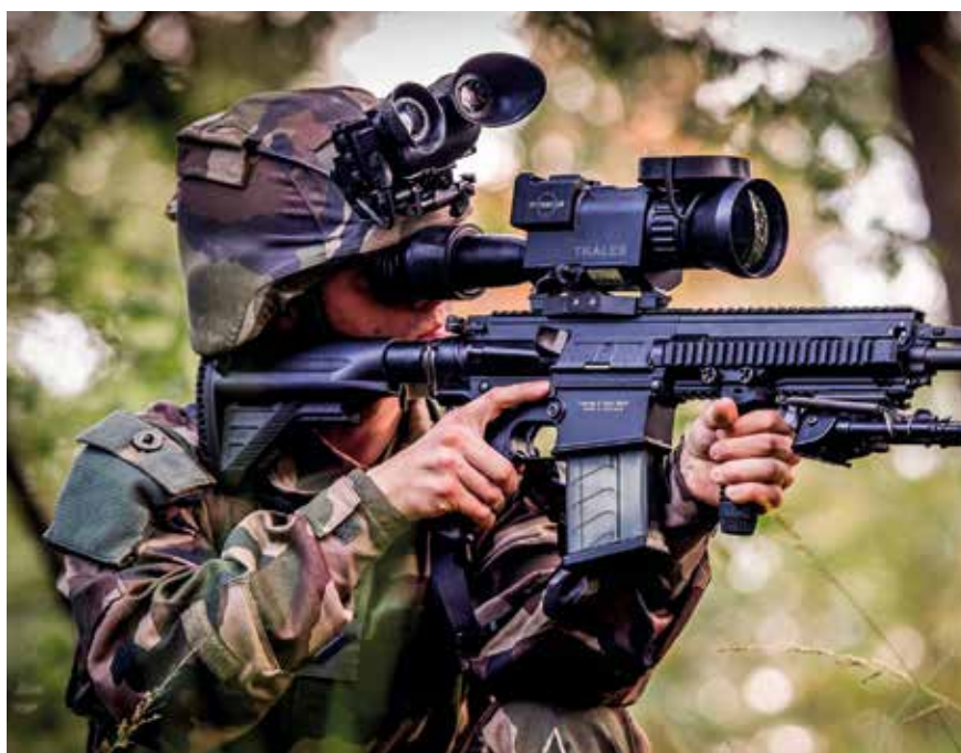
Thales BONIE NVG also incorporates an integrated IR illuminator for use in zero light conditions.
