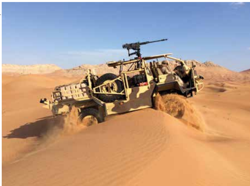
In 2017 SupaCat introduced a new variant of the HMT, the HMT 400 DESERT. "HMT 400 DESERT has been adapted to enhance performance in the desert's harsh environment and climatic conditions. It has no armour and the lighter gross vehicle mass improves the power-to-weight ratio and increases mobility over deep desert sand. Further desert features include cooling, a central tyre inflation system and lightweight bead locks to enable the vehicle to be operated at the lowest tyre pressures."
