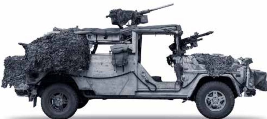
The SERVAL LIS (SO) with the top mounted 12.7mm machine gun and 7.62mm MGs mounted fore and aft
