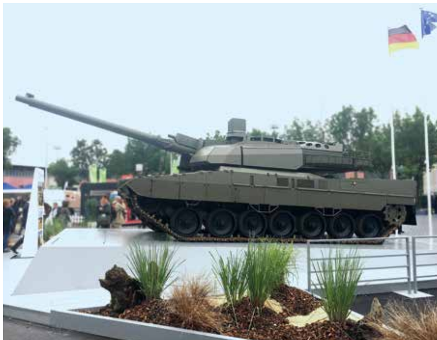
A first demonstrator of the EMBT at Eurosatory 2018. The hull of a LEOPARD 2 A7 was modified to host a LECLERC turret.
