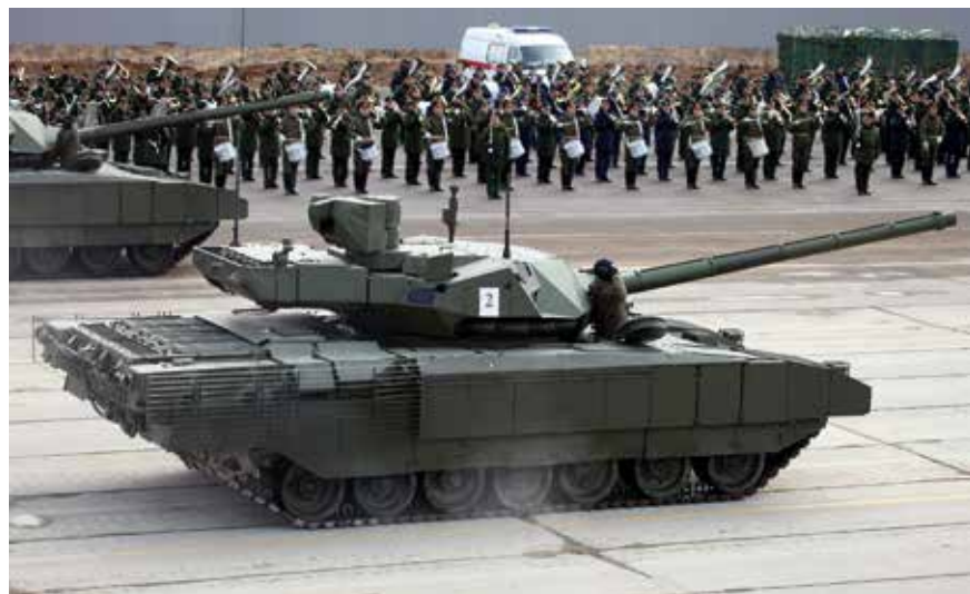
Russia's ARMATA T-14 MBT is equipped with MALACHIT explosive reactive armour and the AFGHANIT APS. Details of the MALACHIT ERA remain classified.
