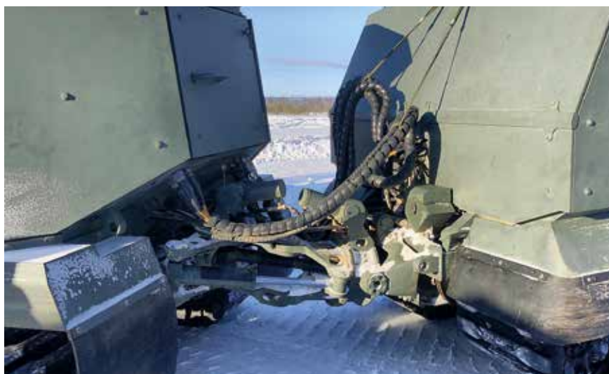
The articulated coupling is the one of the basic features of BRONCO 3
