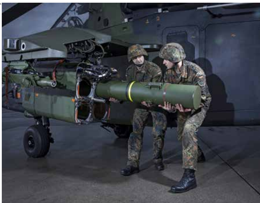
Ground crew loading a containerised PARS 3 LR missile into a launcher mounted under the stub wing of a Eurocopter TIGER
