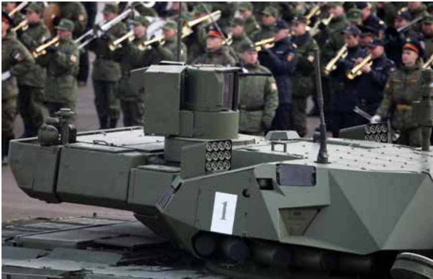
The sensors and countermeasure launchers of the AFGHANIT hard kill APS are positioned atop the turret of the T-14 MBT.
