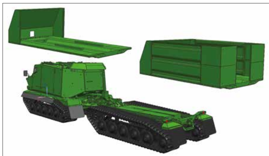
The BRONCO 3's modular design provides a high level of flexibility, facilitating quick and easy mission module switching.
