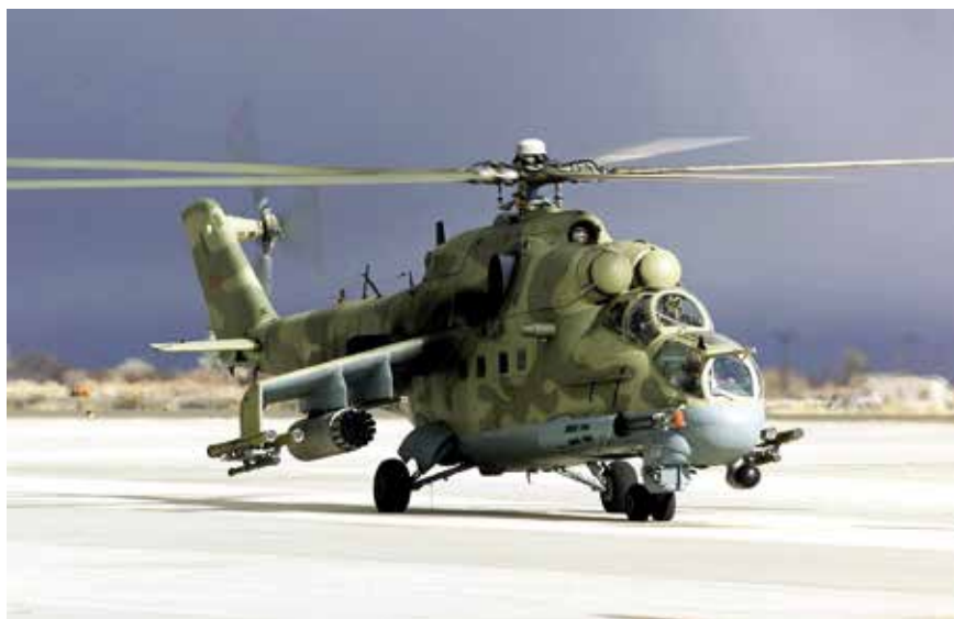
This Russian-made Mi-24 helicopter was used to provide simulated hostile threats during a US Joint Service Combat Search and Rescue (CSAR) exercise in February 2000. The aircraft has fuselage-mounted gun armament, and carries missiles and unguided rockets under its stub wings.
