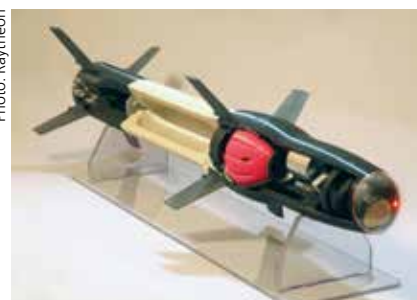
A cutaway model showing the printable components of a small missile.
