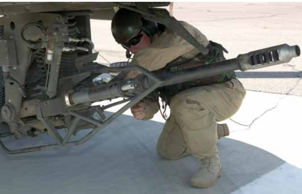
A British Army technician adjusts the 30mm Chain Gun of an AgustaWestland APACHE AH Mk 1 helicopter.
