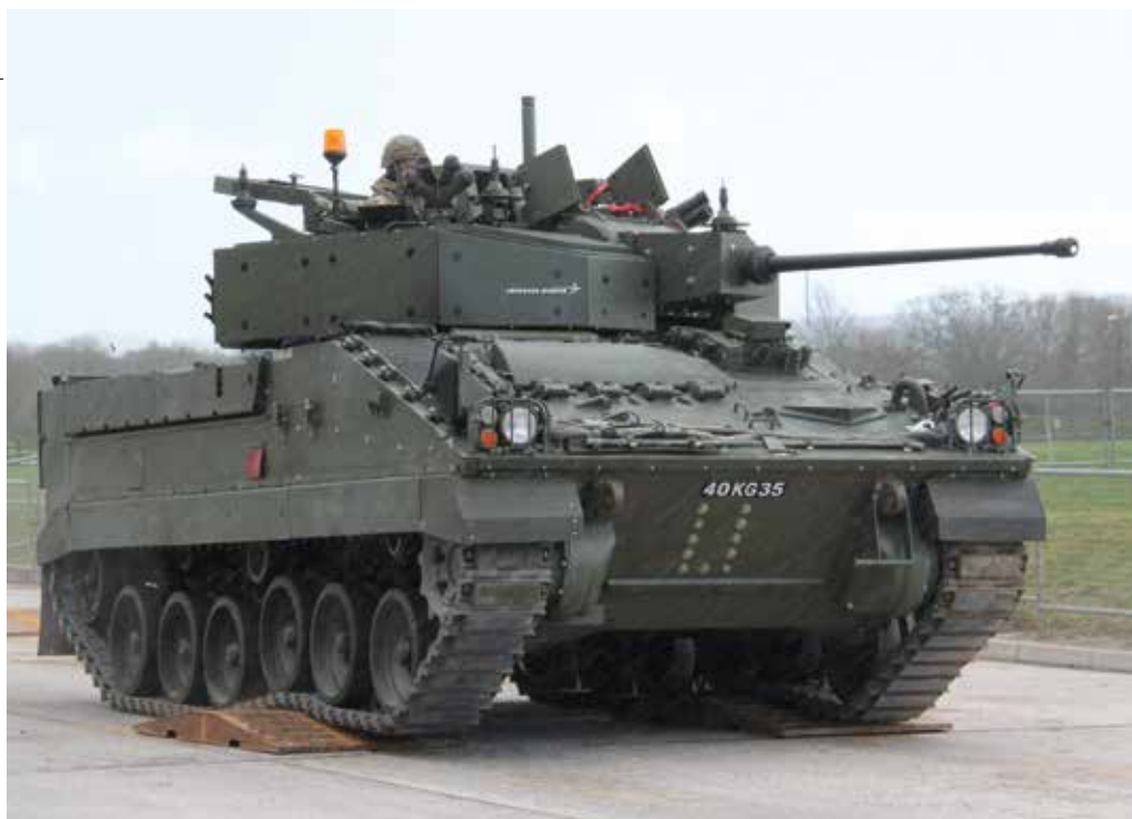
A WARRIOR AIFV upgraded to the WCSP standard
