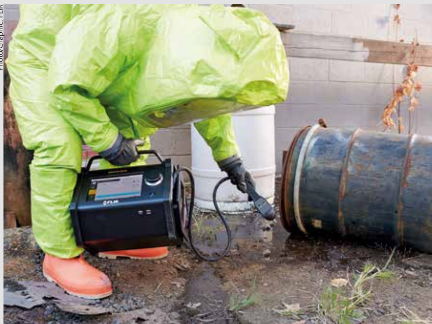
A detection specialist in PPE using the FLIR GRIFFIN G510 GC-MS
