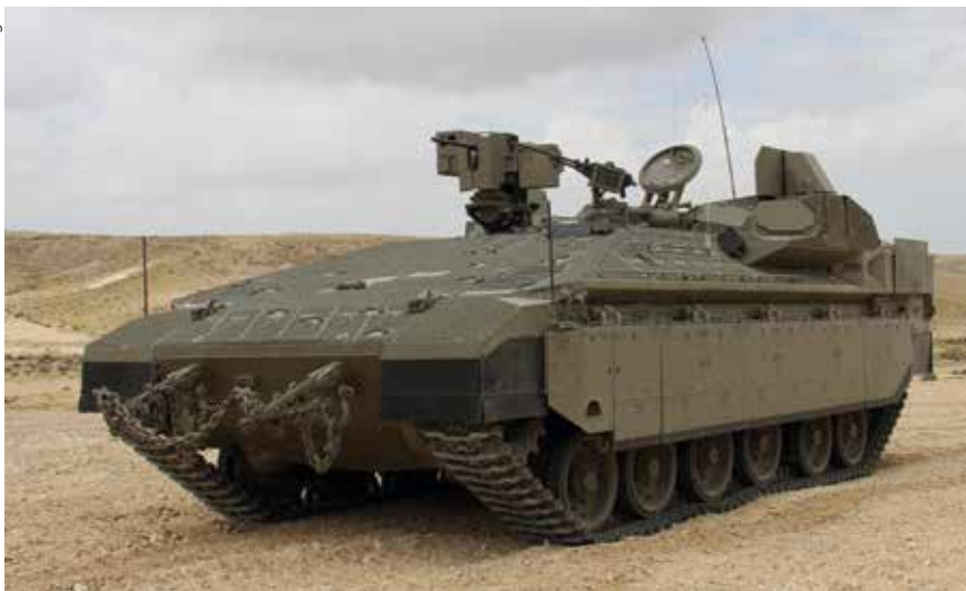
An IDF NAMER IFV. The hexagonal radar (one of four) and trapezoidal countermeasure launcher (one of two) are mounted atop and to the rear of the vehicle.
