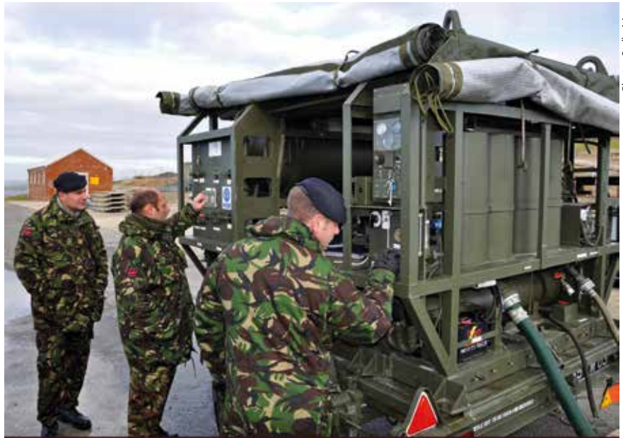
A Stella-Meta NBC FW water purification unit currently in service with the British Army
