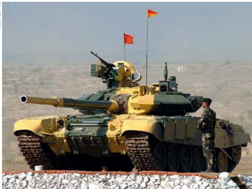
An Indian Army T-90 tank with Russian-made RELIKT-5 reactive armour.
