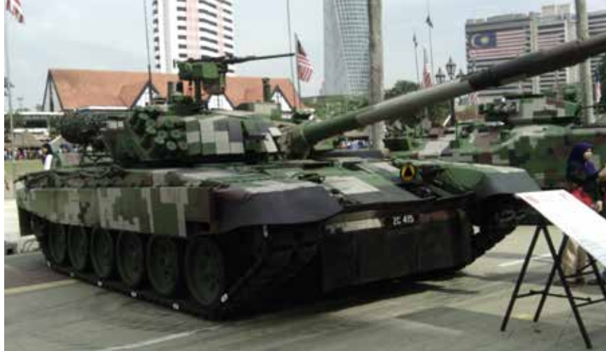
A Polish-built Malaysian Army PT-91M PENDEKAR MBT with Polish ERAWA 2 reactive armour.
