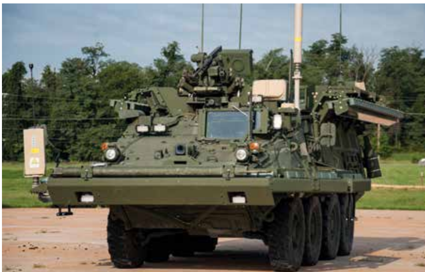
The IRON CURTAIN APS developed by US firm Artis LLC destroys incoming projectiles only centimetres before impact on the protected vehicle. It was under consideration for the STRYKER IFV, but in 2018 the US Army found that, while generally effective, the IRON CURTAIN did not perform sufficiently well under adverse weather conditions.
