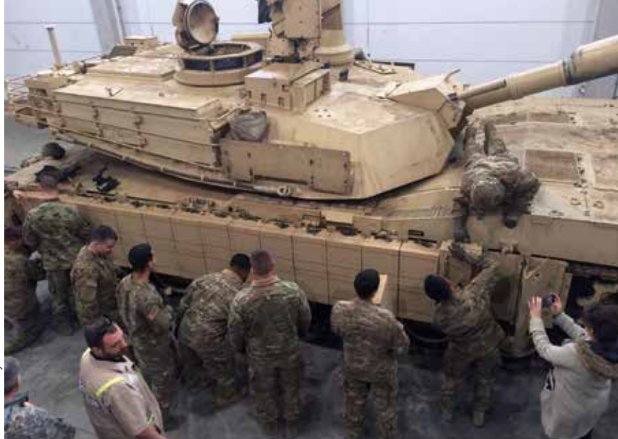
US Army soldiers apply the ABRAMS Reactive Armour Tile 1 M19 to an ABRAMS MBT in Germany.
