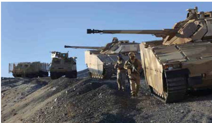
SAAB's Land Electronic Defence System 50 soft-kill electronic countermeasure system is deployed on the Swedish army's CV90 combat vehicles.
