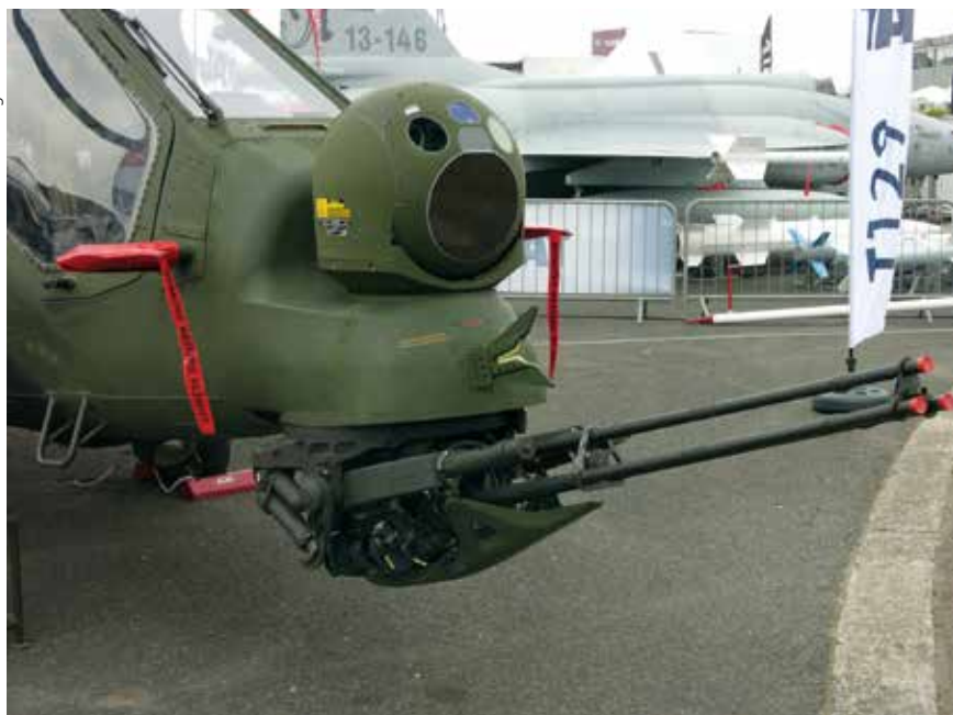
This view of the nose section of a TAI/AgustaWestland T129 ATAK helicopter shows the aircraft's electro-optical turret and M197 three-barrel rotary cannon.
