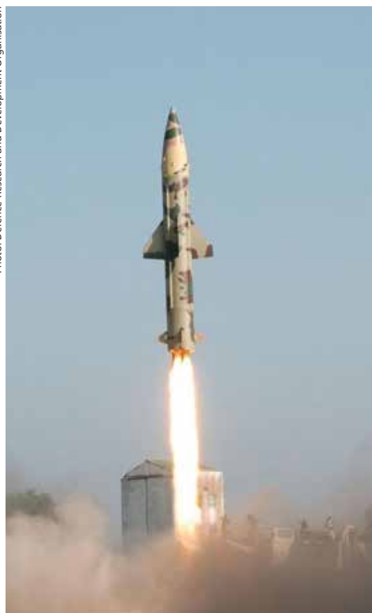
India's PRITHVI II ballistic missile is powered by two side-by-side gimbaled liquid-propellant motors that are based on the 720 rocket motor used in the Russian S-75 (SA-2 'GUIDELINE') surface-to-air missile.
