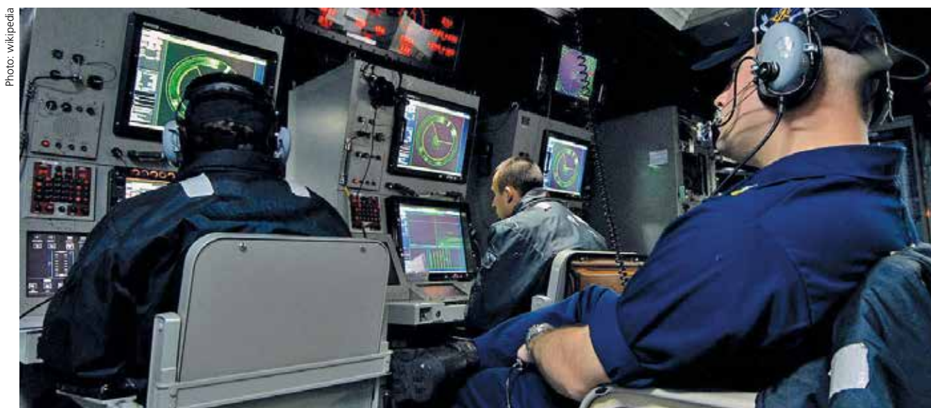
Lockheed Martin's AN/SQQ-89V is the primary ASW system for the US Navy's surface combatants. Shown here are the consoles on board the ARLEIGH BURKE Class destroyer DDG 92 (USS MOMSEN).
