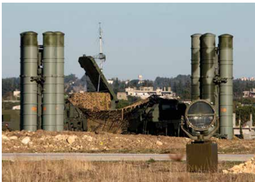
This 92N6 GRAVE STONE fire-control radar and vehicle-mounted vertical missile-launch tubes are part of the S-400 system that Russia deployed to Syria in November of last year.
