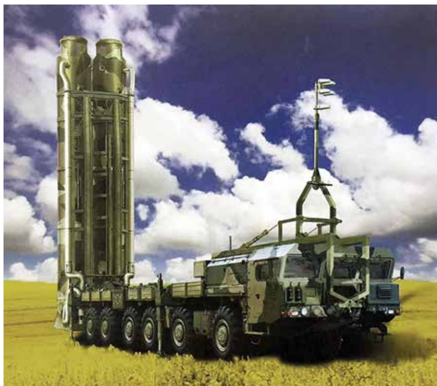
This artwork depicting a launcher for the Almaz-Antey S-500 system shows ducts leading to the top end of the launch tubes. These may be part of a cooling system for the missile's terminal homing seeker.
