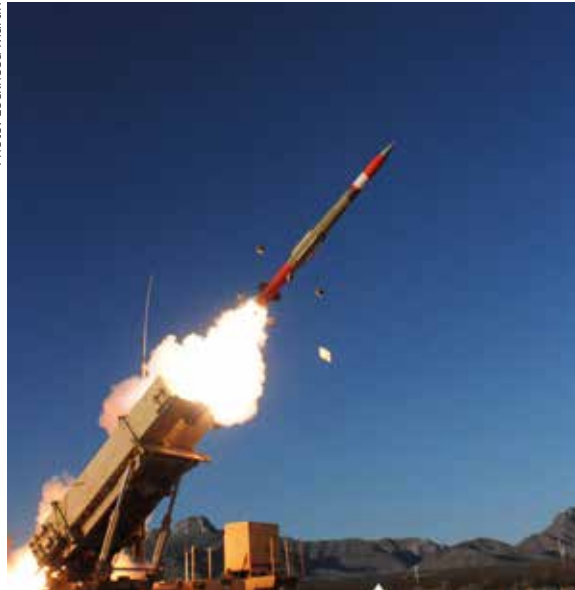
The PATRIOT PAC-3 MSE (Missile Segment Enhancement) incorporates a more powerful rocket motor that provides increased range and greater agility.
