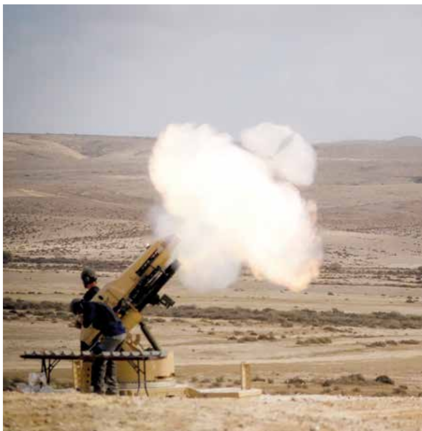
The CARDOM 10 is an upgraded version of the Israeli CARDOM 120 mm mortar which is in use with US STRYKER brigades and the IDF. It is fully automated, supported by a semi-automatic loading system, and has a longer barrel to improve range. It will be integrated with the Danish Army's new PIRANHA APC.
