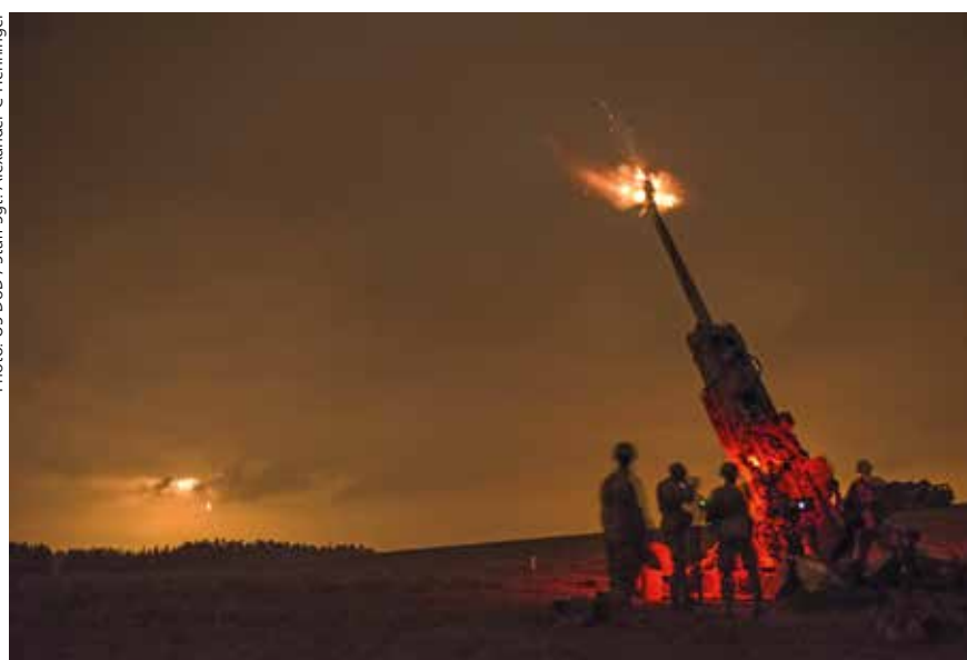
The range of the towed 155mm M777 has been doubled using an XM1113 rocket-assisted projectile (RAP).
