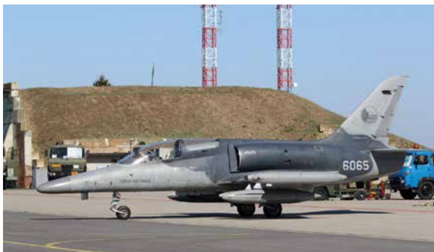
After 18 years of service the L-159s require a much needed mid life update, which could see the avionics upgraded and a targeting pod fitted. The latter is the Jet's biggest need if it is to work seamlessly in the air to land integration role.
