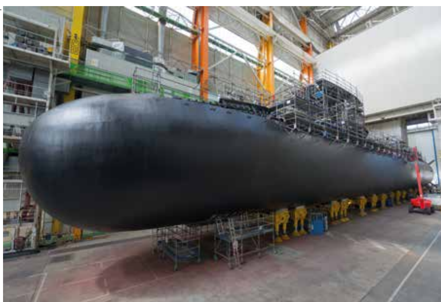
To be delivered in 2020, the SUFFREN SSN will be the first SYCOBS-equipped platform with Safran non-penetrating masts allowing to optimise the location of the control room.
