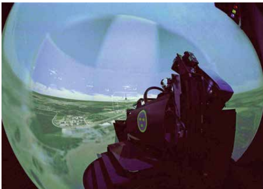
Dome screens such as this one of the Saab Full Mission GRIPEN fighter simulator have now become standard.
