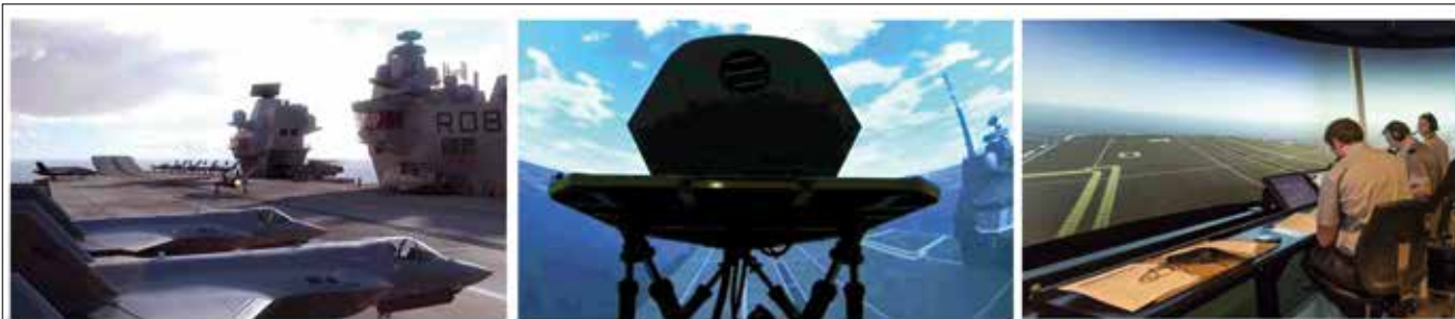
F-35B Simulators at BAE's base at Warton, UK – motion-based aircraft sim and sim of Ships's FlyCo
