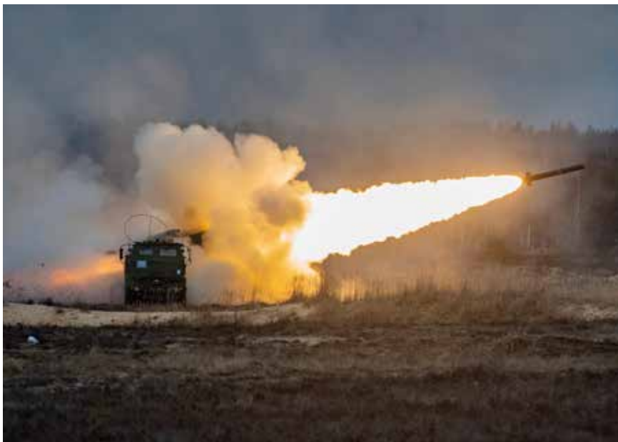
The M142 High Mobility Artillery Rocket System (HIMARS) is a light multiple rocket launcher developed in the late 1990s for the US Army, mounted on a standard Army M1140 truck.
