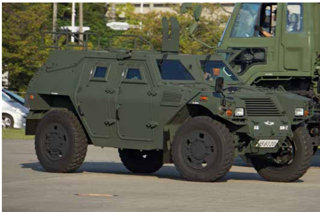
A Komatsu LAV. The roof-top shield has a provision for a machine gun.
