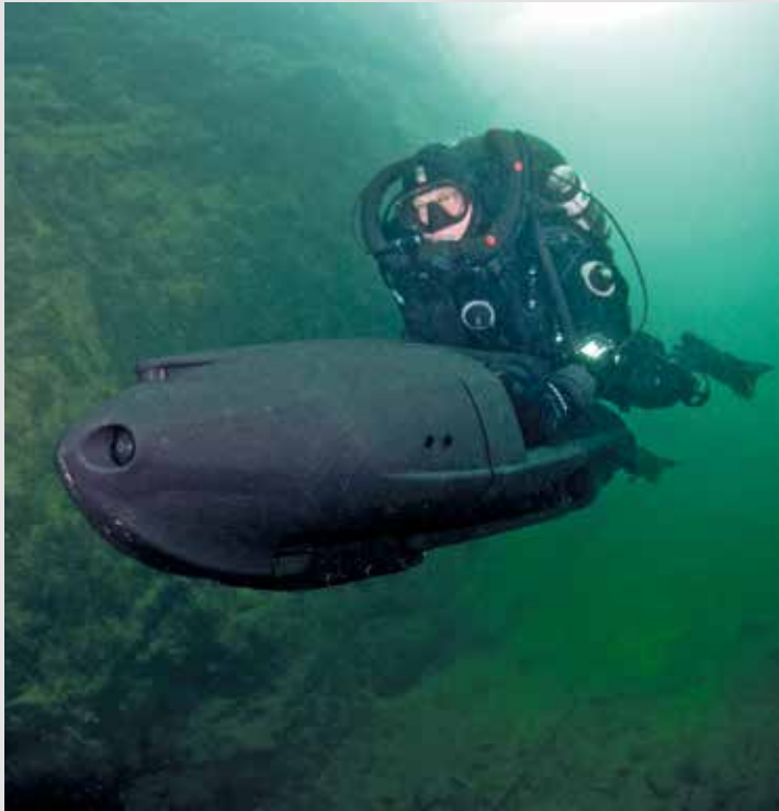
DPD/V's like the RasRotinorJILL8055 can also be used as combat load carriers to include navigation systems, sonar systems and weapons carriage.
