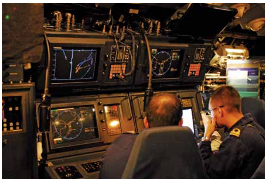
The U212A first batch's control room equipped with Kongsberg's MSI90U combat management system.
