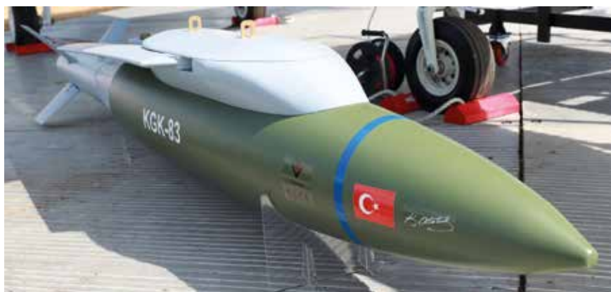
The K GK-83 folding wing-set kit to extend the range of the F-16
