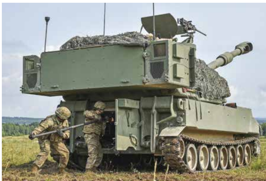
The US Army PALADIN SP gun will receive the new M109A7 chassis and an upgraded turret with an increased bore length of 29 feet instead of 20 to be able to fire extended-range ammo.
