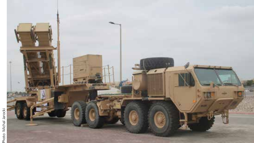
Under the WISLA programme, Poland will acquire eight PATRIOT medium-range range air and missile defence system batteries, each consisting of two firing units. Four launchers and one radar station will be provided per unit, as well as other components.
