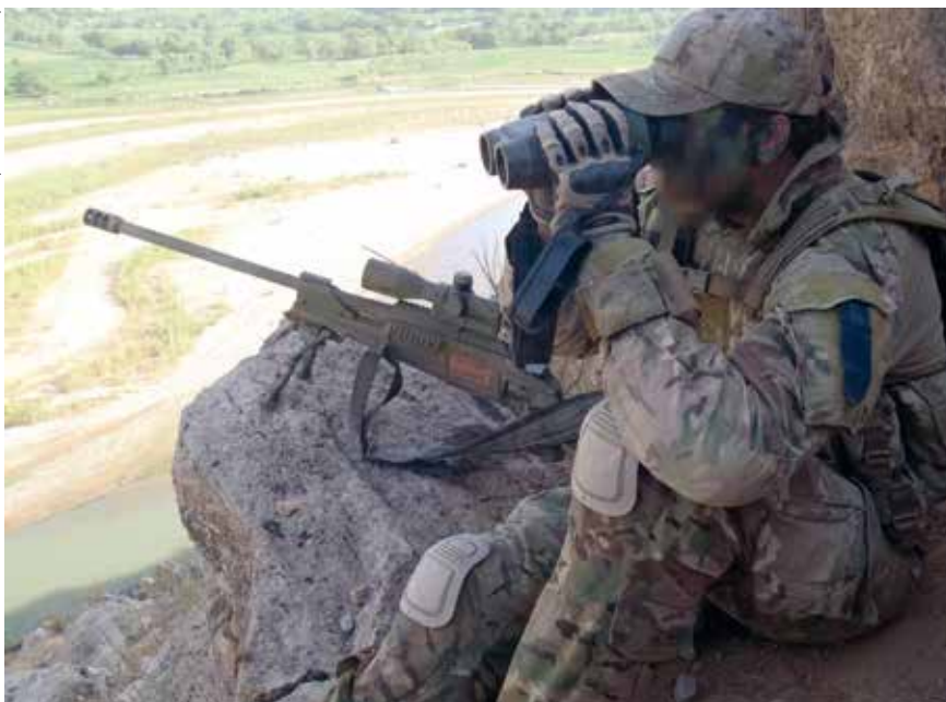
Australian sniper with a .338 Lapua Magnum Blaser TACTICAL 2, Schmidt & Bender riflescope and Vectronix VECTOR binocular laser rangefinder. Magazine capacity: 4 rounds; barrel length: 627 mm; overall length: 1,230 mm; weight: 9.140 kg (operational); effective range: 1,500 metres.
