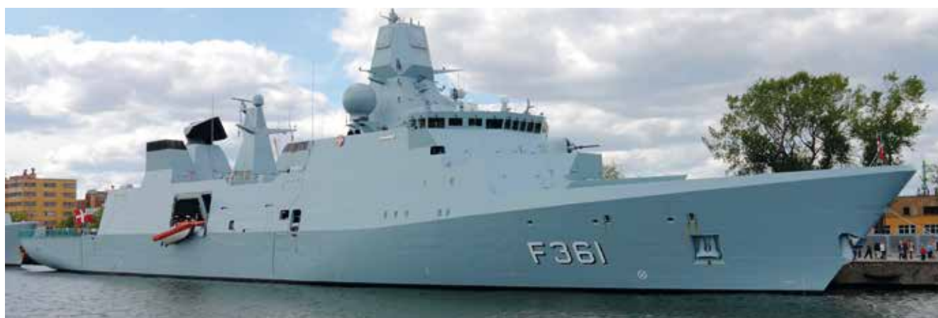
The three frigates of the IVER HUITFELDT Class entered service in 2012 and 2013. Current plans are for an upgrade of their SMART-L long-range surveillance radars in support of an intended ballistic missile defence capability.
