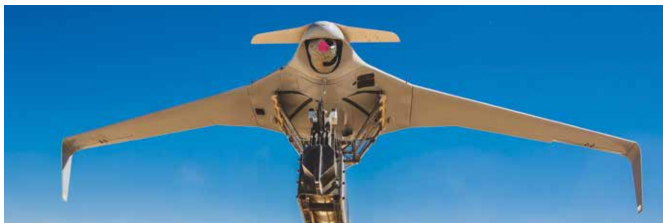
The ORBITER 4 can fly 24 hour missions at up to 150km range and beyond.
