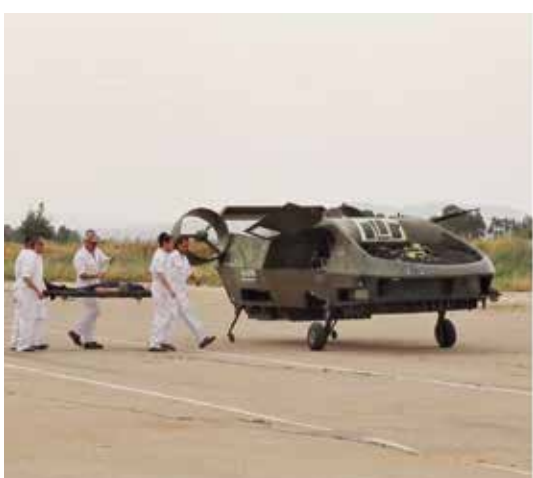
Tactical Robotics' CORMORANT is an unmanned VTOL aircraft which can be used for Casevac and for logistical support missions.
