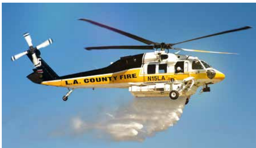
Lockheed Martin / Sikorsky offers a specialised fire-fighting variant of the S-70i called the FIREHAWK. It includes a 3,785-litre water tank and can be configured for casualty evacuation, SAR, or firefighter insertion.
