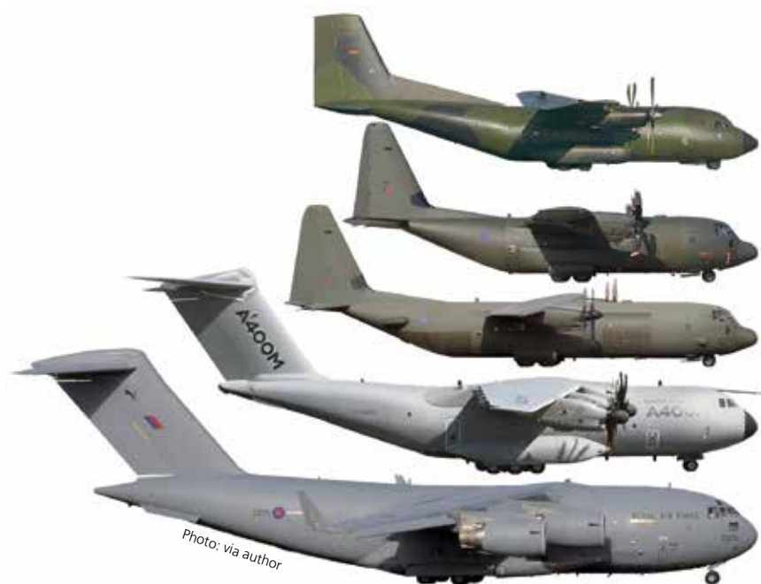
Size comparison of military transport aircraft. Top down: Transall C-160; Lockheed Martin C-130J SUPER HERCULES, C-130J-30 SUPER HERCULES (extended), Airbus A400M ATLAS, Boeing C-17 GLOBEMASTER III
