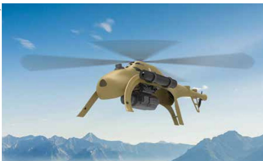
The Zhuhai Ziyang UAV Company BLOWFISH A2 UAS is designed for swarming applications. The system has a max take-off weight of 38 kg, a payload of 10 kg and endurance of 60 minutes. Up to 10 of these systems can be used in a swarming attack according to the company.
