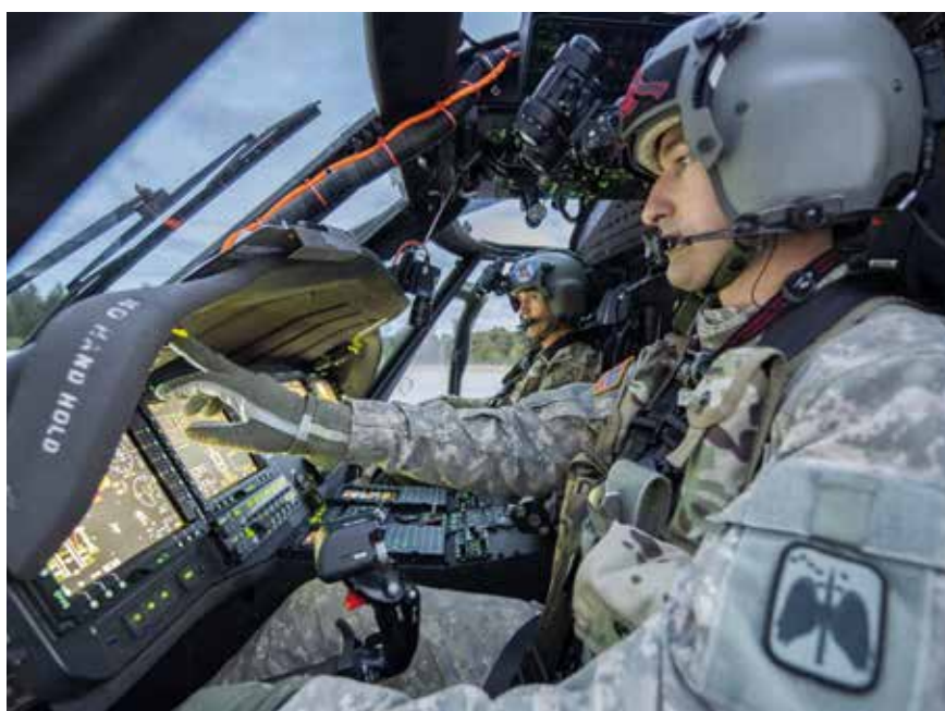
The UH-60V upgrade package outfits older model BLACK HAWK helicopters with a digital cockpit.
