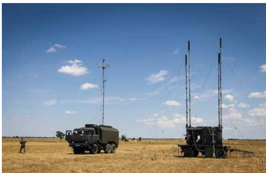
The deployment of military GNSS jammers like the Russian Army's R-330Zh Zhitel system to the Syrian theatre of operations has caused headaches for civilian satellite navigation system users in the Mediterranean.
