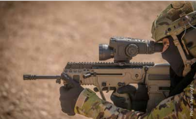
The Meprolight MEPRO NYX-200 is a multi-spectral weapon sight that can also be used as a hand-held device; it can provide an all-in-one solution to both day and night sight requirements. Meprolight unveiled many new sight developments at MILIPOL in November 2017.
