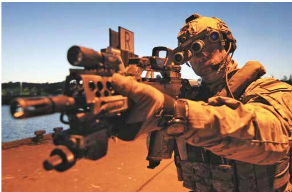
The Quad-Eye GPNVG (Ground Panorama Night Vision Goggle) from L3 in use with a German special forces operator.
