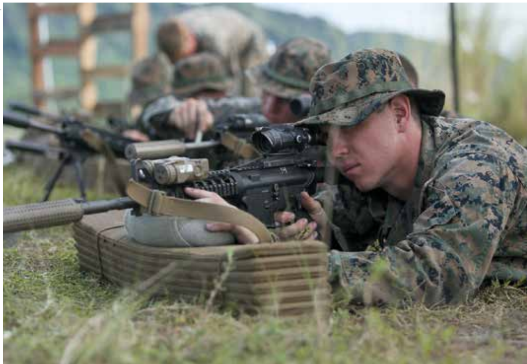
On the range in the Philippines, the Picatinny rail systems opens up a host of possibilities for attaching sights and other devices to a weapon, note the AN/PVQ-31 Rifle Combat Optic otherwise known as the ACOG and the AN/PEQ-5 carbine visible laser on this US Marine Corps M4A1 carbine.
