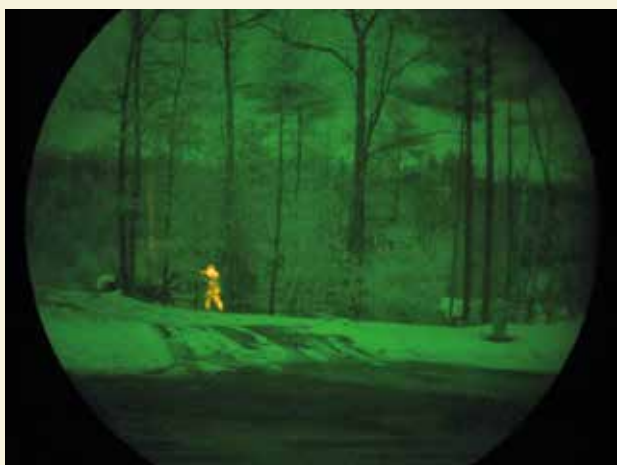
The internally fused image of an AN/PSQ-36 Fusion Goggle Enhanced (FGE) sets the human target clearly apart from the background.
