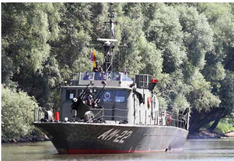
In Hungarian service NEŠTIN class minesweepers, originally from Yugoslavia, are designated MS-25: three - ÓBUDA (shown here), DUNAÚJVÁROS, and DUNAFÖLDVÁR - are operated by HDF 1st EOD & River Flotilla Battalion for river mine clearance.
