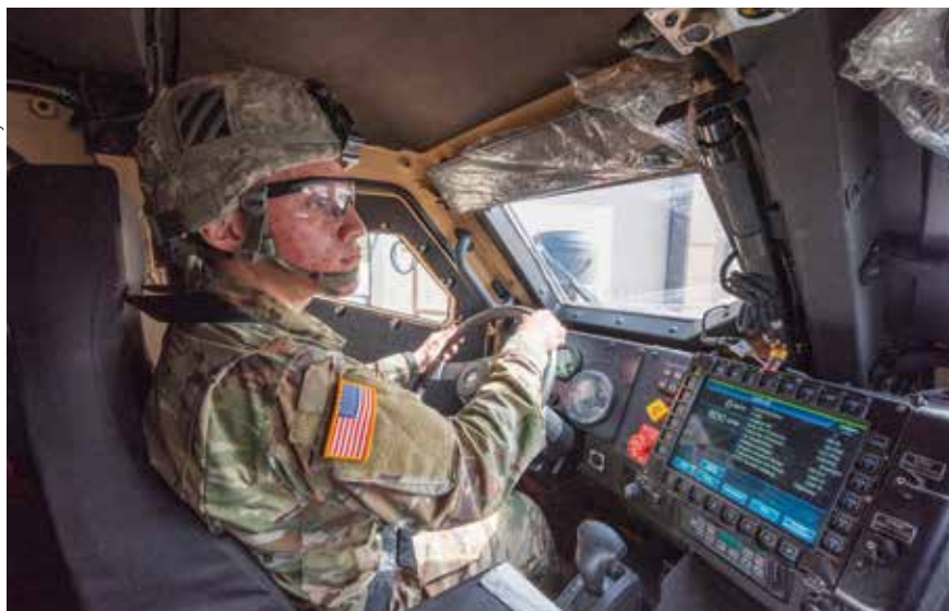
Similar to a touchscreen computer found in a newer car, the driver's smart display unit on the centre console monitors the Joint Light Tactical Vehicle's fluids, filters, tire air pressure and even has a rearview camera.
