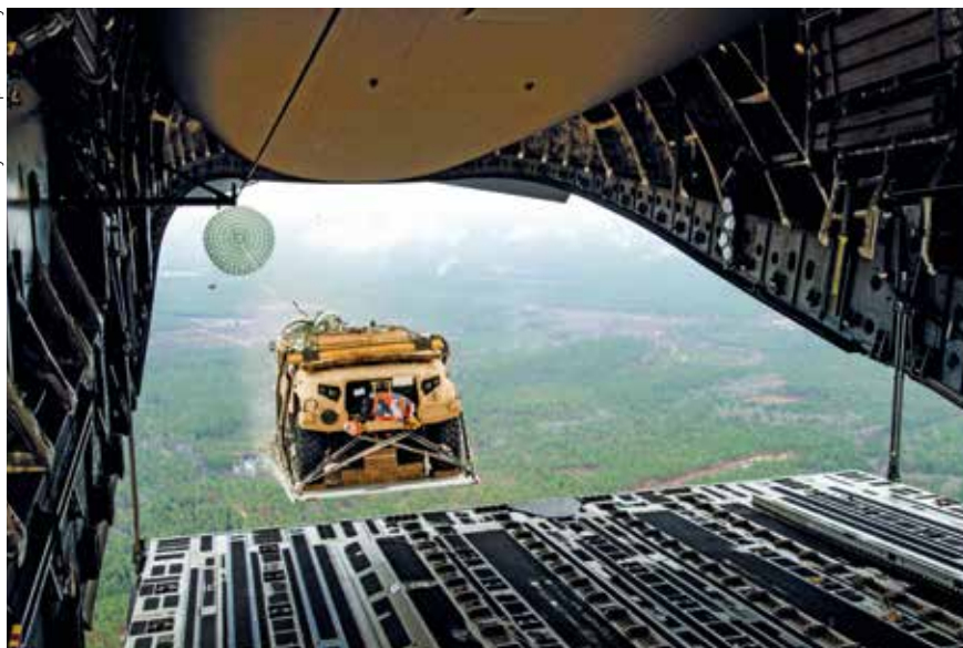
The Joint Light Tactical Vehicle (JLTV) Heavy Gun Carrier is extracted from a C-17 cargo aircraft as part of airdrop testing at Fort Bragg, N.C.
