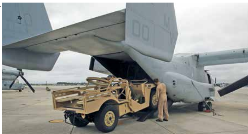
Members of the 22 nd Marine Operational Test and Evaluation Squadron carefully drive the new PHANTOM BADGER tactical vehicle into an MV-22 OSPREY tiltrotor aircraft during a fit test, 26 September 2014. It is six inches narrower than a Mini Cooper as it was designed to be loaded on an OSPREY.
