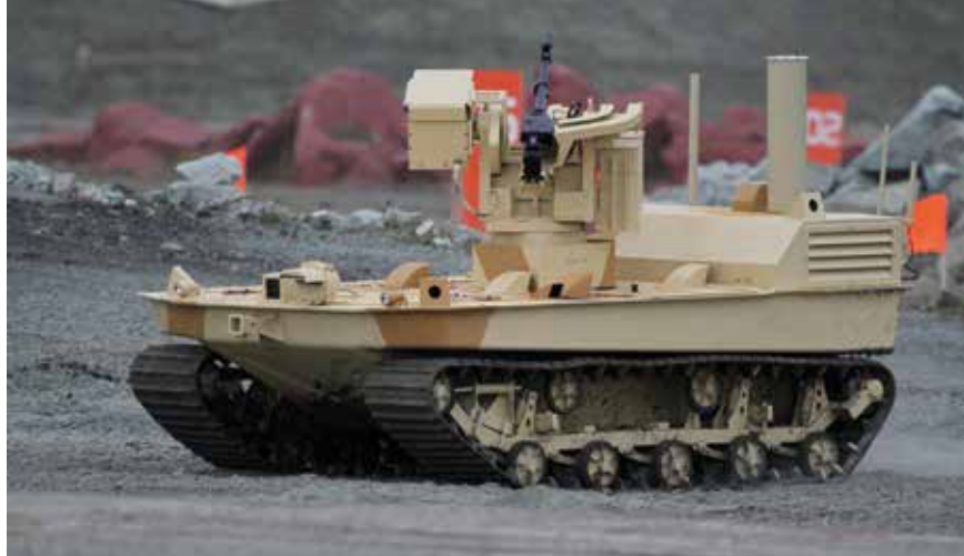
The R-002-BG-57 VOLK-2, equipped with a 7.62mm, or 12.7mm machine gun, or alternatively a 30mm grenade launcher
