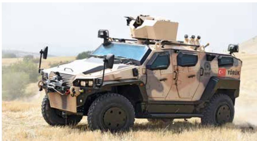
The light armoured vehicle NMS 4x4 weighs eight tonnes and is capable of carrying up to four tonnes.
