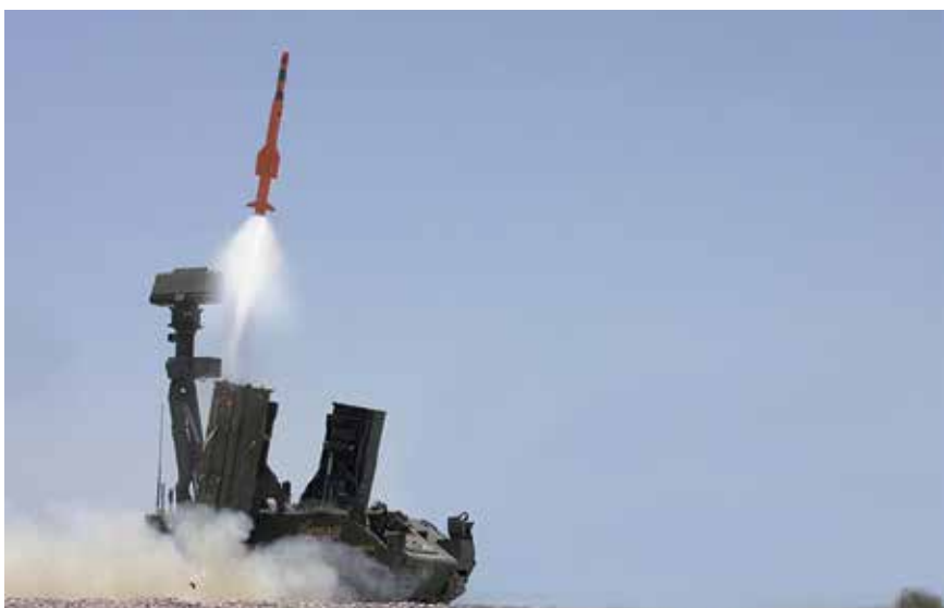
Aselsan's HISAR-A is another example of a missile that combines inertial and IR guidance. The same method is also being used in the heavier, and longer-ranged HISAR-O.
