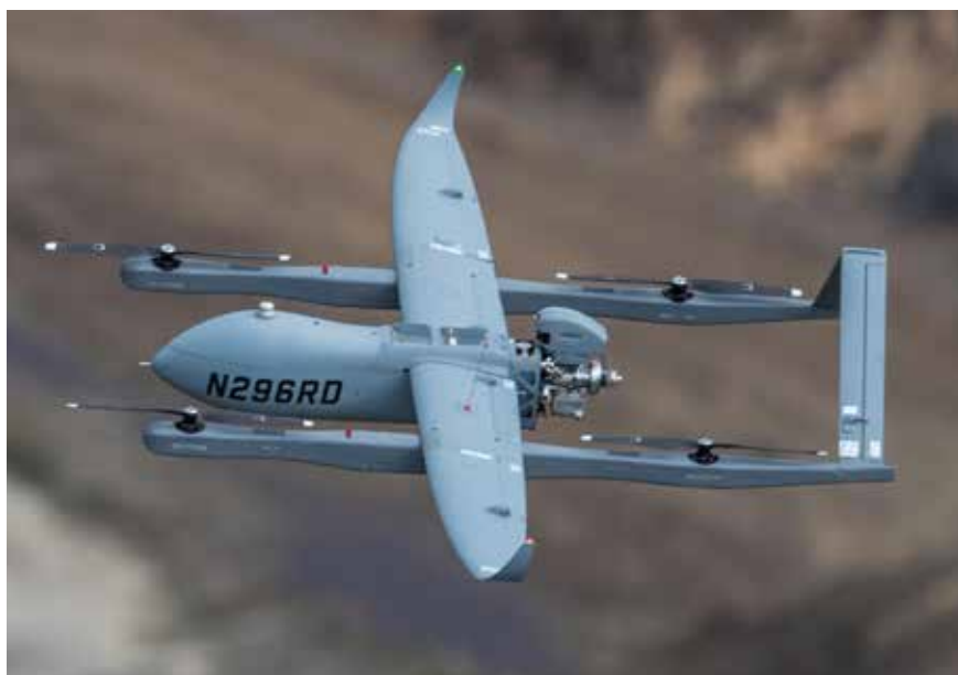
The AEROSONDE HQ is a fixed-wing VTOL.
