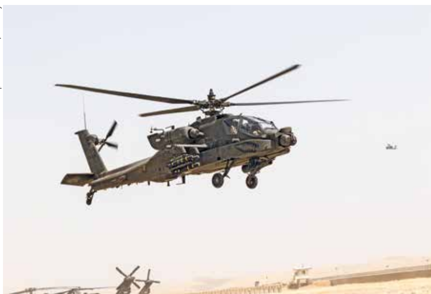
A US Army APACHE equipped with air-air and air-ground datalinks for advanced MUM-T applications
