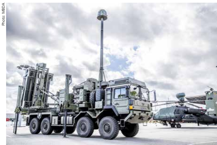
MBDA's LAND CEPTOR uses a missile that combines vertical launch with inertial mid-course guidance and an infrared seeker.
