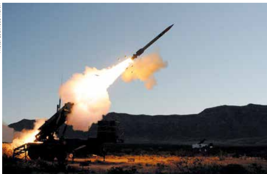
Lockheed Martin's PAC-3 missile was custom-designed for use against ballistic missile targets. It uses sideways-firing Attitude Control Motors mounted in the missile forebody.
