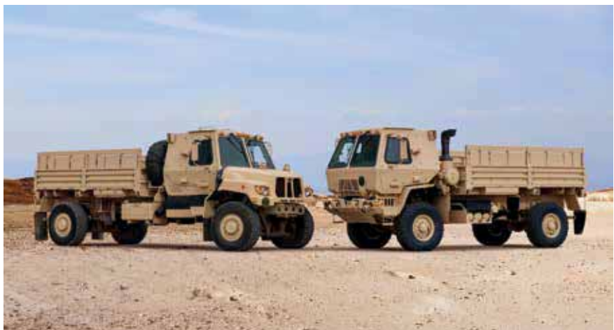
The next generation Oshkosh Family of Medium Tactical Vehicles will have six basic variants, the smallest being the 4x4 cargo truck.
