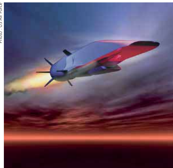
At least theoretically the X-51A WAVERIDER will be capable of surfing on its own shock waves.
