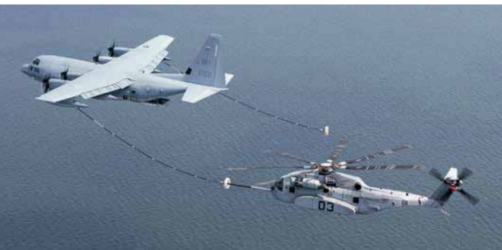
The CH-53K demonstrating air refuelling capabilities with a KC-130J tanker aircraft
