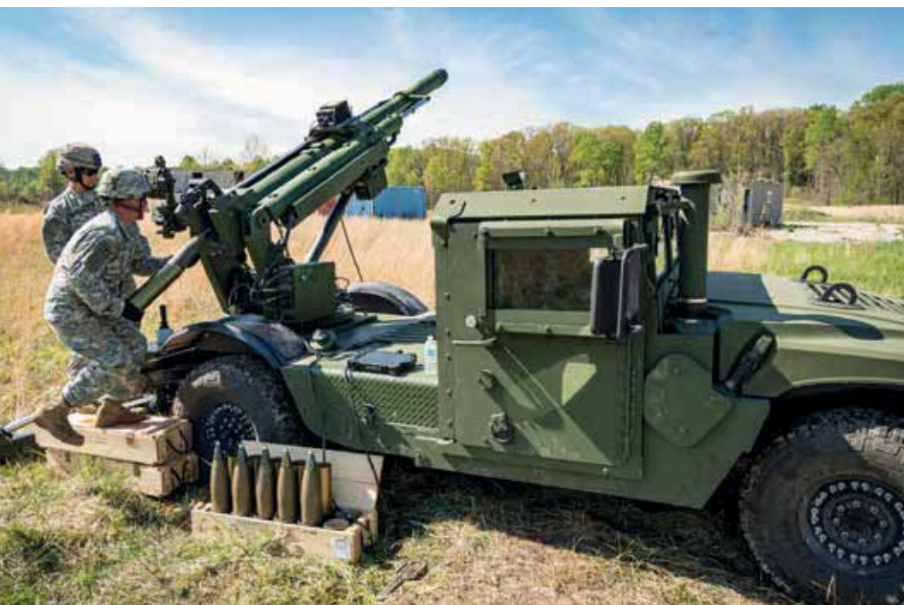
The HAWKEYE soft-recoil howitzer from AM General, here integrated on a HMMWV, is a modern interpretation of the classic lightweight, mobile artillery system.
