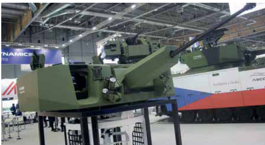
ASCOD 2 for the Czech Republic could be fitted with UT-30MK2 unmanned or MT30 manned turrets from Elbit Systems. GDELS assures, that the IFV will be compatible with any type of turret system selected by the future operator.
