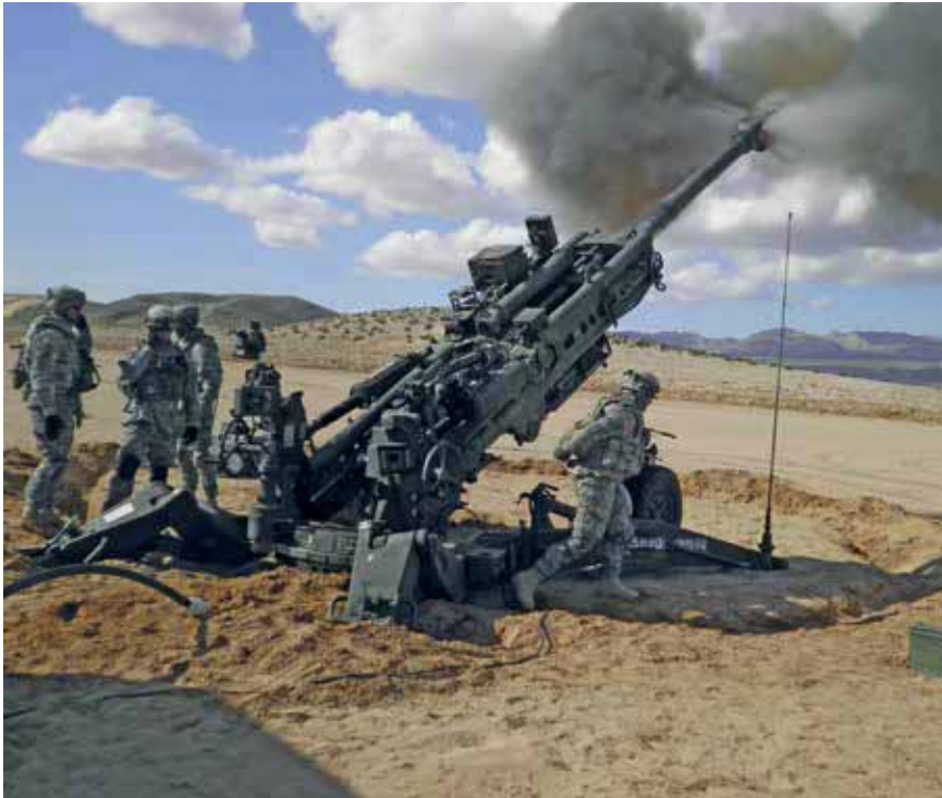
The US Army M777 155mm/39 calibre lightweight howitzer carrying out a fire mission
