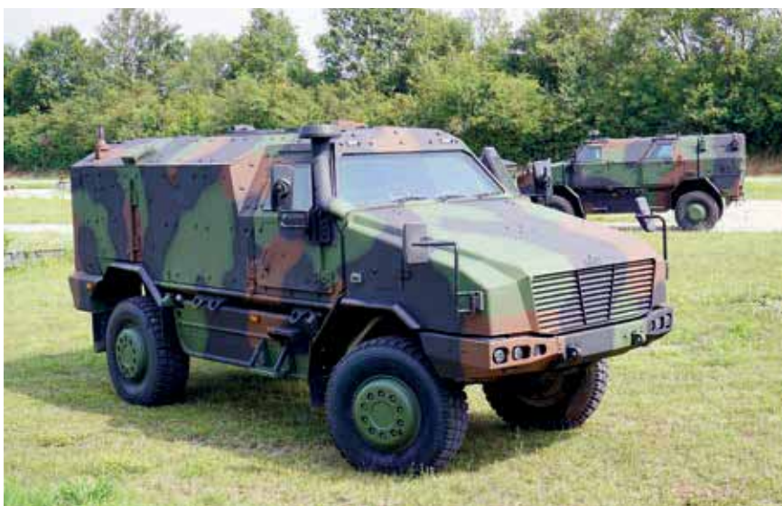
The 4x4 DINGO 3 is based on the Unimog FGA 14.5 chassis.
