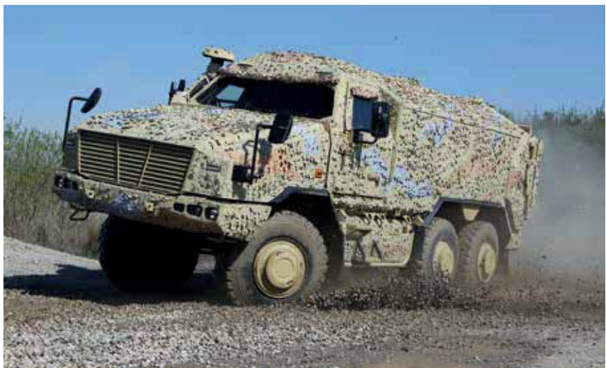
The 6x6 variant of the DINGO 3 is based on the Unimog FG20A chassis. Like the 4x4 variant, it displays excellent mobility across all terrain types.
