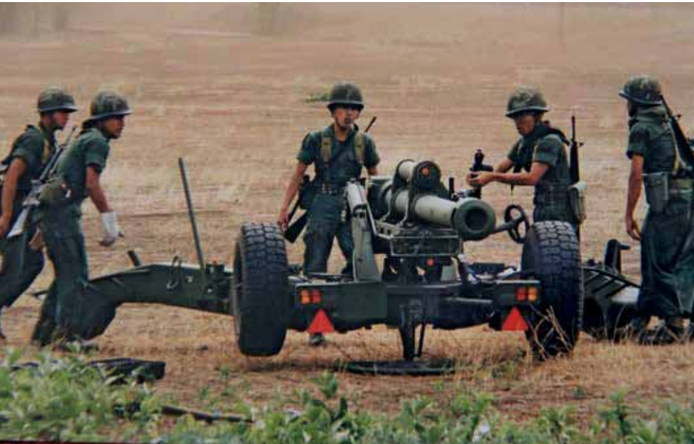
A Thai Army Nexter Systems 105mm LG1 Mk II Light Gun deployed in firing position and clearly showing turntable mounted under split trail carriage.
