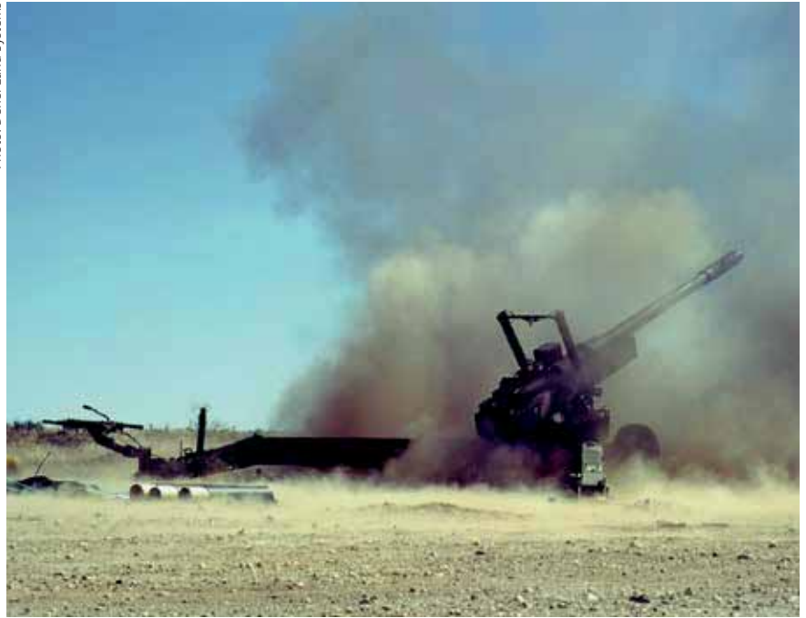
A first prototype of South African Denel Land Systems 105mm Light Experimental Ordnance (LEO) undergoing firing trials
