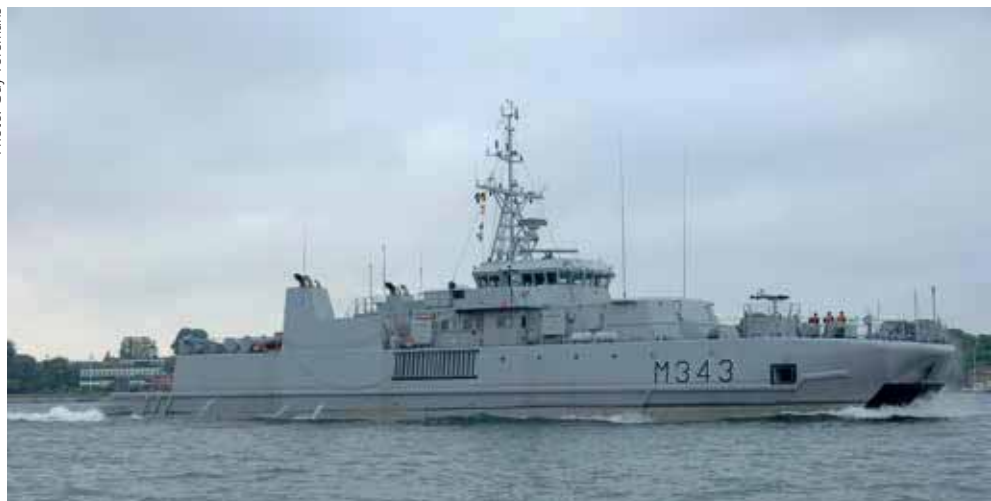
With a length of 55.2m, a width of 13.6m and a draft of only 0.84m the OKSØY/ALTA class MCMVs have a full load displacement of some 395 tons and a crew of 37 (13 officers).
