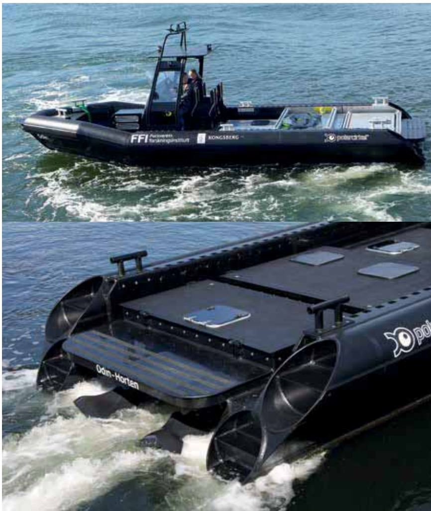
With a length of 10.5 m, a width of 3.5 m and a displacement of some 5.8 tons, Kongsberg's ODIN unmanned surface vehicle is able to embark an AUV such as the HUGIN 1000MR.
