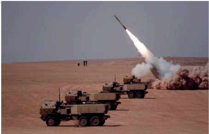
The XM1140A1 carrier vehicle supporting the HIMARS weapon system includes an armoured cab for increased crew protection.
