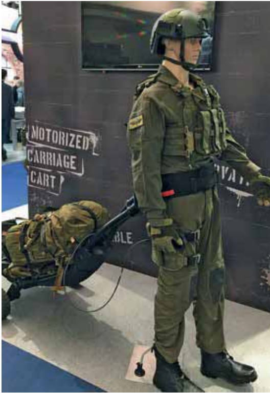
The tactical baggage car WILD GOOSE 4x4 by Marom Dolphin with a load capacity of up to 120 kg.
