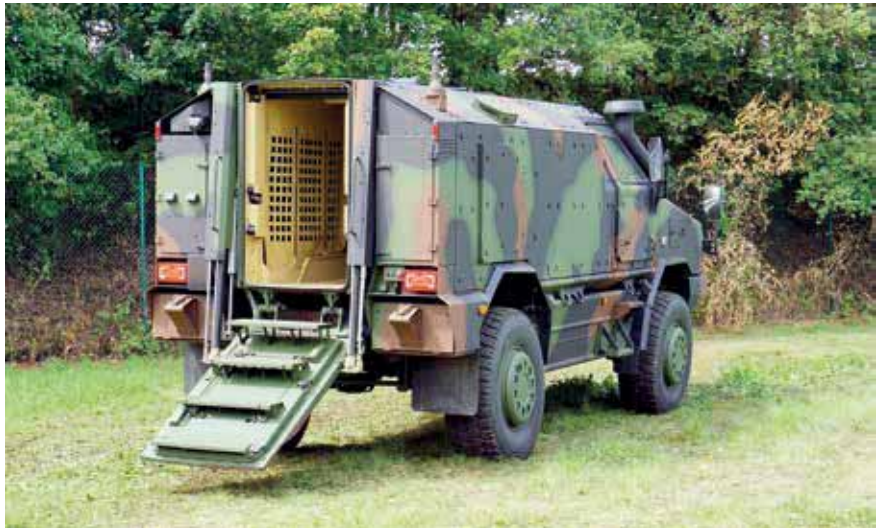
The rear ramp facilitates egress and ingress to the DINGO 3 troop carrier
