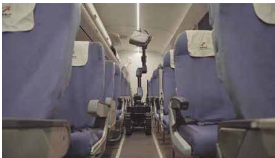
The aunav NEO EOD/IED/CBRN robot with a variable geometry system which allows its width to be increased or decreased automatically in a few seconds
