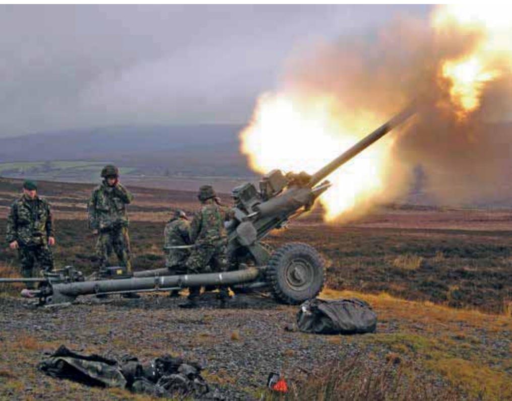
The Royal Artillery BAE Systems 105mm L118 Light Gun fitted with Leonardo LINAPS carrying out a fire mission
