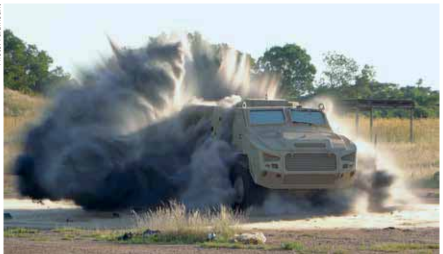
The MBOMBE 4x4 being tested for blast protection
