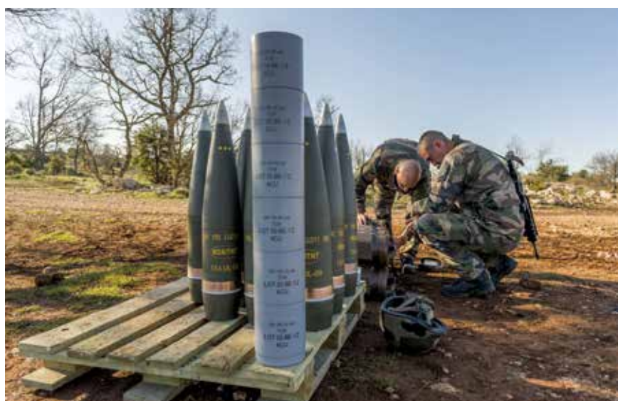
Eurenco's 'Charges Modulaires' TCM 155mm are bi-modular charges including single and multi-base propellants with combustible cases and are compatible with any 155mm gun (52, 45 or 39 calibre), including the K9 and CAESAR.
