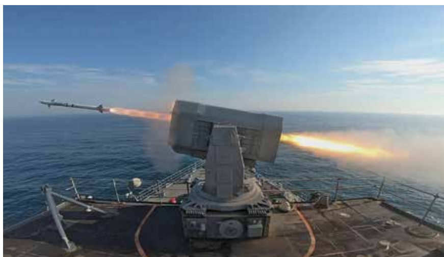
Raytheon's RIM-166 Rolling Airframe Missile weighs only 74 kg, but has a maximum range of around 10 km.
