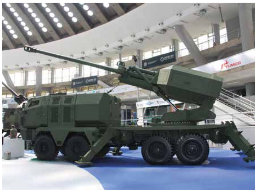
The latest Serbian Yugoimport ALEKSANDAR 155 mm/52 calibre MGS-25 SP artillery system with ordnance elevated and stabilisers deployed
