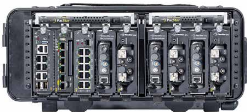
The PacStar Modular Radio Center (MRC) integrates SCI's TOCNET-G4 UVMS to bridge modern and legacy radio networks with industry-standard IP networks.
