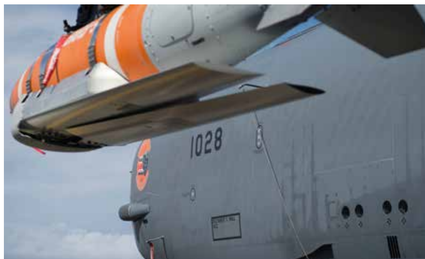
A QUICKSTRIKE-ER Mine in underwing carriage by a B-52 bomber. To prevent damage to the JDAM-Er tail assembly the mine is carried upside down. The folded wings of the JDAM-Er kit are clearly visible.
