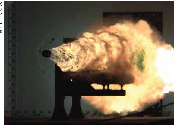
Photo: US Navy A 2008 test of the early 10 MJ railgun firing a 3.2 kg projectile with a muzzle velocity of 2520 meters per second, recorded by a high-speed camera
