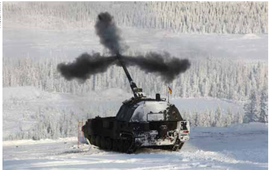
Krauss-Maffei Wegmann PzH 2000 155 mm/52 calibre is the only conventional tube artillery system deployed by the German Army and is now back in production for the third time.
