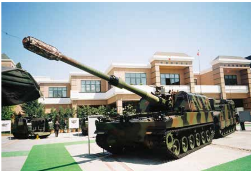
The Turkish FIRTINA 155 mm/52 calibre SP howitzer is based on the South Korean K9 THUNDER and shown here with ammunition resupply vehicle to rear.
