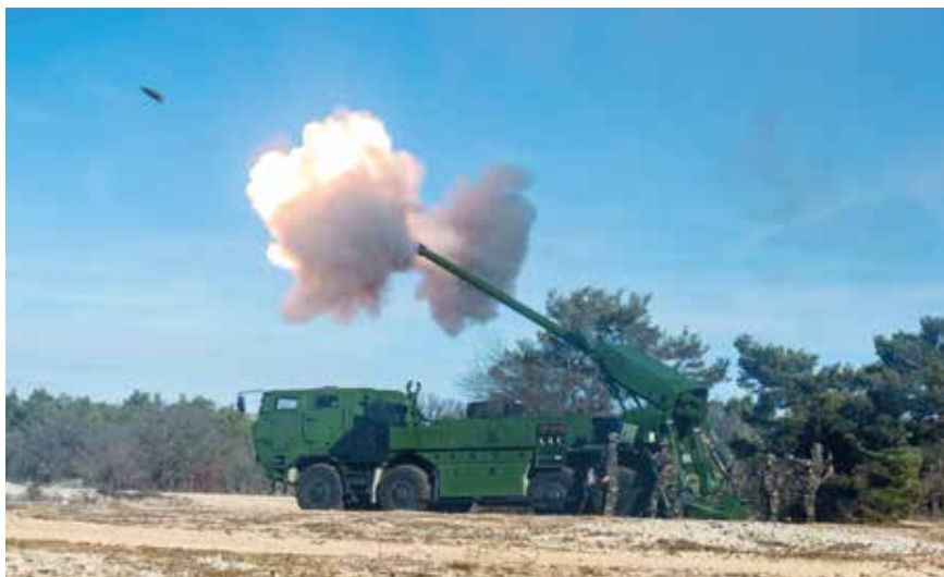
The French Nexter CAESAR (8x8) 155 mm/52 calibre artillery system is based on a Tatra 8x8 chassis with a protected forward control cab, with Denmark being the launch customer.
