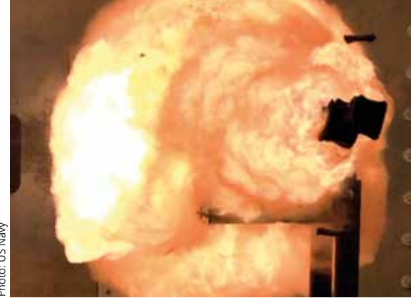
Photo: US Navy Test firing a 32 MJ railgun at NSWC Dahlgren
