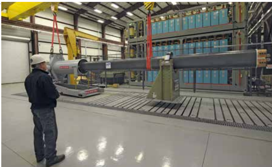
Installing BAE's 32 MJ railgun prototype at NSWC Dahlgren in 2012
