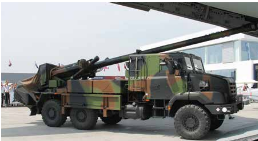
The French Army CAESAR 6x6 155 mm/52 calibre SP artillery system with protected cab can be loaded aboard A400M transport aircraft.
