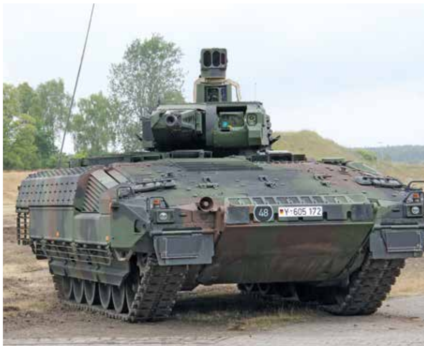
The German PSM PUMA Armoured Infantry Fighting Vehicle fitted with a remote controlled turret armed with a Mauser 30 mm MK 30-2 dual feed cannon capable of firing air burst ammunition and a 5.56 mm co-axial machine gun
