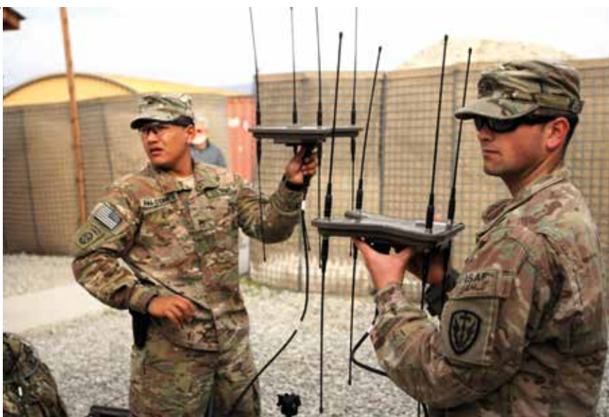
US soldiers demonstrate the hand-held antenna unit of the Praemittias Systems WOLFHOUD Cooperative Radio Direction Finding System.
