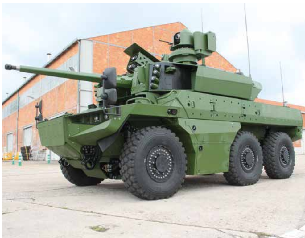
The French JAGUAR (6x6) reconnaissance vehicle is armed with a 40mm Case Telescoped Armament System (CTAS) and a roof-mounted 7.62mm remote controlled weapon system.
