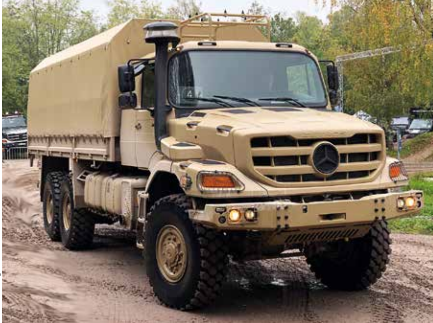
Introduced in 2019, the ZETROS NG is one of the military trucks from Mercedes-Benz along with the AROCS (not shown here). The cab-behind-engine vehicle was the first protected transport vehicle of the German Army.
