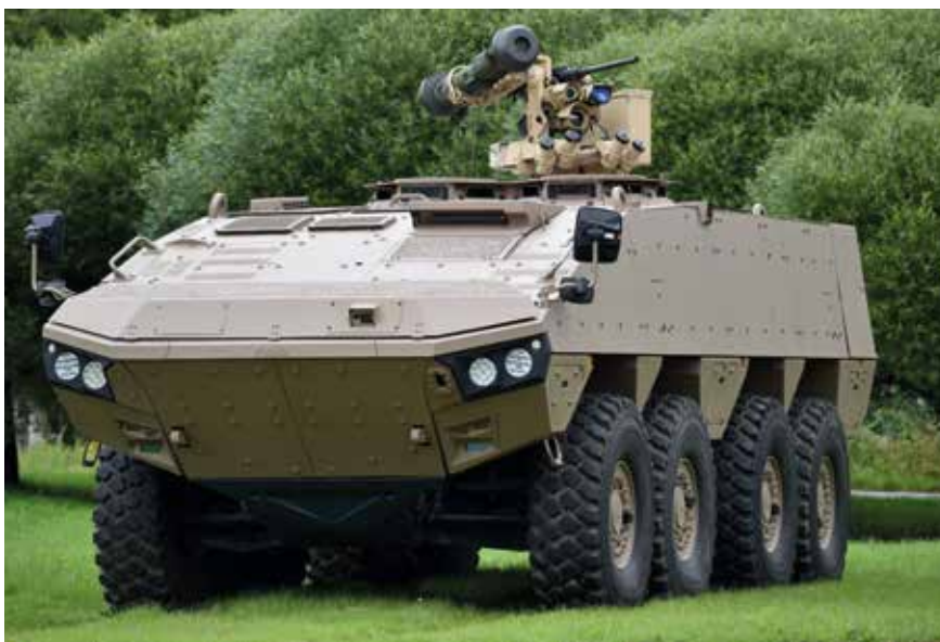
The latest PATRIA Armoured Modular Vehicle XP fitted with a Kongsberg remote weapon station armed with a 12.7mm MG and JAVELIN ATGW
