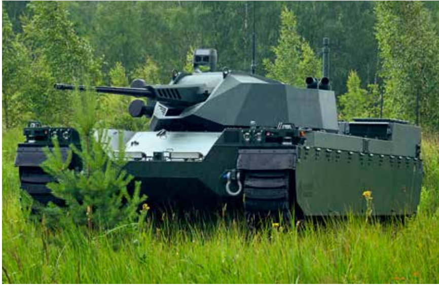
The CPWS Gen II turret on top of the MILREM Type X unmanned ground vehicle
