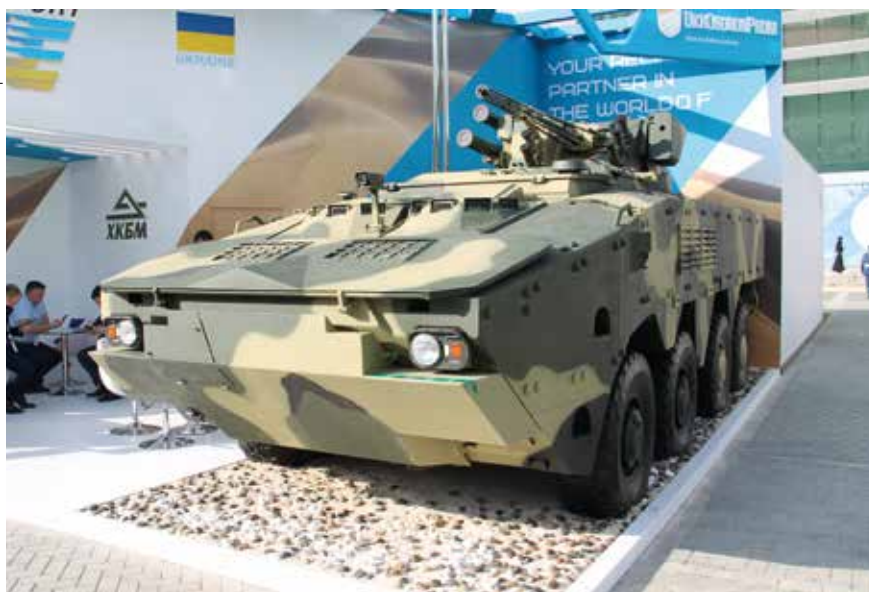
The latest BTR-4 (8x8) from the Ukraine fitted with a remote controlled turret armed with a 30mm cannon, a 7.62mm co-axial MG and two ATGW on the right side.
