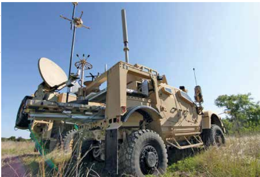
The US Army's PROPHET system – seen here in vehicle-mounted form – covers the HF, VHF and UHF bands.
