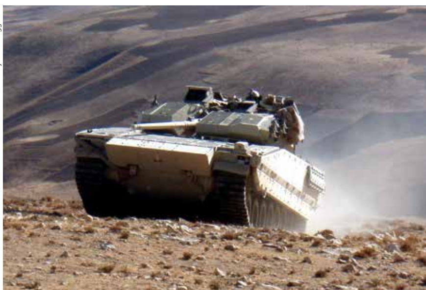
The Norwegian Army CV9030 IFV in Afghanistan armed with a Northrop Grumman 30mm dual feed cannon and 7.62mm co-axial MG. This CV9030 also has additional armour
