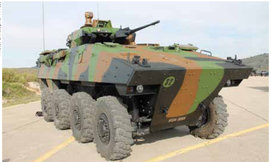
The French Army VBCI IFV fitted with a one-person turret armed with a M811 25mm dual feed cannon and 7.62mm co-axial MG
