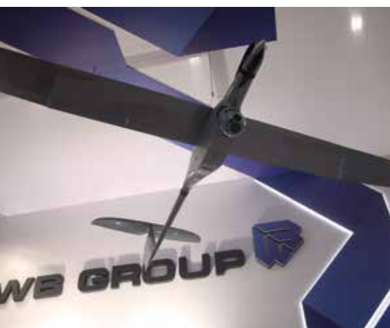
One of WB Group's flagship products is a mini class UAV FLYEYE, a modular system characterised by the ease of assembly and disassembly. Launch readiness can be achieved in less than 10 minutes.
