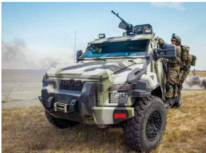
A Kraz SPARTAN armoured car of the Ukrainian National Guard, based on a Ford-F550 chassis
