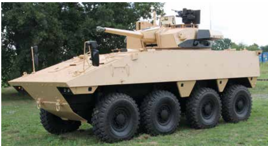
The Nexter VBCI (8x8) fitted with Nexter T-40 turret armed with 40mm CTAS and a roof mounted RWS armed with 7.62mm MG
