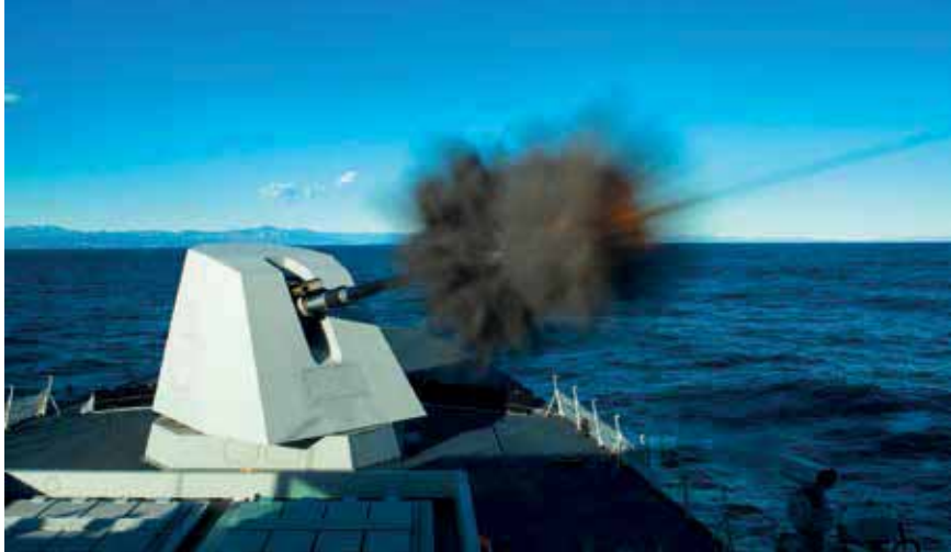
The Leonardo OTO 127/64 LightWeight (LW) VULCANO is the only 127mm gun mount developed and built in Europe and capable of automatically handling and firing the VULCANO family group of guided and unguided long-range ammunition.
