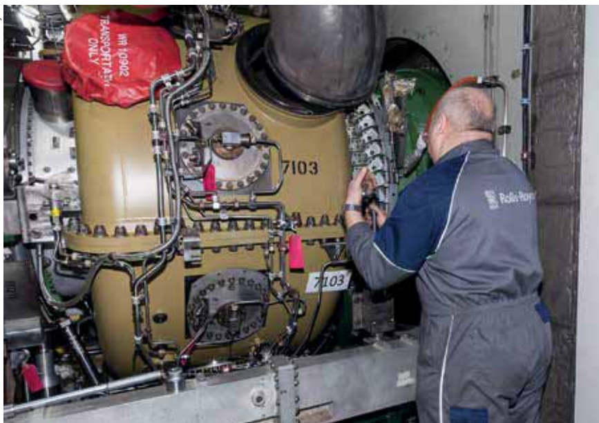
A WR-21 undergoes tests at a dedicated Rolls-Royce facility in Bristol, UK.
