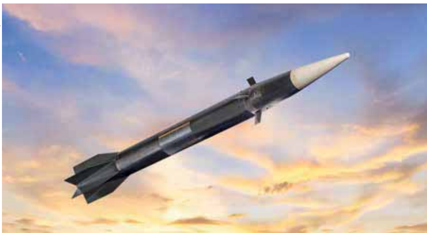
Leonardo's family of VULCANO ammunition includes both the unguided BER round with a 60 km range and the GLR IMU/GPS guided ammunition with up to 85 km range. The latter can be also equipped with a Diehl Defence IR terminal seeker to engage moving sea surface targets.
