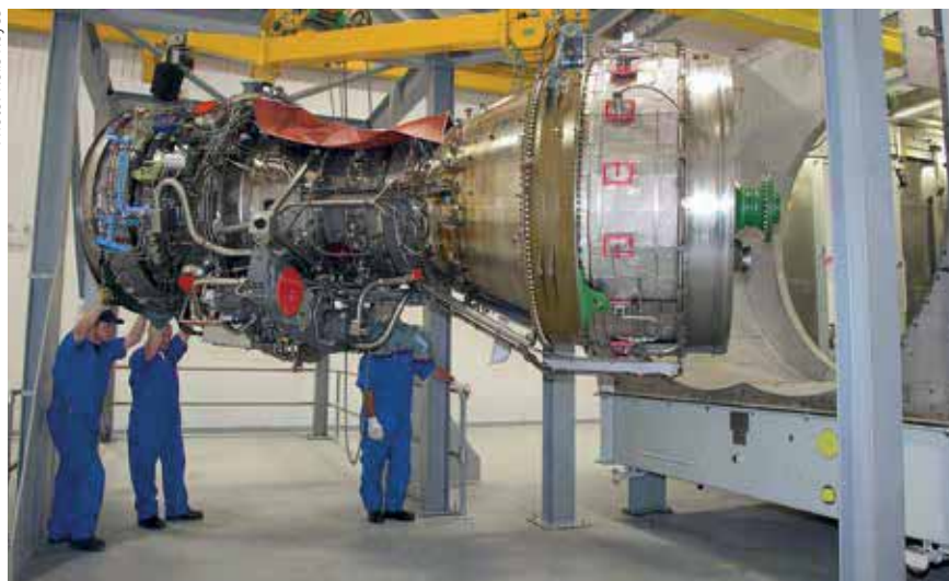
First run in 2002, the Rolls-Royce MT30 has a maximum power rating of 40 MW.
