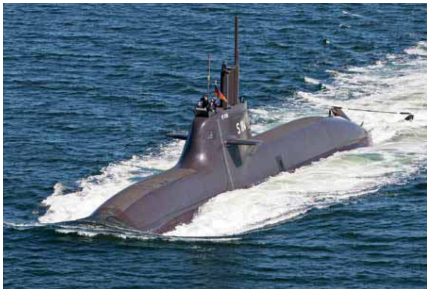
U-34 was the fourth Type 212A submarine to enter service with the German Navy. This class uses a fuel cell based AIP.
