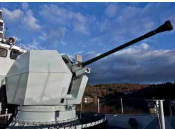
The latest iteration of Bofors 40 gun system family features a substantial reduction in volume, weight and price compared to earlier versions, in addition to providing full compatibility with the latest 'smart' 3P programmable ammunition.
