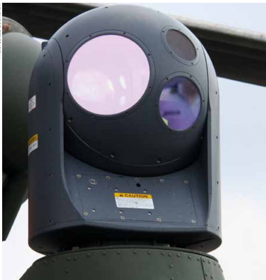
Rafael's TOPLITE EO turret can be fitted with up to four sensors.
