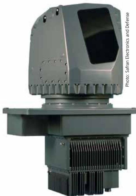
The VAMPIR NG infrared search and track (IRST) system onboard Australia's ANZAC class frigates
