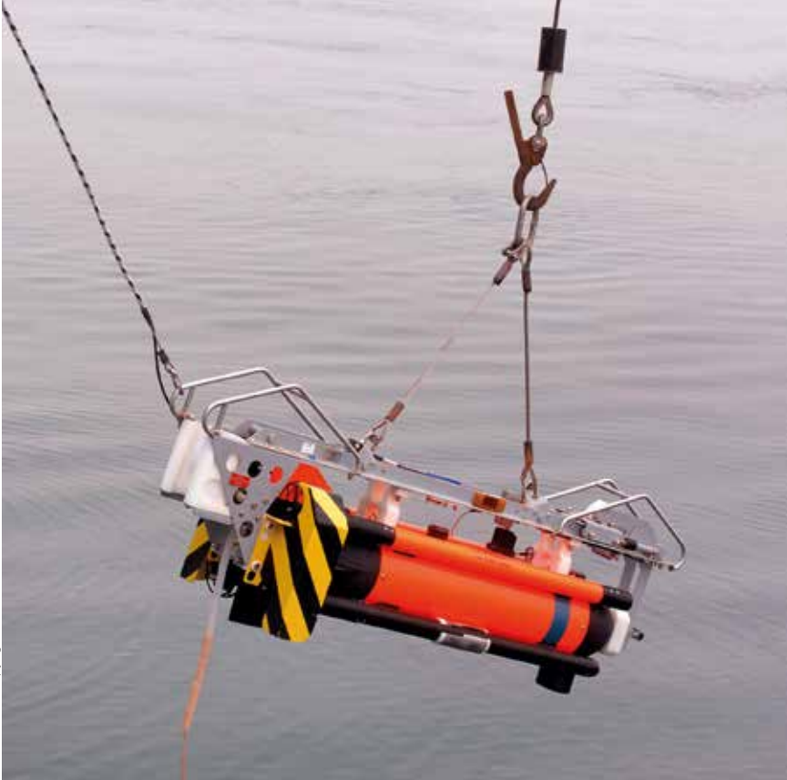
An Atlas Elektronik SeaFox ROV pictured in the course of deployment from a Royal Navy MCMV. Communication with the SeaFox's sensors is implemented by a thin fibre optic cable.
