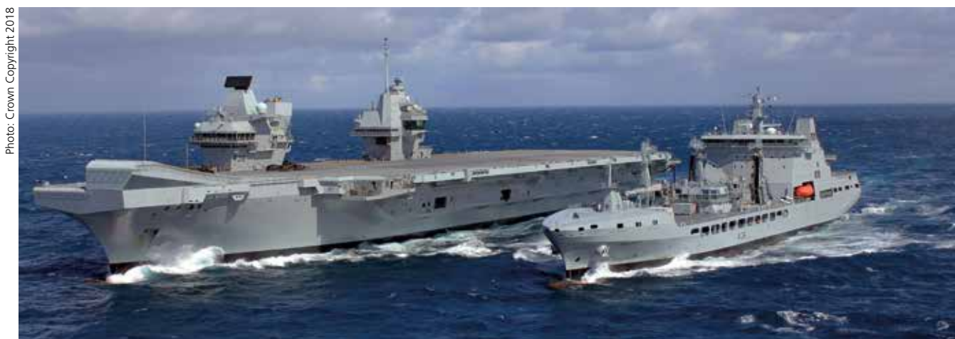
British logistic support ship requirements have been heavily influenced by the need to support the new QUEEN ELIZABETH class aircraft carriers. This is the lead TIDE class fleet tanker TIDESPRING conducting a replenishment at sea exercise with QUEEN ELIZABETH.
