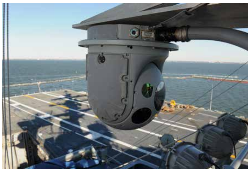
Two electro-optic/infrared sensors placed forward and aft of USS DWIGHT D. EISENHOWER's island provide 360 degree surveillance capability
