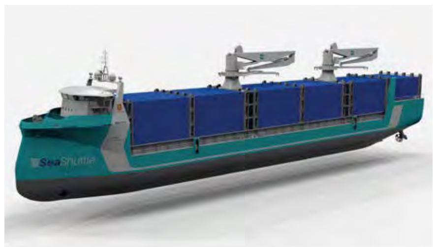
Samskip's SEASHUTTLE project is to cultivate a short distance container ship using hydrogen fuel cells.
