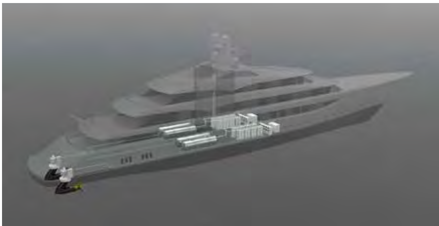
Conceptual layout of MW fuel cell system and hydrogen storage
