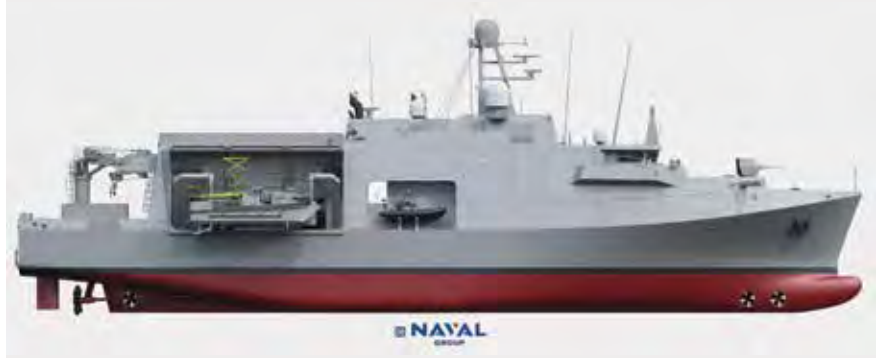
Amidships the MCM motherships are equipped with a large mission bay and Naval Group's Launch and Recovery System (LARS).
