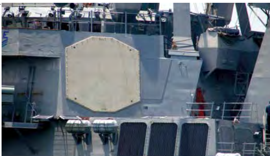
The AN/SPY-1B/D series of naval surveillance radar has given sterling service during its long career. It will be succeeded by Raytheon’s AN/SPY-6(V) family.
