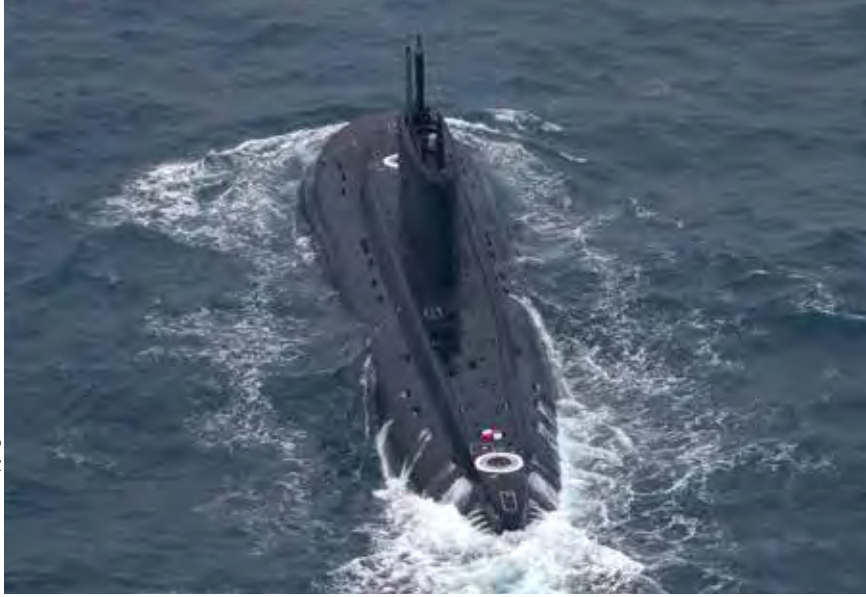
The Project 636.3 VARSHAVYANKA class diesel-electric submarine KRASNODAR is one of twelve improved KILO class submarines ordered for the Black Sea and Pacific Fleets.
