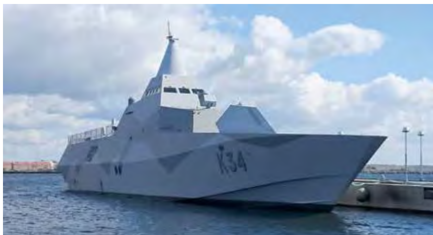
The low RCS design of the Royal Swedish Navy's VISBY class corvettes is representative of the trend for reducing the RCS of comparatively smaller surface combatants.
