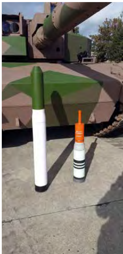
The stark difference size between a 140mm round (left) and a conventional 120mm round (right) is evident. The implications for ammunition stowage and handling are self-evident.
