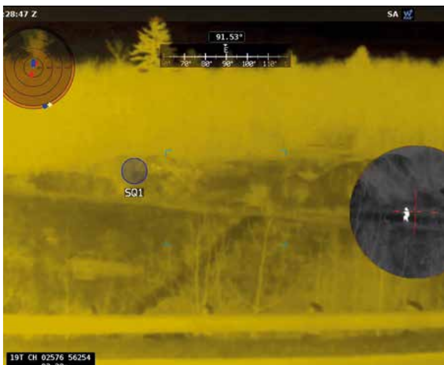
Rapid target acquisition: Thanks to the wireless interconnectivity with the Family of Weapon Sight-Individual, (FWS-I) the weapon site reticle is displayed in the ENVG-B.
