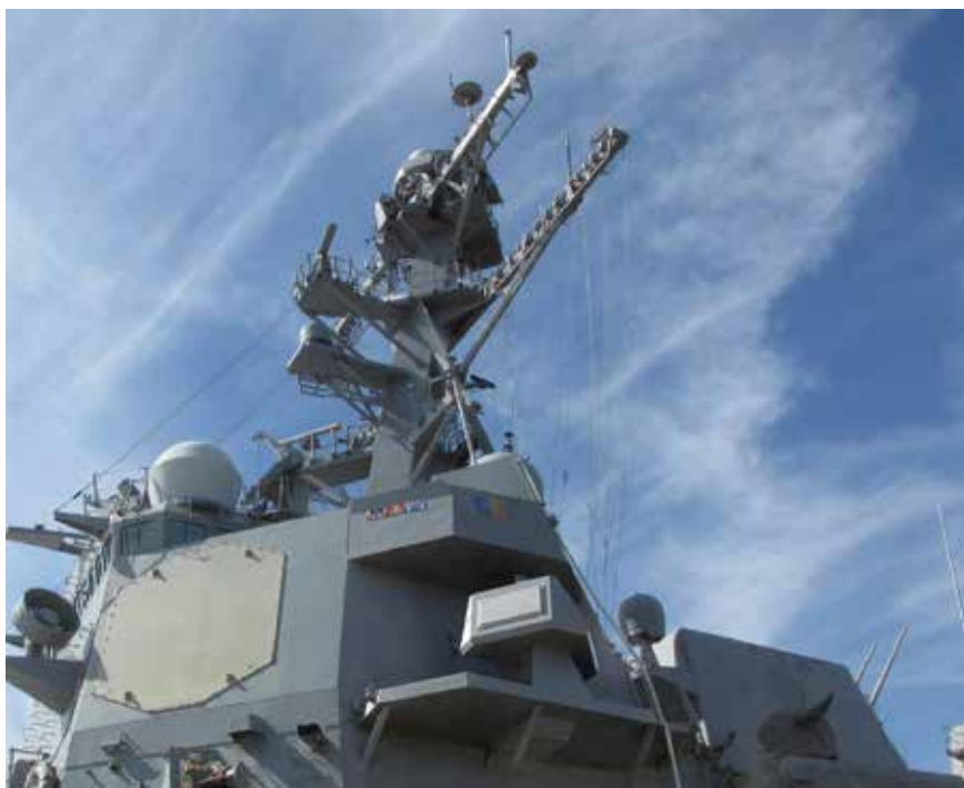
The small rectangular antenna seen on the right-hand side of this photograph on the USN destroyer USS BAINBRIDGE is part of the vessel's SEWIP installation.
