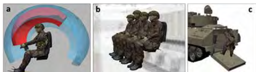
RAMSIS Defense: (a) Analysis of hand grasp areas; (b) analysis of space requirements; (c) movement simulation
