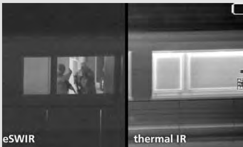
People behind a window - on the left the eSWIR image, on the right a view through a thermal imaging device
