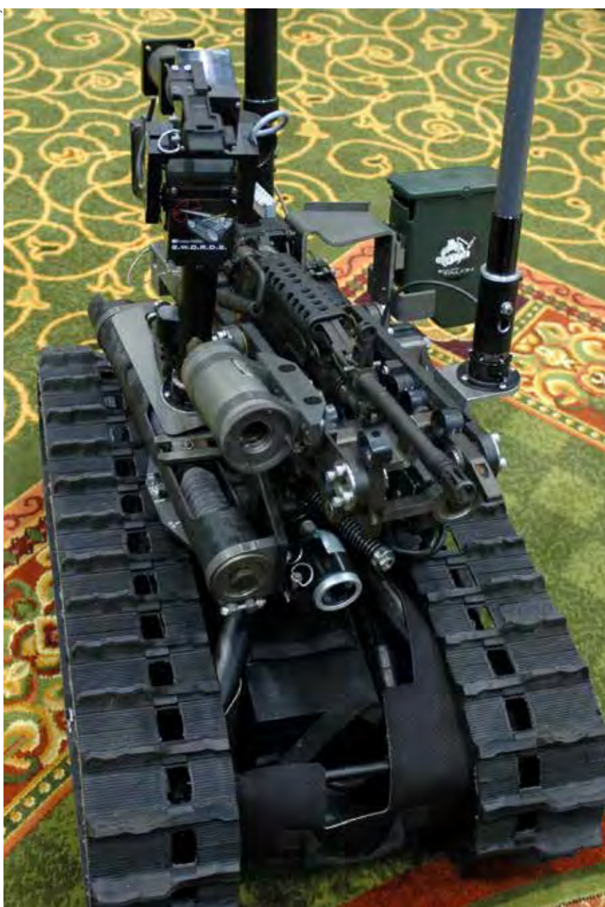
Developed for the US Army, Foster-Miller's Special Weapons Observation Reconnaissance Detection System (SWORDS) was sent to Iraq in 2017, but was never adopted for service.
