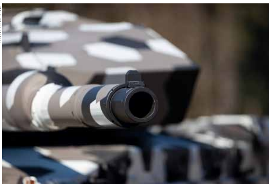
CHALLENGER 2 demonstrator fitted with new turret armed with Rheinmetall 130mm smooth-bore gun
