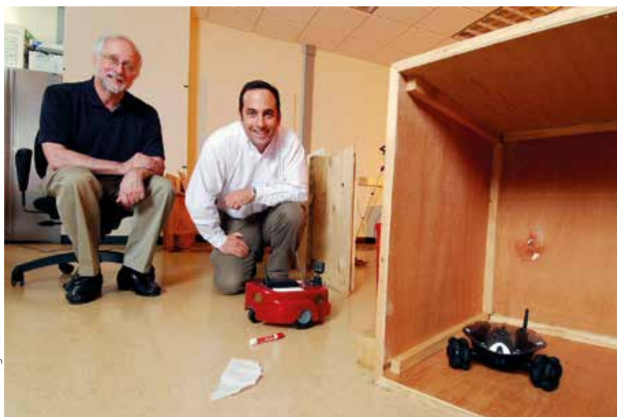
At Georgia Tech, Professor Ronald Arkin (left) is developing algorithms that will allow a robot to use tactics intended to deceive a human or other robot, reducing its chance of being detected and tracked. In this test conducted by Arkin and research engineer Alan Wagner (centre), the black robot deliberately knocked down the red marker in order to deceive the red robot, then hid inside the box seen on the right.
