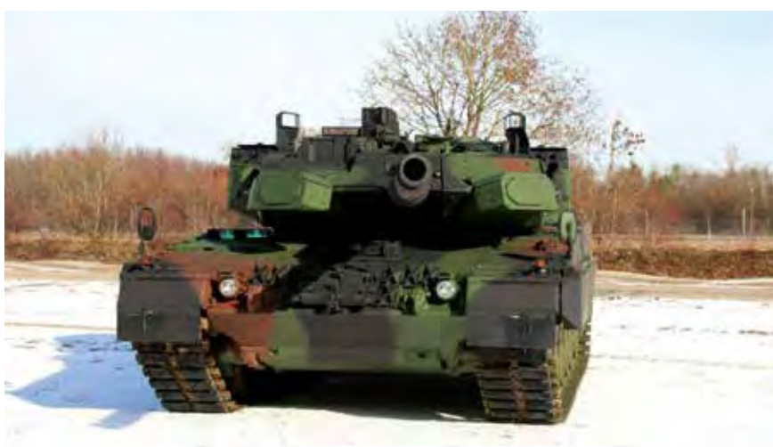
Germany's LEOPARD 2A7A1, the latest LEOPARD 2 development, will mount the L55A1 main gun and ultimately will fire the KE2020Neo round. It is will also be fitted with the TROPHY HV Active Protection System (APS).
