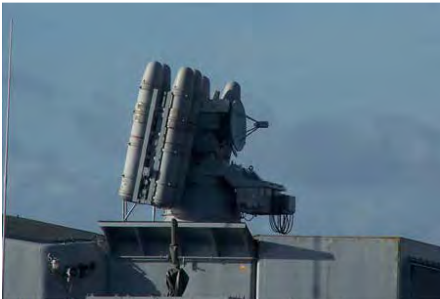
Radar echoes produced by structures like missile launchers have led to such systems being recessed in a ship's hull to help reduce RCS.
