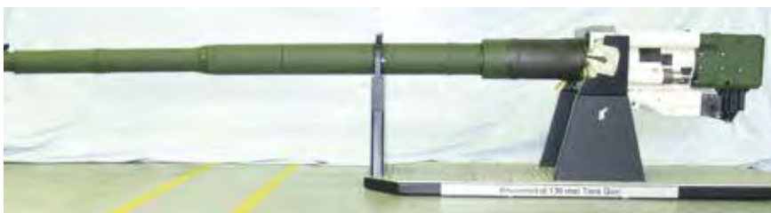
The 130mm L/51 gun is a substantial increase in size and mass over the existing 120mm weapon, but is claimed to bring up to 50% increase in performance.
