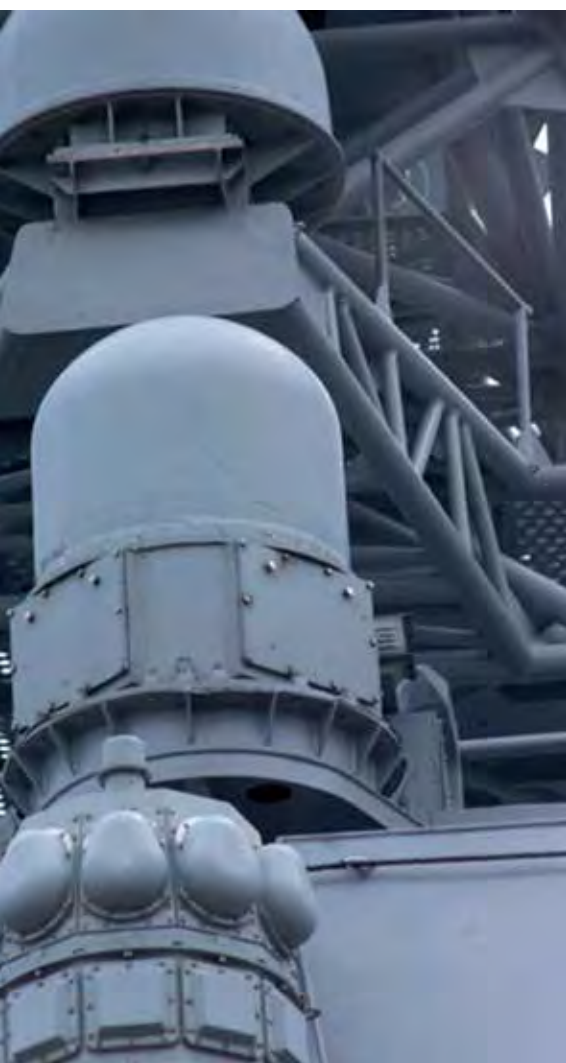
Russia's TK-25E shipborne electronic countermeasures system is designed to intercept and jam RF emissions from target-acquisition radars, fire-control radars, and anti-ship missile seekers.
