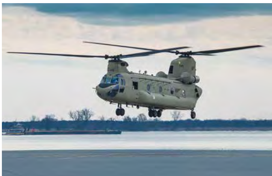
The CH-47F features an integrated digital cockpit management system. It is also equipped with advanced capabilities that enable efficient cargo handling.
