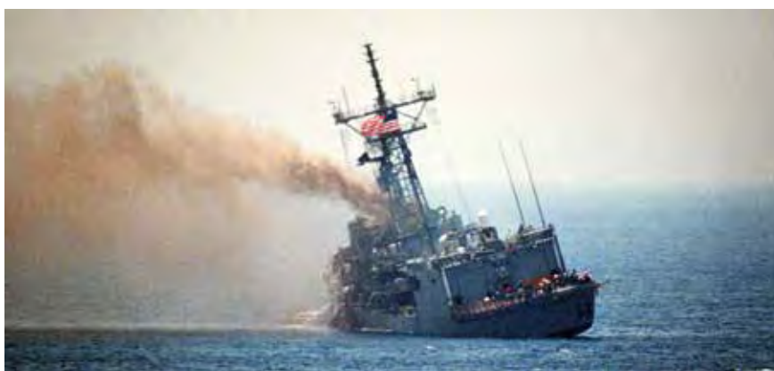
The USN frigate USS STARK was hit by two Iraqi EXOCET missile on 17 May 1987. Although the ship's Super Rapid Blooming Offboard Chaff (SBROC) launchers were armed, they were not used. Following the missile impacts, the ship's captain ordered that the starboard side be deliberately flooded in order to keep the hole on the hull's port side above water.
