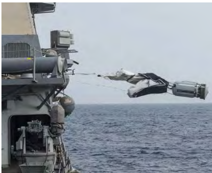
The USN destroyer USS RAMAGE launches a MK-59 decoy. Made by Irvin Aerospace and marketed as the IDS300, this inflates after release, and floats on the sea surface.
