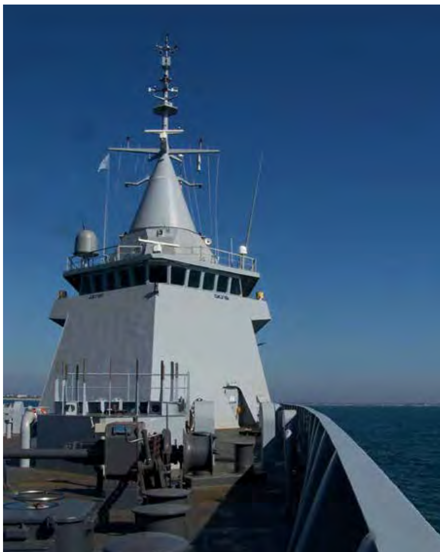
Integrated masts like that equipping the Argentine Navy's ARA BOUCHARD OPV are a major step forward in helping reduce the RCS of a ship's superstructure.
