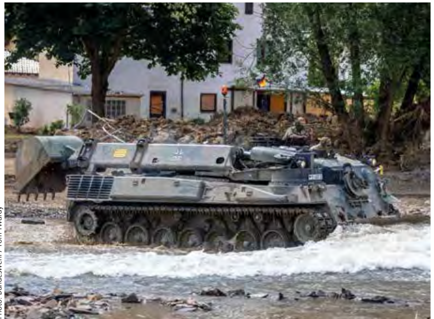
German soldiers use a DACHS engineer tank to dredge a ford for disaster relief vehicles during the flood in the Ahr Valley, on 26 July 2021.
