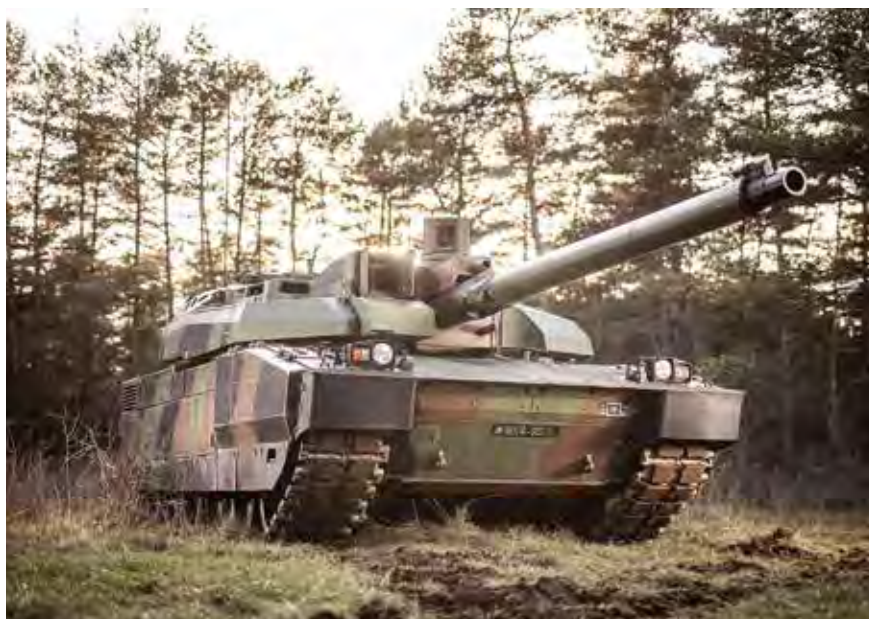
The French Army will retain 200 LECLERC MBTs which will be upgraded by Nexter Systems to extend their operational lives. The LECLERC is the only MBT in NATO armed with a 120 mm smooth-bore gun fed by an automatic loader.
