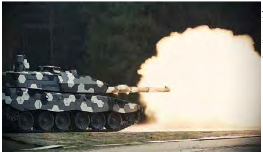
A CHALLENGER 2 testbed hull mounting Rheinmetall's new turret and 130mm L/51 smoothbore gun
