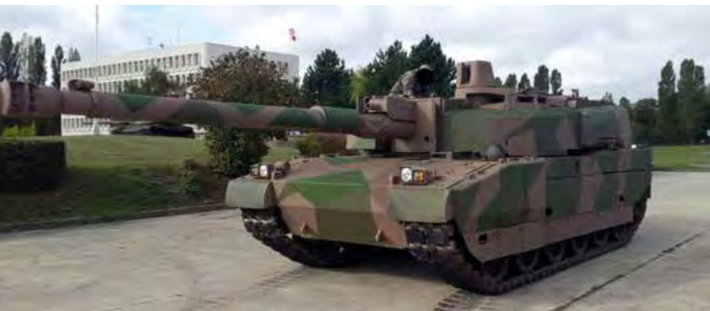
The so-called LECLERC "Terminateur", a testbed platform mounting Nexter's 140mm smoothbore gun on the existing LECLERC hull
