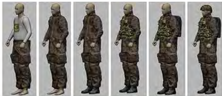
(a) Rough scan; (b) conversion into a CAD model; (c) data volume reduction; (d) color scan overlay
