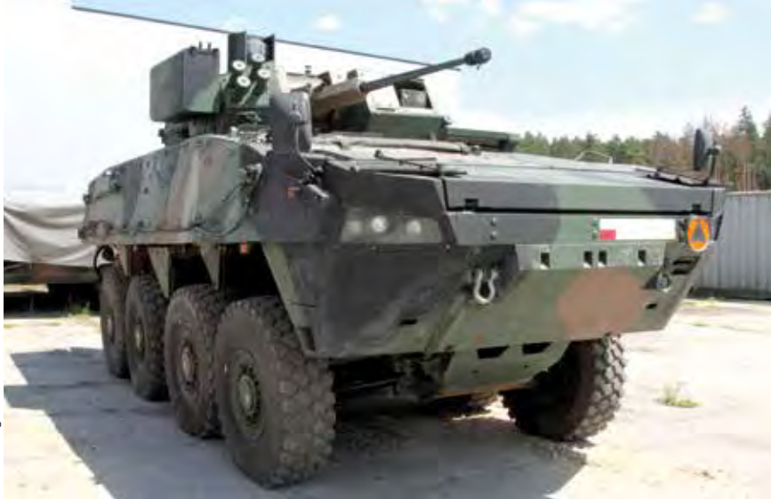
Wheeled IFV ROSOMAK equipped with ZSSW 30 remote controlled turret system
