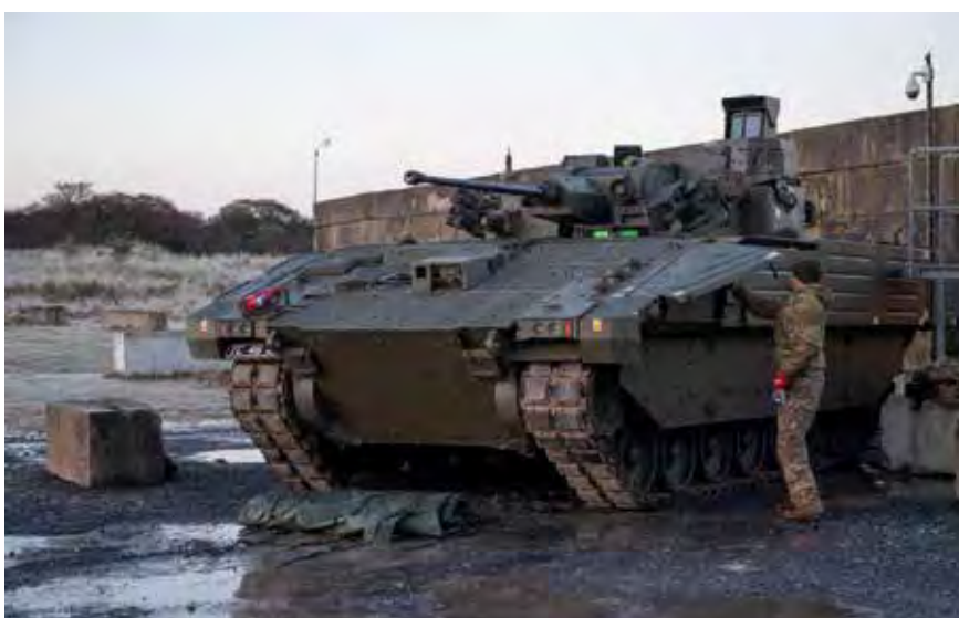
The AJAX ISTAR variant is equipped with the CTA International Case Telescoped Armament System (CTAS) 40mm CT cannon. This image comes from the AJAX firing trials. The AJAX programme is beset with difficulties due to noise and vibration impacts on crew health.
