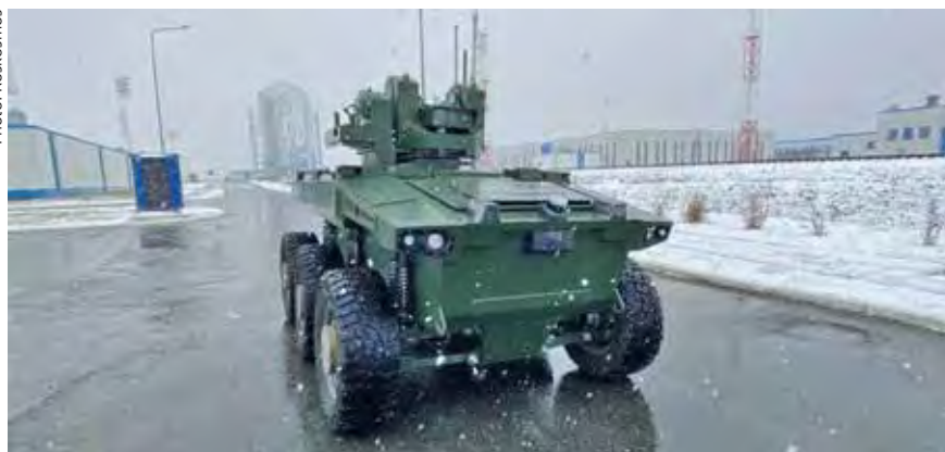
The Foundation for Advanced Research (FPI) is developing the autonomous capabilities of the Marker UGV to operate in a group and interact with other robots.
