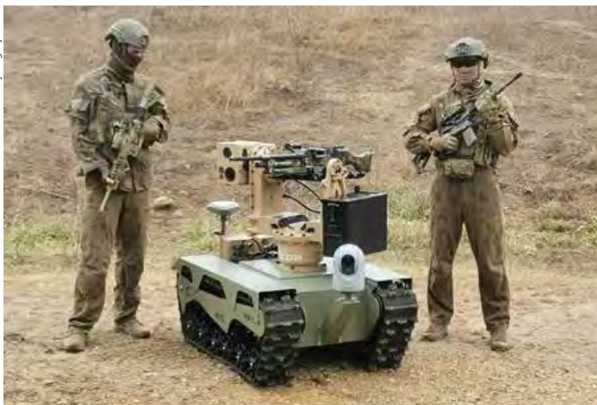
The WARFIGHTER UGV is equipped with the vision-based ATHENA AI system for target evaluation, terrain analysis and integrated Rules of Engagement (RoE) considerations.
