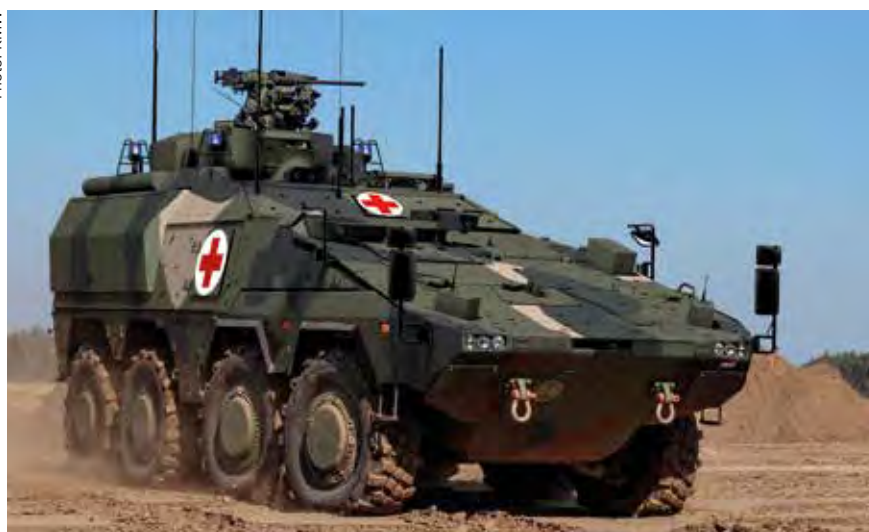
The ARTEC BOXER (8x8) is being fielded in a wide range of battlefield missions including the ambulance with a raised roof line for more internal volume.
