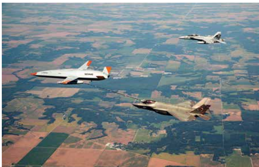
A MQ-25 test aircraft uses the probe-and-drogue method to refuel an F-35 combat aircraft in September 2021.
