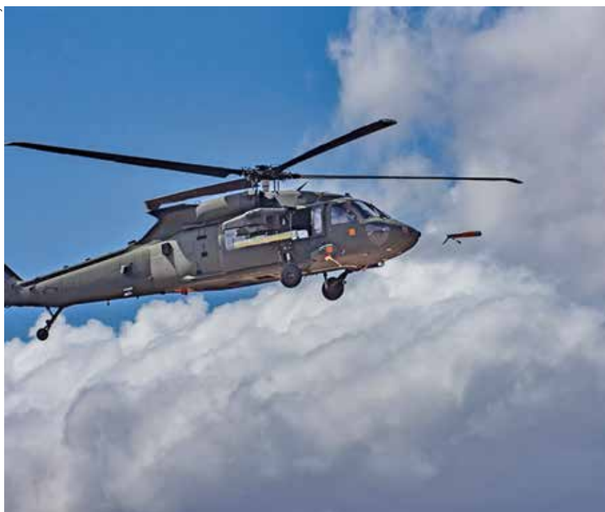
Launch of an ALTIUS 600 tube-launched UAV from a US Army UH-60 BLACKHAWK helicopter. Similar air-launched effectors are likely to be deployed on the FLRAA.
