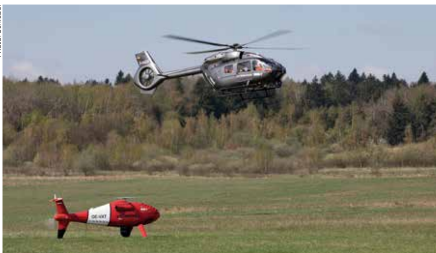
Various continental armies are pursuing MUM-T capabilities. In 2018, an Airbus H145 manned helicopter and a Schiebel S-100 CAMCOPTER demonstrated Level 5 teaming (the helicopter crew controlled all aspects of the UAV's flight including take-off and landing), with the UAV conducting reconnaissance ahead of the H145.
