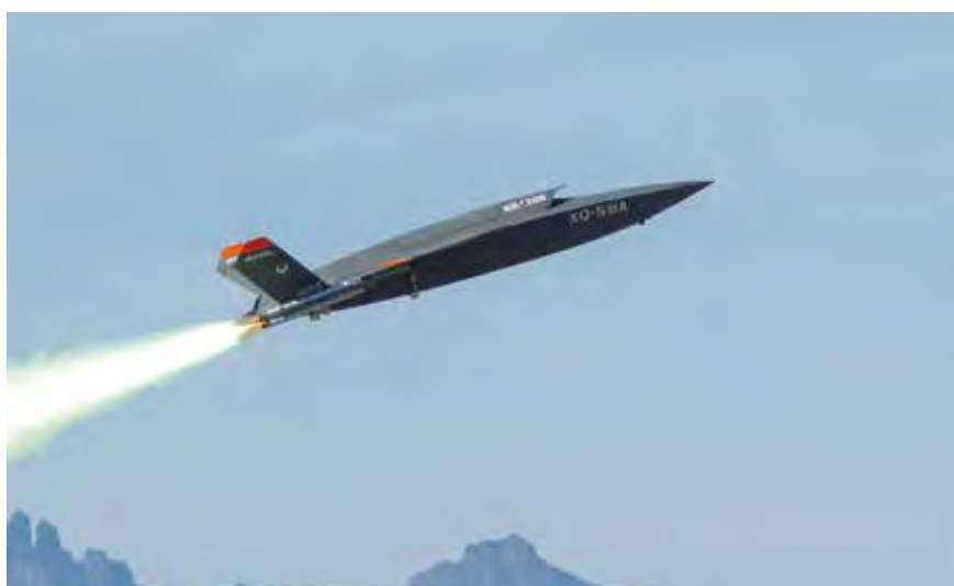
A VALKYRIE prototype utilising Rocket-Assisted Take-Off (RATO) to operate from short or improvised runways
