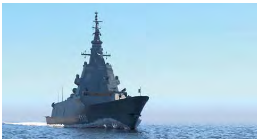
Spain is contributing to the naval Alliance and European BMD efforts with the ÁLVARO DE BAZÁN class F-100 frigates' AEGIS combat system and ANISPY-1D radar, which will be further enlarged with the new class of F-110 frigates entering service from 2027.
