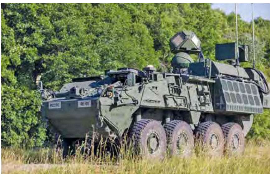
The DE variant of US Army STRYKER M-SHORAD mounts a radar, electro-optical cueing system and 60kW laser used as an air defence and counter-UAS weapon.
