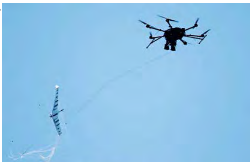
Fortem Technologies' DroneHunter is part of the SkyDome C-UAS system.
