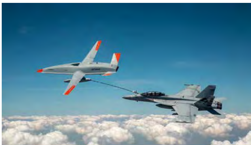
The Boeing MQ-25 T1 test asset transfers fuel to a US Navy F/A-18 SUPER HORNET in 2021, marking the first time in history that an unmanned aircraft has refuelled another aircraft.
