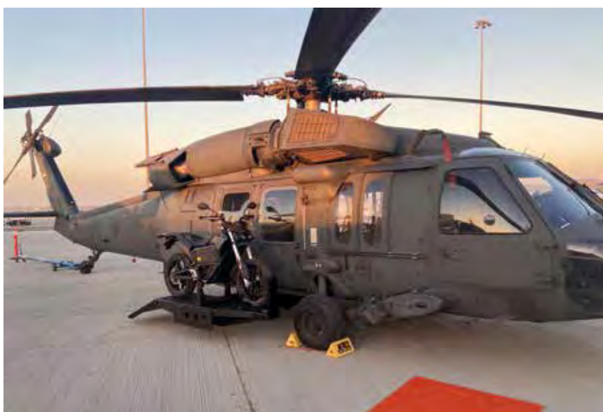
The UAE Special Forces have developed, together with Sikorsky, a kit that can transport two electro-bikes at the sides of the BLACKHAWK.
