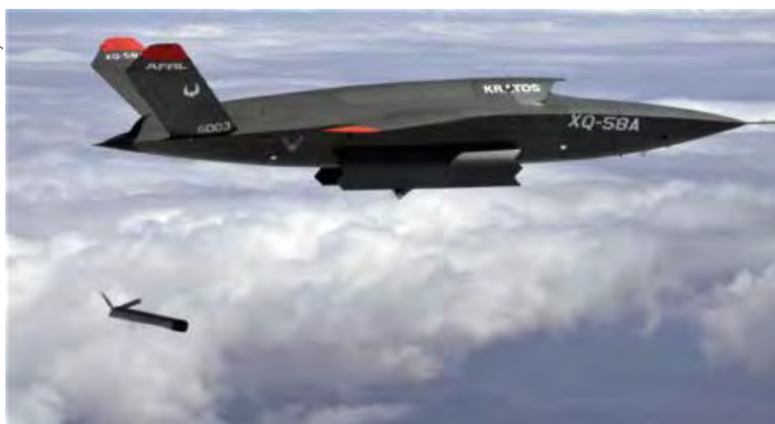
The XQ-58A VALKYRIE demonstrates the separation of the ALTIUS-600 small UAS in a test at the U.S. Army Yuma Proving Ground test range, Arizona. This test was the first time the weapons bay doors have been opened in flight.
