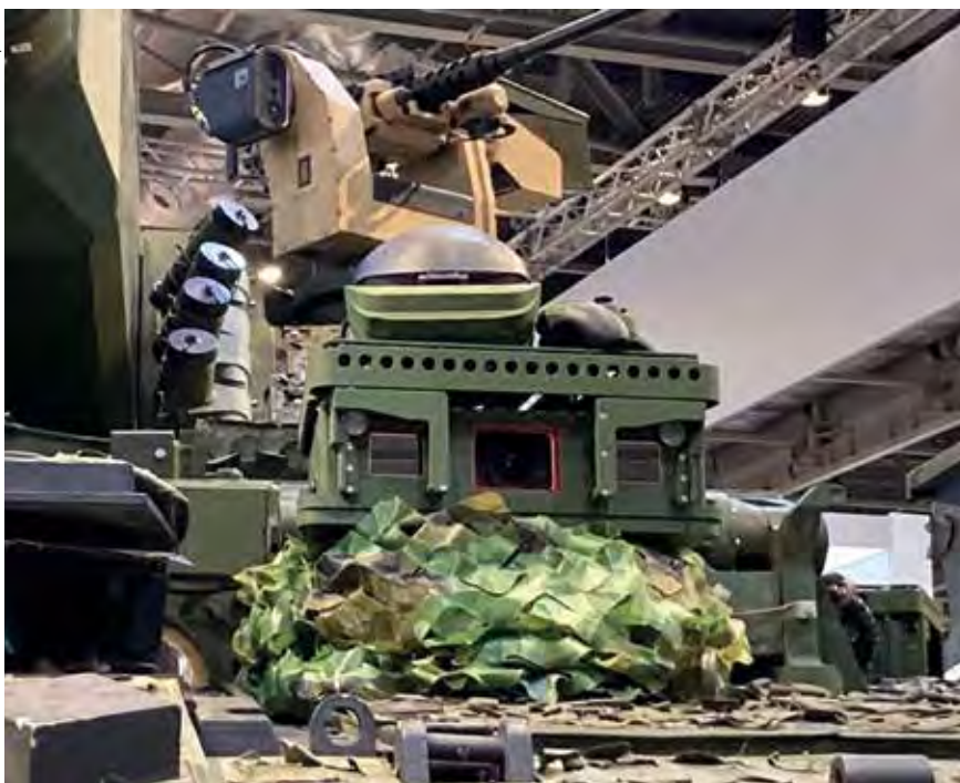
This integrated camera module (ICM) is part of the SETAS (see-through armour system) from HENSOLDT. The camera views can be displayed on digital screens or in augmented reality on helmet-mounted displays shown above the ICM.
