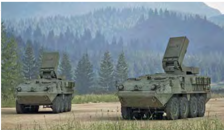
Illustration depicting Epirus' LEONIDAS HPM effector mounted on a C-UAS STRYKER.
