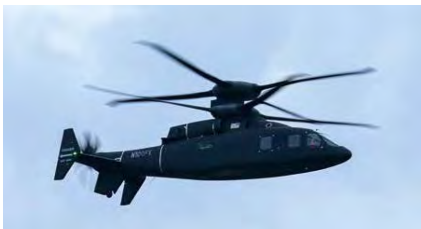
The Sikorsky-Boeing technology demonstrator SB-1 DEFIANT first took flight in March 2019 and leverages Sikorsky's X2 technology with a rigid compound rotor and pusher propeller.
