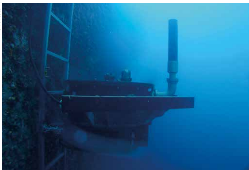
The Israeli DSIT Solutions' AQUASHIELD fix installation Diver Detection Sonar (DDS) system operating at 'a 60 KHz central frequency' offers a long range detection with up to 3,000 metres diameter coverage.
