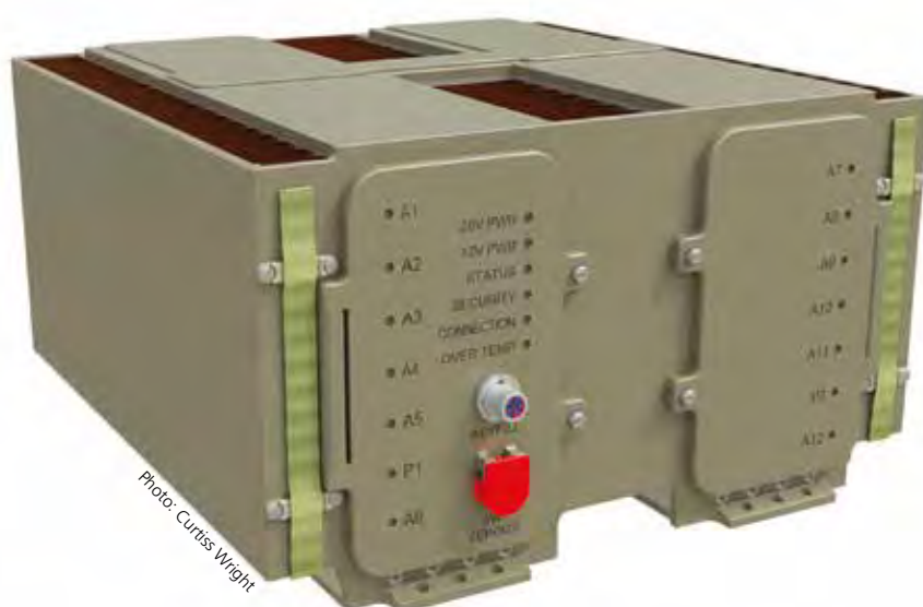
This 8-slot, user integration-ready powered enclosure uses natural convection cooling and is aligned to serve as part of the A-kit hardware infrastructure of the Modular Open Systems Approach (MOSA) for all future military platforms.
