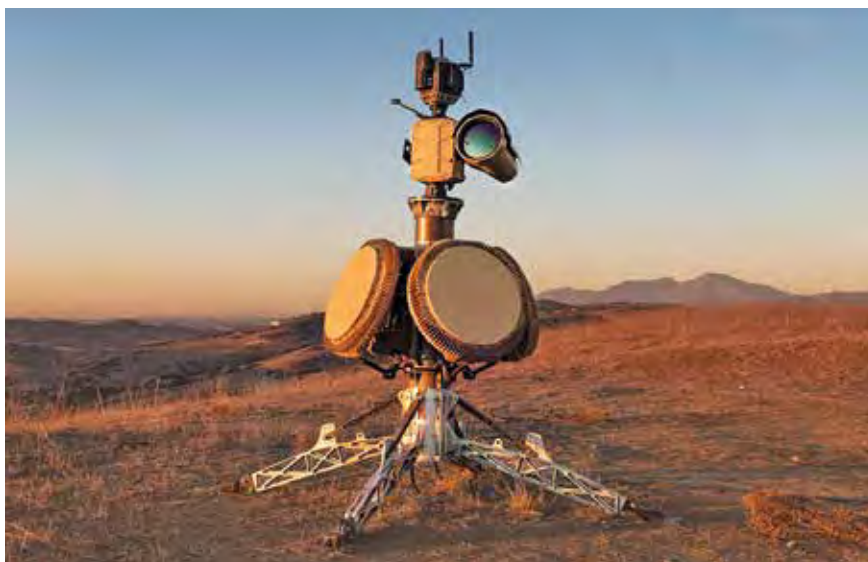
Anduril's sentry towers connect to lattice C2 system to detect and track rogue drones threatening perimeters of military bases.
