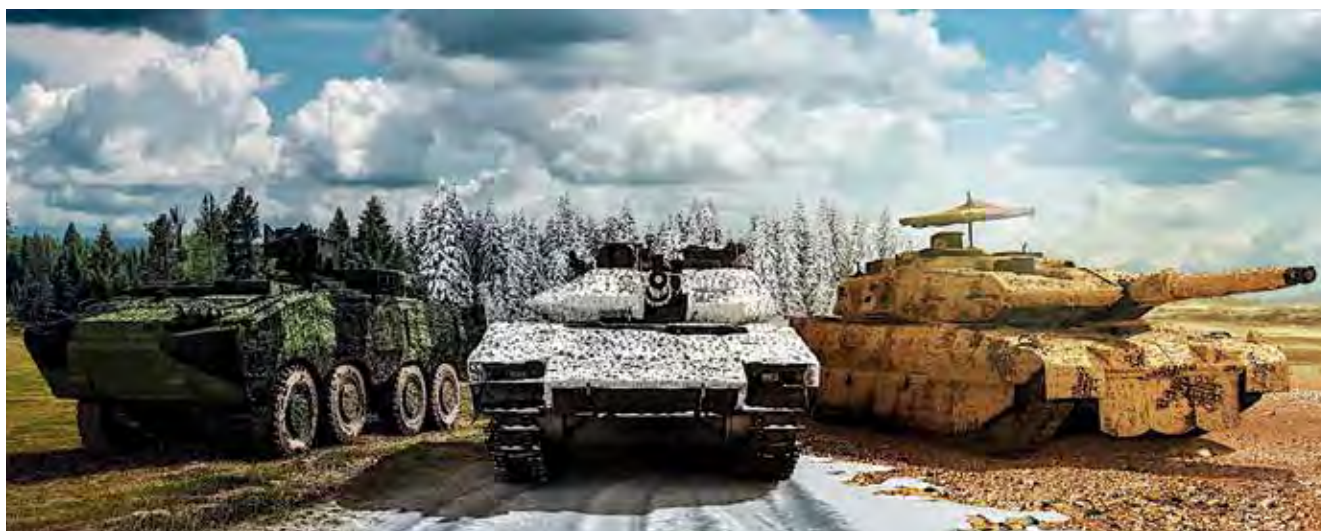
Military vehicles need new multispectral camouflage to neutralise threats. The SAAB Mobile Camouflage System (MCS) is a multispectral camouflage designed to reduce optical and thermal signatures while the vehicle is stationary or on the move.
