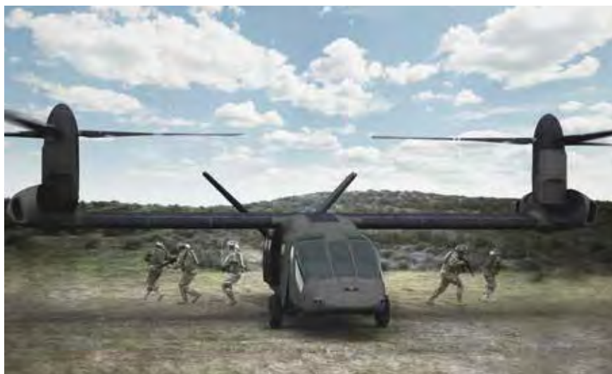
Soldiers egress through two 1.8 metre wide sliding doors in this artist concept of the V-280 VALOR technology demonstrator, as presented in 2015.
