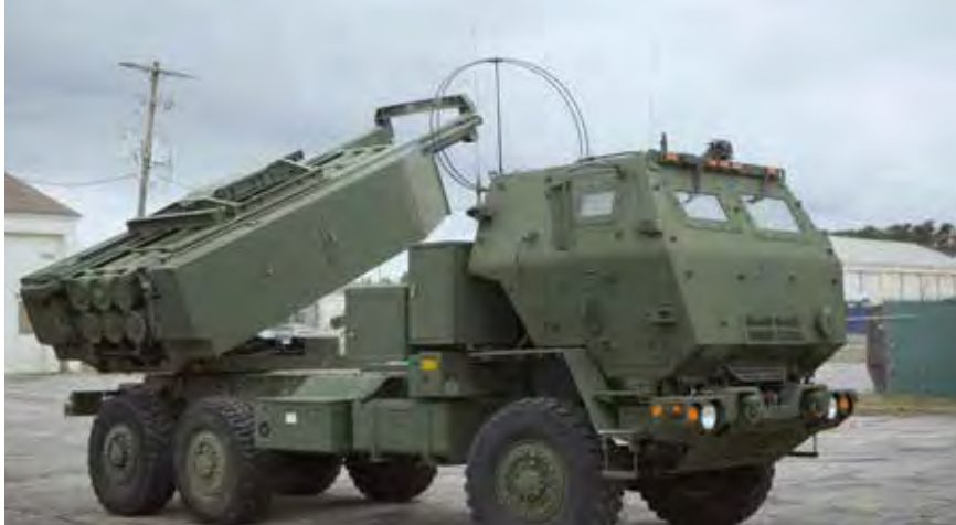
An M142 High Mobility Artillery Rocket System (HIMARS) conducts pre-shoot standard operating procedure checks at Marine Corps Air Station Cherry Point, North Carolina in March 2021. HIMARS is mounted on the FMTV tactical truck and can use a six-rocket MLRS pod or a single ATACMS rocket.
