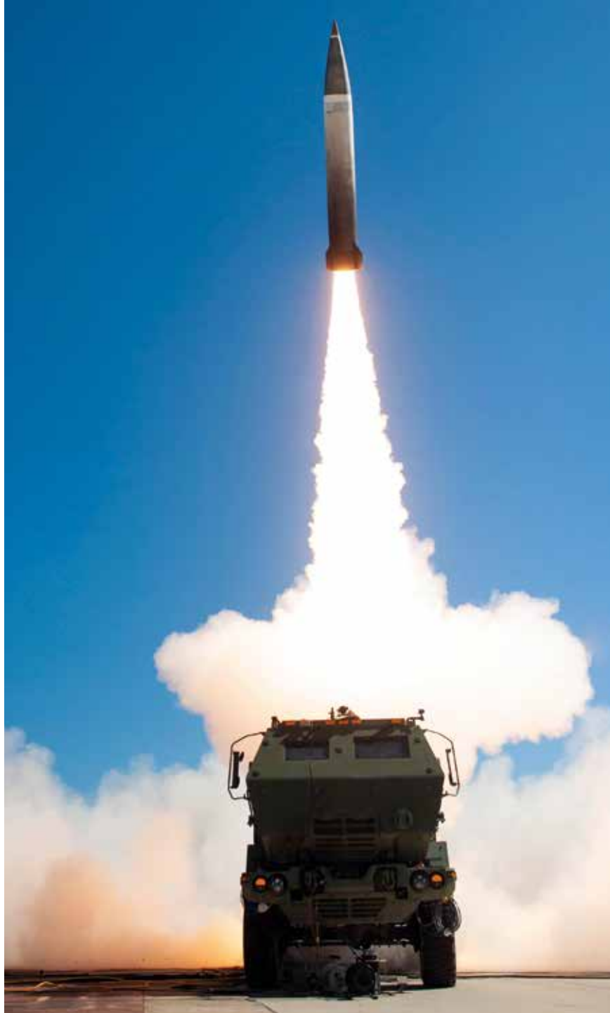
A Lockheed Martin Precision Strike Missile (PrSM) launches from a HIMARS at Vandenberg Space Force Base, California, in October 2021. PrSM will give MLRS users a deep fires weapon to replace ATACMS; it will have a range in excess of 499 km.
