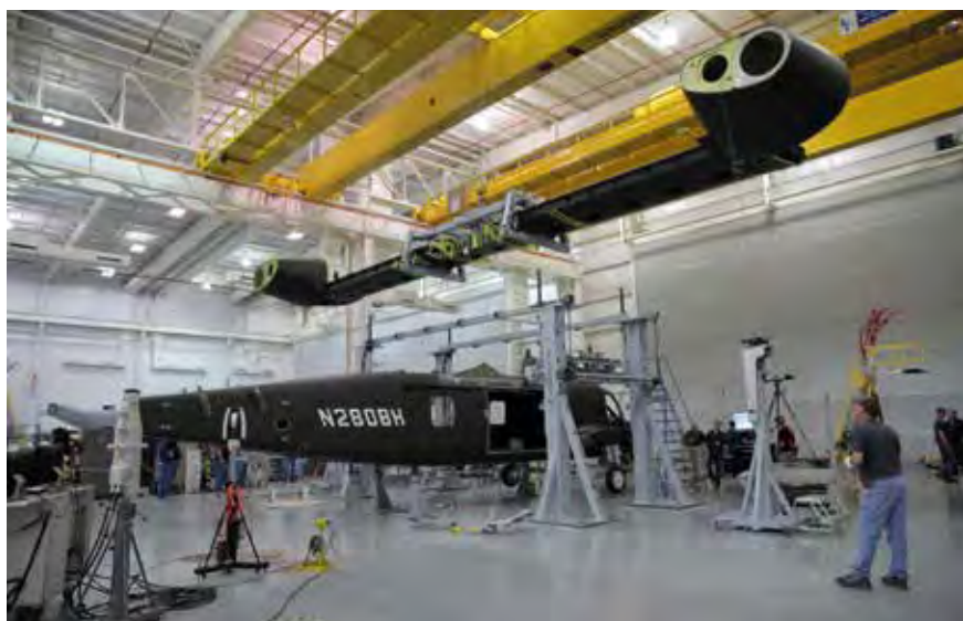
A wing is lowered onto the fuselage of a Bell V-280 VALOR at the Bell facility in Amarillo, Texas.
