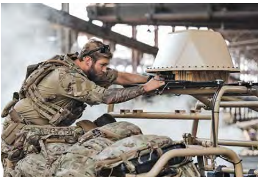
Fitted on top of such all-terrain vehicles, Drone Sentry X provides a mobile protection bubble for vehicles and convoys.
