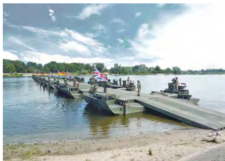
German and British Army M3 Amphibious Bridge and Ferry System units coupled together to form a bridge
