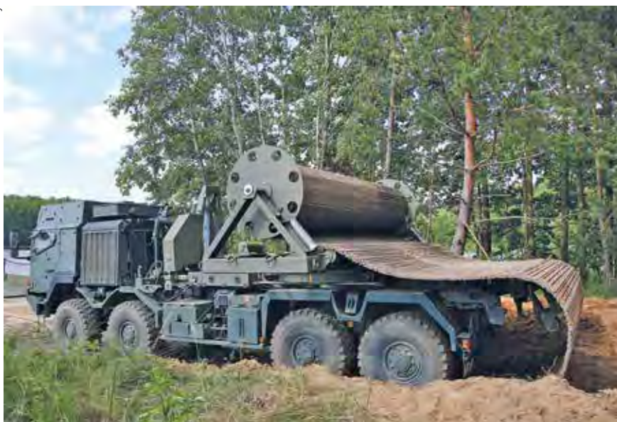
A Faun TRACKWAY Heavy Ground Mobility System (HGMS) being laid over rear of Rheinmetall MAN Military Vehicles (8x8) truck with a protected cab at a bridge crossing point
