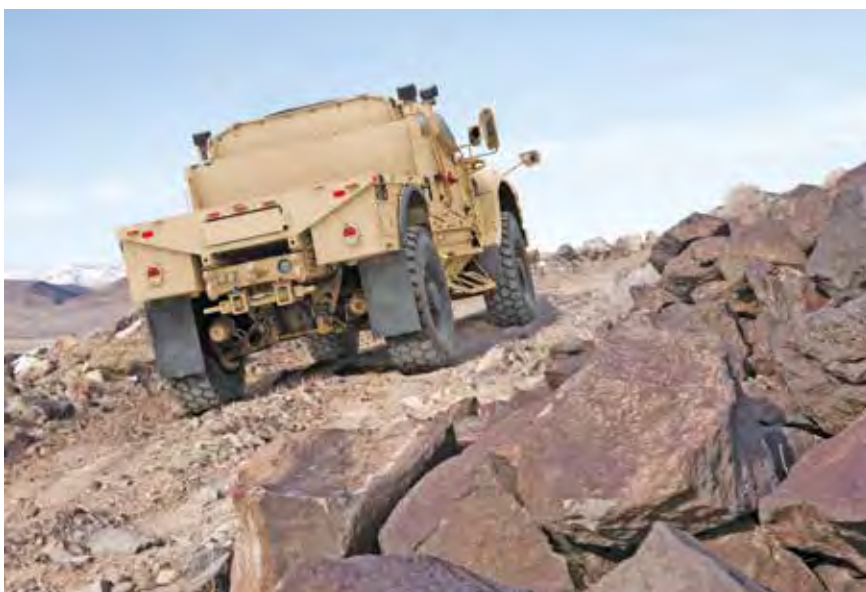
The MATV Utility variant seats 5 and has a 3,181 kg payload capacity. The flatbed has ISO-lock corner fixings.
