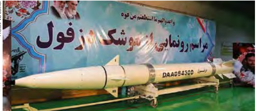
DEZFUL is a surface-to-surface ballistic missile of the FATEH family. With a weight of 1.5 tonnes and a length of more than 12 metres it is said to reach a range of up to 1,000 kilometres.
