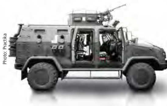
The KOZAK 2M1 has four side doors and a rear hatch for easy egress.
