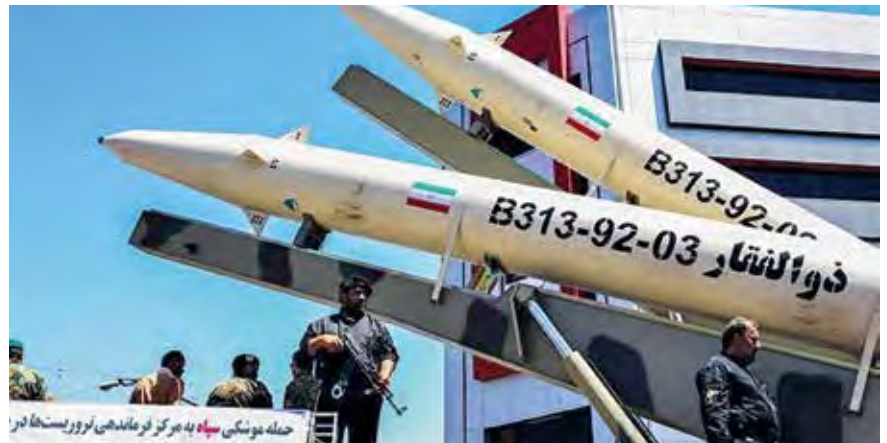
ZOLFAGHAR is a road-mobile, [2] single-stage, solid-propelled SRBM believed to be derived from the FATEH-110 SRBM family. It entered service in 2017 as a longer range version of the FATEH-110 SRBM.
