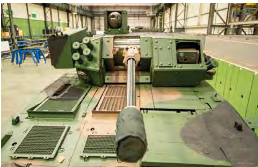
The main armament of Poland's BORSUK is the ATK Mk44 BUSHMASTER II 30 mm cannon and two SPIKE-LR ATGMs
