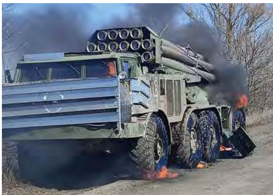
A destroyed BM-27 URAGAN 9P140 16-tube 220 mm calibre MRL system. Each BTG has an attached MRL battery.
