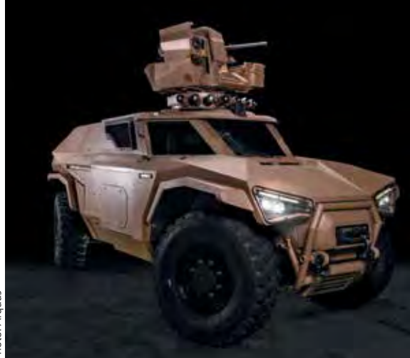
The SCARABEE compact armoured vehicle with remote weapons turret
