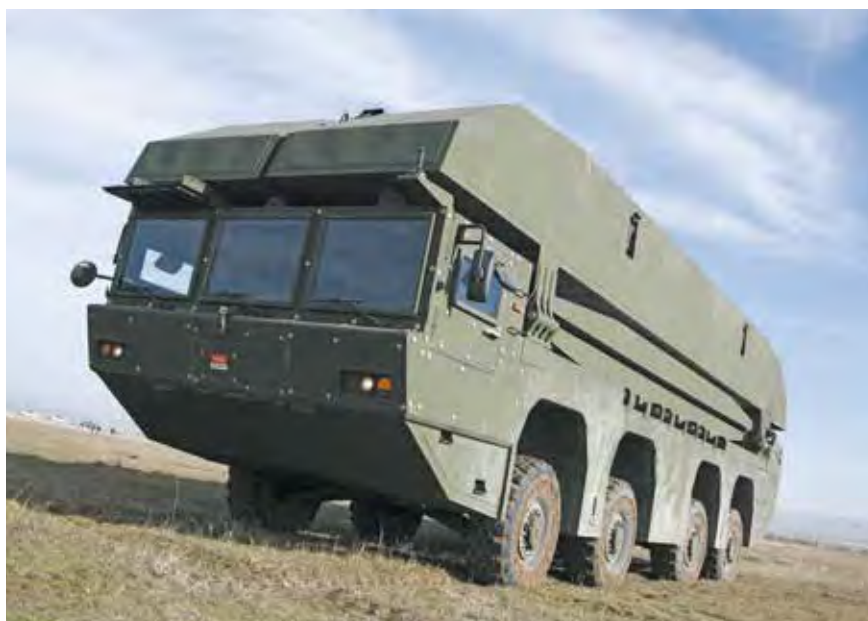
The Single Turkish OTTER rapid deployable amphibious wet gap crossing system in travelling configuration and showing armoured cab at the front
