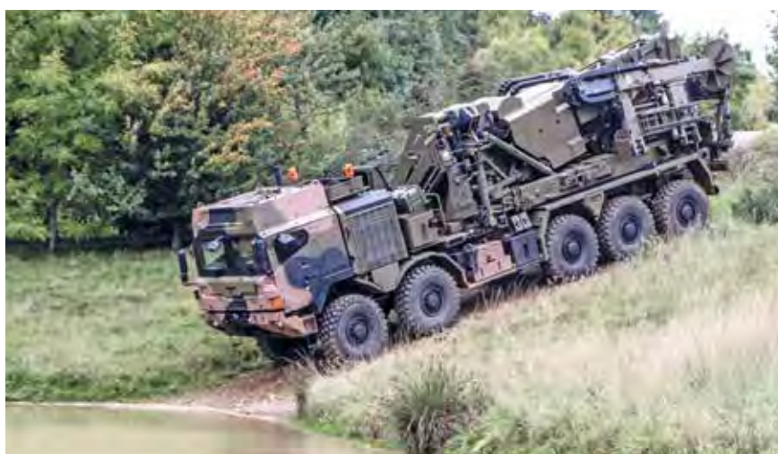
An Australian Army WFEL Dry Support Bridge launcher-based on a Rheinmetall MAN Military Vehicles (10x10) cross-country chassis with fully protected cab
