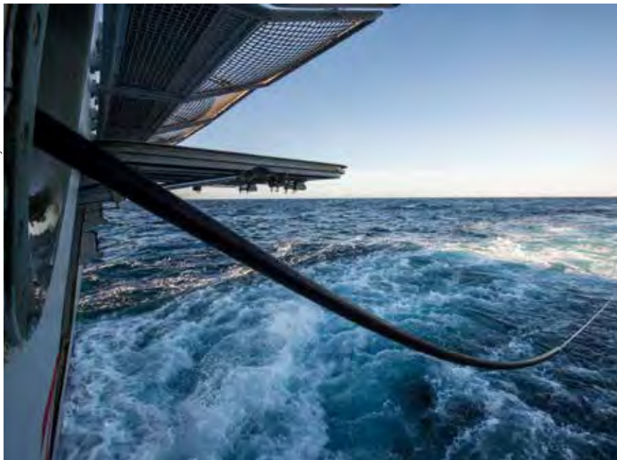
More than 60 CAPTAS systems are in operation across 10 member navies and more systems and naval forces are coming. Depicted here is the towed passive array deployed by Italian Navy's CARABINIERE ASW FREMM.
