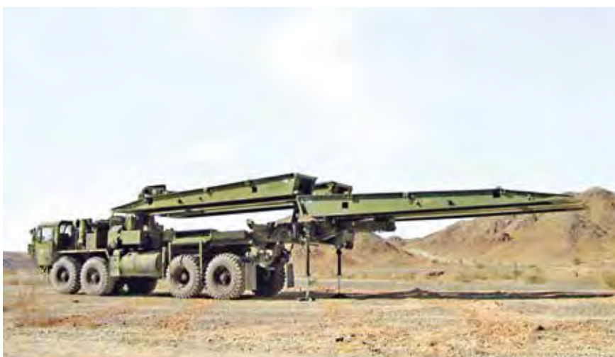
A US Army GDELS-Bridging PYTHON Rapidly Emplaced Bridge System (REBS) being launched over the rear of the Oshkosh (8x8) truck chassis with two bridge elements almost aligned and stabilisers lowered
