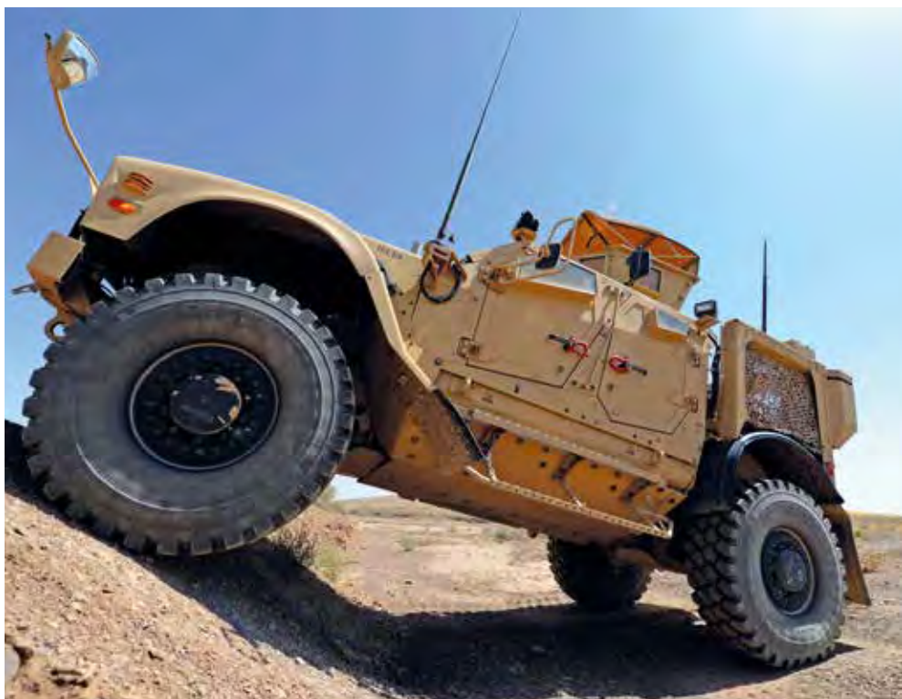
The MATV climbs a 60% gradient and crosses a 50 cm trench.
