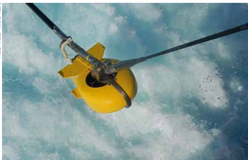
Thales offers the smaller CAPTAS-1 with a typical detection range up to 30 km, for installation on Offshore Patrol Vessels (OPVs) down to about 800 tonnes, using a single dependent tow for both the active sonar source and a triplet receiver array.
