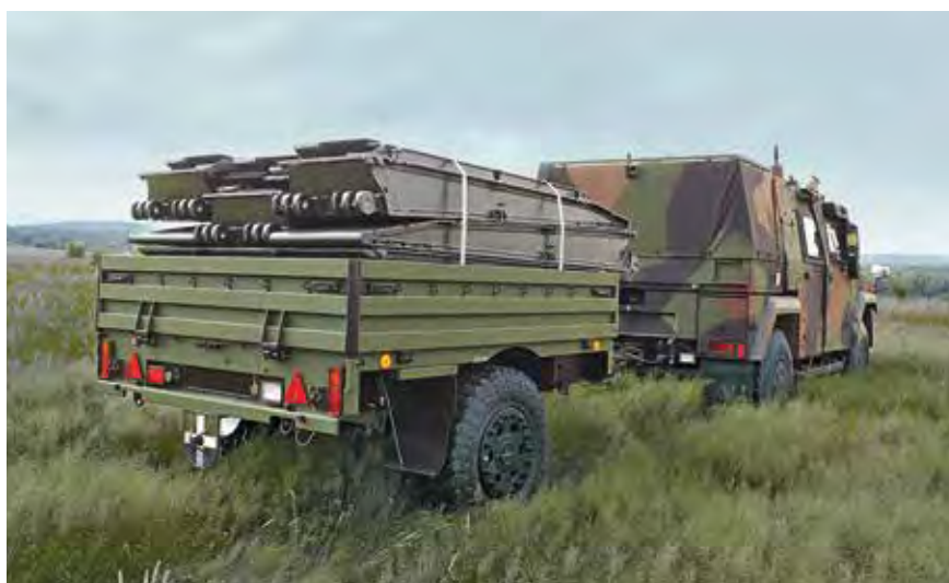
The VIPER in travelling configuration with bridge elements in a trailer being towed by an EAGLE (4x4) vehicle
