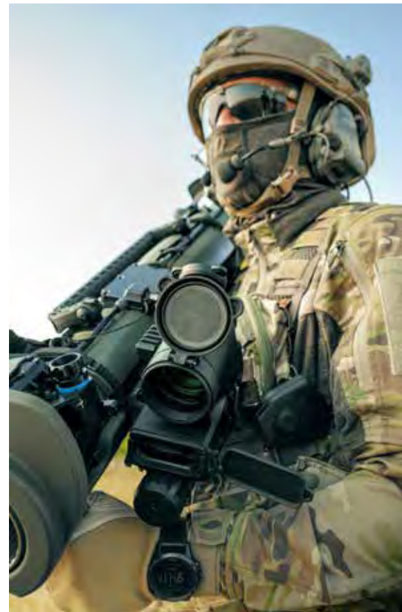
The FCS13RE multi-weapon fire control system mounted here on a CARL GUSTAV M4
