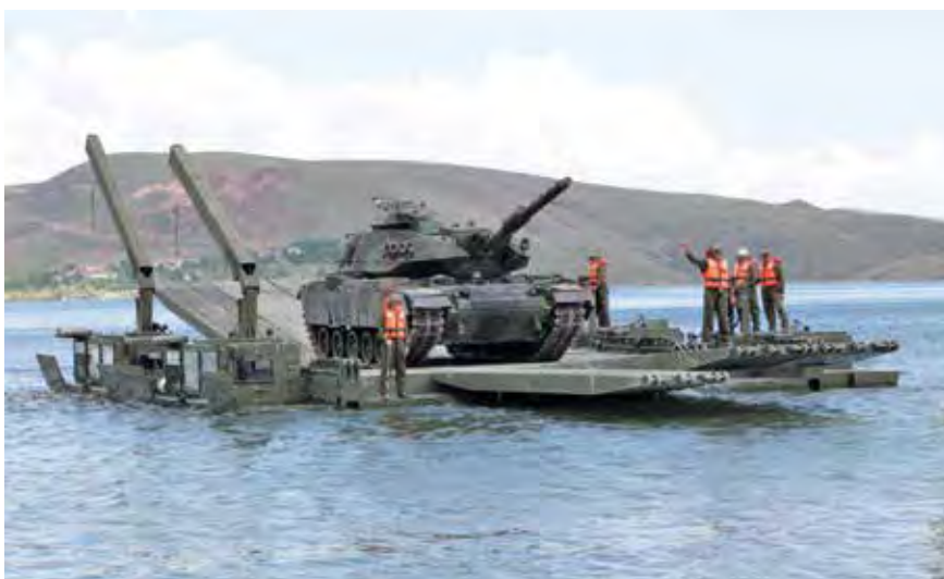
Two units of the Turkish OTTER rapid deployable amphibious wet gap crossing system being used as a ferry with ramps raised and transporting an upgraded M60T MBT
