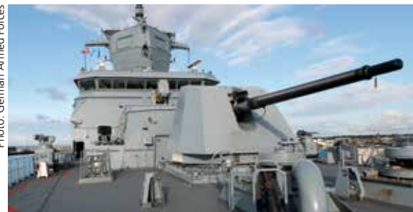
As is the case for their predecessors, Germany's F126 class frigates will be armed with the OTO 127/64 (LW) VULCANO naval gun.
