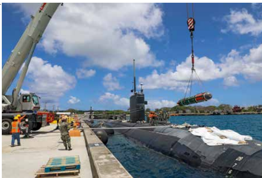
A Mk 67 Submarine Launched Mobile Mine (SLMM) is loaded into the US Navy attack submarine ANNAPOLIS (SSN-760). Using a handful of UUVs to clandestinely lay mines, instead of laying them with a valuable, multi-mission submarine is a self-evident improvement.
