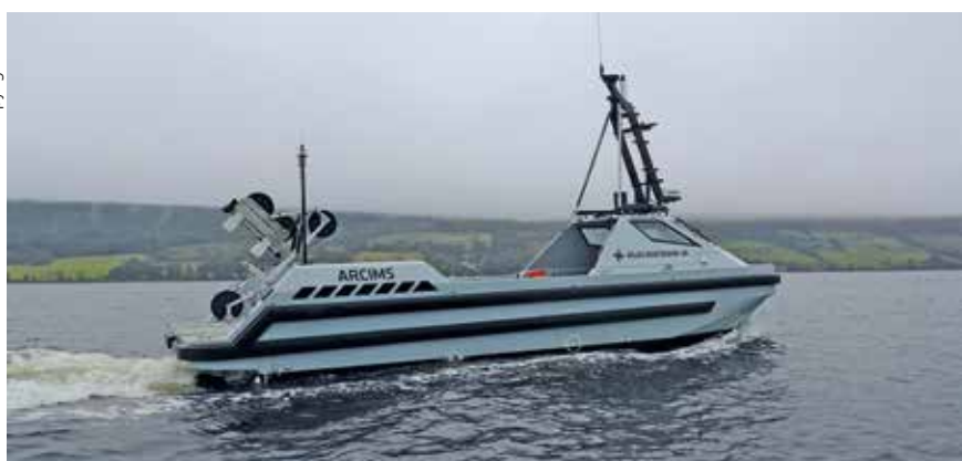
The British Royal Navy's ARCIMS (Atlas Remote Capability Integrated Mission Suite) modular 11 metre USV is one of the many un-crewed systems that are being increasingly used for MCM.
