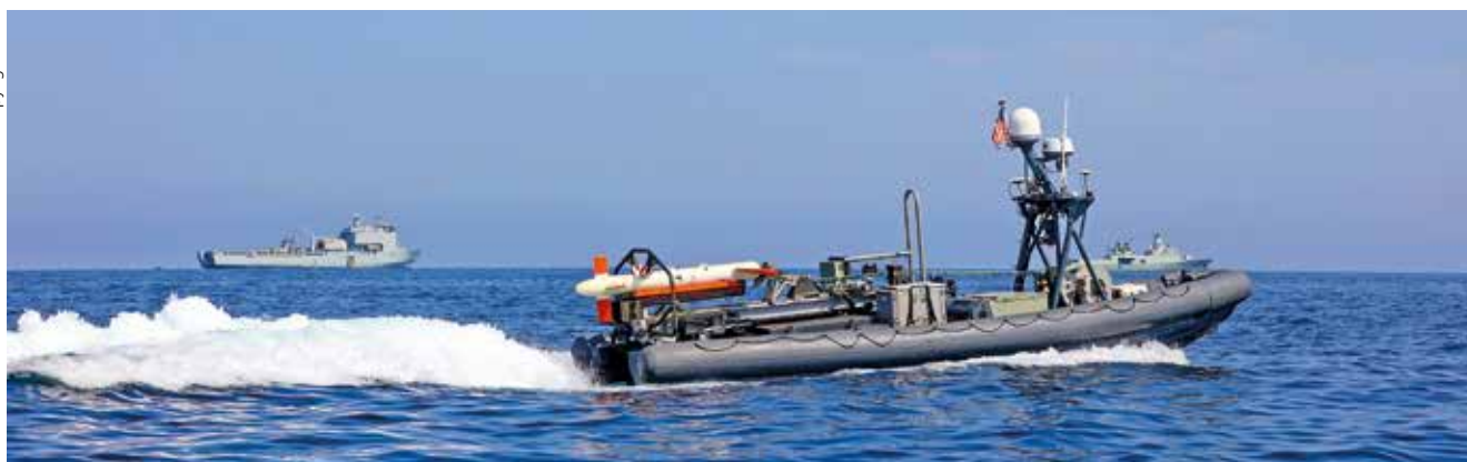
An unmanned US Navy RHIB deploying the AN/AQS-24 mine hunting sonar system participates in MCM operations. The extent to which mines sink ships and stymie fleets in any given situation will depend heavily on the extent to which each side wields emerging mine warfare technologies well.
