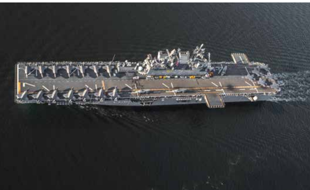
An April 2022 picture of the US Navy amphibious assault ship TRIPOLI (LHA-7) with as many as 20 F-35B LIGHTNING II strike fighters embarked as part of ongoing trials of the "Lightning Carrier" concept.
