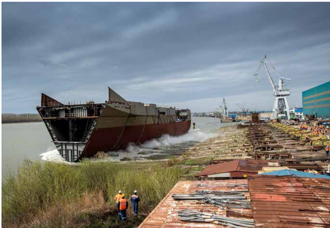
Launching of the partly completed hull of the Combat Support Ship on the site of Damen Shipyards Galati in Romania.
