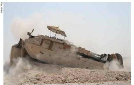
Wisent 2 Armoured Support Platform in AEV configuration using its front mounted dozer blade and with crane with bucket attach in stowed position
