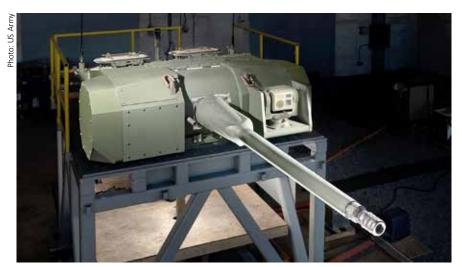
The XM913 shown here is designed to enhance the lethality of the US Army's next generation IFV. It is chambered for the 50 mm 'Supershot' cartridge.
