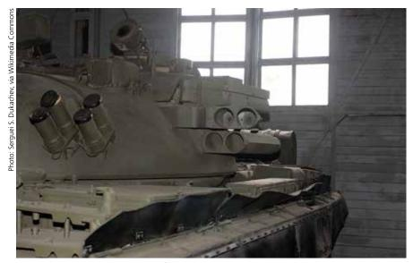
Drozd was the Red Army's first APS. It is seen here mounted on the side of this T-55AD tank, with launchers unloaded. Its use of K-band radar continued into later Soviet and Russian APSs like Arena and Afghanit.
