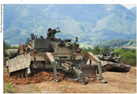
Hyundai Rotem AEV based on the K1 ARV, showing crane with bucket traversed to rear and fitted with Pearson Route Opening Mine Plough in deployed position
