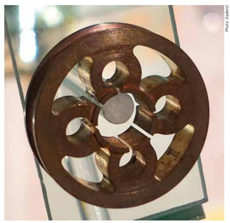
This photo of a cavity magnetron clearly shows the space in the centre for the cathode and the entrances to the cavities orbiting the hollow space between the cathode and the surrounding anode's inner wall.
