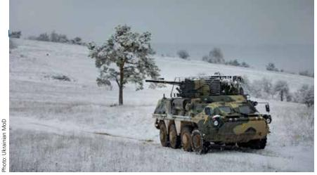
The BTR-4 is lighter than most western wheeled IFVs and has proven itself to be an effective fighting platform despite lacking the protection deemed necessary by most in Europe.
