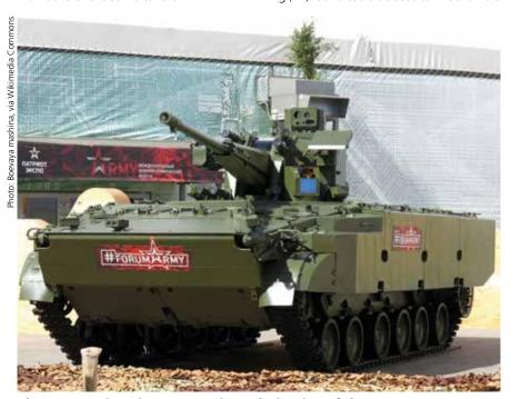
The 2538 Derivatsiya-PVO carries a derivative of the AU-220M turret, armed with a 2A91 57 mm cannon. It is designed for short-range tactical air defence although it could also provide direct fire in support of ground formations.
