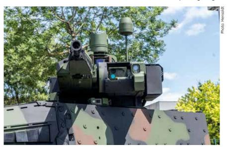
The SETAS high-resolution optronic vision system can recognise a human out to a range of 300 m, with the HMD effectively enabling the wearer to see through the vehicle to the world outside.
