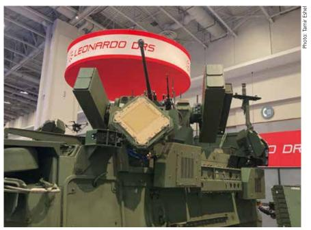
Remotely operated weapons enable interesting syntheses of weapons and systems, such as this Mobile Anti Low-Slow-Small Unmanned Aircraft Integrated Defeat Systems - MLIDS Stryker from Leonardo, mounting a 30 mm cannon, 12.7 mm machine gun, and four Coyote II counter-UAV munitions on the RWIP turret platform. This complex system is operated by three crew members
