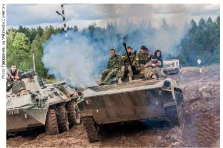
An important element of off-road mobility is the number of vehicle passes over a given piece of terrain. More passes will degrade soil strength and make travel more difficult for subsequent vehicles.
