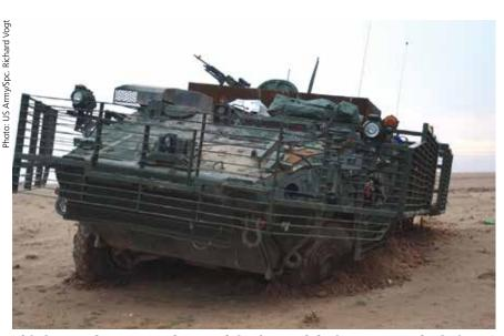
This image shows a Stryker stuck in the mud during n a patrol mission in the Anbar Province. A joint task force of US and Iraqi soldiers had to spend the night nearby to protect the vehicle, which reflects the potential vulnerabilities wheeled vehicles can create.
