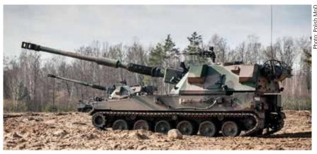
The Krab has been a noteworthy example of Polish-Korean industrial cooperation. Consisting of a K9 hull mated with the AS90 'Braveheart' turret, the vehicle is a capable SPH which has performed in Ukraine.
