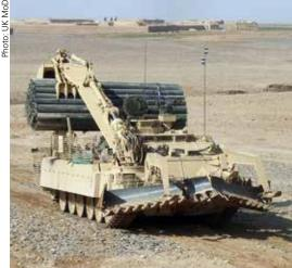
British Army Trojan breacher deployed to Afghanistan and fitted with Pearson Engineering Full Width Mine Plough in raised position and pipe fascine carried at rear
