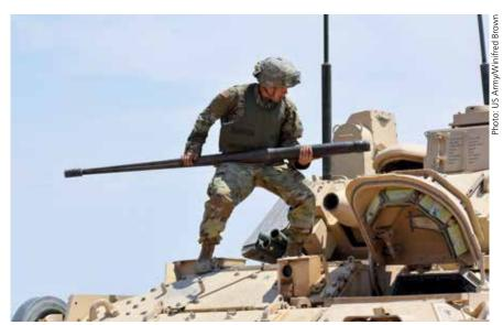
Pfc. James Ormsby, assigned to 2nd Squadron, 13th Cavalry, 3rd Armored Brigade Combat Team, 1st Armored Division, prepares to replace the barrel of a M242 Bushmaster 25 mm Chain Gun on an M2A3 Bradley Fighting Vehicle during gunnery training at the Doña Ana Range Complex, N.M..
