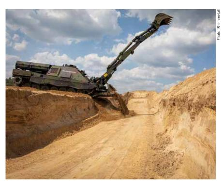
Kodiak AEV using its front mounted dozer blade to start filling in a trench and with the hydraulic arm with bucket attached extended over the front of the hull
