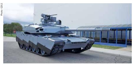
At the AUSA exhibition in Washington DC in October 2022, General Dynamics Land Systems (GDLS) displayed the Abrams X, their view of a possible series of evolutionary developments for the Abrams tank using currently available technology. The Abrams X features a hybrid propulsion system.
