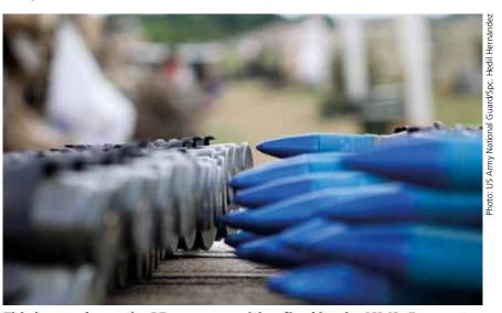
This image shows the 25 mm ammunition fired by the M242. For most of the service lives of medium calibre weapons, lethality advances have been found through innovations in ammunition design.
