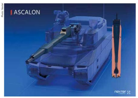
The 140 mm smoothbore ASCALON gun fires telescoped rounds 130 cm long, and is designed for scalable effects. Nexter is proposing the ASCALON as the MGCS main armament.
