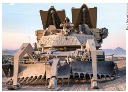
**US Assault Breacher Vehicle showing Pearson Engineering Full Width Mine** Plough lowered to the ground and rocket propelled mine clearing equipment deployed at the rear
