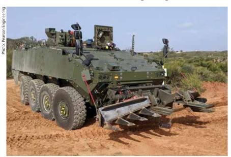
Spanish GDELS Santa-Barbara Sistema's Dragon (8x8) fitted with the Pearson Engineering Vector plough type mine clearing device on the front of the hull, in the raised position.
