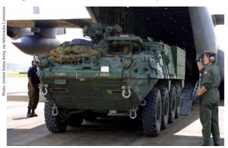
When the Stryker was selected for the US Army in the 1990s, it was expected to be air transported via C-130 to provide greater strategic mobility. However, it has often been found that in a C-130 compliant configuration the vehicles lack protection, and so must have armour removed before flight. To some, the supposed strategic benefits of 8×8s are therefore limited.
