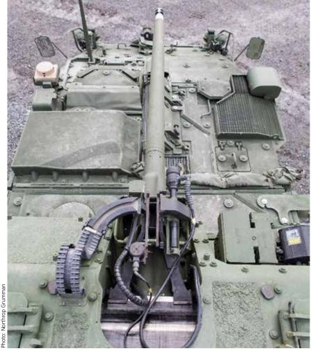
This top down image shows the Northrop Grumman XM813 fitted to a US Army Stryker Dragoon. The 30 mm cannon has been retrofitted to increase lethality of the Stryker fleet.
