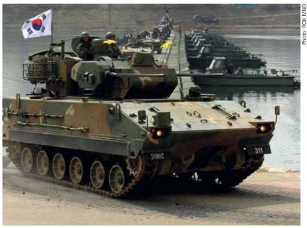
The K30 Biho was developed to provide the ROK Army with a mobile air defence gun system and is equipped with two 30 mm KKCB automatic cannons. More recently, the system's capability has been enhanced with the installation of launchers for the indigenous Shingung (also known as 'Charon') VSHORAD missile, with four missiles being carried.
