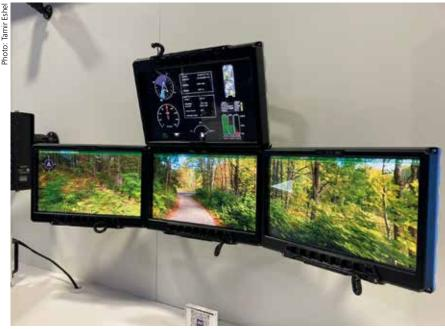
A modern crew workstation comprises multiple screens and augmented reality to provide multi-layered situational awareness combined with onboard sensor data and information from vehicles and the BMS.
