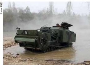
Turkish Armoured Amphibious Combat Earthmover is fully amphibious being propelled in the water by rear-mounted two water jets.
