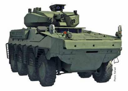
Image shows the Rafael Samson 30 mm Remote Turret with Spike and Trophy APS. The array of sensors and new weapon systems onboard latest armoured vehicles place huge demands for power on the vehicle systems.
