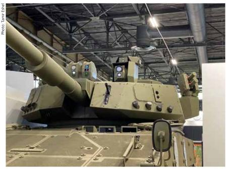
Elbit Systems mounted its Sabrah 105 mm gun turret on the ASCOD 2 tracked vehicle for the Philippines.
