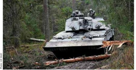
A Challenger 2 of the Queens Royal Hussars, with a dozer attachment fitted, breaks through an abatis obstacle on a training exercise in Estonia. Thought has been given to a hybrid or a full electric propulsion system as a replacement for the conventional engine system in the Challenger 2.
