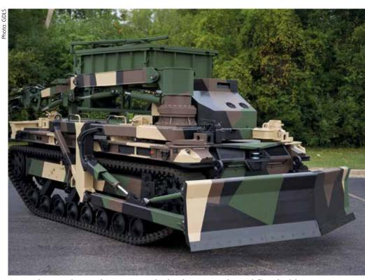
General Dynamics Land Systems Tracked Robot 10 ton (TWRX) fitted with the Pearson Engineering obstacle clearing pack which includes a front mounted V-obstacle blade
