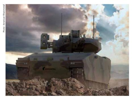
The Lynx OMFV's turret, designed by Raytheon, supports a 50 mm automatic cannon, a Multi-Mission Launcher for ATGMs and attack drones, and a next-generation array of sensors including 3rd Generation FLIR and 360° surround vision.
