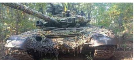
The T-90A shown here is fitted with the Shtora-1 active protection system that defends against some types of guided missiles from the frontal arc of the tank. The tanks have been used both in Ukraine, Syria, and Iraq with varying degrees of success reflecting the importance of effective tactics and employment.
