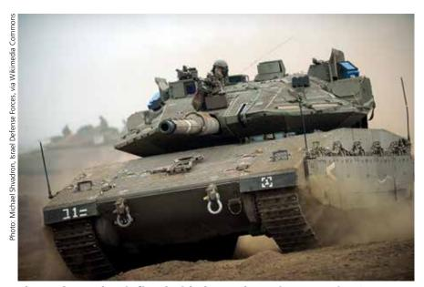
The Merkava Mk IV is fitted with the Trophy Active Protection System (APS) to provide enhanced protection from against RPGs and ATGMs.
