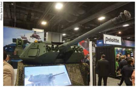
Elbit Systems has developed this turret mounting the new XM913 50 mm automatic cannon for US Army testing under the OMFV program.
