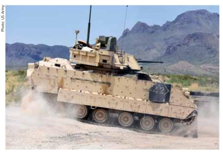
The M2 Bradley is armed with a 25 mm automatic cannon, two TOW ATGM, and a 7.62mm MG.
