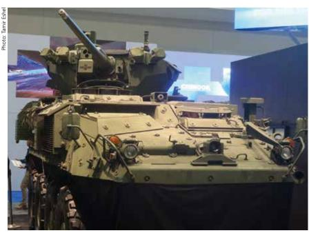
The Medium-Calibre Weapon System (MCWS) unmanned turret was developed by Rafael based on the Samson design. It was adapted specifically for Stryker.
