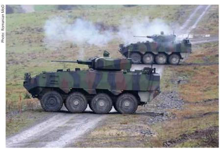
The Piranha V is shown here in its IFV configuration for Romania. The turret and armour used to make the vehicle an IFV add significantly to its weight. However, it is ultimately the vehicle's use case and the way that it is employed that will shape how effective it is.
