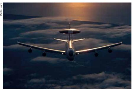
NATO's E-3A AWACS aircraft is a modified Boeing 707/320 commercial airframe with a distinctive rotating radome equipped with long-range radar and passive sensors capable of detecting air and surface contacts at long range.
