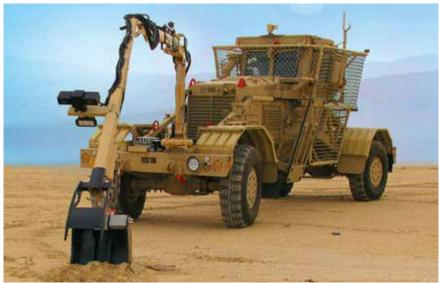
The two-operator Husky 2G clearance vehicle was born from an operational requirement for longer, more complex, mounted clearance missions and employment of more sophisticated vehicle payloads.
