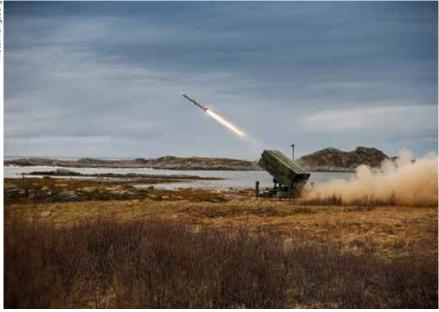
Currently in service with Oman, Raytheon's National Advanced Surfaceto-Air Missile System (NASAMS) is seen here launching an AIM-120 Advanced Medium Range Air-to-Air Missile (AMRAAM), but the system is known to be compatible with the AMRAAM-Extended Range missile and the AIM-9X Sidewinder.
