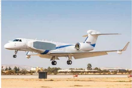
Unveiled by the Israeli Air Force officially in April 2021, the multi-mission Nachshon Oron G-550 based platform is reported to be capable to conduct surveillance and intelligence operations in support of ground and naval forces and act as flying relay platform.
