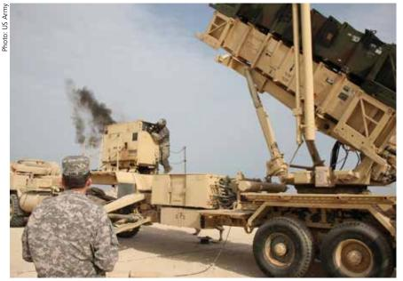
The technology of the newer variants of PATRIOT may be state-of-theart, but the overall system has some conventional 'low-tech' components. The diesel-powered electrical generator of this Bahrain-based Patriot unit emits dense smoke as it is started up.
