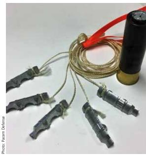
The ALS12SKY-Mi5 is a 12 gauge anti-drone round designed to be rapidly deployed against commercially available drones. Upon firing, the five tethered segments separate with centrifugal force and create a 1.5 m wide 'capture net' to effectively trap the drone's propellers causing it to fail.
