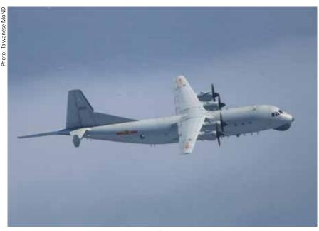
The Y-9 is available in multiple configurations. The pictured Y-9Q variant in service with the PLAN is configured for anti-submarine warfare, with a notably long tail boom housing a magnetic anomaly detector.
