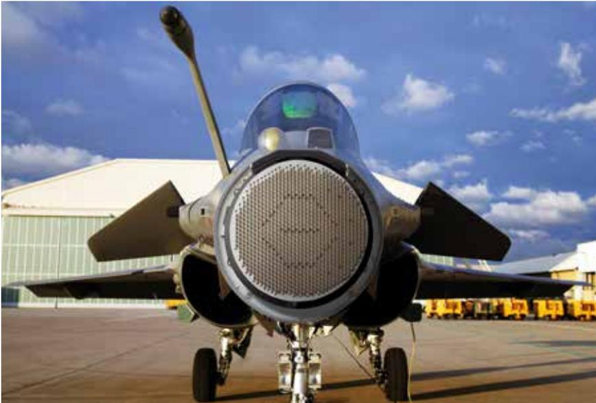
**The multitude of individual transmit/receive modules are clearly seen on the antenna of this Thales RBE2 AESA radar equipping a Dassault Rafale combat aircraft.**
