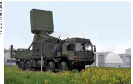
TRML-4D uses Active Electronically Scanned Array (AESA) radar technology with multiple digitally shaped beams. According to the company, it is capable of detecting, tracking and classifying various types of aerial targets, with a focus on small, fast and low-flying and/or manoeuvring cruise missiles and aircraft, as well as helicopters. It ensures the rapid detection and tracking of about 1,500 targets in a radius of up to 250 km.
