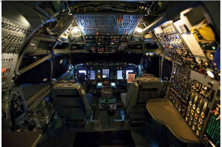
**Boeing's 2018 cockpit and avionics upgrades of NATO's AWACS aircraft, included five full-colour displays providing crew with customisable engine, navigation and weather data.**
