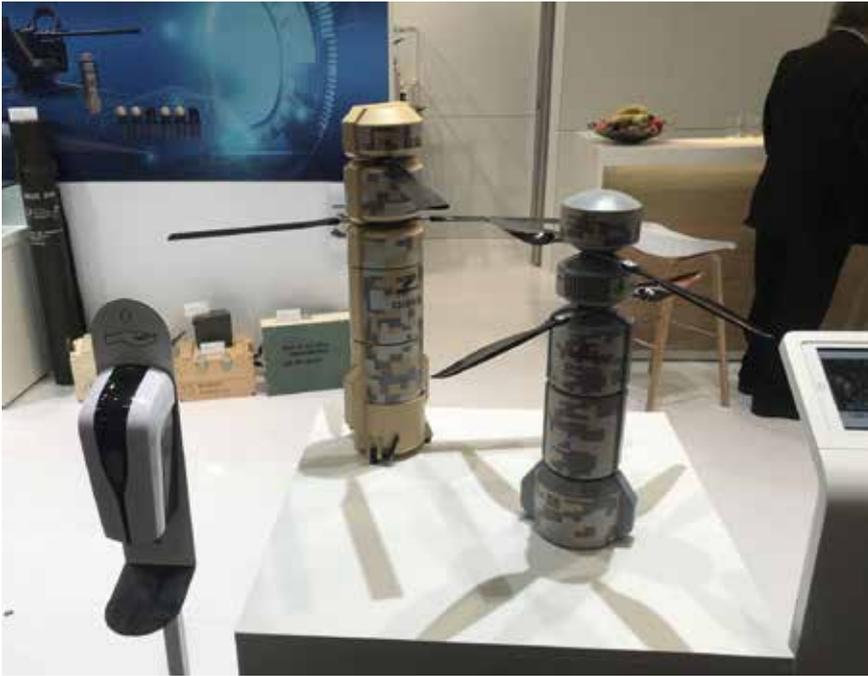
**The Libelle Loitering Munition is available in two variants (pictured), the one on the left is intended for use with vehicles, while the one on the right is intended for dismounted operation.**
