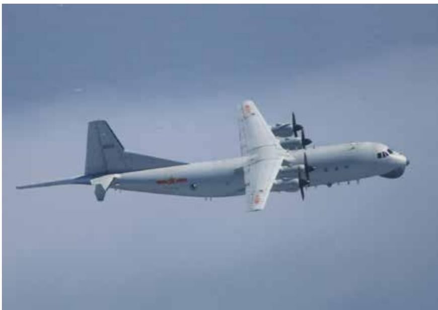
**The Y-9 is available in multiple configurations. The pictured Y-9Q variant in service with the PLAN is configured for anti-submarine warfare, with a notably long tail boom housing a magnetic anomaly detector.**
