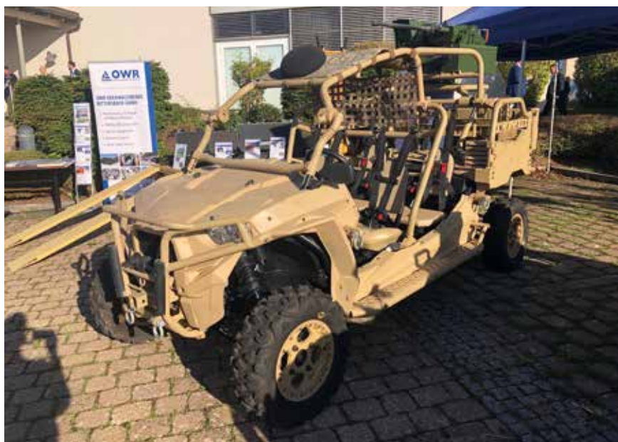
Polaris MRZR D4, shown fitted with an acoustic gunshot detection system on the roof and RWS on the rear.
