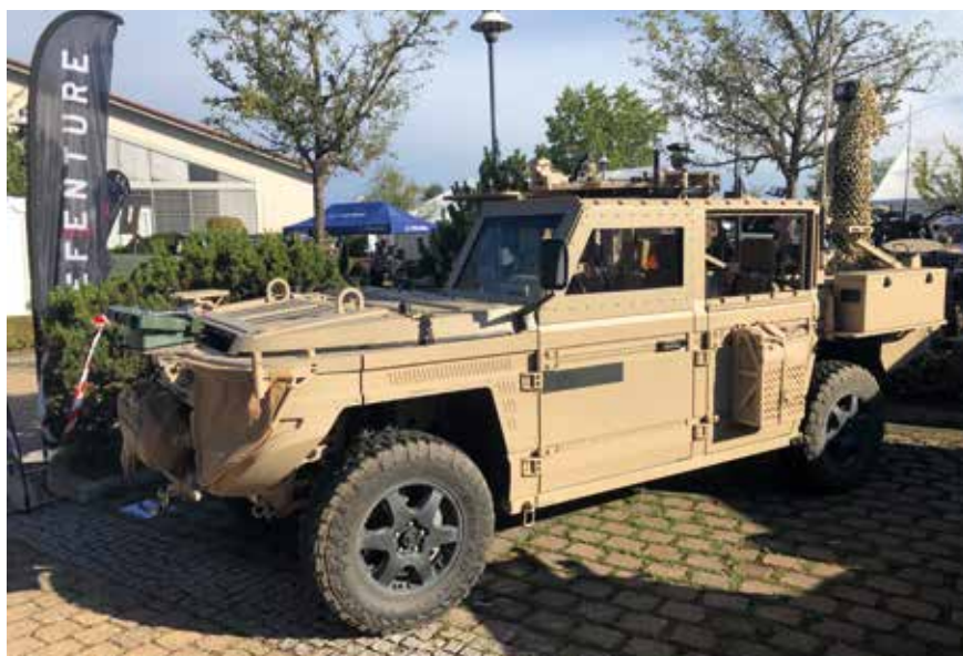
Defecture GRF 4x4, shown with a Rheinmetall ROSY smoke launcher on the front and Optronic mast on the rear.
