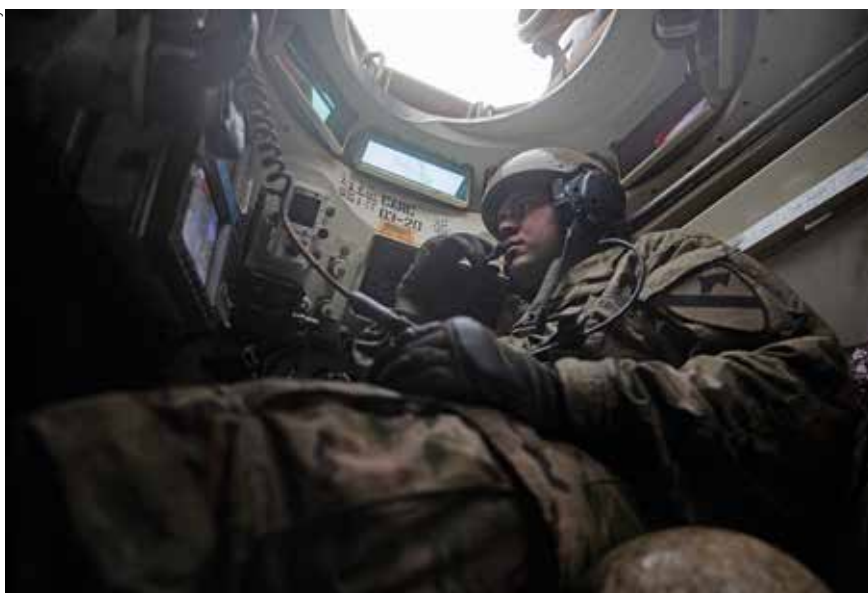
The commander and crew of the M1A2 obtain a situational picture from multiple screens feeding sight, sensor, and BMS information in a graphical and visual display.
