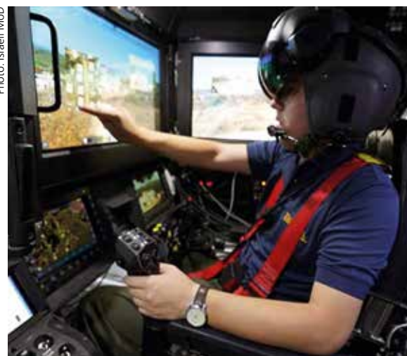
Israel's project Carmel demonstrated innovative operations of armoured fighting vehicles by two crewmembers, using large digital screens and helmet-mounted displays.
