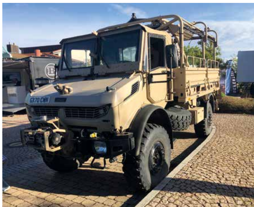
The Jankel Light Tactical Transport Vehicle (LTTV) is based on the Mercedes-Benz UNIMOG design.
