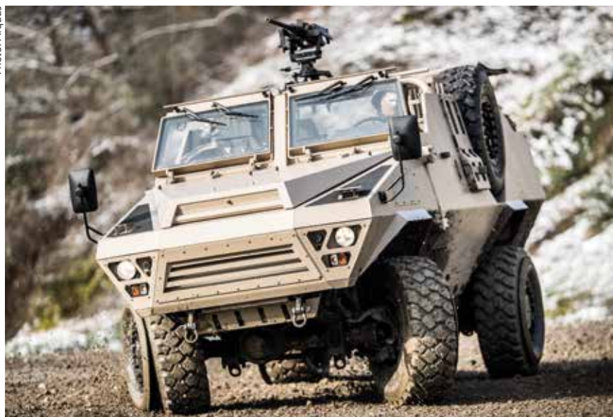
Arquus Patsas 4x4, shown here with a ring mount fitted with a 12.7 mm HMG.
