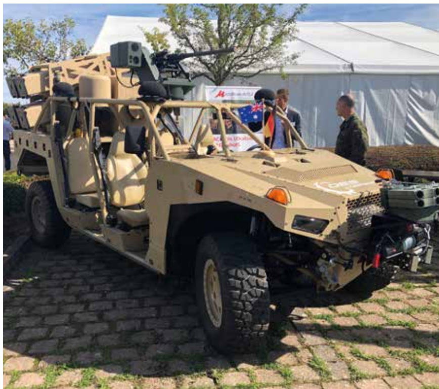
The DAGOR 4x4, shown here with an RWS and a four-round launcher for Spike NLOS ATGMs.
