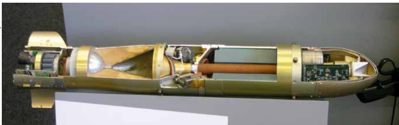
Displayed at defence exhibitions by Yugoimport, this cutaway of the Bugar missile shows a close resemblance to the internal layout of the MBDA Eryx.
