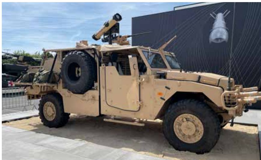
The SF's vehicles are less-armoured but faster than those of the conventional forces, reaching a balance between protection and speed. Here is the Sherpa Light Special Forces Variant.
