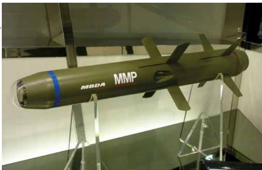
MBDA's Akeron MP (formerly Missile Moyenne Portée (MMP)) combines visual and IR seekers with a fibre-optic datalink.
