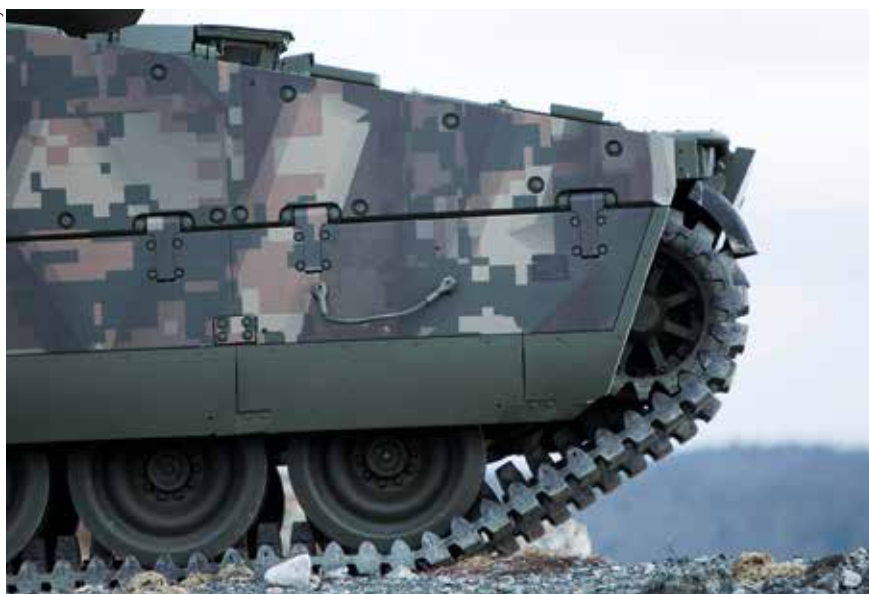
Weight reduction just one among many of the benefits CRTs bring to the table when compared to conventional steel tracks.
