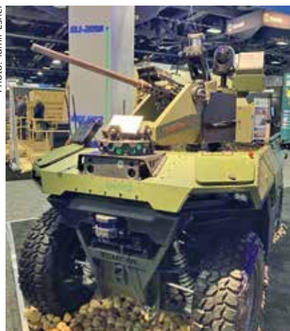
REX MK2 loaded with sensors and weapon station for autonomous border security patrols.
