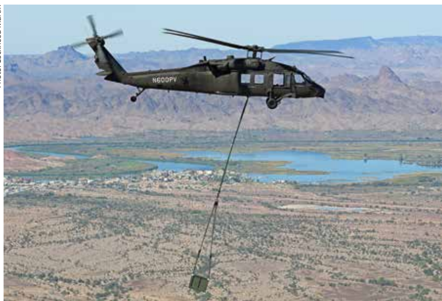
During the Project Convergence 22 experiment in October 2022, a specially configured UH-60M Black Hawk helicopter performed unmanned flight manoeuvres including autonomous resupply missions.
