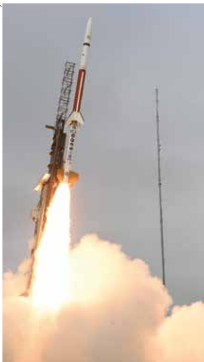
The Navy employs sounding rockets carrying experimental payloads in support of the hypersonic weapons programme. The experiments provide data on the performance of materials and systems in a realistic hypersonic environment.
