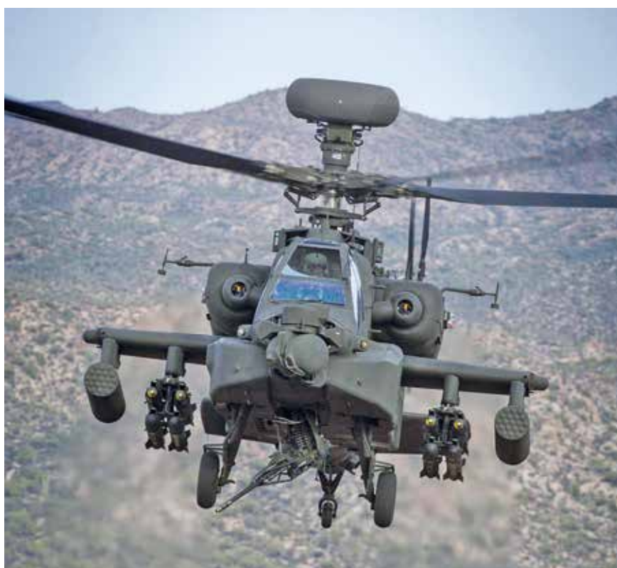
A US Army AH-64E Guardian with the distinctive AN/APG-78 Longbow fire control radar above the rotor blades.
