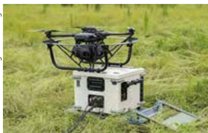
A tethered drone equipped with the MicroKestrel WAMI payload.
