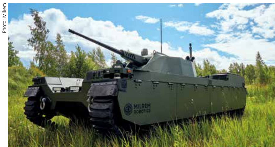
Milrem's Type-X demonstrates the degree to which UGVs can be made smaller and lighter than manned vehicles while retaining solid firepower.
