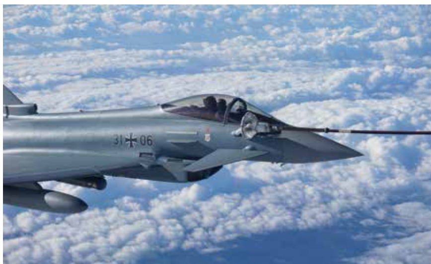
A single-seat Eurofighter Typhoon (31+06) following successful coupling with the MRTT's drogue refuelling system.
