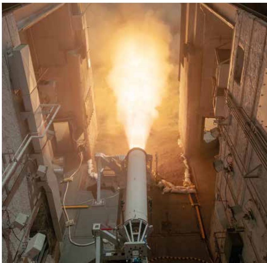
May 2021 live-fire ground test of the CPS' first stage solid rocket motor, which was developed by Northrop Grumman.
