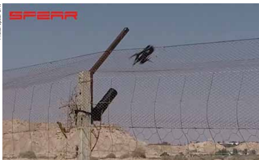
An unattended launcher deploys a Ninox micro-drone from a smart fence installation.
