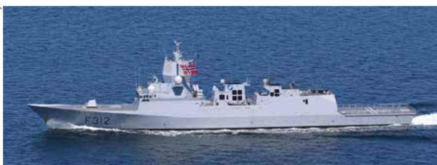
Otto Sverdrup is one of Norway's Fridtjof Nansen class frigates, the smallest and lightest class of Aegis-armed ships. It mounts a scaled-down SPY-1 radar and only eight vertical launch cells.
