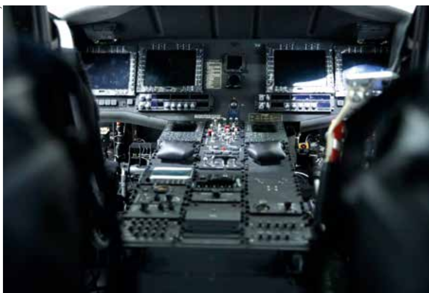
Both the UH-60M and UH-60V feature a digital or 'glass' cockpit layout.
