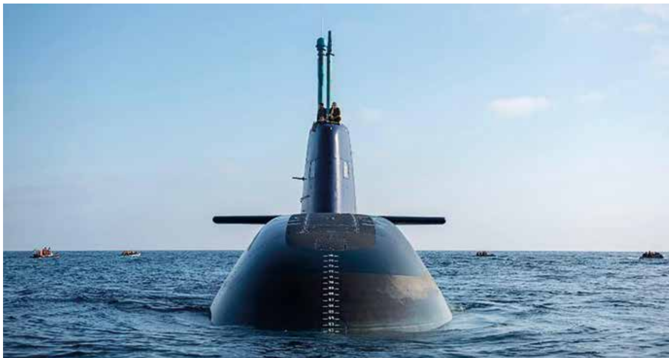
The Dolphin-II series of submarines is equipped with air-independent propulsion, bringing an important new capability to Israel's undersea fleet.
