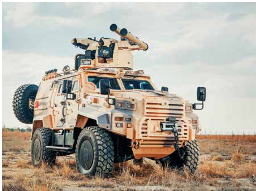
The pictured configuration of the Ejder Yalçın possesses a good mix of anti-personnel and anti-armour capabilities, armed with an HMG, a GPMG, and two ATGMs. The vehicle is also provided with an armoured engine bay to preserve mobility when hit, and thereby increase survivability in various tactical scenarios.
