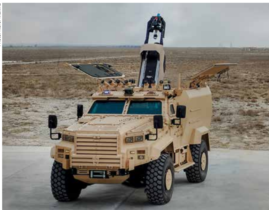
High-angle view of the Ejder Yalçın mortar configuration, showing the Alkar mortar's semi-automatic muzzle loading mechanism.
