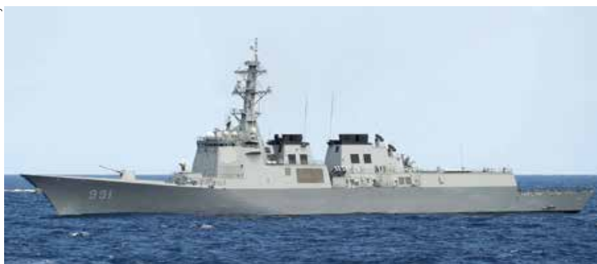
South Korea's Sejong the Great was the lead ship of the largest and heaviest type of Aegis cruiser, and is sized to accommodate 80 vertical-launch cells for the Standard Missile family.
