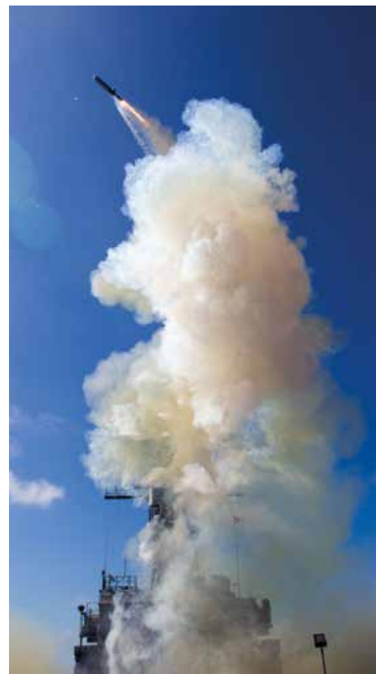
A VLS-launched LRASM is test-fired from a surface ship. Deck-mounted launchers can also be used to provide surface ship strike capacity.
