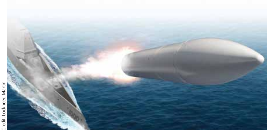
Artist concept of a CPS launch from a surface warship. The image shows a notional configuration in which only one 155 mm gun turret has been replaced, while in fact both turrets will be removed.
