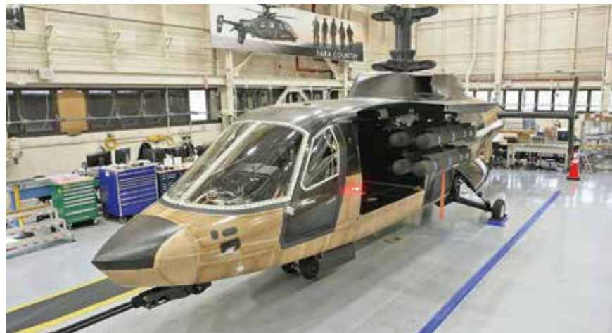
The RaiderX prototype under construction. Mock-up weapons are "deployed" from the internal weapons bay.
