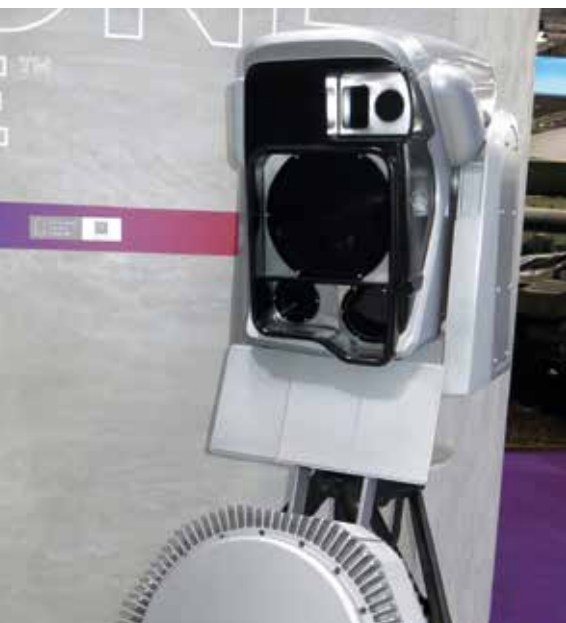
Rafael is developing the LITE BEAM, a 7.5 kW laser effector to defeat small drones.
