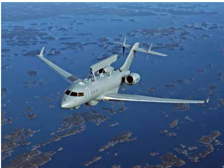
GlobalEye airborne early warning & control (AEW&C) Aircraft, equipped with SAAB's Erieye Extended Range (ER) Radar.
