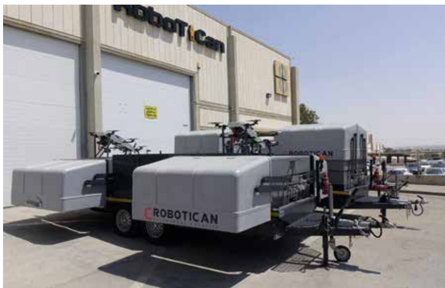
Goshawk, developed by Robotican, autonomously intercepts drones by swiping the rogue drone with an arresting net.
