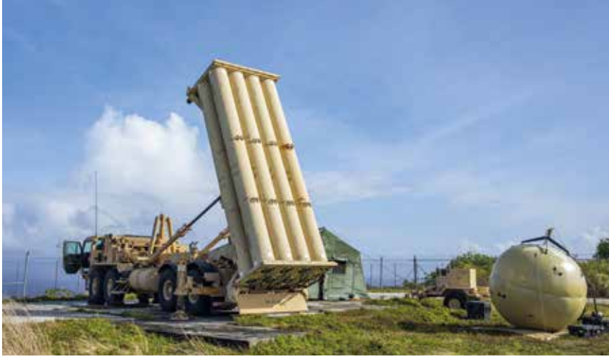
A THAAD launcher and a globe-shaped Transportable Tactical Command Communications (T2C2) node on the island of Rota, Mariana Islands. The T2C2 node serves as the portable interface between the centralised fire control unit and dispersed THAAD launchers.
