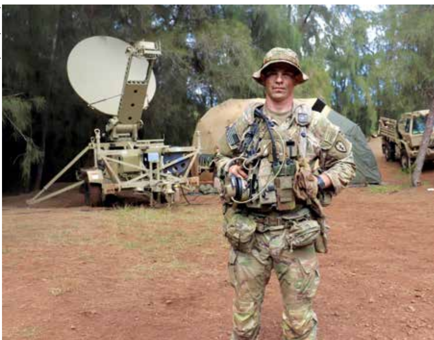
A platoon leader wearing the Integrated Tactical Network (ITN) dismounted kit at Kahuku Training Area, Hawaii, which includes two-channel AN/PRC-163 leader radios, a single-channel shadow radio and the ATAK end-user situational awareness device.
