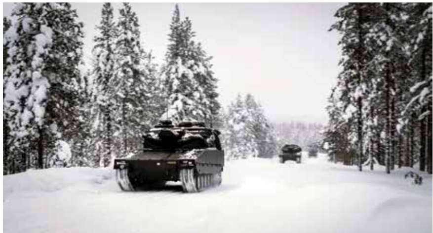
Sweden's CV90-based Granatkastarpansarbandvagn 90 (Grkpbv 90), armed with two muzzle-loaded 120 mm Mortars.
