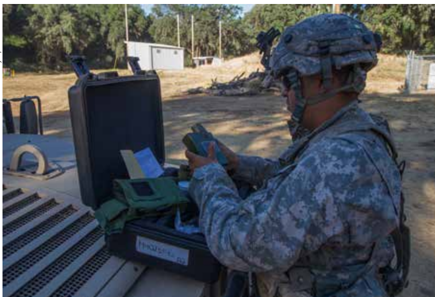
The M4 JCAD, also known as the LCD outside the USA, is a widely used ion mobility chemical warfare detector.
