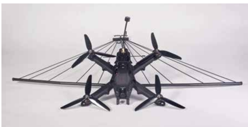
The Griffon system developed by Xtend uses a detachable arresting apparatus to intercept and disable rogue drones
