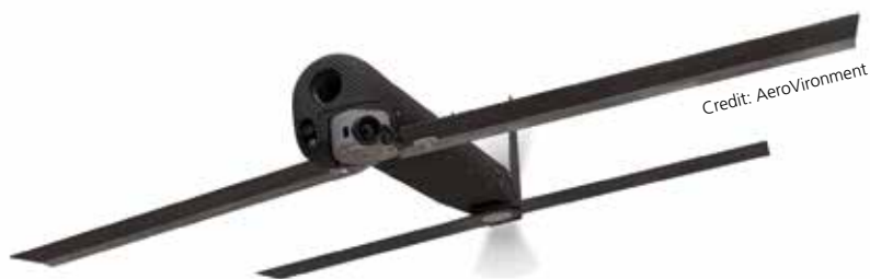
SWITCHBLADE 300 BLOCK 20 has a new panning camera suite enabling direct cueing while circling.
