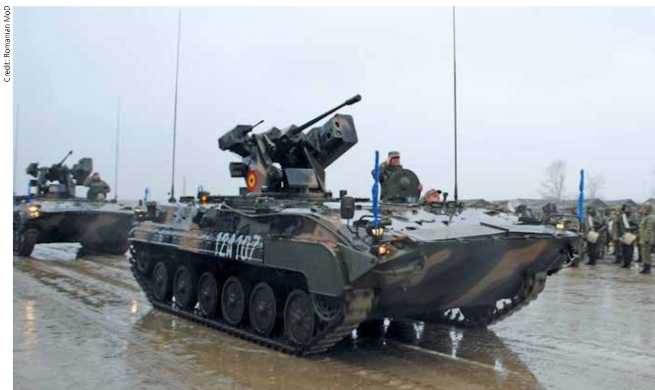
The Romanian MLI-84M IFV is an indigenous development of the BMP-1, this modernised variant is equipped with an OWS mounting a 25 mm cannon and anti-tank missiles. There is interest in the acquisition of a new IFV to replace the MLI-84.
