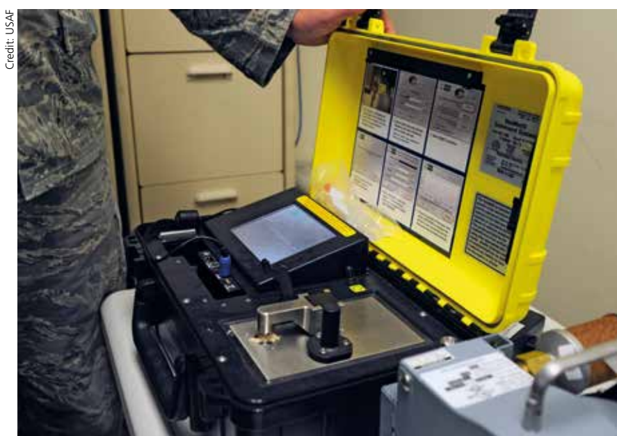
FTIR devices like the Smiths Detection HazmatID can help identify unknown solids and liquids.
