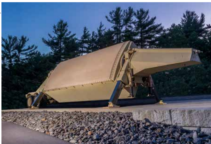
The Raytheon AN/TPY-2 radar detects, classifies and tracks ballistic missiles and can guide interceptors to descending warheads.
