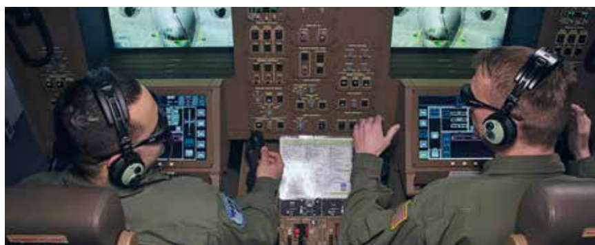
Personnel at the Aerial Refueler Operating Station (AROS) need special stereoscopic glasses to view the 3D images on their displays.
