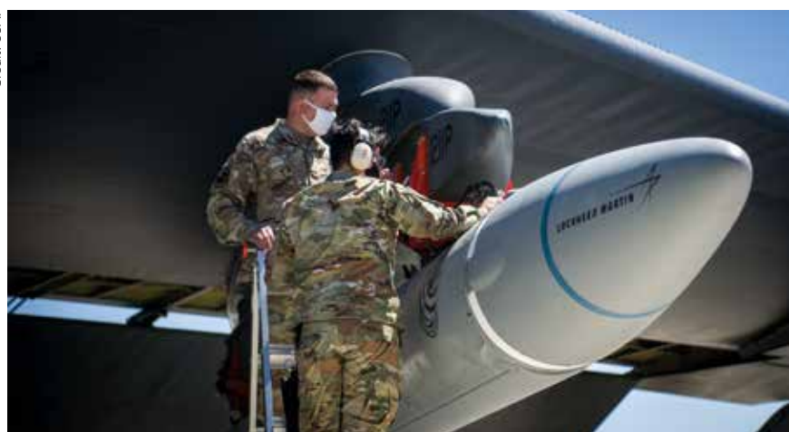
Airmen ready an AGM-183A for a 2020 captive carry test beneath the wing of a B-52 bomber.
