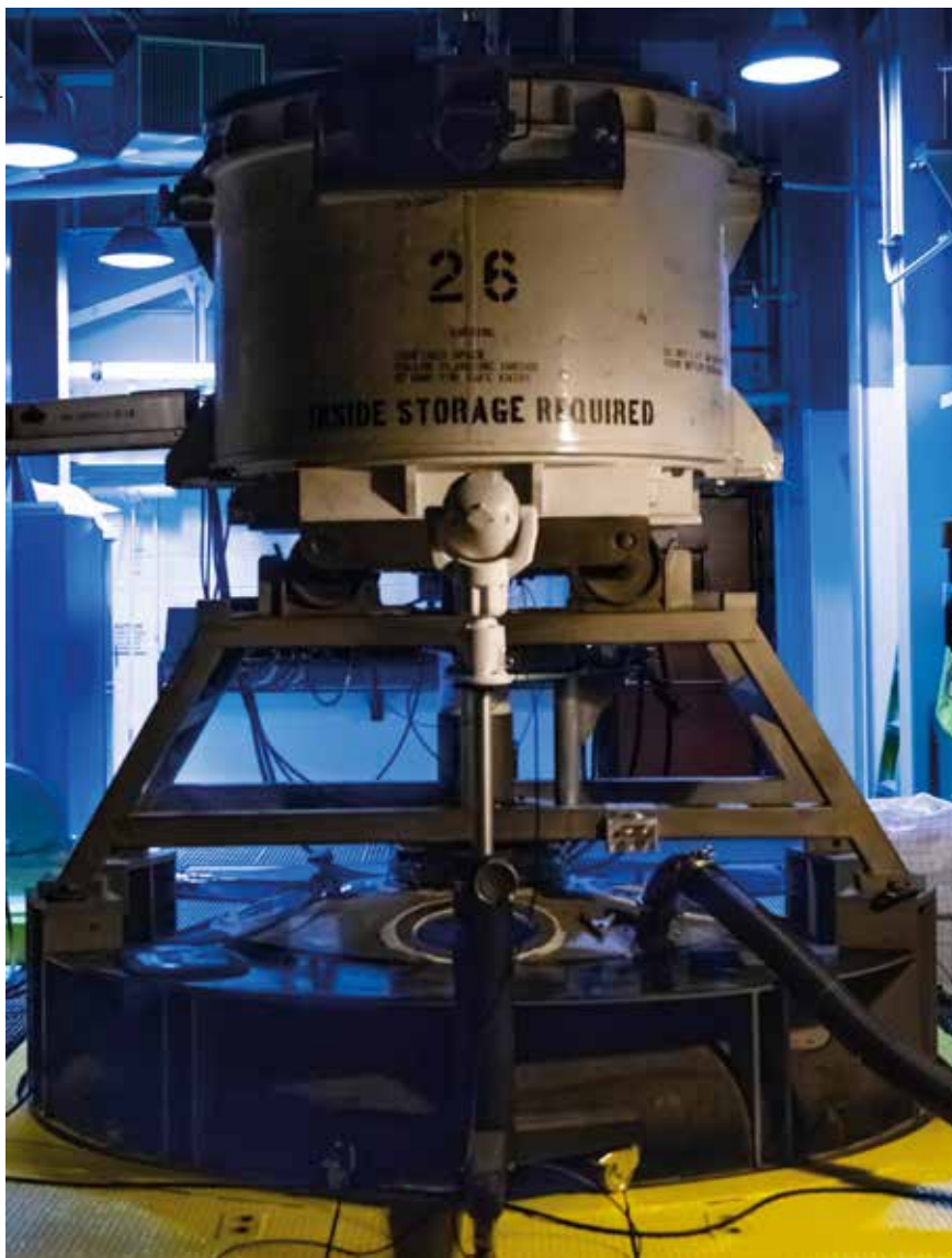
Sentinel solid rocket motor casting is a complex process of pouring rocket motor propellant into motor cases.
