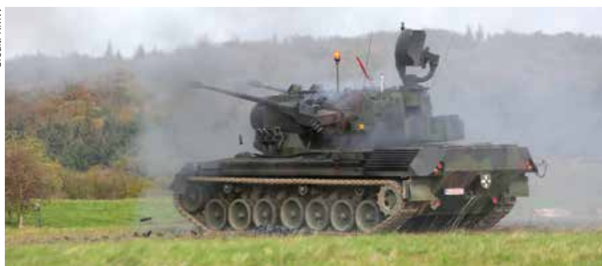
The Flakpanzer Gepard SPAAG has been a more cost-effective point defence system compared to SAMs, when it comes to for engaging low-cost targets such as Shahed-136 loitering munitions.
