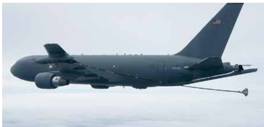
A KC-46A deploying the hose and drogue basket from one underwing refuelling pod.
