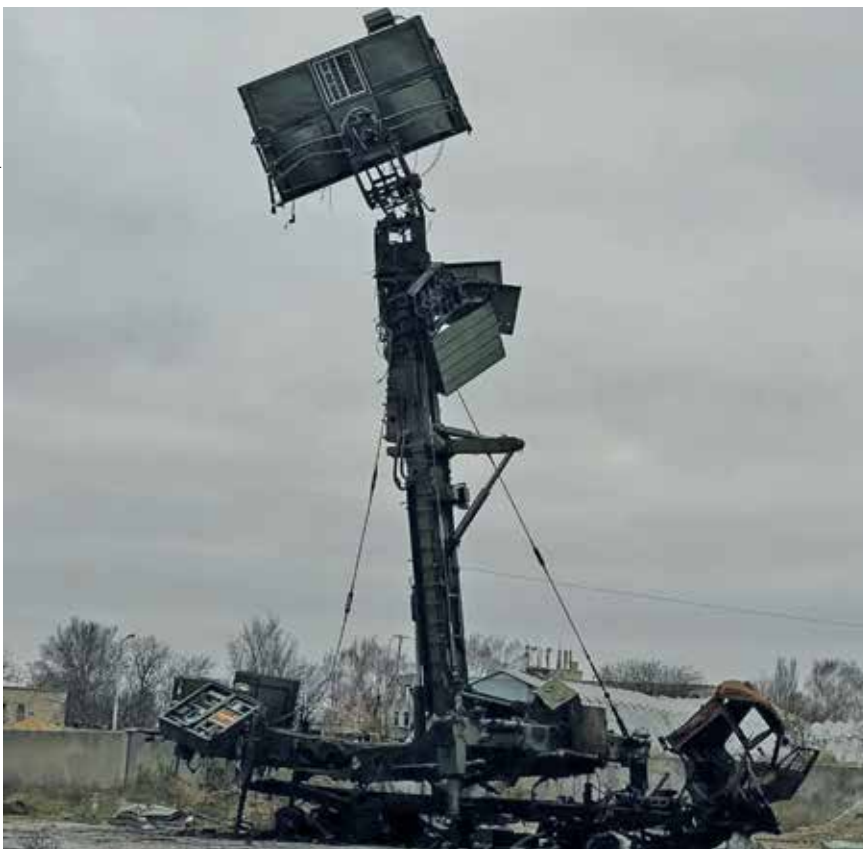
Image shows a damaged Russian Army 48Ya6-K1 Podlet-K1 ground-based air surveillance radar. The offensive counter-air battle involves suppression/destruction of enemy air defence attacks against hostile radar. As well as using kinetic effects, these threats can be attacked electronically and cybernetically.
