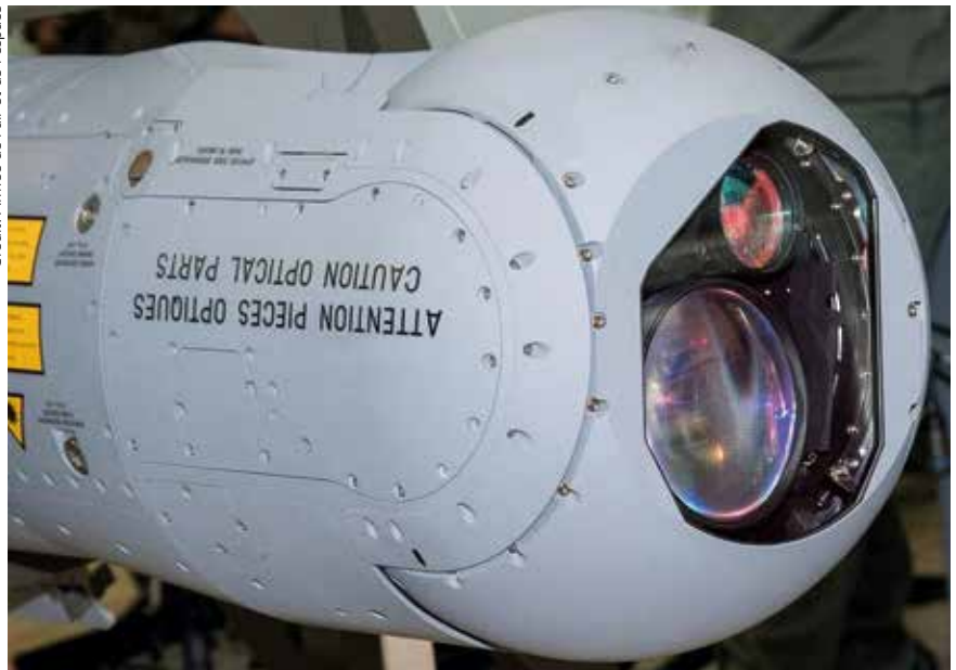
Close up of the TALIOS pod gimbal head housing the sensor suite.
