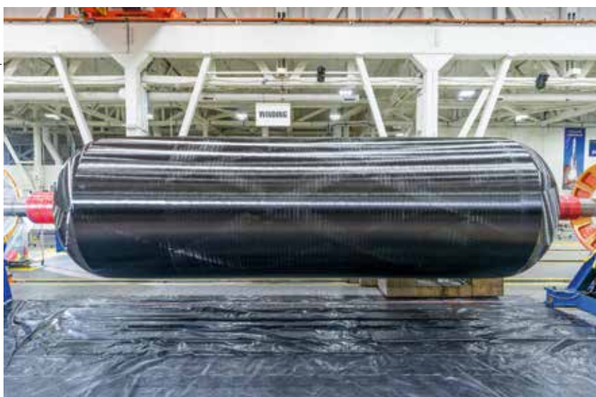
Northrop Grumman performs the case wind process for the first-stage solid rocket motor, applying composite material to form the outer shell of the motor.
