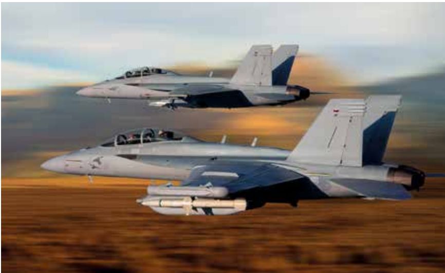
A US Navy E/A-18G Growler electronic warfare aircraft is seen here in the foreground of this picture carrying an AN/ALQ-99 jamming pod on one of its under-wing hardpoints behind an AGM-88 missile. The AN/ALQ-99 will eventually be replaced by the NGJ variants.
