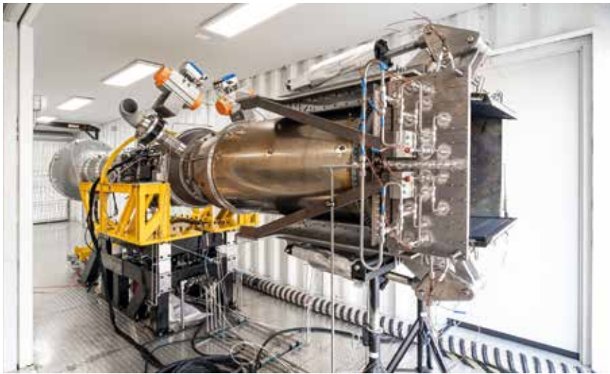
The Chimera TBCC demonstrated transition from turbojet to ramjet propulsion mode in November 2022 in a testbed simulating high-Mach temperatures and pressures.
