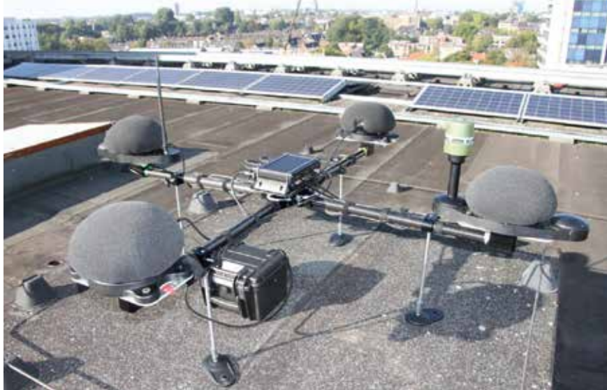
Acoustic sensors, such as Microflown AVISA's Castle sensor package are capable of detecting targets even without a direct line-of-sight.
