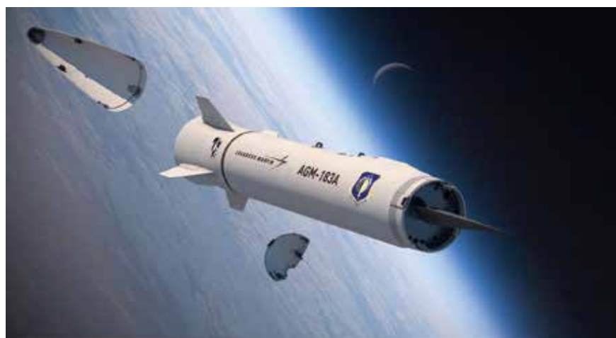
The protective nose cone separates from the ARRW to reveal the warhead in this concept image.
