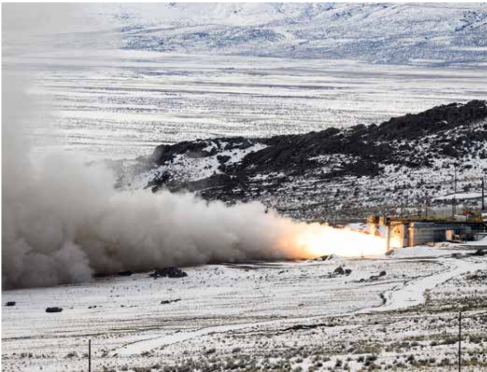
Air Force and Northrop Grumman Corporation conduct first full-scale static test fire of the Sentinel stage-one solid rocket motor.
