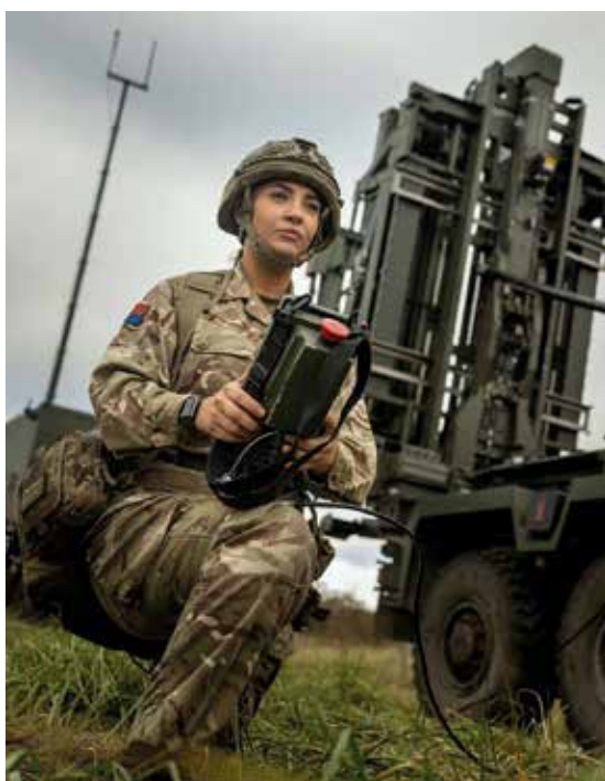
Soldier belonging to the 16th Regiment, T deploying the Agile Multi-Beam surveillance radar of the new Sky Sabre Air defence missile system.
