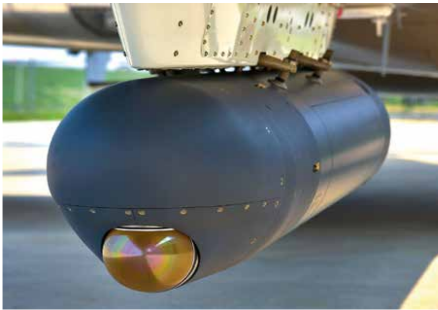
Front View Of Northrop Grumman's Openpod.
