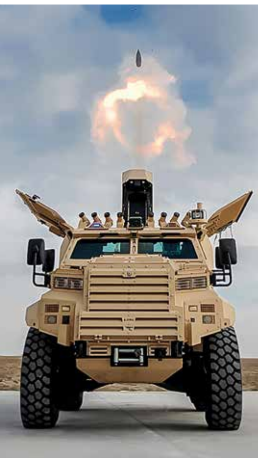
The Ejder Yalçın mortar configuration (Havan), conducts a test firing with its on-board semi-automatically loaded Aselsan Alkar 120 mm mortar.
