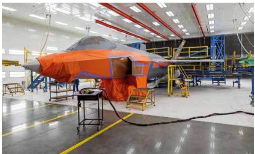
TUSAS utilises robotic painting stations for painting the Kaan's fuselage and components. This was established with an investment of approximately USD 25 M, and uses locally-produced special paint.
