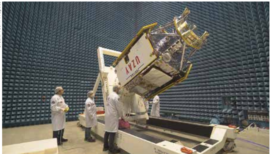
Imece undergoes testing in an anechoic chamber.
