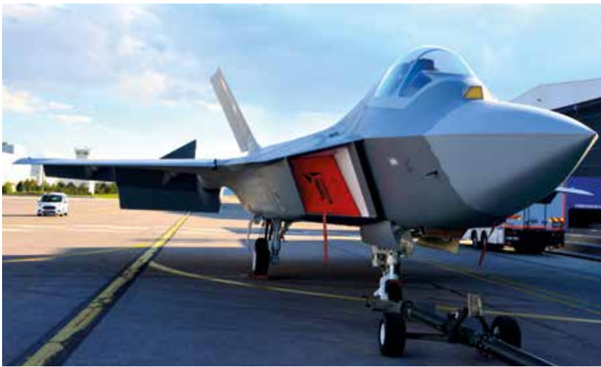
Prototypes and initial batches of Kaan are to be powered by a pair of F110-GE-129E turbofan engines.
