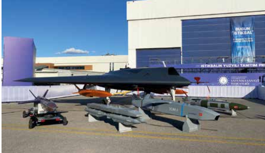
Using a stealthy flying wing design, the Anka-III is a high-altitude, long-range and high-speed UAV, long-range reconnaissance and strike missions in hostile environments
