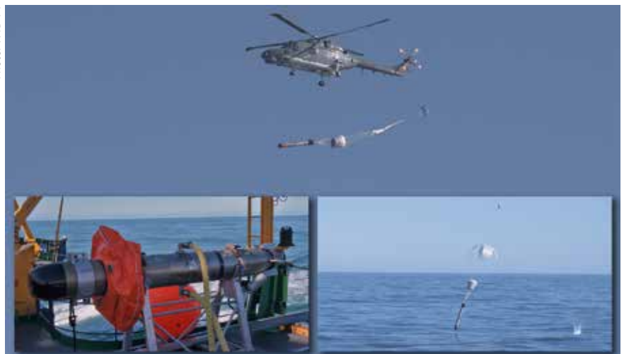
The new parachute drops the torpedo safely into the water.
