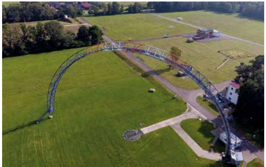
Vehicles can be measured from different angles using the sensor training system.
