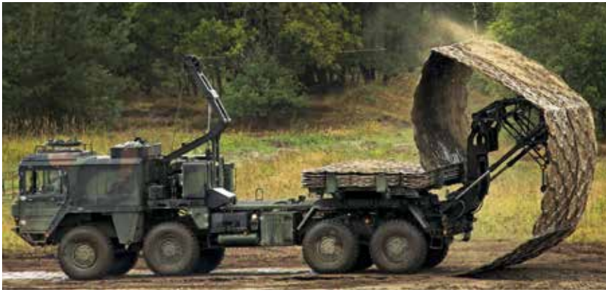
Road layer from KMW, using a folding road made from hexagonal aluminium plates
