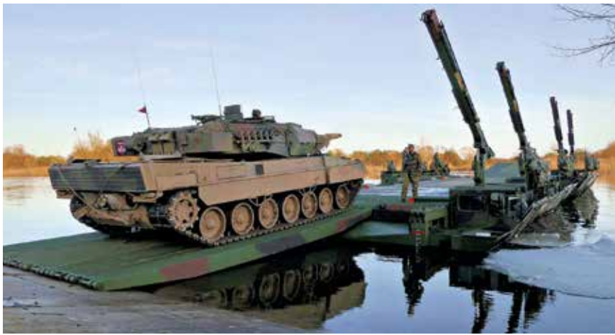
The M3 amphibious bridge, due to be replaced in future by the 'Schnellschwimmbrücke 2' bridging system.
