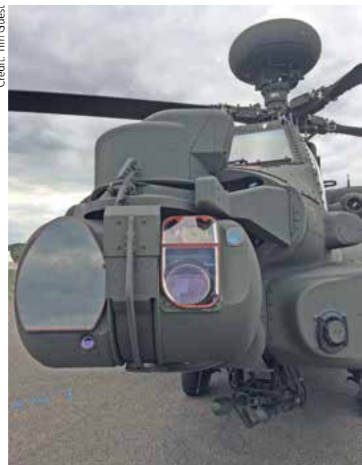
AH-64E at DVD 2022 latest optical and FLIR sensors.
