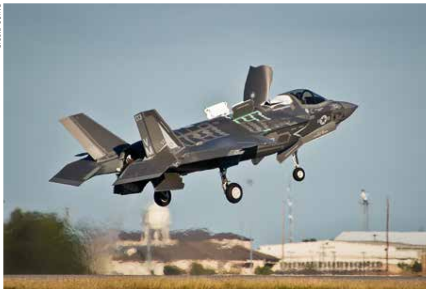
The aft-mounted swivel duct and the forward mounted lift fan provide vertical thrust for the F-35B.
