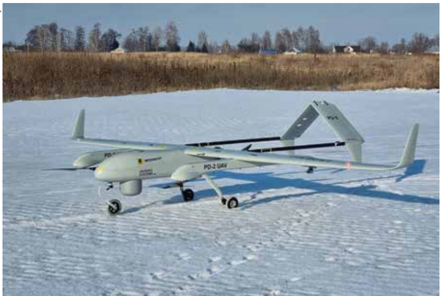
The PD-2 VTOL UAV fitted with Infozahyst's ELINT package forms the aerial component of the Gekata system.
