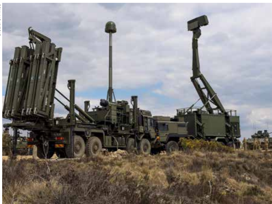
Prior to being ready for engagement, Sky Sabre's components need to set up for operation, lowering their stabilisers and raising radar or communications masts, as well as elevating the launch assembly to the vertical launch position.
