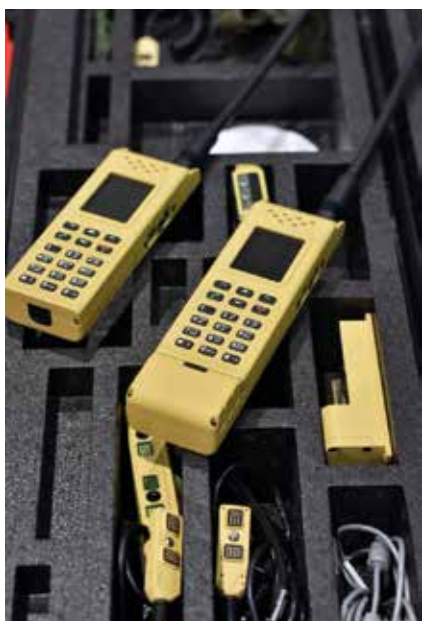
The R-187P1 handheld variant of the Azart family, shown here fitted with the AB standard-capacity battery (left) and the larger AB-12 expanded-capacity battery (right).
