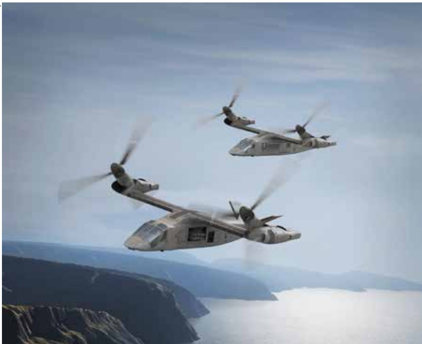
The Bell V-280s depicted in this concept image have more than twice the speed and range of current helicopter platforms. The image shows the FLRAA in the background, escorted by a notional tiltrotor configured Future Attack and Reconnaissance Aircraft.
