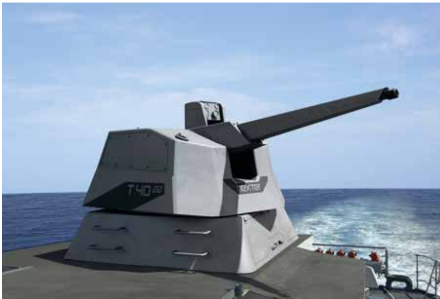
The T40 RapidFire developed by Nexter and Thales is equipped with the CTA International 40 mm CT40 automatic cannon, firing case telescoped ammunition.
