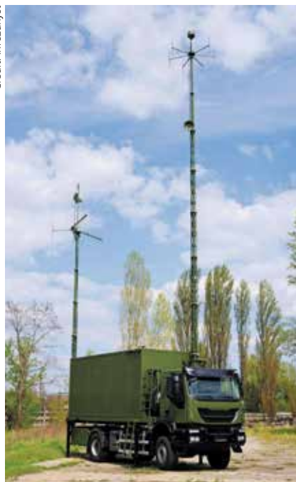
The Khortytsia-M mobile COMINT/Direction Finder system shown with its two telescopic masts extended, ready for operation. The system can be used either standalone or as part of a COMINT network, as a node or managing other systems subordinated to it.
