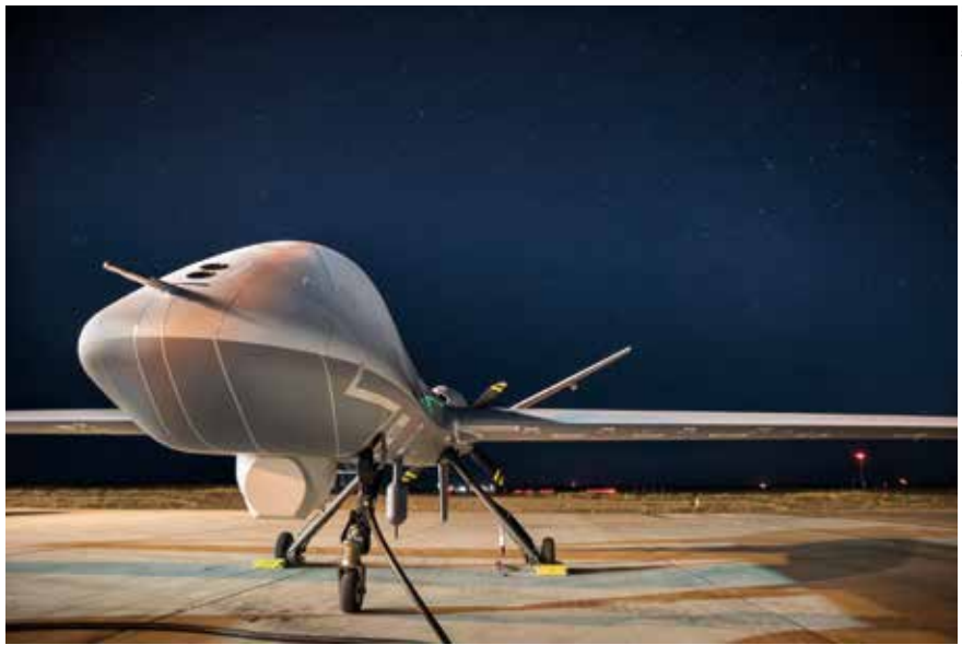
Front view of the Protector with the optical sensor gimbal mount clearly visible.
