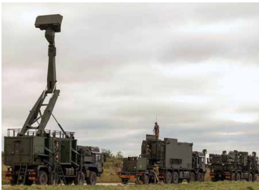
The image shows the key combat components of a Sky Sabre battery, comprising the Giraffe AMB radar (left), SAMOC (middle), and TEL (right).
