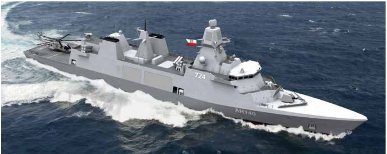
A computer generated graphic of the Polish Arrowhead 140-based Miecznik frigate. The design, which has evolved since this image was released in 2022, has similarities with the British Type 31 frigate but is equipped with a more comprehensive outfit of weapons and sensors in line with the Polish Navy's requirements.
