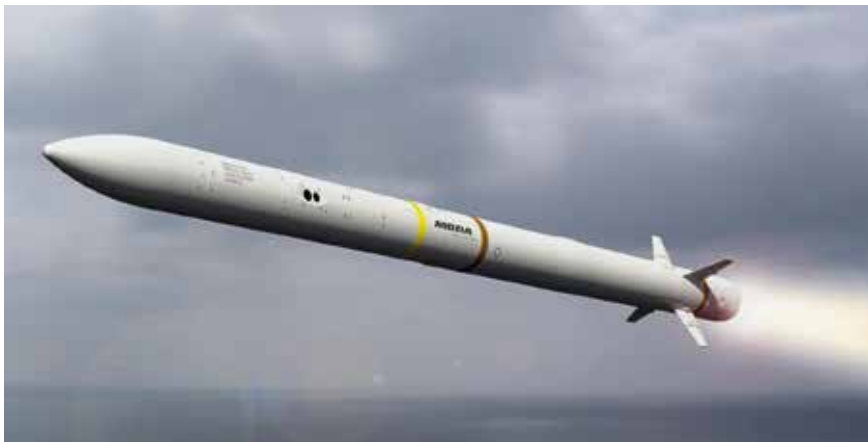
A closeup of the CAMM, showing the key external features of the missile. The optical windows for the laser proximity fuze are visible forward of the warhead section.
