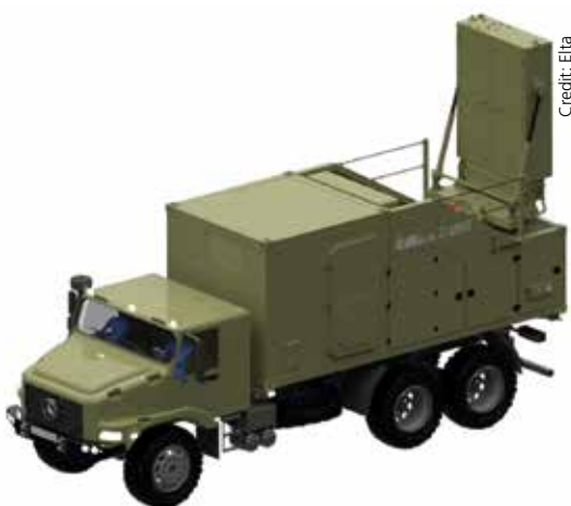
The ELM-2133 C-MMR is carried and containerised on a single vehicle with just two operators/crew. It has advanced ECCM and signal processing capabilities, enabling it to handle a variety of targets and environmental conditions.
