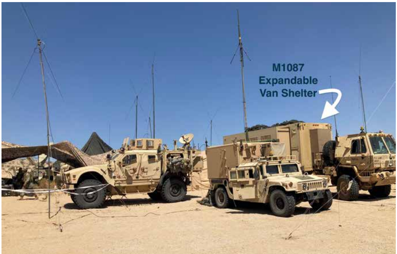
An Armoured Brigade Combat Team (ABCT) Tactical Operations Centre operates at the National Training Centre, Fort Irwin, California, in September 2022. ABCTs now have M1087 Expandable Van Shelters, known as 'Expando-Vans', to use for CPs. These vans are easier to set up than tents but offer no significant protection.
