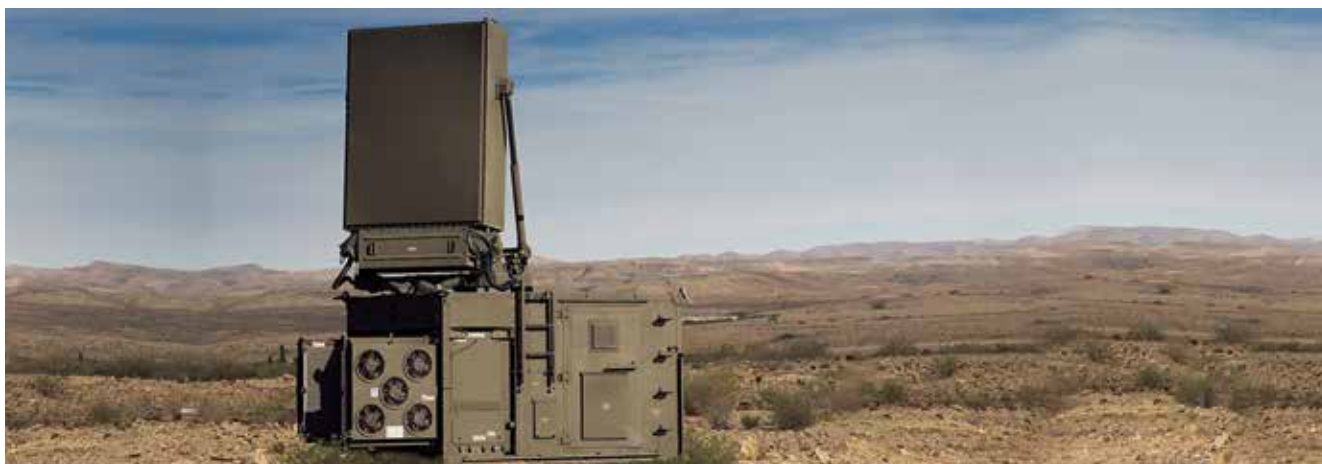
SERPENS has settled for the vehicle-mounted ELM-2133 C-MMR from IAI-Elta, an active electronically scanned array system.
