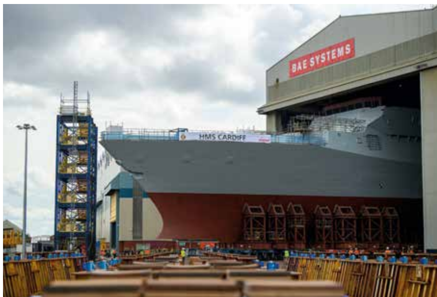
The bow section of the second Type 26 HMS Cardiff is rolled out of the shipbuilding hall at BAE Systems' Govan shipyard, prior to being joined with the stern section on Govan's hardstanding. In future, all ships-in-class will be assembled undercover, in a new shipbuilding hall currently under construction.
