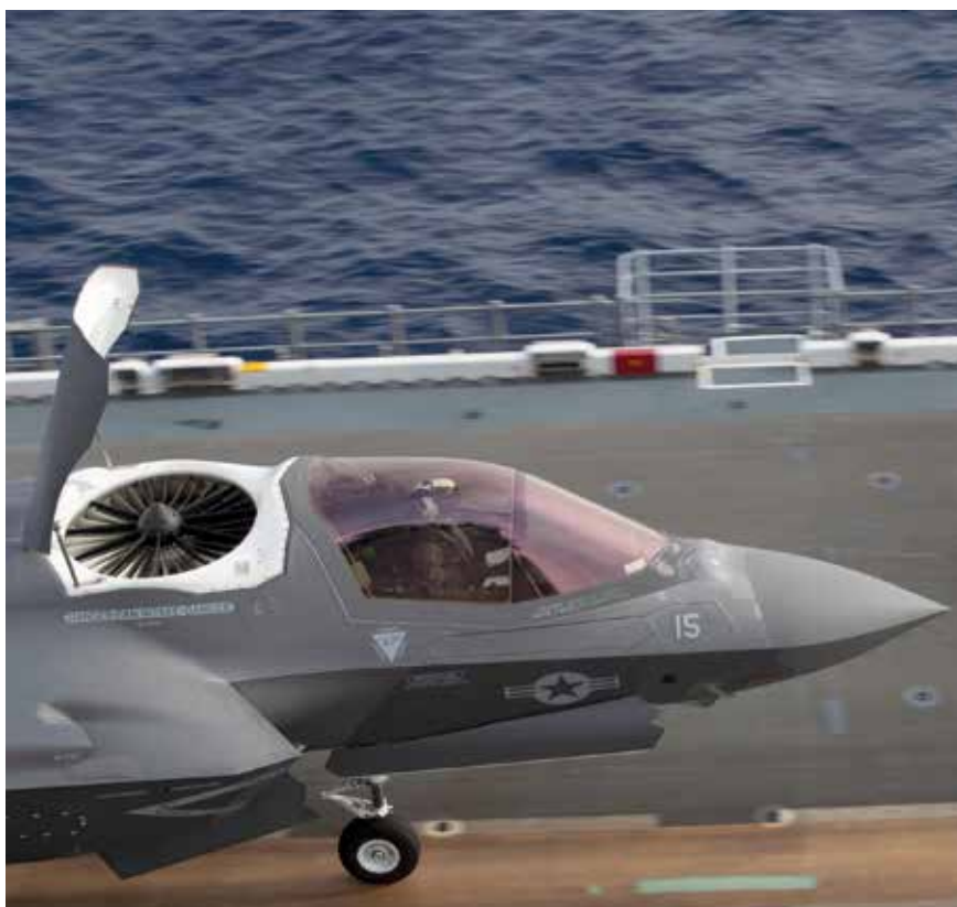
The F-35B's Rolls-Royce designed lift fan provides 9,072 kgf of thrust for vertical flight.
