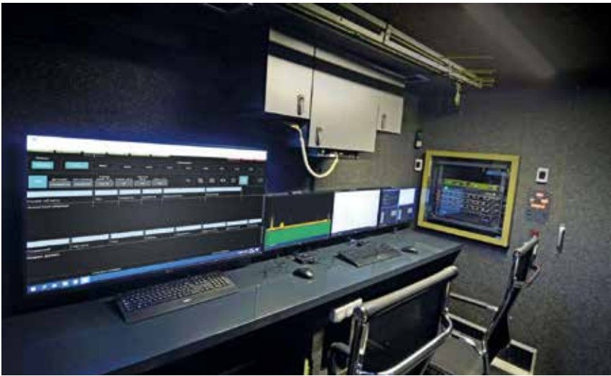
The interior of the Khortytsia-M mobile COMINT complex has two workstations for operators who control the operation of COMINT and direction finding devices, including the Apella automated multifunctional COMINT complex, and Plastun-RP3000. Additionally, the container is equipped with a living area for the crew during extended operations.
