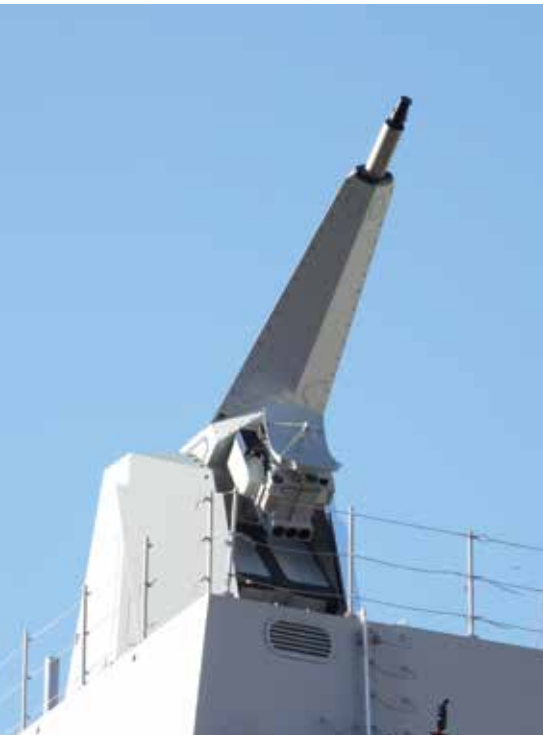
Leonardo's 'Single Deck' (Sovraponte) is a completely new light and low footprint 76/62 mm gun mount with the same capabilities as the SRGM/Strales. The Netherlands and Belgium are the first international customers.
