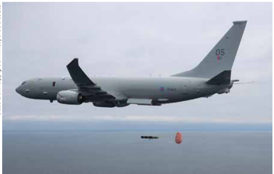
A UK Royal Air Force P-8A test launches a Mk 54 lightweight ASW torpedo, during trials off the Scottish coast in 2021. The various global P-8A operators usually follow the standard USN fit for Poseidon sensors and weapons.
