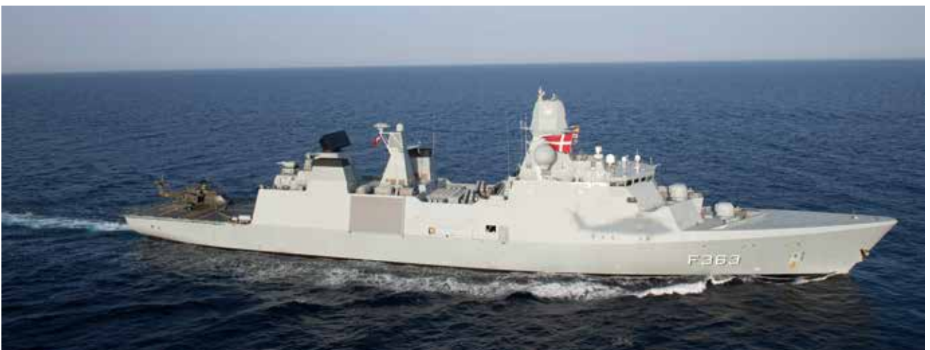
The Babcock Arrowhead 140 design is based on the hull of the Royal Danish Navy's Iver Huitfeldt class air defence frigates. This photograph shows HDMS Niels Juel, the third and final member of the class.
