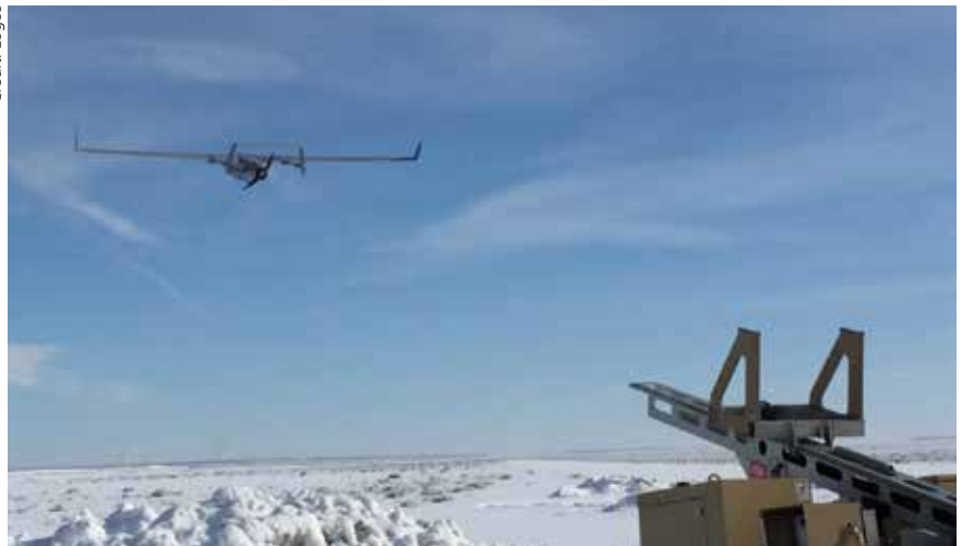
Logos tested the Redkite-1 WAMI sensor on the RQ-21 UAV in 2017.
