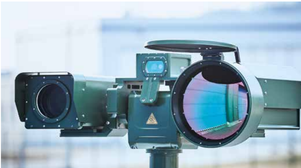
Longer-range vision systems, such as the EVPU Defence Sirius optronic sight pictured above, incorporate day and thermal sensors, and are capable of detecting targets out to ranges of 25 km, depending on the variant.
