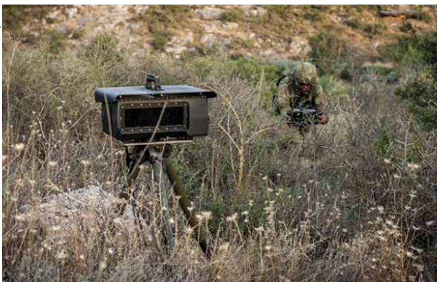
SupervisIR is a passive, staring IR sensor for covert missions requiring persistent surveillance.
