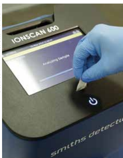
IMS detectors, such as this Smiths Detection Ionscan 600, typically use swabs of cloth or paper rubbed on a given surface, in order to detect a target substance.
