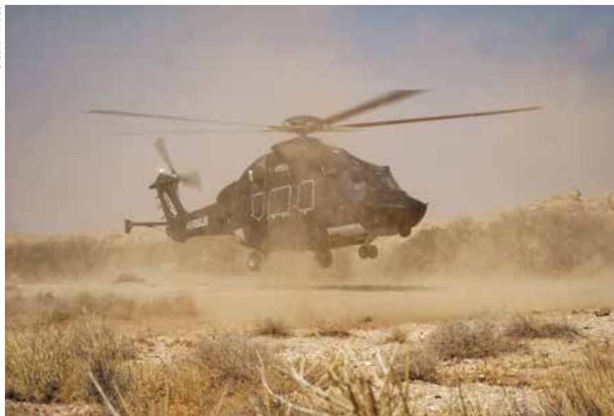
The H175M has recently completed testing in Saudi Arabia. On the larger side of the spectrum – Airbus calls it a 'Super-Medium' helicopter – it has a large internal cabin of 12 m 3 with space for 16 troops, internal fuel tanks providing a range of up to 1,111 km, and an integrated Electronic Warfare capability.
