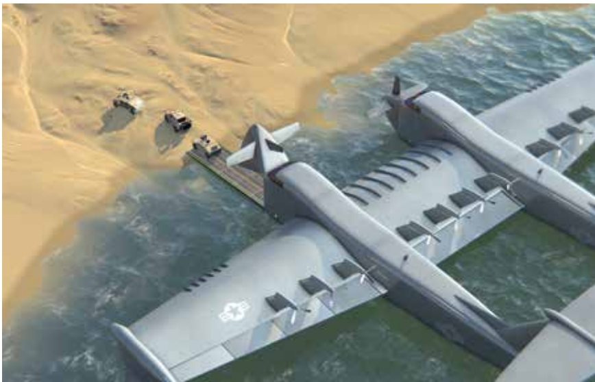
General Atomics' Liberty Lifter concept presents a dual-hull connected by a third wing-segment.
