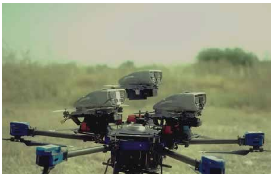
Up to three Lanius micro-UAVs can be transported closer to the target by a 'mothership' UAV.
