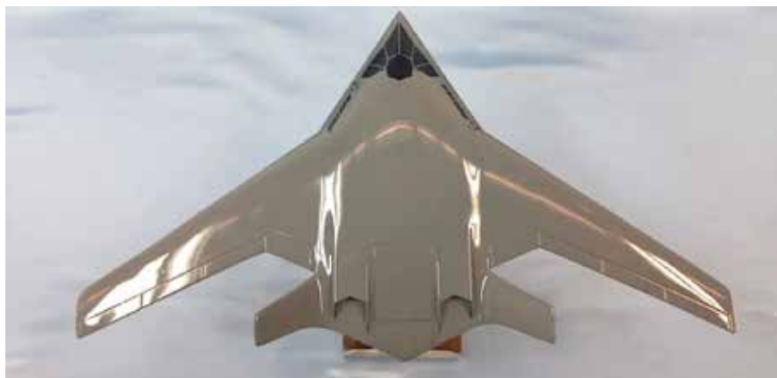
The top-down view of Boeing's BWB stealth design clearly displays the internal engine carriage and the top-mounted exhaust system.
