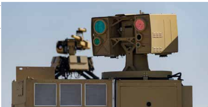
The P-HEL palletised high energy laser at Yuma proving ground.
