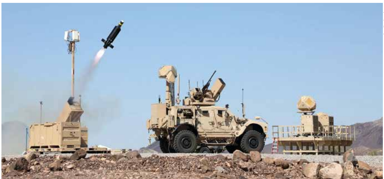
A Raytheon Coyote Block 2 interceptor being launched. FS-LIDS palletised components are visible in the background, while an M-LIDS kinetic effects vehicle is visible in the middle foreground.
