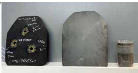
Three stages in the production of Boron carbide body armour: (right to left) powder, sintered Boron carbide plate, completed plate (showing ballistic damage). The completed plate comprises a fabric layer at the front, sintered Boron carbide plate in the middle, and backing at the rear to dissipate projectile energy and prevent splinters from reaching the body.
