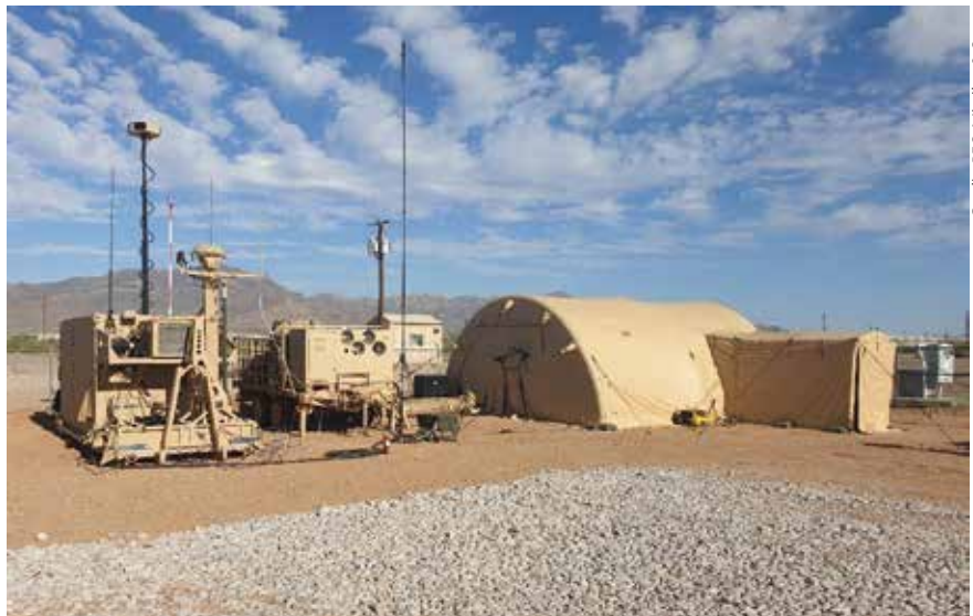
The IBCS from Northrup Grumman shown here was designed to provide a sensor fusion capability to air defence. It has been tested using various radars and sensors from the air and land. It is in production for the US Army and various other users.
