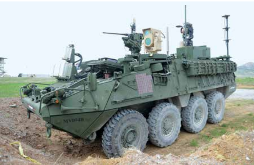
A MEHEL Stryker fitted with a 5 kW CLWS laser weapon during MFX-17 at Fort Sill, in April 2017.
