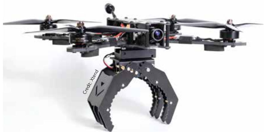
The Wolverine micro-UAV equipped with a claw manipulator.
