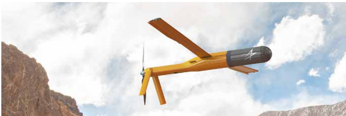
Lockheed Martin's tube-launched MORFIUS can use its HPM warhead to defeat UAV swarms that may be out of range of terrestrial HPM systems.
