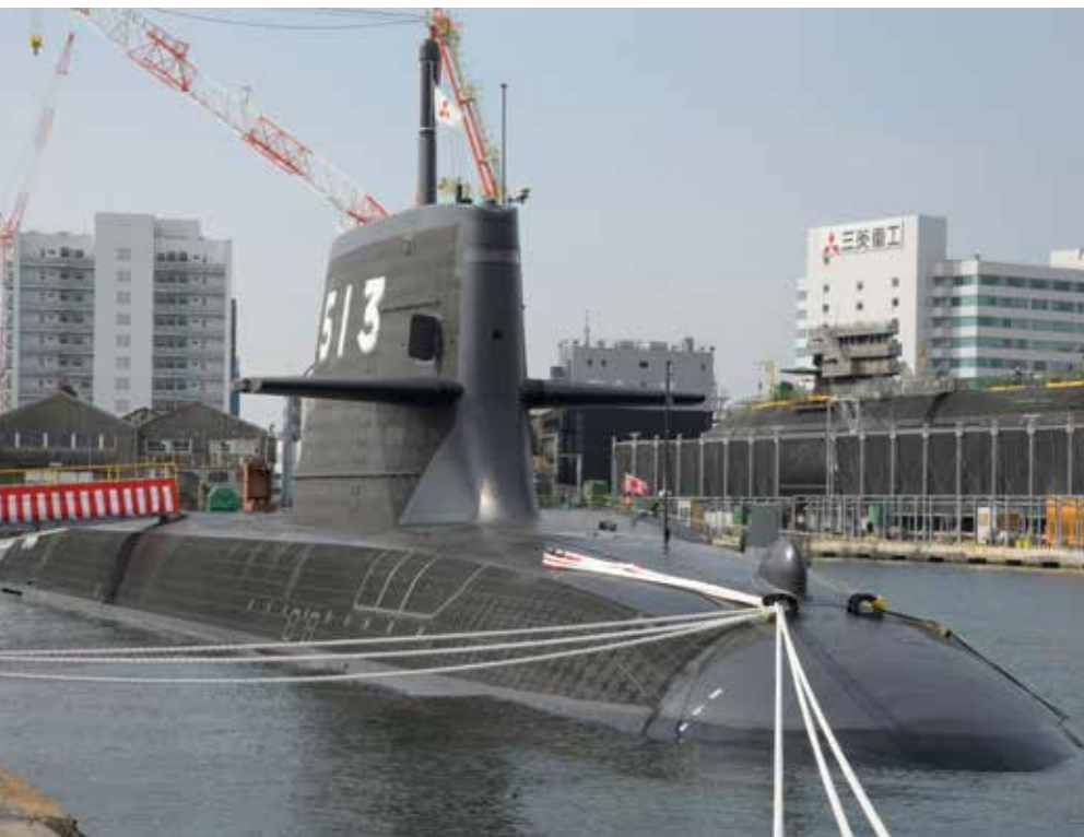
JDS Taigei (SS-513) is the first of a class of new Japanese diesel-electric submarines equipped with lithium-ion batteries.
