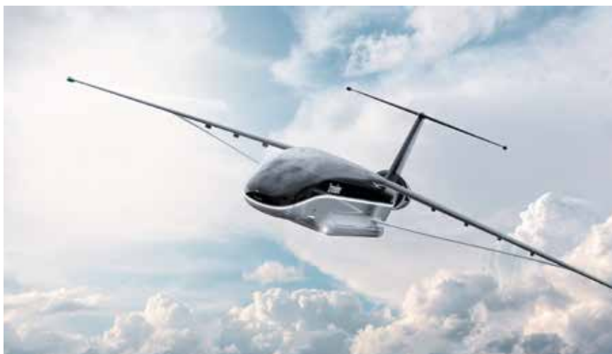
The DL200 unmanned transport's design features electric propulsion and a capacity of 35-40 ISO containers.
