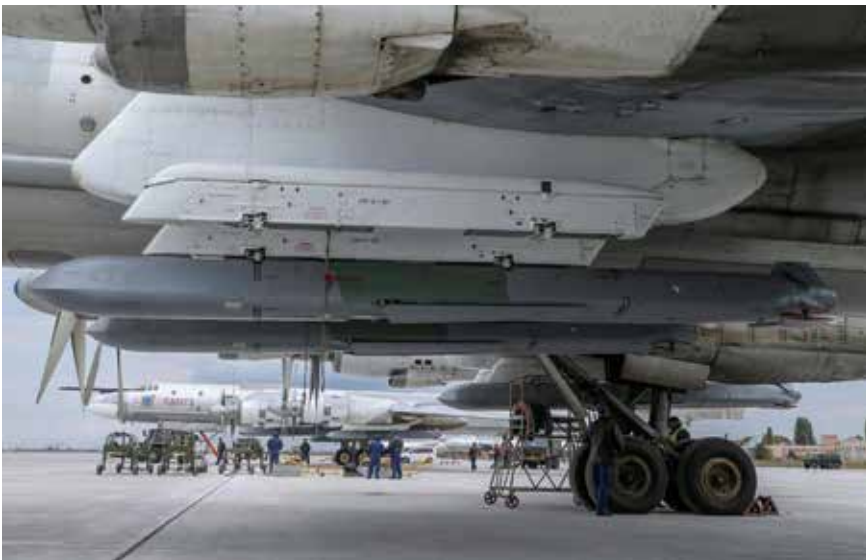
Nuclear-capable cruise missiles such as the Kh-101 are deployed from bombers such as the Tu-95.
