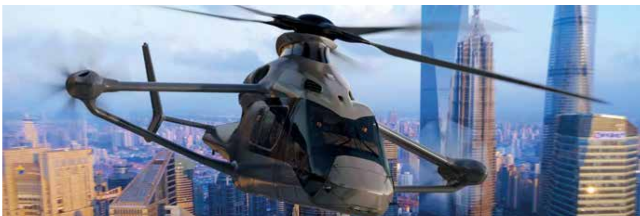
The Airbus Racer demonstrator was developed as part of the European Clean Sky 2 research programme. It could be a harbinger of things to come for medium weight helicopters in the future with a hybrid metallic-composite airframe designed for low weight, 30% fuel savings in cruise mode and lower acoustic footprint.
