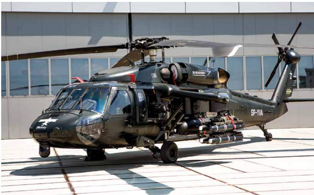
The S-70M being offered for the NMH requirement by Lockheed Martin UK is based on the S-70i ‘International’ Black Hawk manufactured by Sikorsky subsidiary PZL Mielec in Poland.
