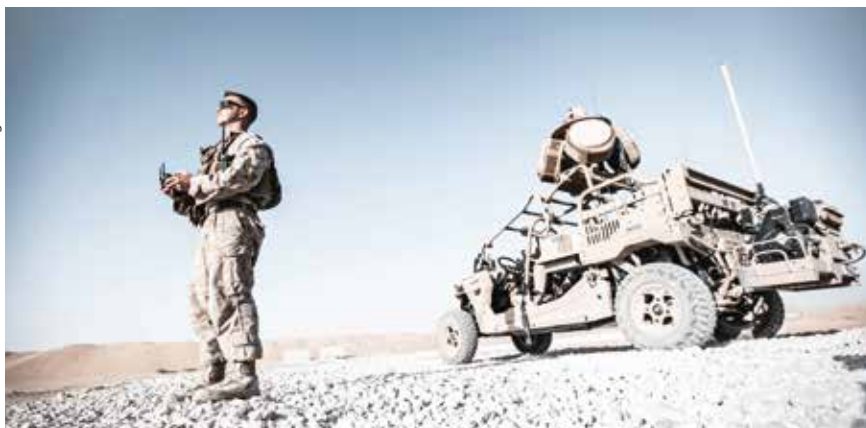
Early version of LMADIS is visible in the background, while a Low Altitude Air Defense (LAAD) Officer operates a drone during C-UAV training in the Kingdom of Saudi Arabia, on 12 June 2021. This version of the system used the RPS-42 radars and CM202 mast-mounted sight, both of which were replaced on the version of LMADIS shown in 2023.
