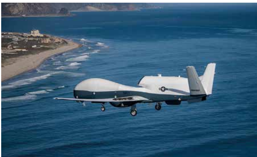
At the larger end of the spectrum, high-altitude long-endurance UAVs such as the Triton, in service in the US and Australia, are less concerned with SWaP aspects of their propulsion systems than with reliability and flexibility.
