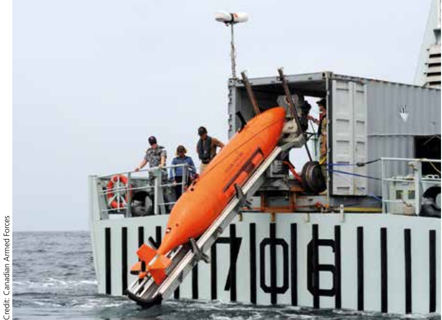
A Royal Canadian Navy Kingston-class maritime coastal defence vessel operates a containerised HUGIN AUV during the USN-led 'RIMPAC' exercise in 2016. Containerising capability is a key operational concept for navies in deploying AUVs and ROVs.
