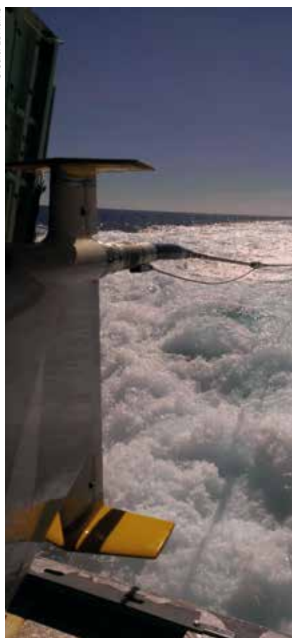
Active Low Frequency Towed Array Sonar (ALOFTS) from L3Harris combines a high-powered, active source in a variable-depth towed body. A directional towed array receives active and passive signals.
