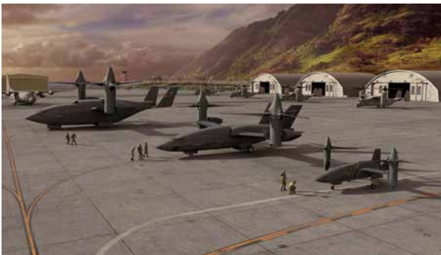
Bell's heavy, medium and light HSVTOL concepts. The C-130 and V-22 in the background provide scale.
