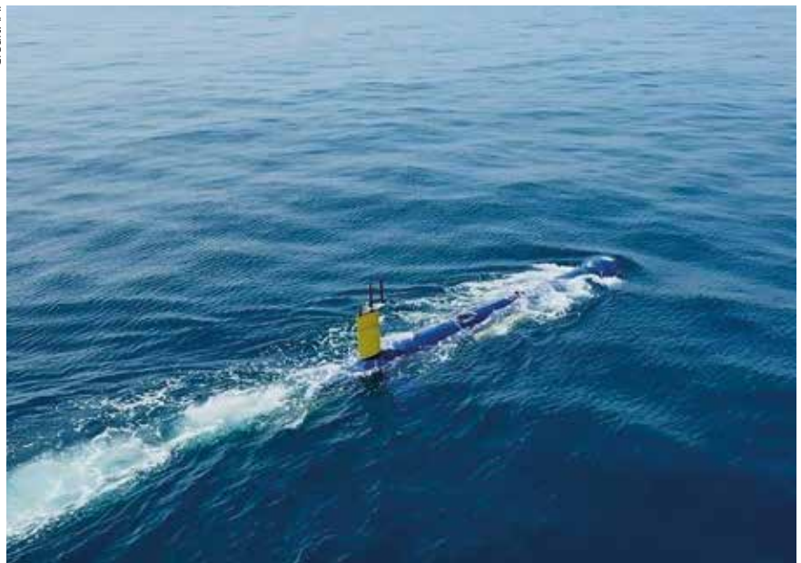
The BlueWhale AUV, developed by IAI. AUVs such as this one are capable of undertaking a range of missions, including intelligence-gathering above and below the sea surface, as well as detection of underwater targets such as submarines and naval mines on the seabed.
