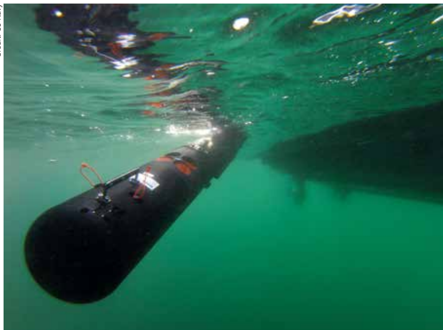
A REMUS 100 autonomous underwater vehicle (AUV) is tested at a 'REPMUS' exercise. AUVs, along with underwater gliders, will be a core component of NATO ASW Barrier concepts.
