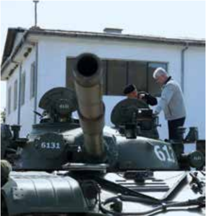
The modernised T-72 comes with an auxiliary power unit, four laser-warning receivers, a new fire-control system, thermal gunner's sight, a battle management system, driver's thermal camera, a new thermal sleeve for the main gun, and an upgraded intercommunication system for the crew.
