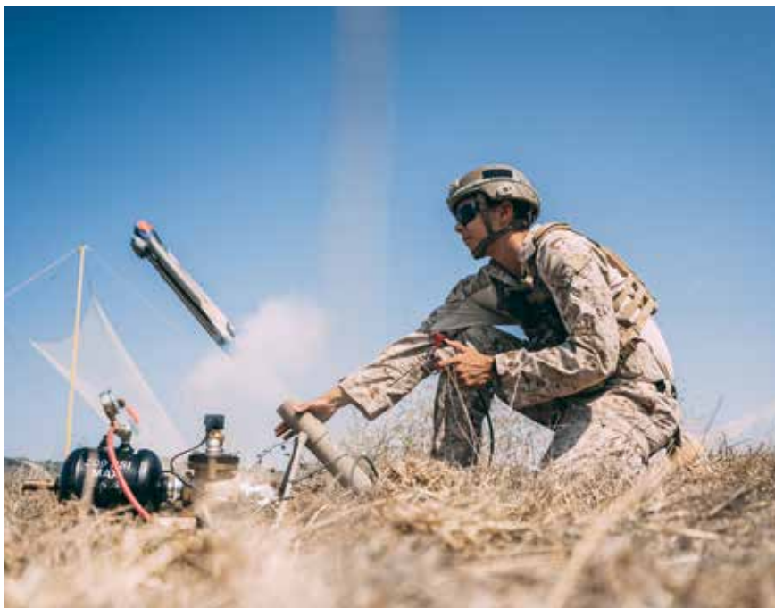
A tube-launched Switchblade 300 lethal miniature aerial missile system is launched with the aid of compressed gas.
