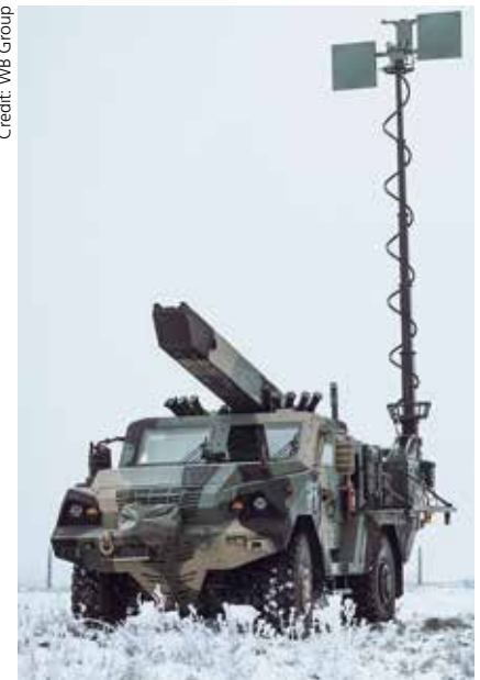
A Waran wheeled armoured vehicle (Polish version of the Czech PATRIOT II) serves, among others, as the launcher of the Gladius reconnaissance and attack UAV.
