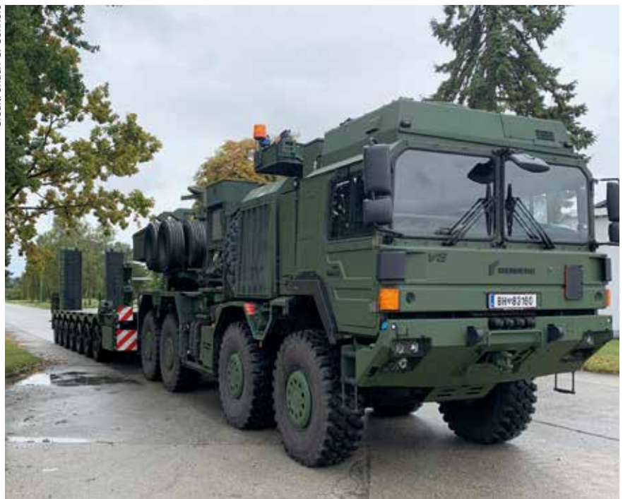
The seven-axle semi-trailer coupled to this Austrian Army HX81 tractor may well allow for complaint road transport of all Austrian Army loads on road in peacetime, but it is an inescapable fact that in environments such as those currently found in the Ukraine, that trailer would not be capable of being dragged undamaged where the tractor unit could drag it.
