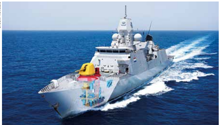
Nevesbu has been contracted by both Leonardo and COMMIT to develop the integration and associated design change package for the 127/64 LW gun installation, the revised ammunition compartment, and the new automated handling system.
