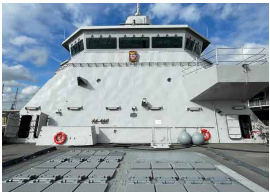
The LCF frigates – HNLMS De Ruyter is pictured here – are each fitted with five eight-cell Mk 41 vertical launch modules.
