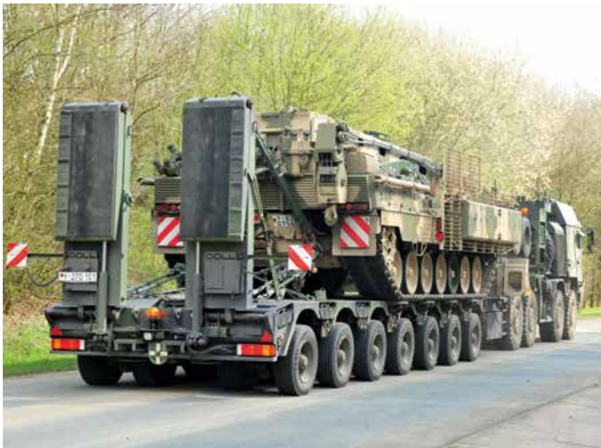
From the rear, a current German Army HX81/Doll semi-trailer combination. To enable escort-free movement when unladen, to accommodate an MBT (or similar) payload the trailer requires the use of extending 'greedy boards'.
