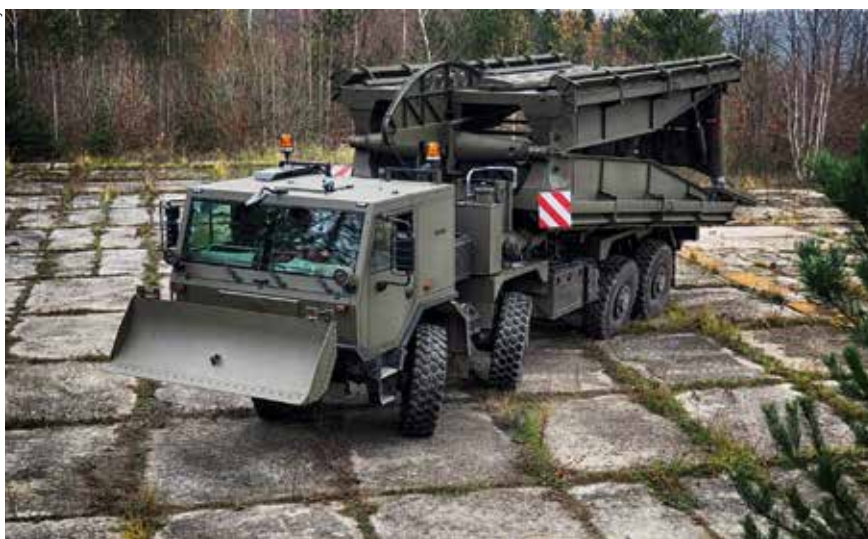
The AM-70 EX, based on the T-815-7 8x8 chassis, could be the future replacement of the legacy AM-50 bridge-laying vehicles operated by the 15th Engineer Regiment.
