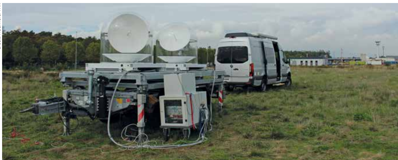
The two antennas comprising the Sabbia-2.0 architecture are clearly visible in this picture. One antenna samples and records Starlink downlink signals, the other monitors signals for signs of disturbances caused by targets.
