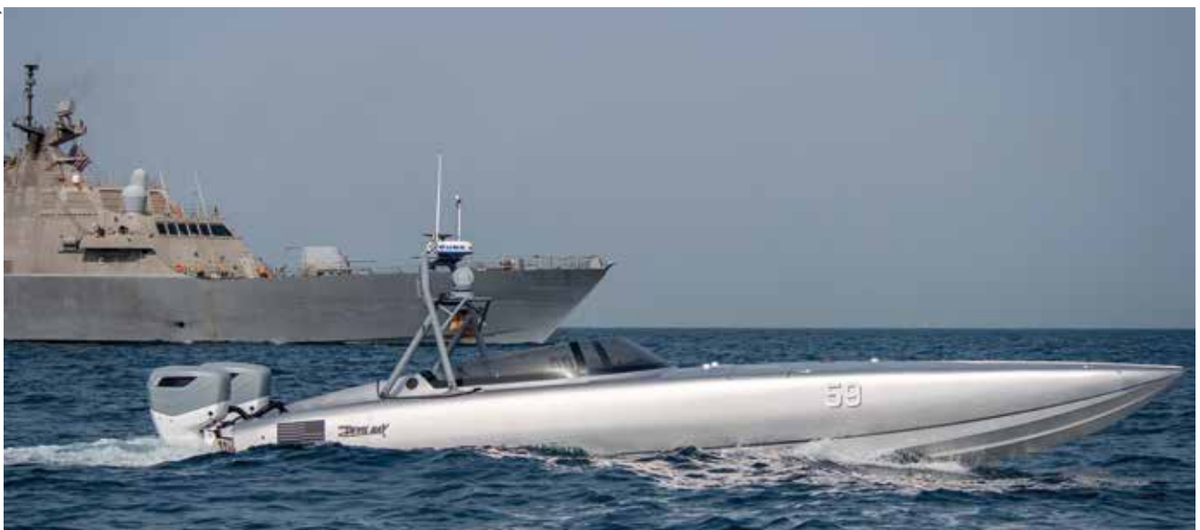
A Devil Ray T-38 USV escorts USS Sioux City (LCS-11) in the Arabian Sea. The T-38 achieves speeds of 80 knots and can pull six G's during high-speed manoeuvres.
