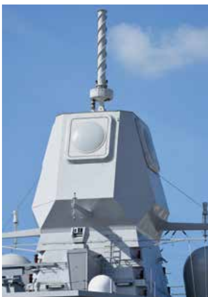
The APAR X-band multifunction radar performs horizon search, multi-target tracking, missile guidance support, and terminal illumination for the LCFs' ESSM Block 1 and SM-2 Block IIIA missiles.
