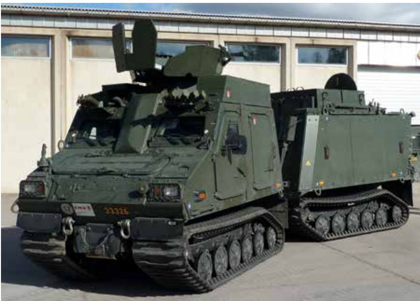
Beowulf, also known as Husky 4, is the unarmoured variant of the CATV.
