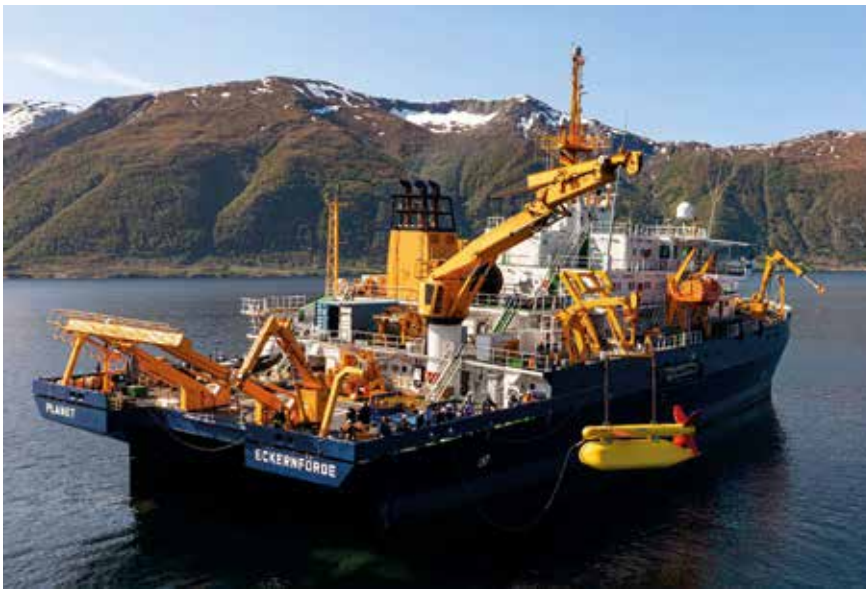
Research vessel Planet in the Sognefjord deploying the towed body FLAME II for acoustic self-noise investigations.
