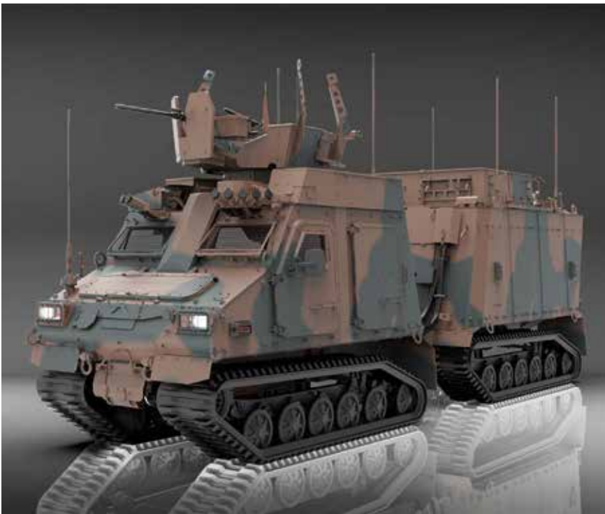
The Collaborative All-Terrain Vehicle (CATV), also known as Husky 3, is an armoured articulated all-terrain tracked vehicle.
