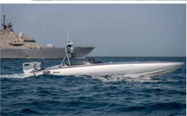
The 11-metre T38 „Devil Ray“ achieves top speeds of 80 knots and can be carried aboard most ship classes. It can be deployed as an armed escort for the parent vessel when transiting dangerous waters, or be sent forward to conduct reconnaissance and attack missions. (© US Navy)
