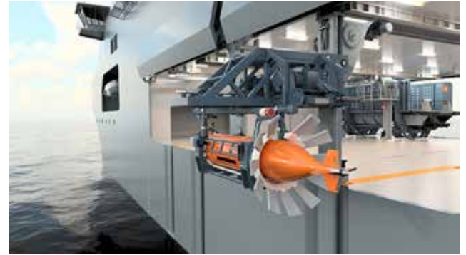
Mission Bay Handling system was developed in response to this growing need for ships to be versatile (© Kongsberg)
