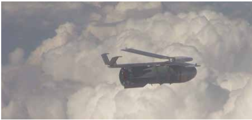
This image shows a FAB-3000 with a UMPK guidance kit during flight. The size of glide bombs has increased steadily throughout the war with the result that the much greater blast radius places a lower burden upon accuracy.
