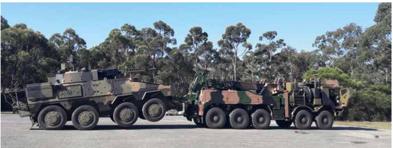
In one package costing around EUR 2.5 million, the 45M is technically capable of winch recovering, suspend towing or uprighting all Boxer variants. The rotator is also capable of lifting all mission modules. No single Boxer recovery variant (costing an estimated EUR 10-12 million) would be capable of this.
