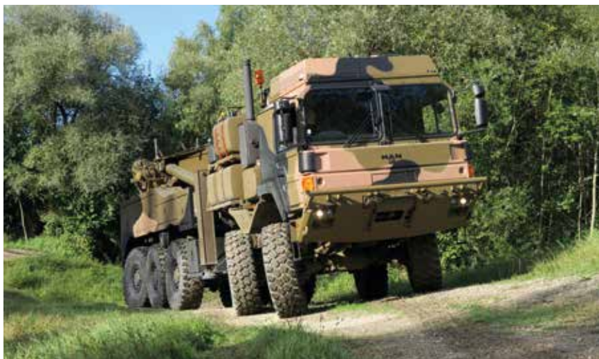
During trials in Australia, a 45M suspend tows a HX77. Note the difference in tyre size between the two; 395/85 R 20 on the HX77, 16.00 R 20 on the 45M
