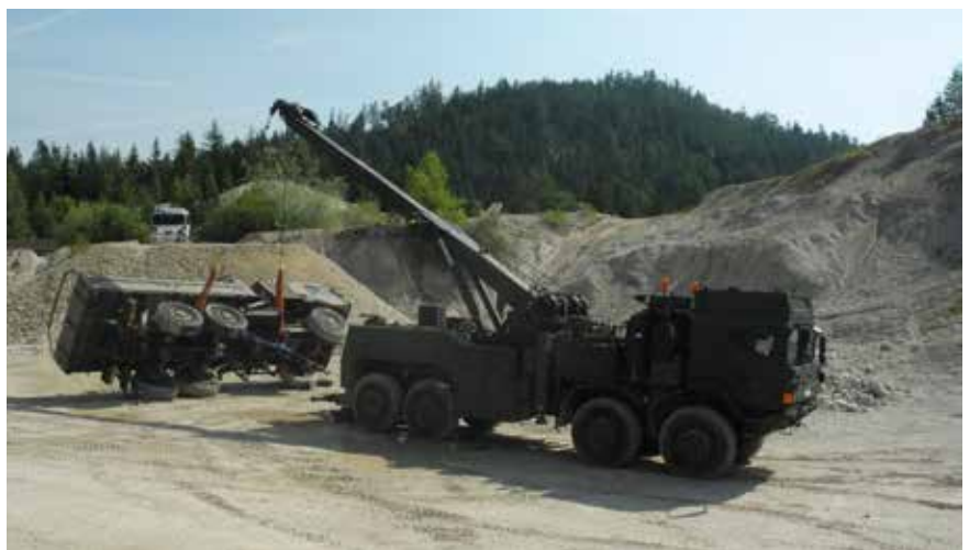
Using the rotator and main winch, a Canadian spec 44M demonstrates the type of controlled recovery of an overturned casualty that is possible with this set-up
