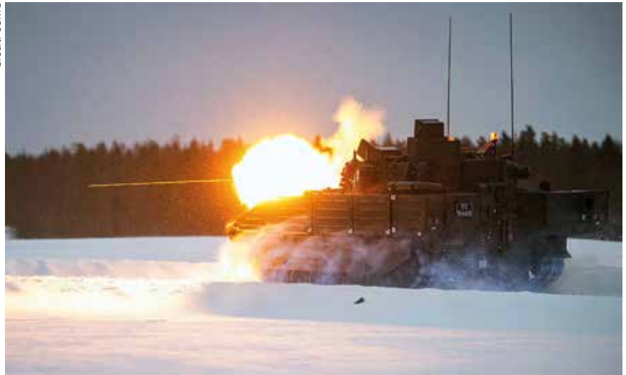
An Ajax vehicle of the Household Cavalry conducts a live fire of its 40 mm CTA cannon as part of an extreme weather testing programme in Lapland, Sweden, where temperatures dropped to -30°C. The capability to fire the gun system on the move was successfully demonstrated.
