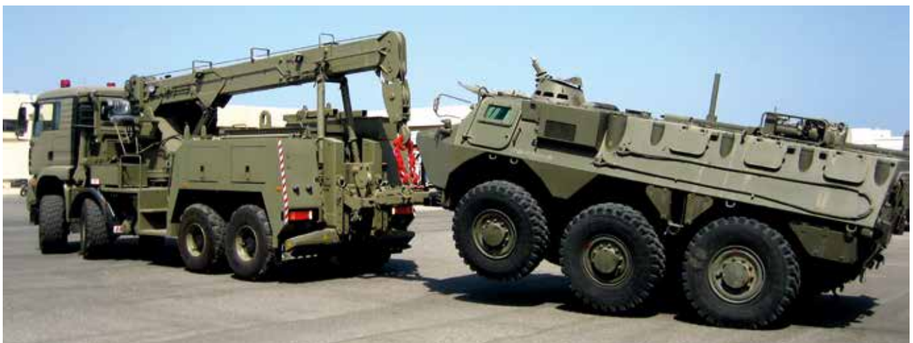
Technically the entire MAN portfolio can be fitted with military recovery bodies, but in general nothing smaller than a three-axle truck is. This TGS 8x8 was photographed on trial in Asia.
