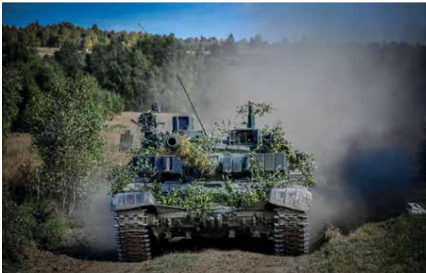
The Czech T-72M4CZ is one of the better T-72 upgrades that has been put into service. Every aspect on the iron triangle (firepower, mobility, survivability) was addressed in a comprehensive modernisation. However, obsolescence has severely hampered availability rates for the tank.
