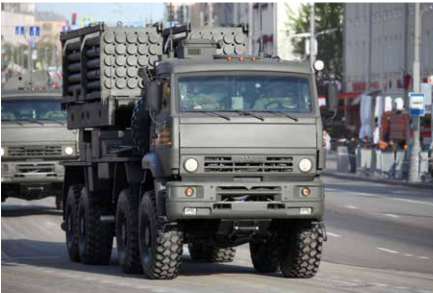
The ISDM Zemledelie (foreground) remote mine-laying system, followed by its transloader vehicle (background).
