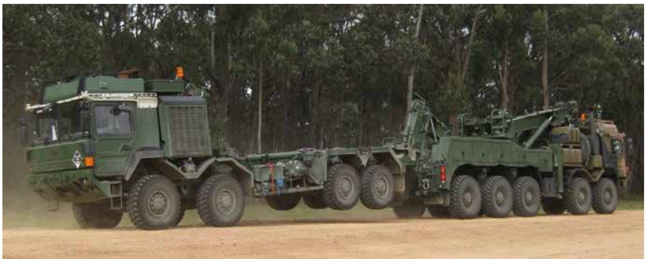
An Australian Army 45M with a softskin cab. Note the contra-steer of the rearmost axle, this giving the 45M a slightly smaller turning circle than the 8x8 44M.
