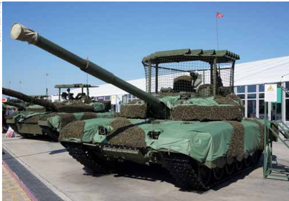
A T-90M on display at the Army 2023 exhibition. This example is fitted with overhead protection and the 'Nakidka' thermal and visual camouflage package, along with a row of Kontakt-1 explosive reactive armour (ERA) over the toe plate.
