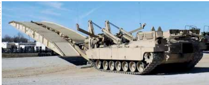
The US Army's M1074 JAB, being based on the M1 Abrams platform, can support a much heavier payload than the older M60 AVLB and has greater mobility.
