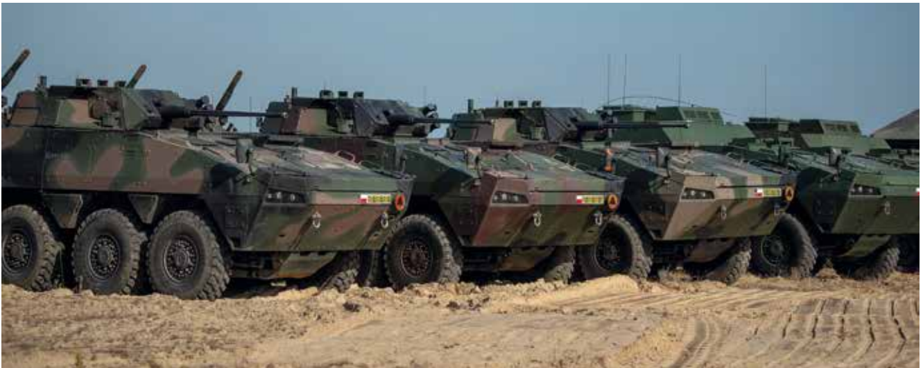
Shown here are three Rosomaks with the original Hitfist-30P turret. In July 2024, Poland signed a second contract for the KTO Rosomak. Under this agreement, 58 vehicles will be fitted with the ZSSW-30 remote turret, which are designed and manufactured domestically.
