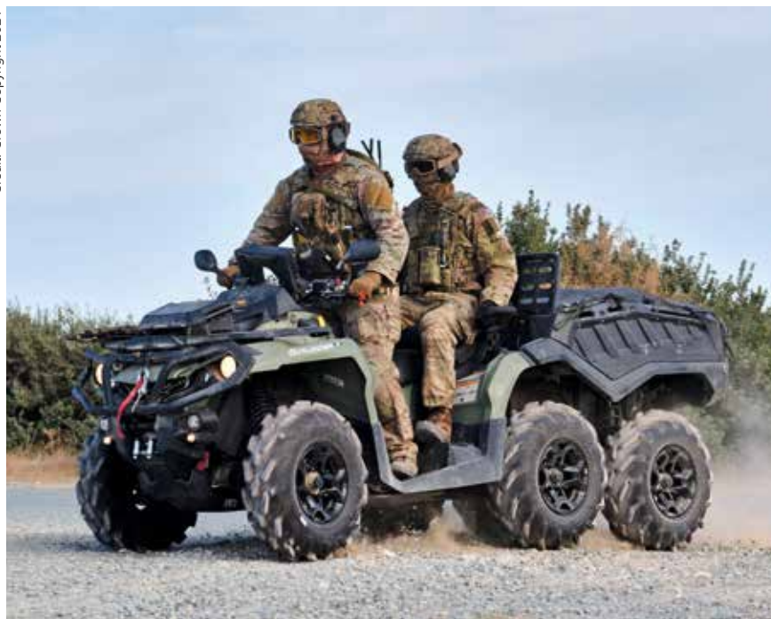
Bravo Company, 40 Commando Royal Marines, on exercise in Cyprus with the Canadian American (CAN-AM) 6-wheeled Outlander Warrior vehicle. The British Army has tested and also operated a wide range of ATVs/UTVs, including unmanned systems. This will form the basis for its Light Tactical Mobility Platform (LTMP) efforts.
