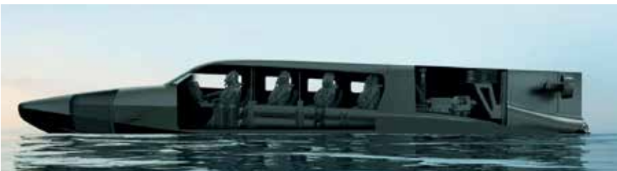
This cutaway image shows the Victa's seating arrangement and its waterproof battery chamber.
