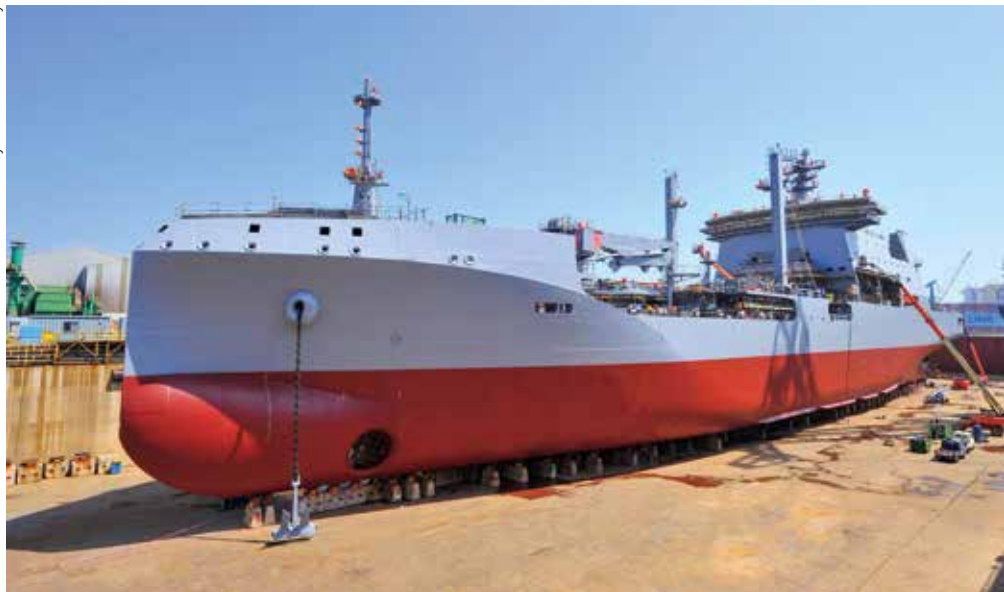
A view of HMNZS Aotearoa under construction at Hyundai Heavy Industries showing her innovative hull form.
