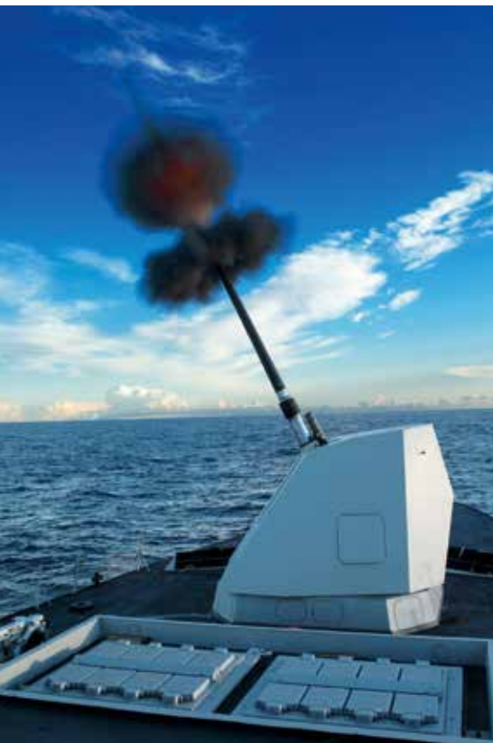
Leonardo's OTO 127/64 LW (lightweight) medium calibre mounting can fire Vulcano munitions out to ranges of 100 km.
