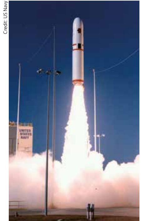
A test launch of the Trident II (D-5) missile, taking place at 18:45 on 12 June 1987, from Complex 46 on Cape Canaveral. The D5 is a three-stage, solid propellant, inertially guided fleet ballistic missile launched underwater from US Navy Ohio class, and Royal Navy Vanguard class submarines.
