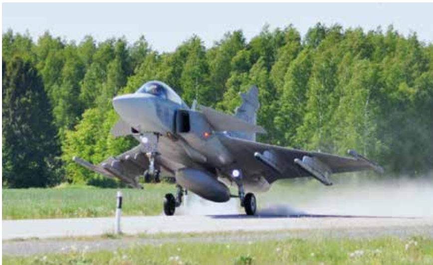
A Gripen C landing on a Swedish highway near Sâtenäs Air Base during a SwAF ACE exercise on 17 May 2024. Gripens need just 700 m of road to land and take off during ACE operations: a capability that could prove very valuable to the Ukrainian Air Force.
