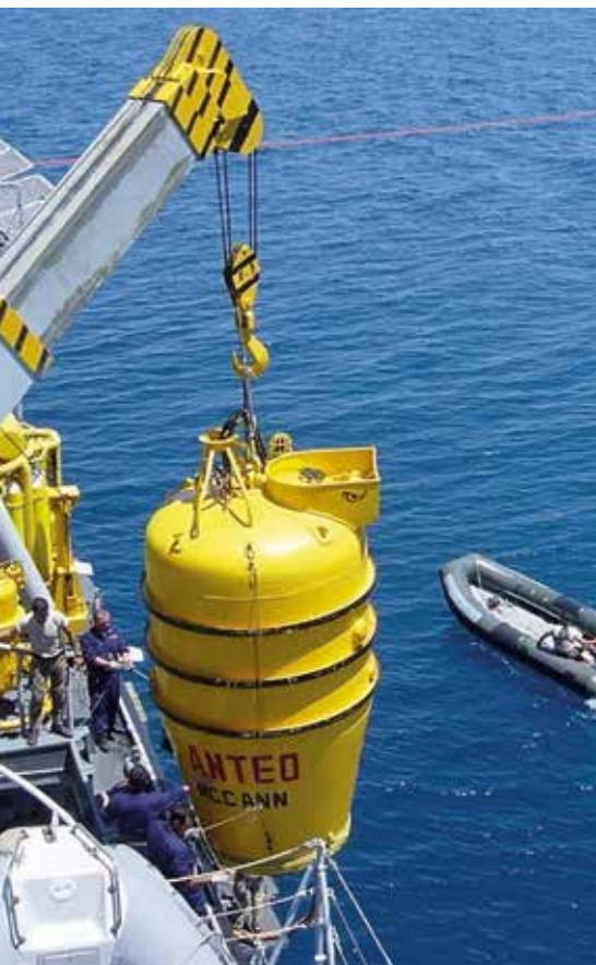
Italian Navy's McCann chamber descending from Mother Ship (MOSHIP) Anteo.
