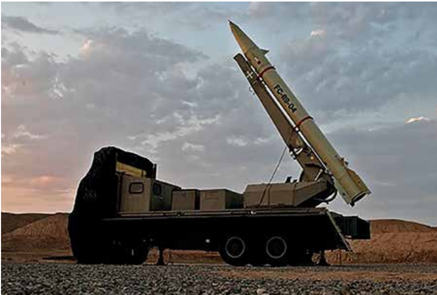
This 2012 image shows the Fateh-110 during launch from an Iranian TEL. A derivative of the Fateh-110 is believed to provide the Houthi ASBM capability.
