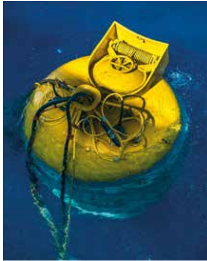
Turkish McCann Submarine Rescue Chamber from TSC Alemdar MOSHIP.
