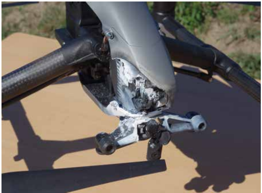
Pictured: damage to a drone after several seconds of illumination by a high-energy laser.
