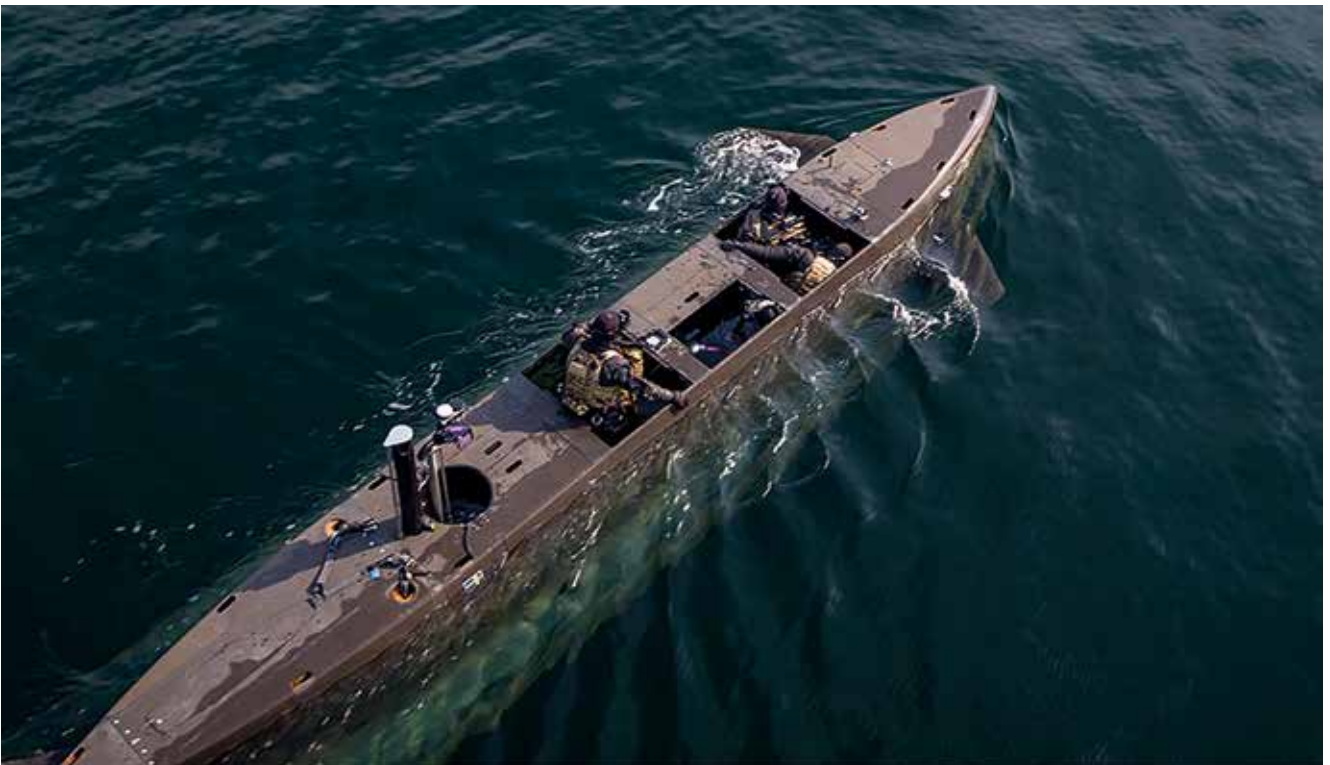
Carrier Seal TDV from above showing hatches for rapid entry/exit of boarded passengers and two crew at forward controls.
