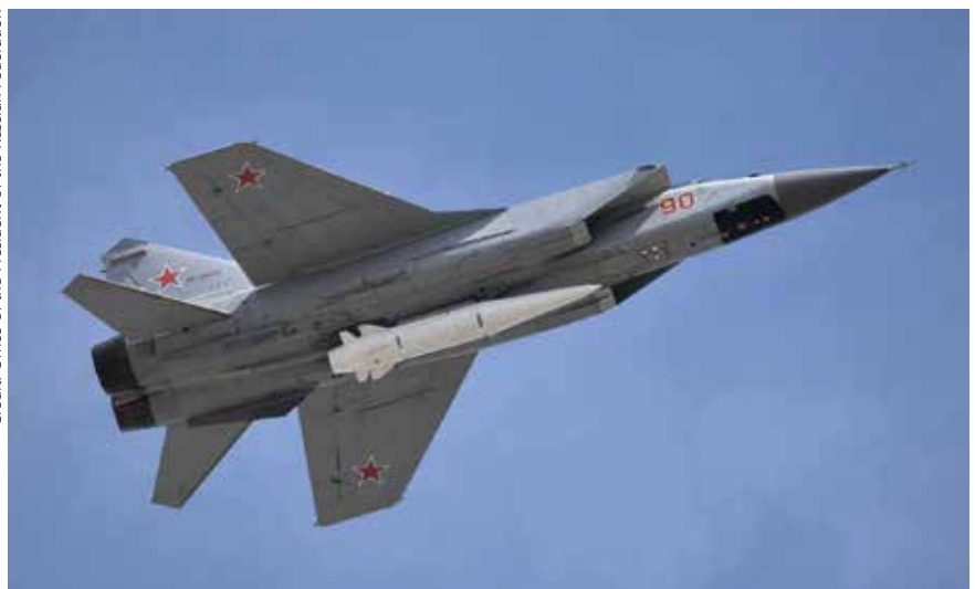
The Kh-47M2 Kinzhal is an air-launched version of the 9M723. Its speed and approach make it very difficult to intercept.
