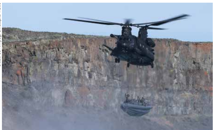
Army MH-47G helicopters are used to transport US Navy special boat team watercraft and personnel to and from lakes when overland transport is not practical.
