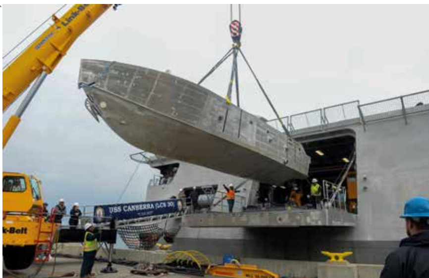
An unmanned surface vehicle is craned aboard the Independence variant littoral combat ship USS Canberra (LCS-30), as a part of the first embarkation of the MCM mission package in April 2024.
