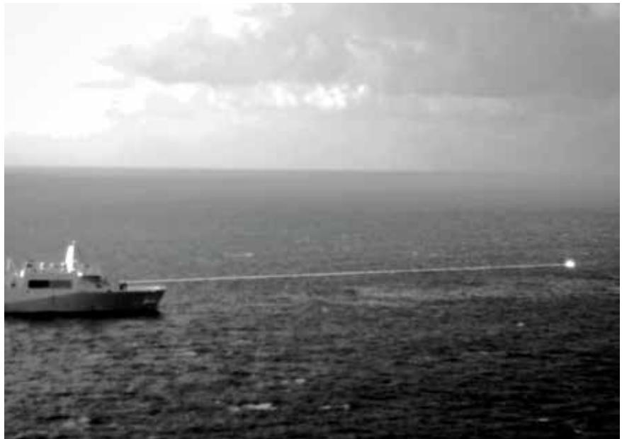
The US Navy has one of the oldest and largest research and development programmes; this photo shows a laser demonstrator trial against a UAV conducted by the amphibious transport dock USS Portland (LPD-27) in May 2020.
