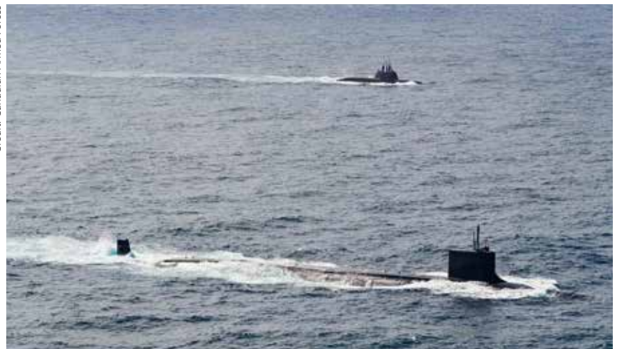
An SSN – the US Navy (USN) Virginia class nuclear-powered submarine USS John Warner (foreground) – sails with an SSK – the German Navy Type 212A diesel-electric boat U-35 – during the NATO anti-submarine warfare exercise 'Dynamic Manta' in 2022. Nuclear propulsion offers the most sustainable and flexible option for submarine operational output; conventional propulsion offers still significant, but more affordable, capability.
