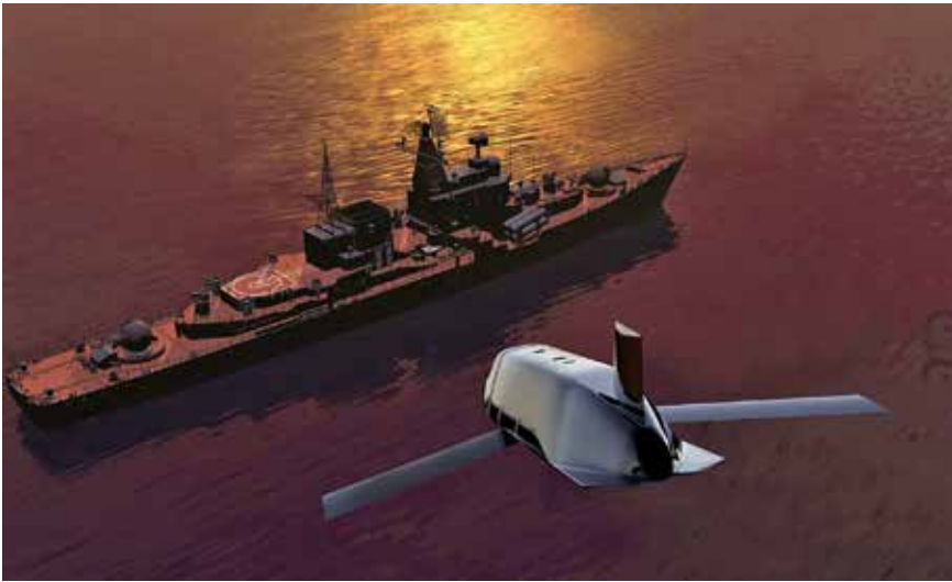
LRASM is designed to penetrate surface ship defences and destroy vessels from stand-off ranges of some 80 km.
