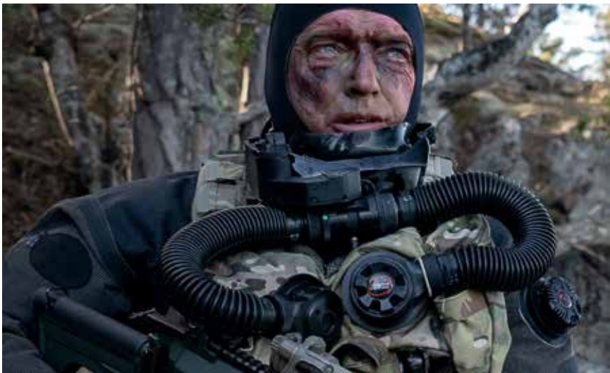
The TRUAS will be capable of carrying a payload of roughly 70 kg of The depth to which TDVs can operate depends on the LSS of the divers onboard. Pictured: Shadow tactical diving LSS, weighs 9 kg, offers a duration of 4–6 hours; maximum depth of Shadow Excursion using nitrox is 30 metres of seawater.
