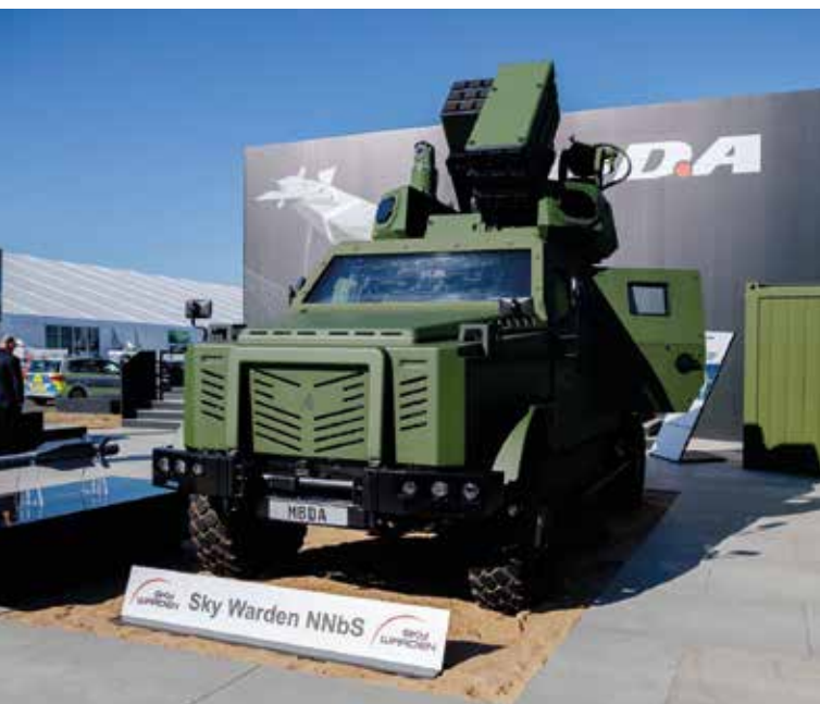
▲ The Skywarden NNbS on display at ILA 2022. Shown here mounted on an ACS Enok 9.5, with two nine-cell launchers for SADM. [MBDA]
