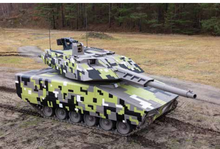
▲ The Lynx 120 FSV variant of the Lynx KF41, shown here in the 2022 configuration, with what appeared to be the KF51 Panther turret. [Rheinmetall]
