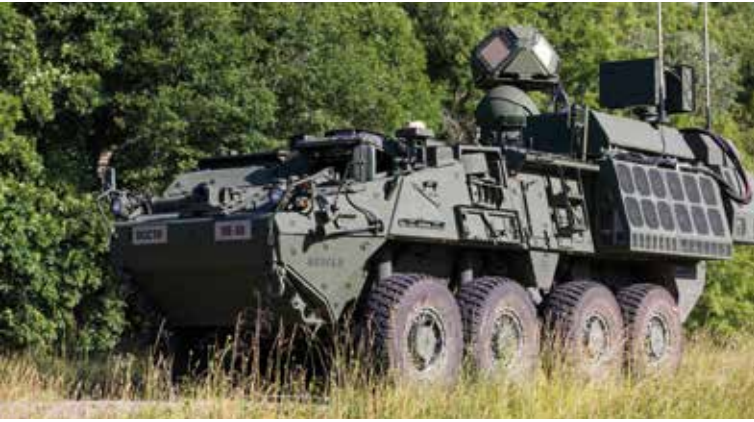
▲ A Stryker-mounted DE-M-SHORAD laser system during testing at Fort Sill, Oklahoma. [US Army]
