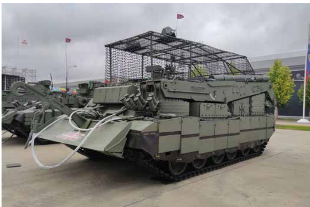
▲ A BREM-80 ARV featuring a combination of Relikt ERA, anti-drone nets and two drone jammers on the roof at the Armiya 2024 exhibition. [Alexey Tarasov]
