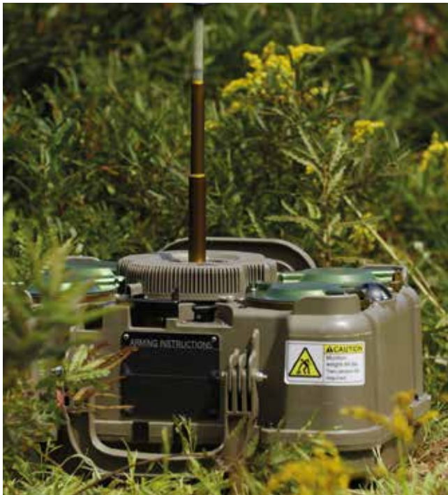
▲ Hand-emplaced, XM204 top-attack EFP-delivering system, sits deployed and waiting for a target. [Textron]
