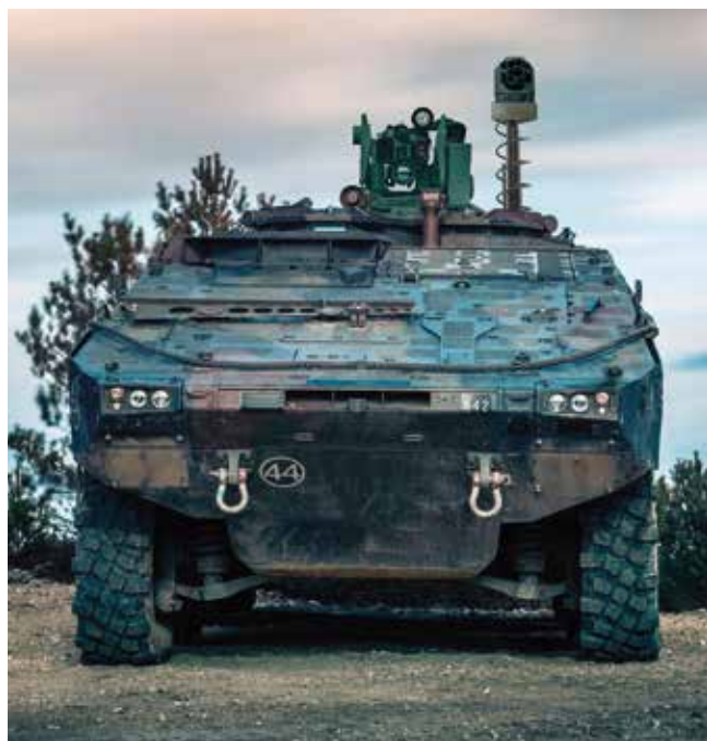
▲ The Thales PAAG system, installed here on a Boxer multi-role armoured vehicle, allows under-armour target designation instead of exposing a dismounted soldier to do the job. [Thales]
