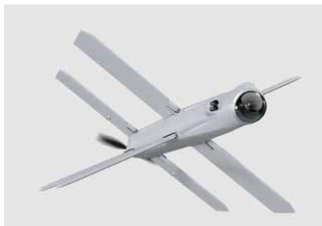
▲ The Izdeliye-52 variant (pictured) of Zala's Lancet family was designed to conduct strike missions at ranges of more than 30 km. [Zala]
