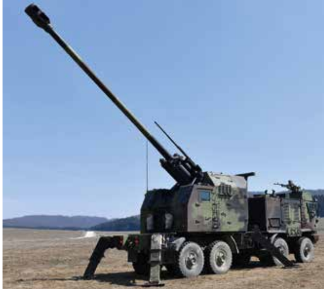
▲ Clearly visible, the four substantial outriggers fitted to Serbia's NORA-B52. [Serbian MoD]
