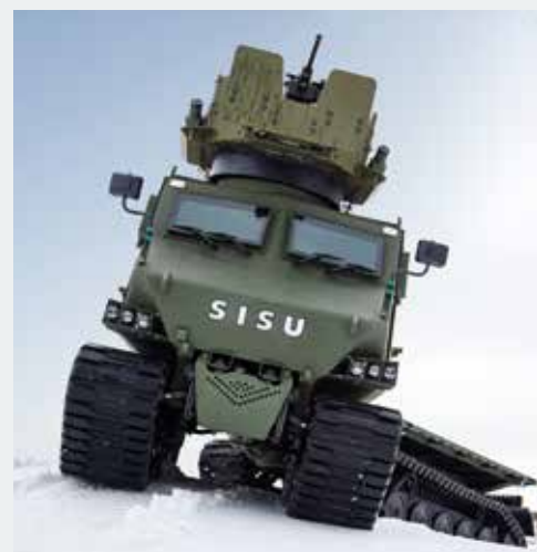
▶ Sisu GTT All-Terrain Vehicle fitted with motorised RM-750 ring mount, equipped with a 12.7 mm (.50 cal.) Heavy Machine Gun and 76 mm Wegmann Protection System. [SIMA Innovation]
