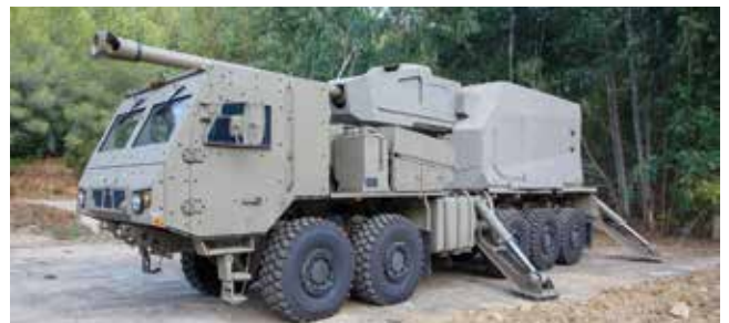
▲ Elbit's SIGMA/Roem is based on a military specific Oshkosh chassis and believed to have independent suspension, CTIS and 16.00 R 20 tyres. [Elbit Systems]
