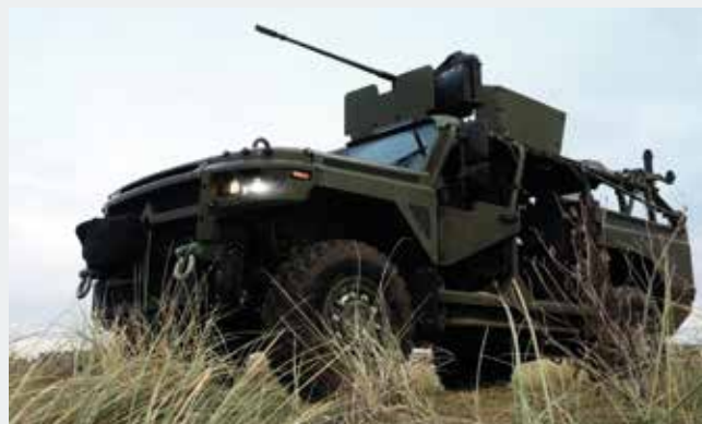
▲ Defenture Mammoth 4x4 multirole combat platform fitted with motorised RM-750 ring mount carrying the KNDS France P20 pintle-mounted 20 M 621 20 mm automatic cannon. [SIMA Innovation]
