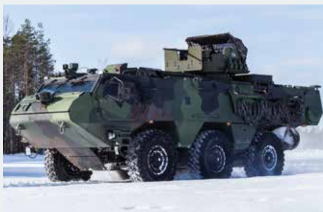
▲ Patria 6x6 APC fitted with motorised RM-750 ring mount, equipped with a 12.7 mm (.50 cal.) Heavy Machine Gun and 76 mm Wegmann Protection System. [SIMA Innovation]
