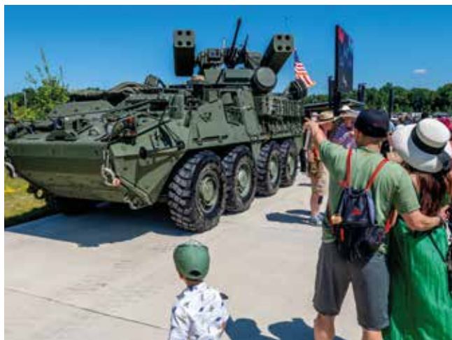
▲ The US Army displayed the two-Stinger pod configuration of 'Sgt Stout' during the 249th Army Birthday Festival at the National Museum of the US Army, Fort Belvoir, Virginia, on 15 June 2024. [US Army/Bernardo Fuller]
