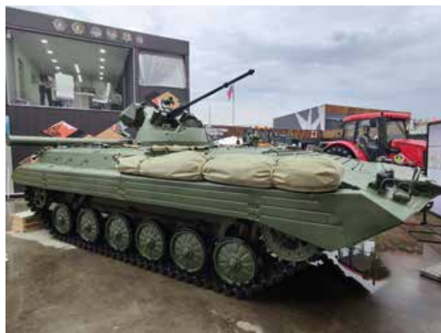
▲ A BRM-1K at the Army-2021 event. The vehicle is equipped with an unmanned turret featuring a 2A72 30 mm autocannon and PKTM 7.62 mm machine gun. [Alexey Tarasov]
