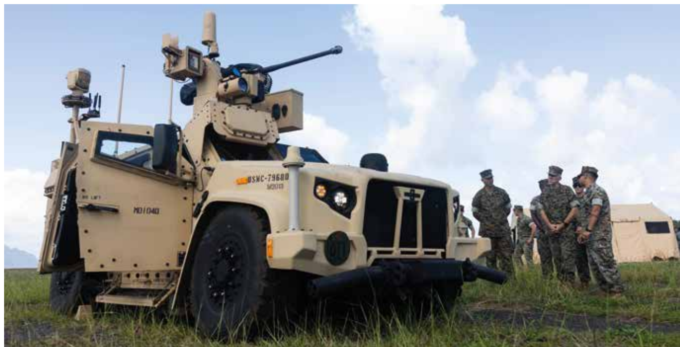
▲ The Northrop Grumman XM914 30 mm cannon has been used to arm the JLTV-based MADIS C-UAV/VSHORAD vehicle, shown here in the Mk2 configuration at Marine Corps Base Hawaii, on 14 January 2025. [USMC/Cpl Eric Huynh]
