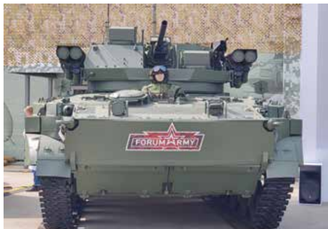
▲ A B19 IFV fitted with the Epokha unmanned turret at the Army-2022 exhibition. While this turret has seen limited production, its current status remains unclear. [Alexey Tarasov]
