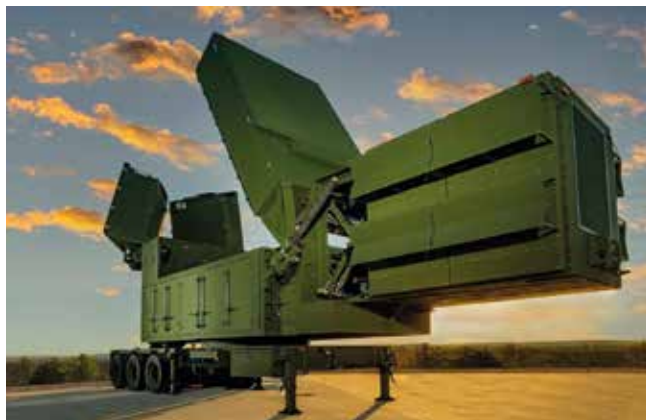
▲ A view of the LTAMDS (pronounced: L-TAMS) radar, which increases detection range substantially over the legacy PATRIOT radars. [PEO Missiles & Space/Darrell Ames]
