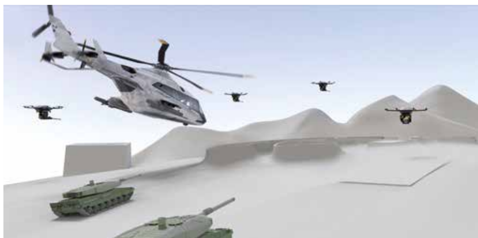
▲ A conceptual image published by Airbus when it was selected for an NGRC Concept Study Five contract in July 2024 depicted a rotorcraft with a main rotor and twin lateral propellers accompanied by armed rotary-wing UAVs. [Airbus]
