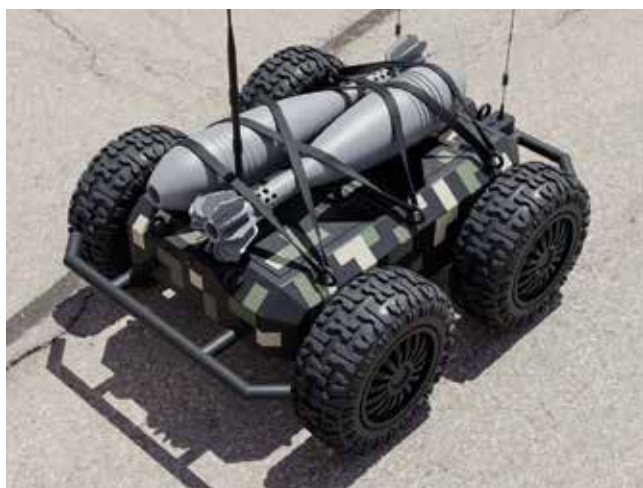
▲ As this Ukrainian Ratel-3 unmanned ground vehicle demonstrates, off-the-shelf ordnance can be mounted in an improvised manner. [Brave1]
