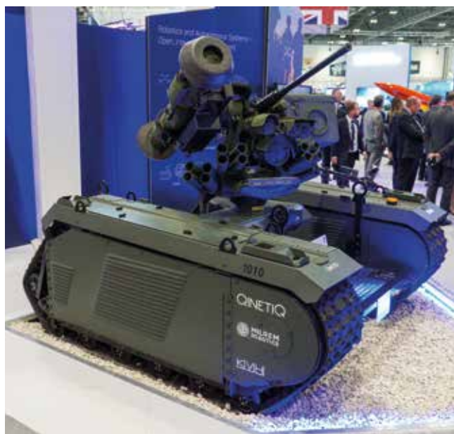
▲ A TheMIS UGV fitted with remote weapon station (RWS) with FGM-148 Javelin. [RecoMonkey]
