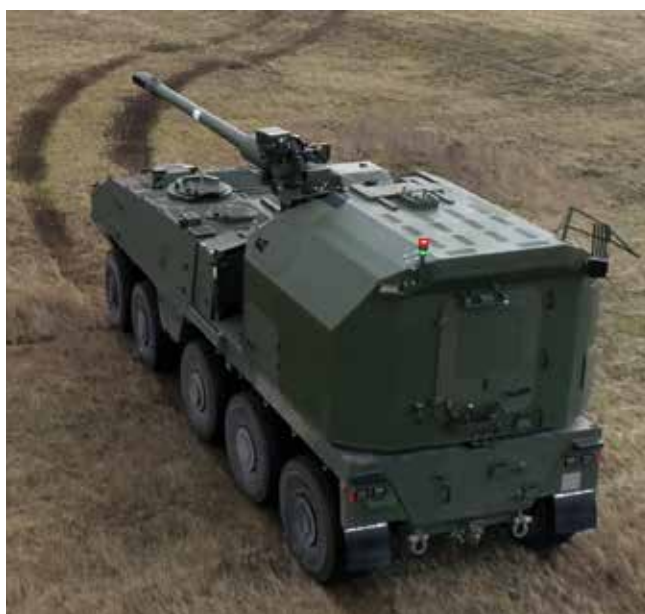
▲ Pictured: Piranha IV HMC 10x10 with KNDS' AGM module. Compared to their tracked counterparts, wheeled SPA will be lighter, but they will also be narrower and taller. [GDELS]
