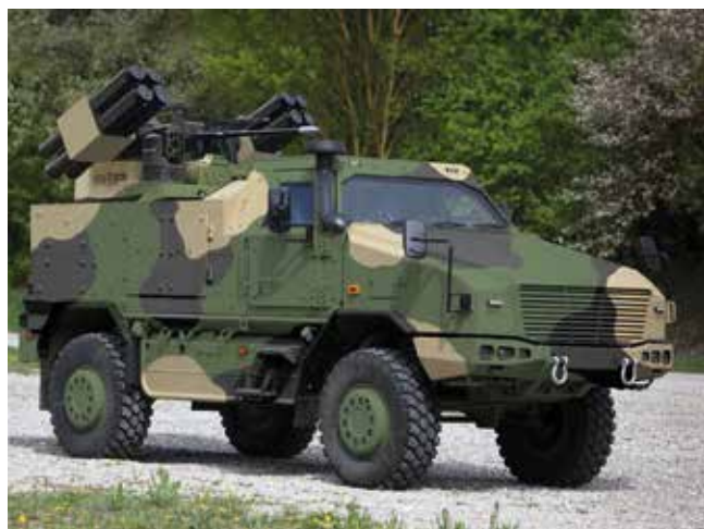
▲ A DINGO 3 protected vehicle fitted with Moog's R1wP turret in VSHORAD configuration [KNDS Deutschland]
