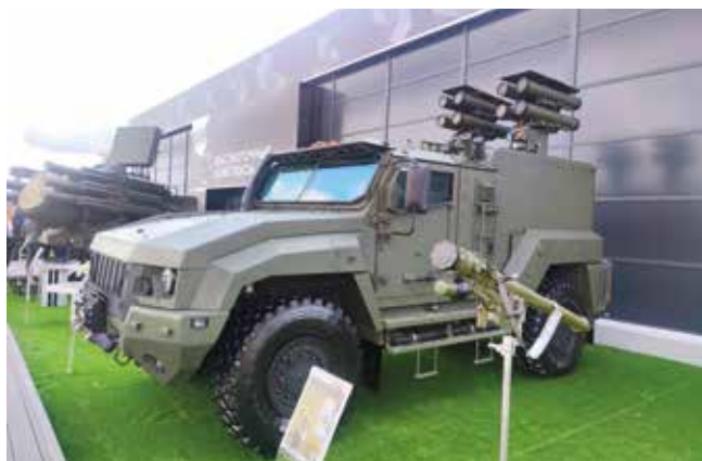
▲ 9P163-3 Kornet-EM vehicle, shown with Kornet quad-launchers deployed. This version displayed at the Armiya-2024 exhibition is based on the Remdizel K-53949 Taifun-K 4x4 platform. [Alexey Tarasov]
