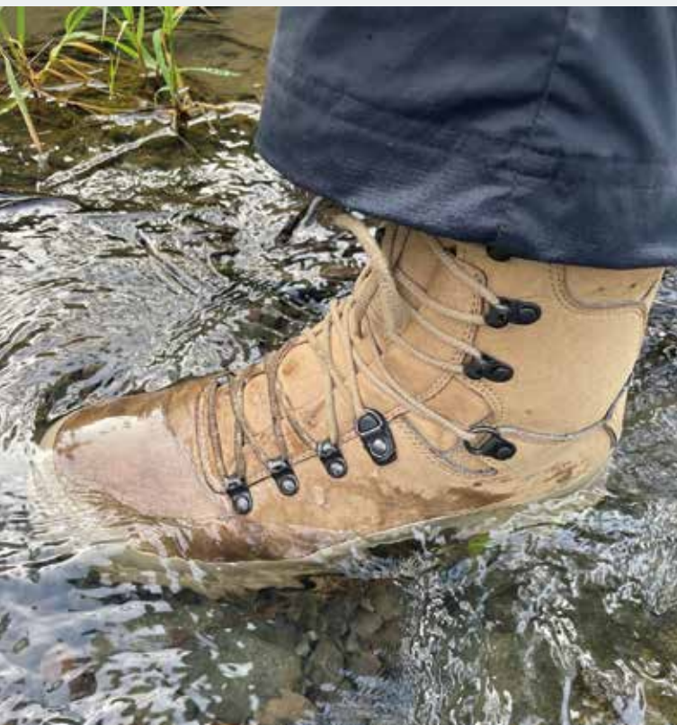
▲ Meindl combat boot in the water test. One advantage is said to be the lower moisture absorption. [André Forkert]
