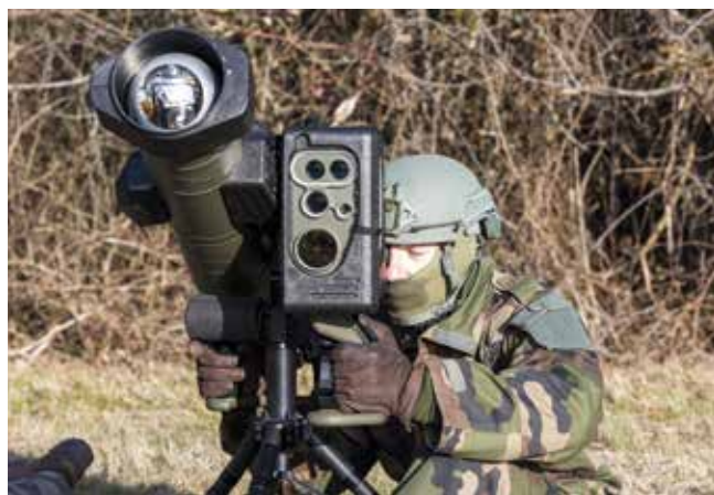
▲ Front view of MBDA's Akeron MP ATGM, showing the dual-band (Day TV and IIR) seeker. At Bourges, on 26 January 2017. [MBDA/Laurent Guichardon]
