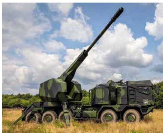
▲ RMMV's SPA offering, known officially as the WASD (Wheeled Artillery System Demonstrator) is shown here with the 'Artillery Turret Interface (ATI)' outrigger stabilisers engineered by Supashock of Australia. The latest WASD prototype, scheduled to commence live fire testing shortly, will have an ATI developed by Elbit Systems, similar to that fitted to the Oshkosh-based Elbit SIGMA/Roem. [RMMV]
