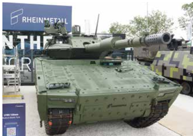
▲ A combat vehicle marketed as Lynx 120 mm medium battle tank unveiled at Eurosatory 2024. A HITFACT MkII turret fitted on a KF41 medium-tracked platform. [RecoMonkey]
