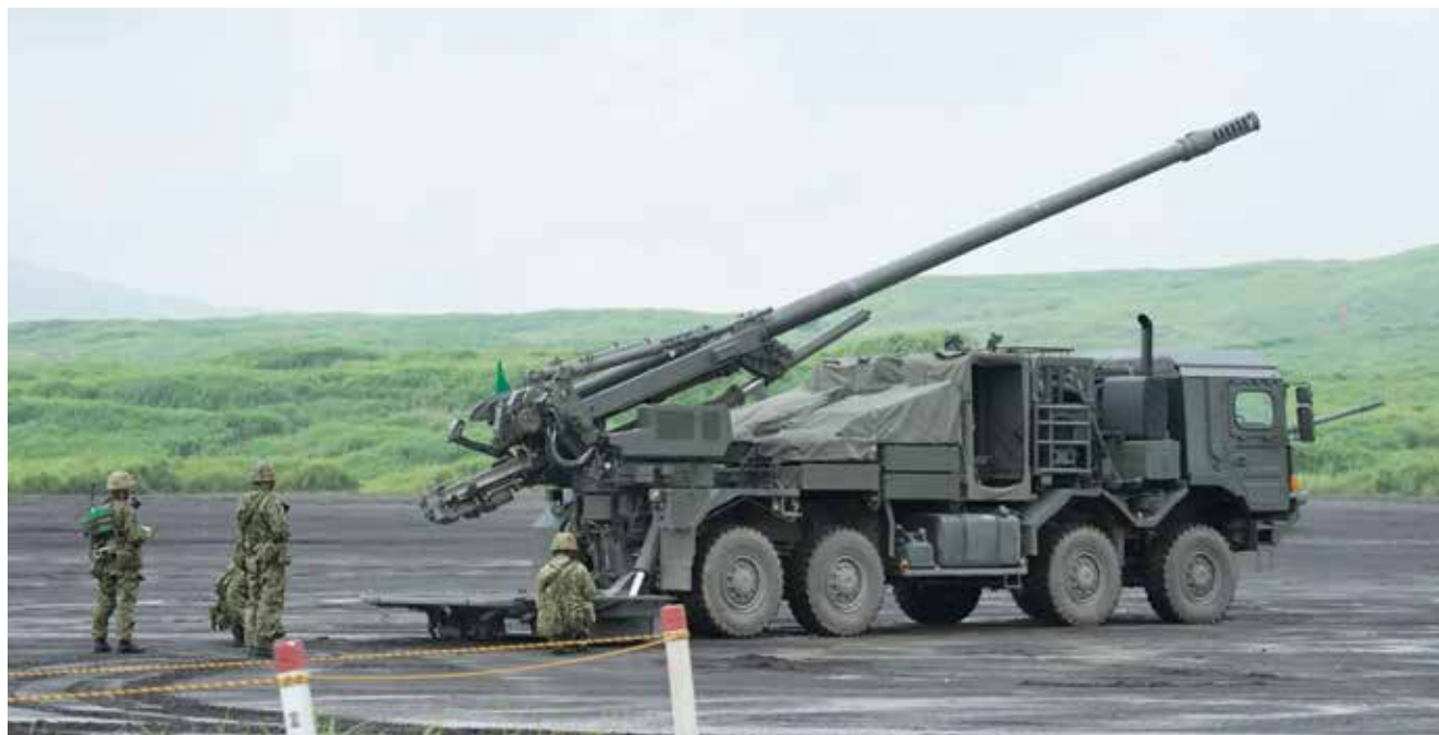
▲ Pictured: Type 19 155 mm SPH of the Japanese Ground Self-Defense Force. Most but not all wheeled SPA being adopted by top-tier armed forces feature enclosed and automated ordnance and a ballistically-protected cab for the crew. [JGSDF]
