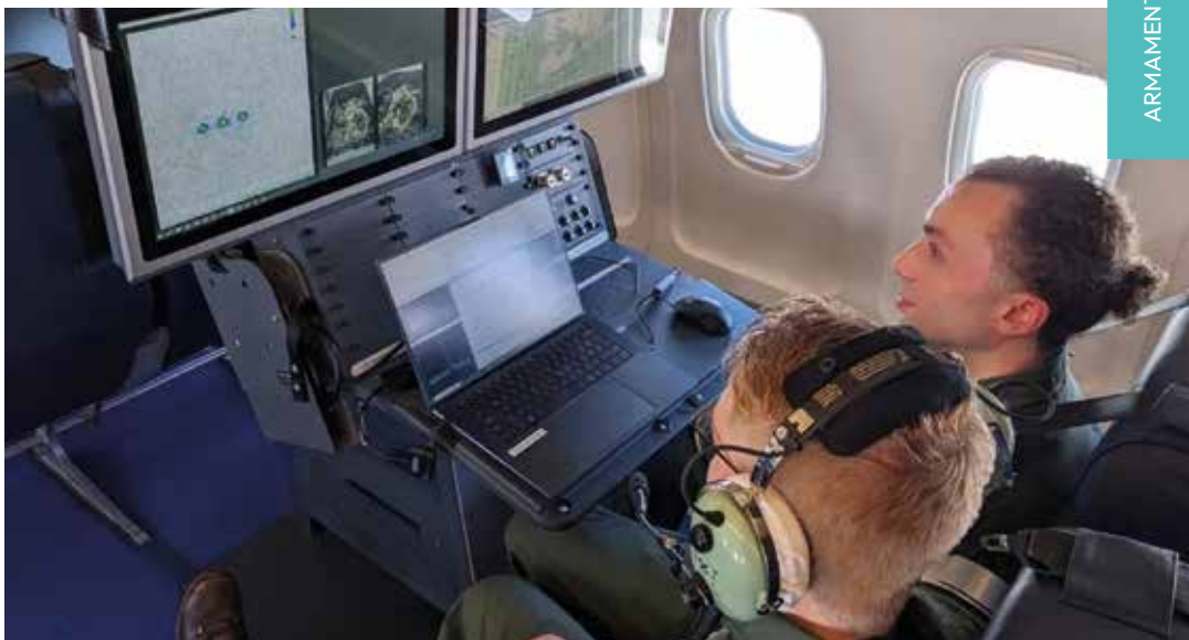
▲ In May 2024, QinetiQ conducted flight tests of an experimental quantum-inertial system. When fully developed, this technology will eliminate the gradual build-up of errors experienced with electro-mechanical inertial navigation hardware. [QinetiQ]
