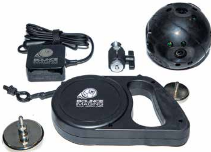
▲ The Recce 360 throwable sensor and accessories. [Bounce Imaging]
