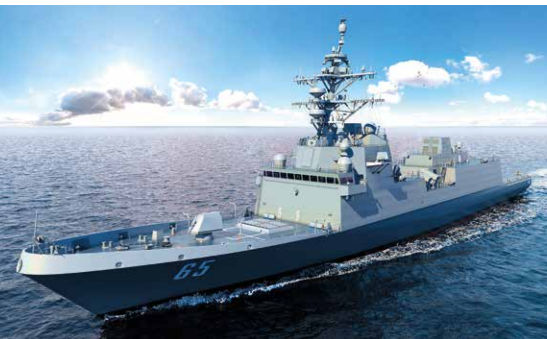
▲ An artist's rendering, published in 2023, of a US Navy FFG-62 Constellation class frigate. These future frigates bring an ASW suite integrated around and into the Navy's Aegis combat system. [US Navy]
