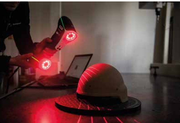
▲ Pictured: Helmet scanning during the manufacturing process; advanced methods and processes ensure optimum ballistic protection levels are achieved from latest materials and designs. [NP Aerospace]
