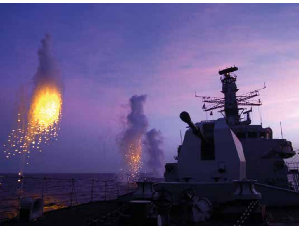
▲ A Mk 245 IR seduction round being fired from a RN Type 23 frigate. The Mk 245 deploys a series of sub-munitions in a 'walk-off' pattern. [Crown Copyright]
