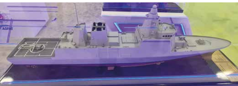
◆ A model of the TF-2000 air defence destroyer. She carries a total of 96 VLS cells located forward and amidships. Her multifunction radar arrays are split between the forward and aft superstructure/masts. [Devrim Yaylali]
