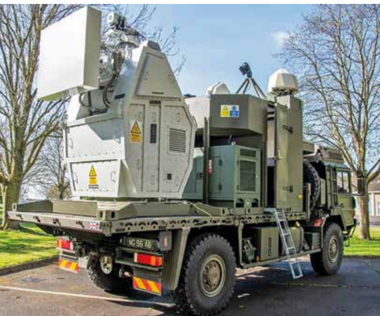
▲ The 'RapidDestroyer' HPM system on an RMMV HX60 4x4 truck platform during British Army trials. [UK MoD]
