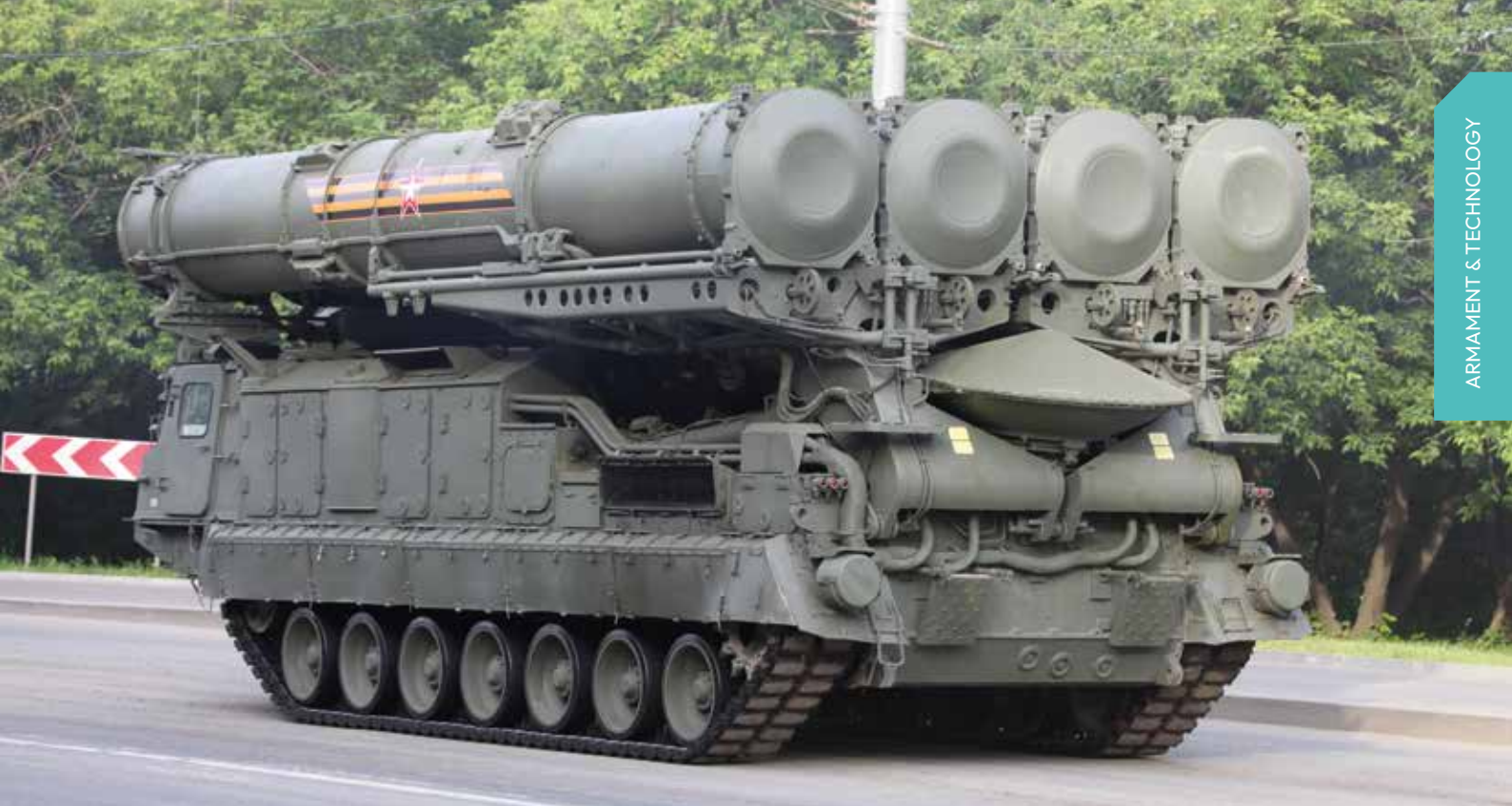
▲ A 9A83M transporter, erector, launcher, and radar (TELAR) of the S-300V4 system. The continuous wave illumination radar for the track-via-missile (TVM) guidance system can be seen folded over the rear deck, under the missile containers. [RecoMonkey]
